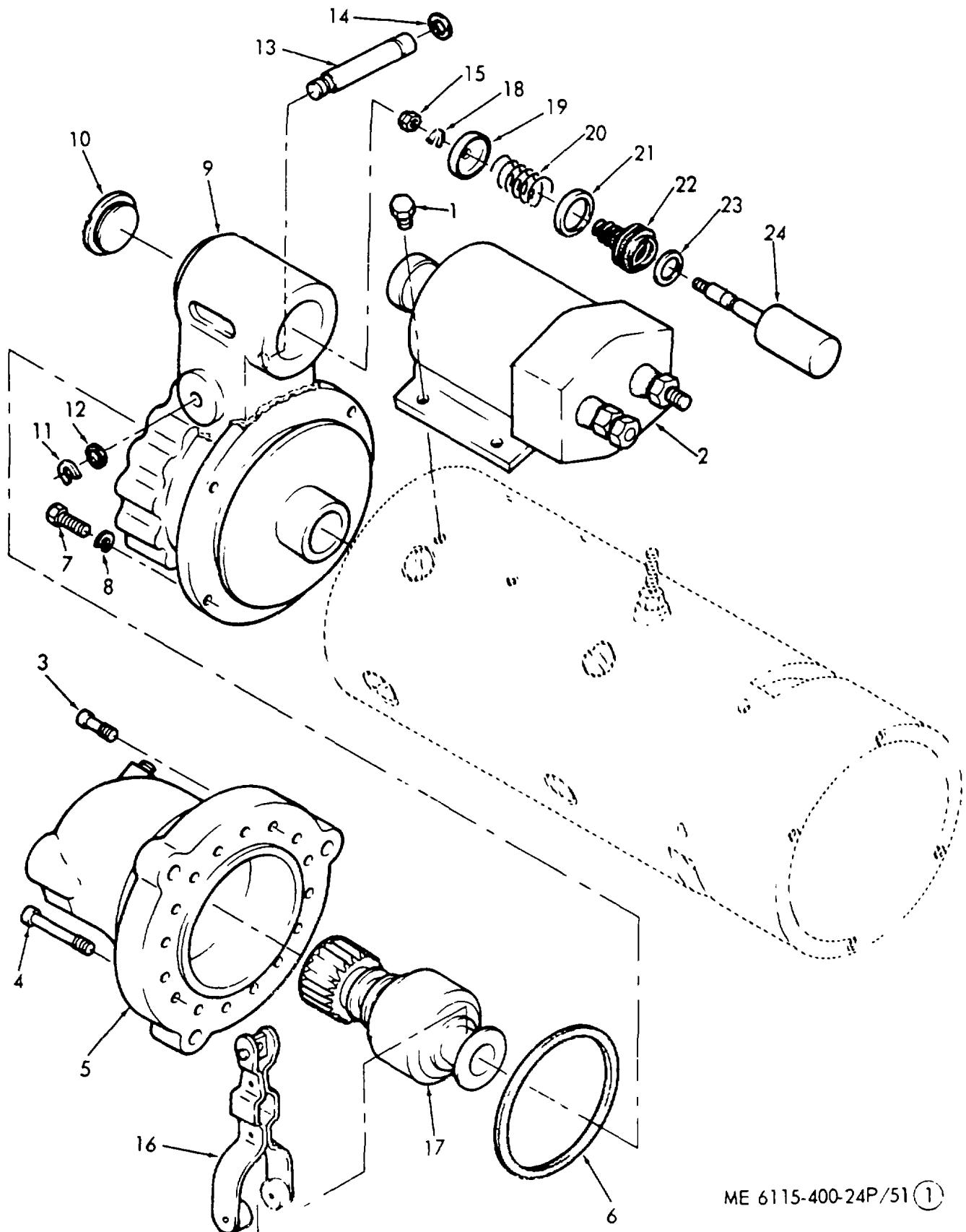
Figure 51. Engine Starting Motor (Sheet 1 of 2).
