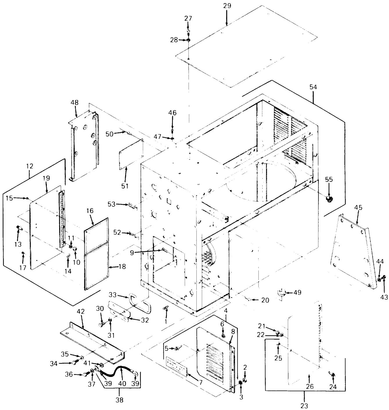
Figure 9. Heater Case Assembly
