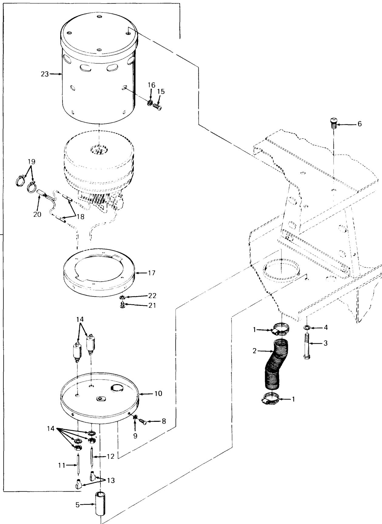
Figure 14. Combustion Blower and Housing
