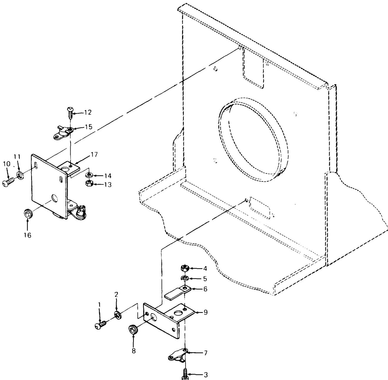
Figure 13. Thermostat and Flame Switch Assemblies
