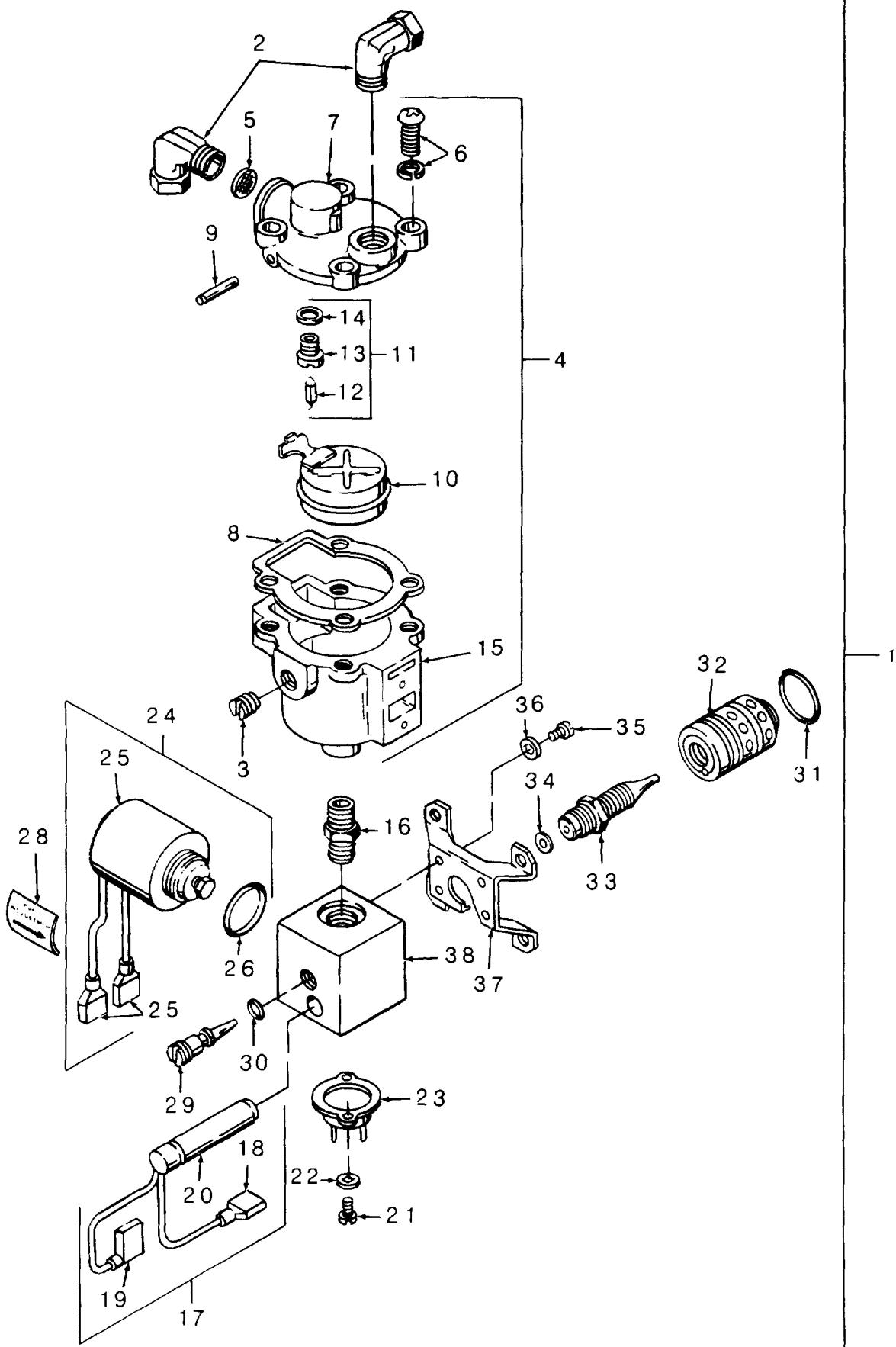
Figure 12. Carburetor Assembly
