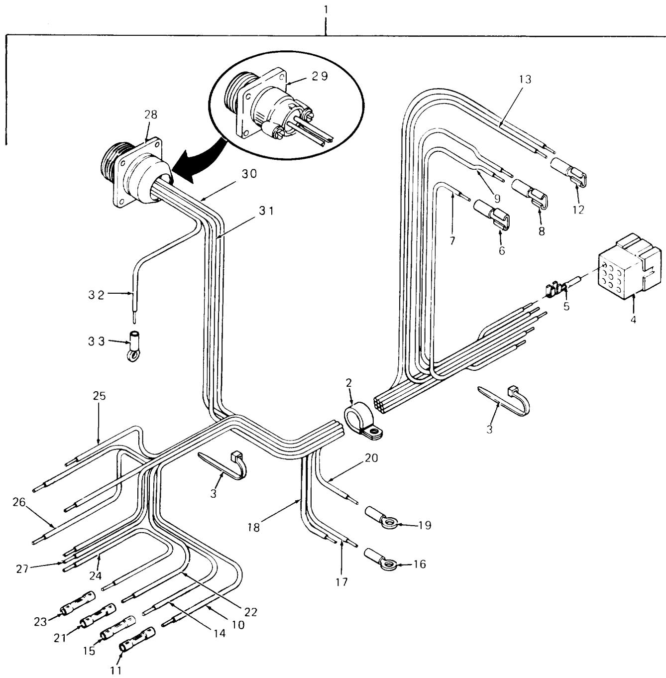
Figure 5. Control Box Harness Assembly
