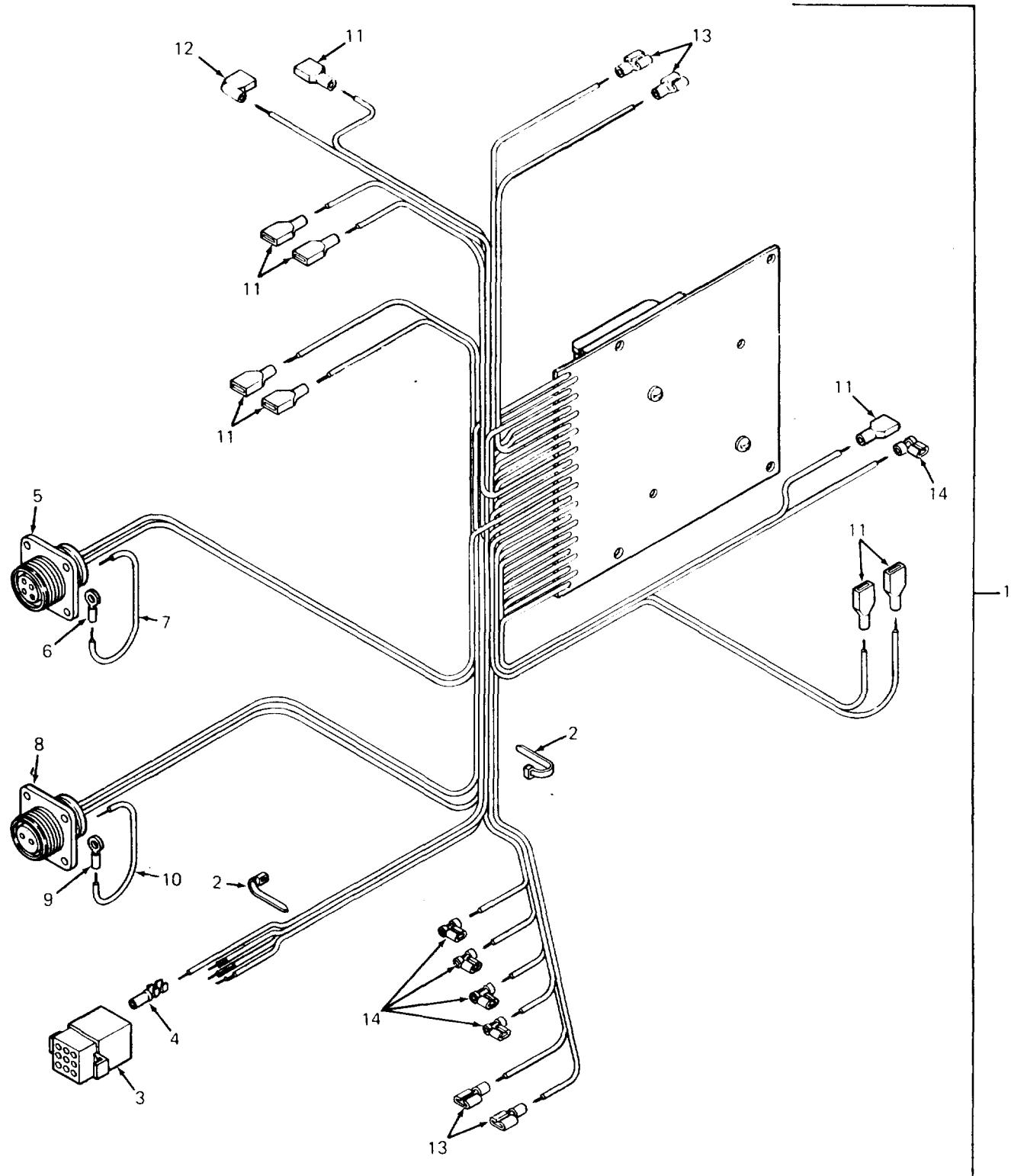
Figure 2. P.C. Board Assembly, Model UH-68G
