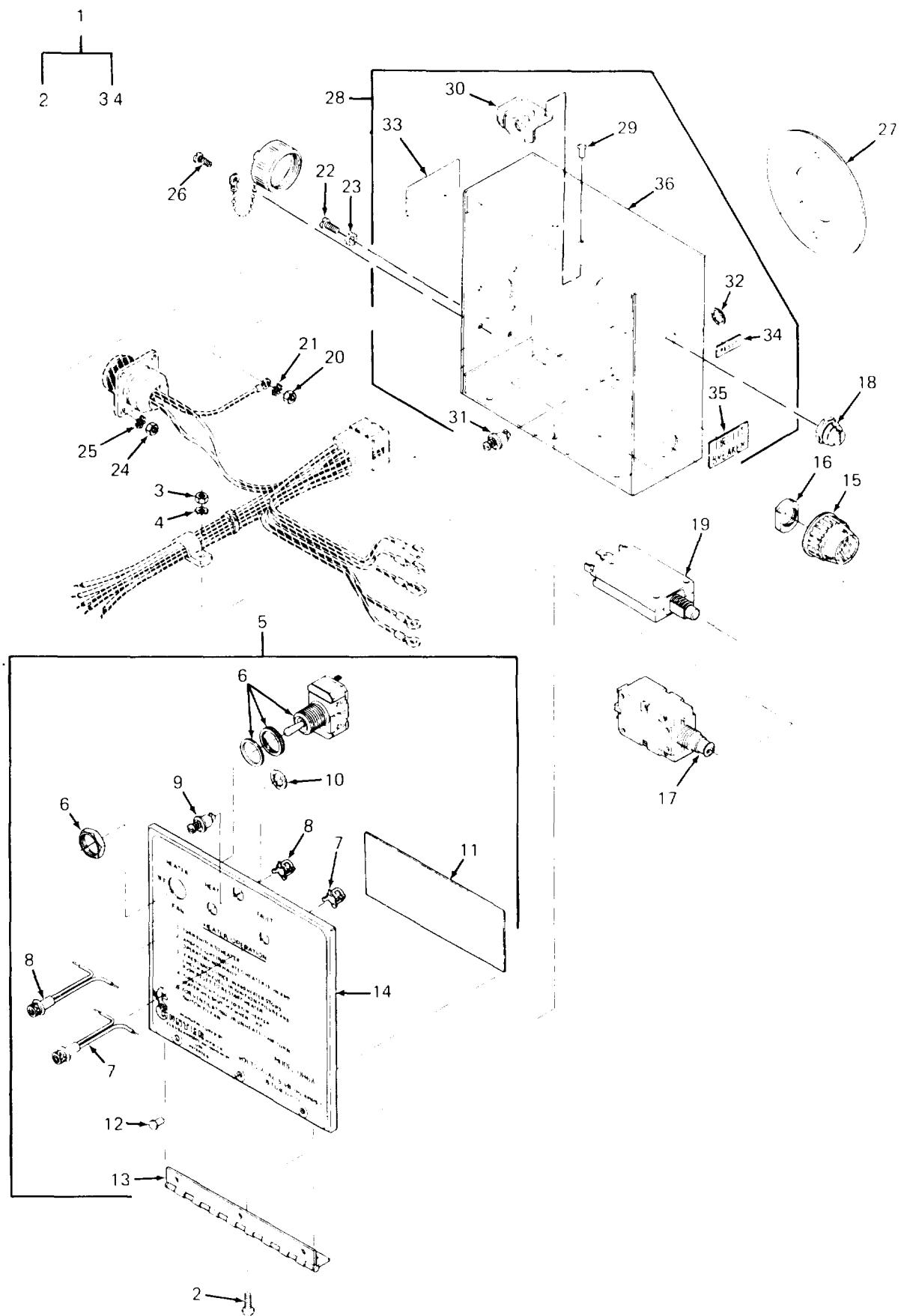
Figure 4. Control Box Assembly
