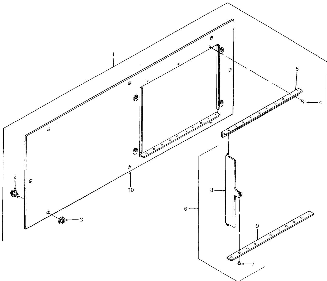
*Figure 7. Right Hand Louver Panel Assembly*
