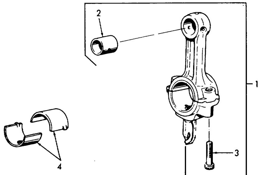
Figure 14. Connecting Rod.
