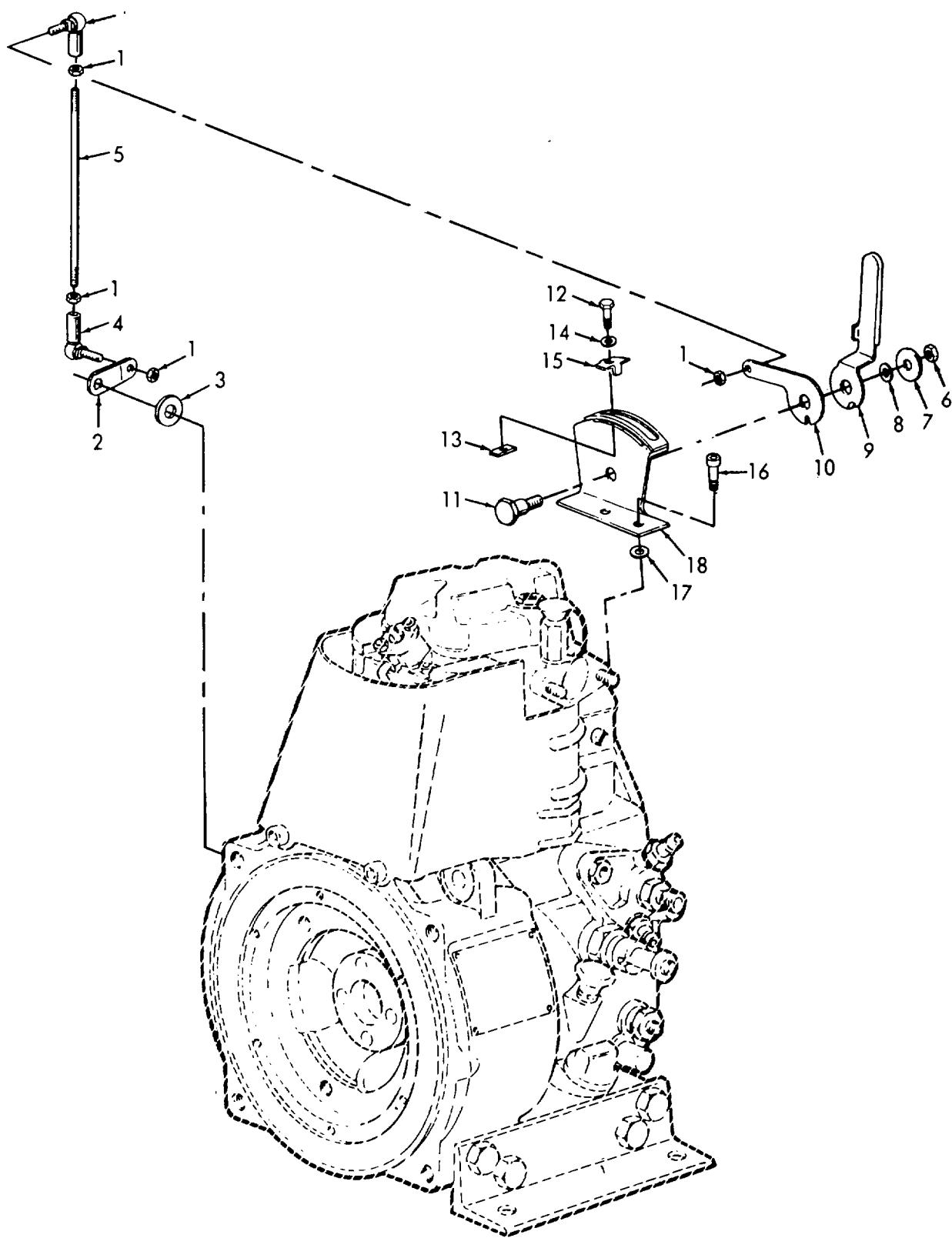
Figure 8. Throttle Controls.
