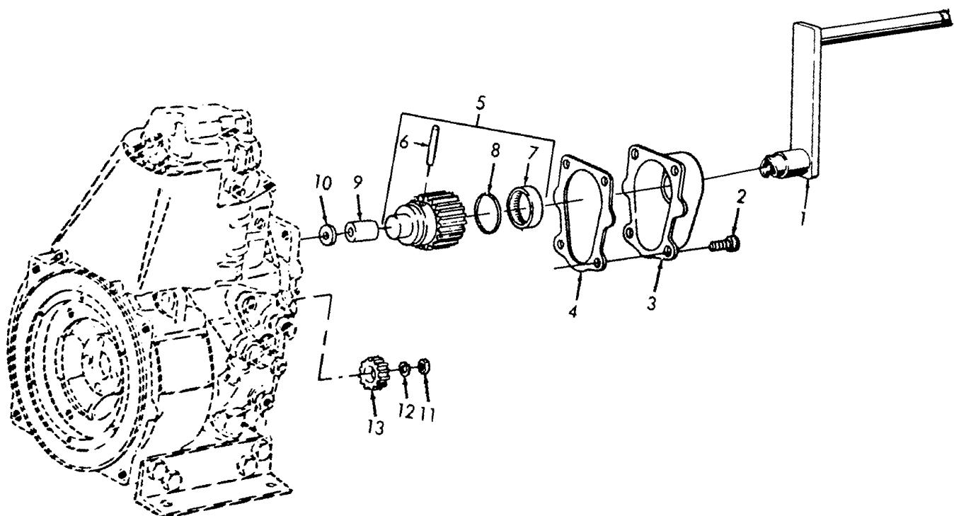
Figure 9. Crank Assembly, Cover and Gears.
