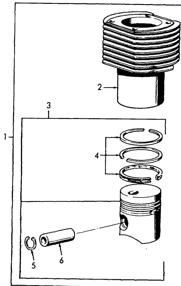
Figure 13. Cylinder and Piston.
