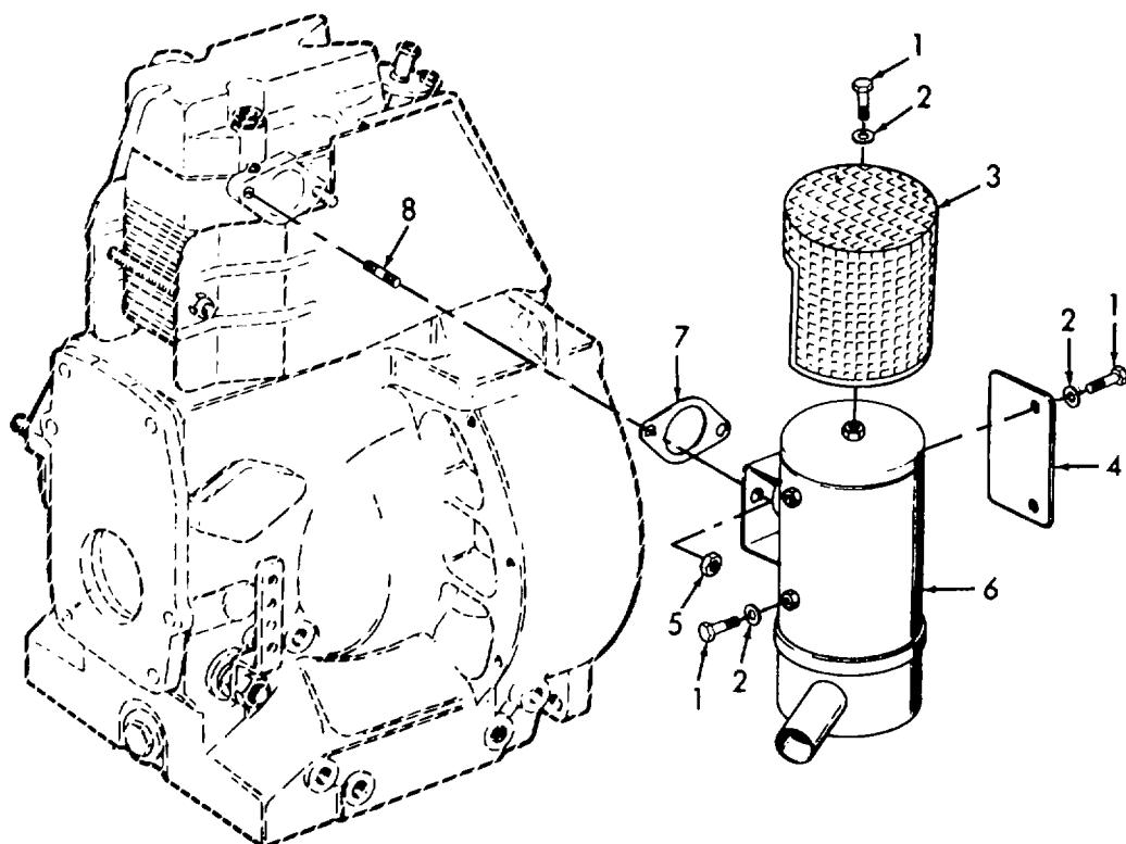
Figure 7. Muffler and Guard.
