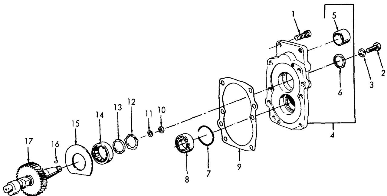
Figure 15. Timing Cover and Camshaft.
