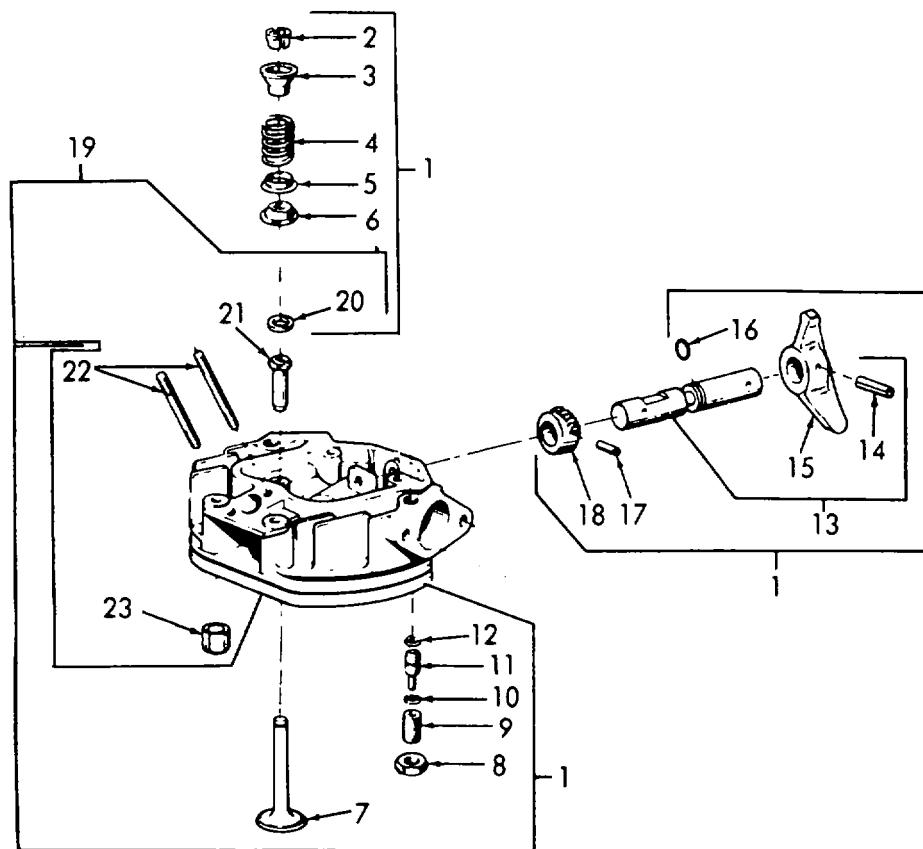
Figure 12. Cylinder Head and Valve Assembly.
