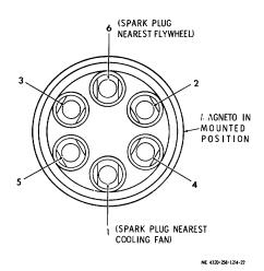
Figure 4-22. Magneto-to-spark plug connections.
