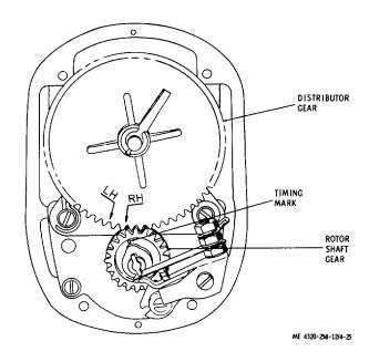
Figure 4-25. Distributor gear properly alined with rotor shaft gear.
