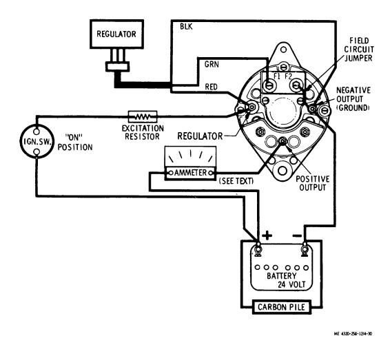
Figure 4-30. Alternator output and system test setup.
