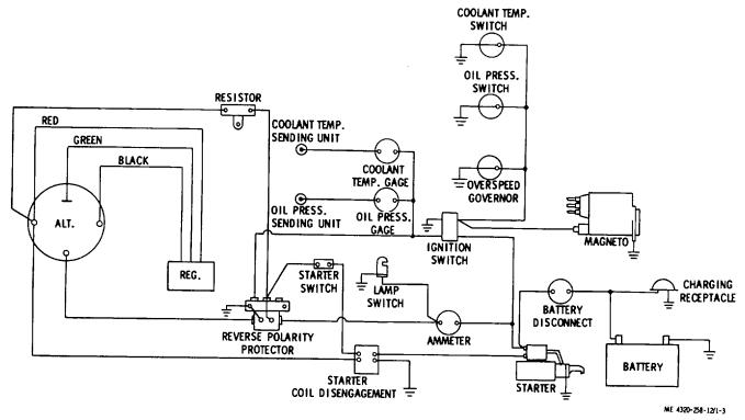
Figure 1-3. Engine wiring diagram.
