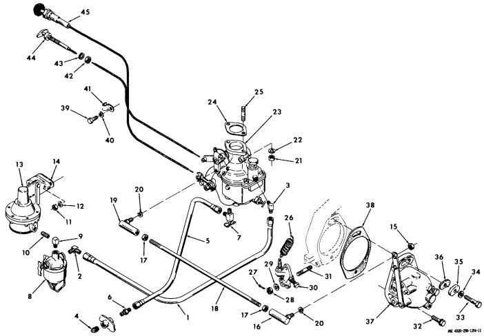
Figure 4-11. Fuel system components, exploded view.
