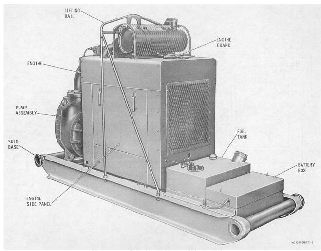
Figure 1-2. Centrifugal pump, right rear view.
