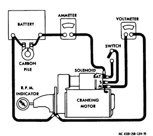
Figure 4-35. Engine starter test setup.
