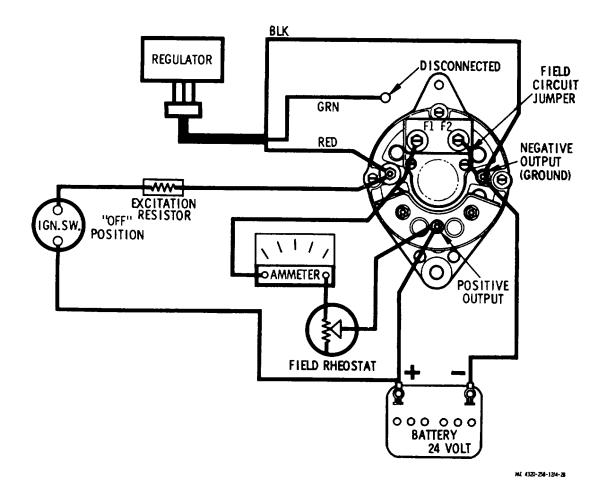
Figure 4-28. Field current draw test setup.
