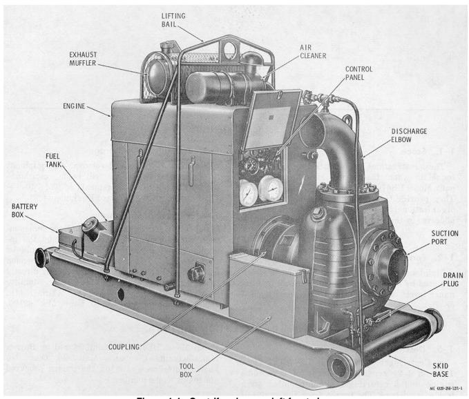
Figure 1-1. Centrifugal pump, left front view.
