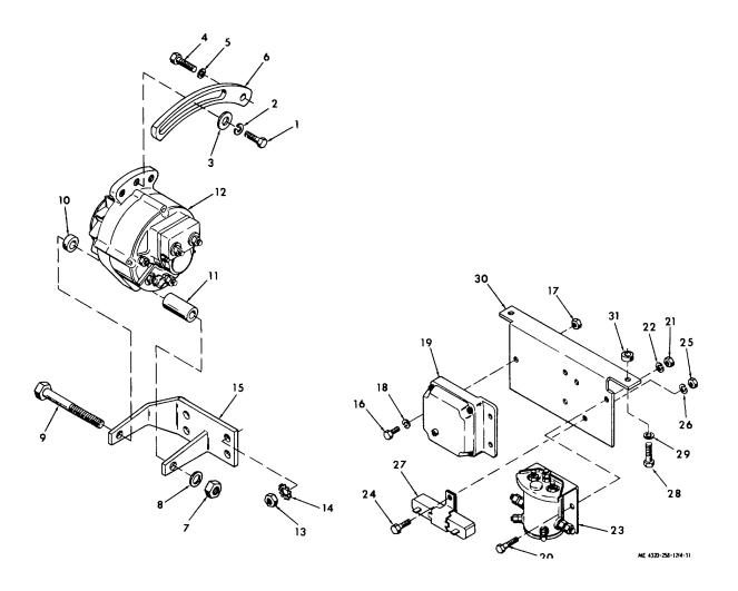
1. Adjusting screw 12. Alternator 22. Lock washer 2. Lock washer 13. Nut 23. Reverse polarity protector Cap screw 3. Flatwasher 14. Lock washer 24. 4. Strap mounting screw 15. Alternator mounting bracket 26. Nut 5. Lock washer 16. Cap screw 26. Lock washer 6. Adjusting strap 17. 27. **Excitation resistor** Nut 7. Nut 18. Lock washer 28. Cap screw 8. Flat washer Voltage regulator 29. Lock washer 19. Bolt Cap screw Mounting bracket 20. 30. 10. Spacer 21. Nut 31. Spacer 11. Spacer
