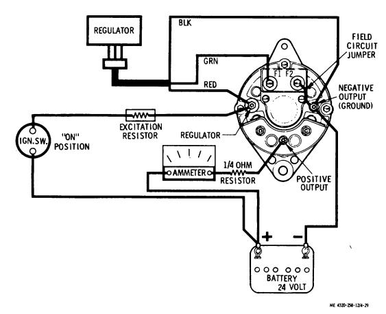
Figure 4-29. Voltage regulator operating voltage test setup.
