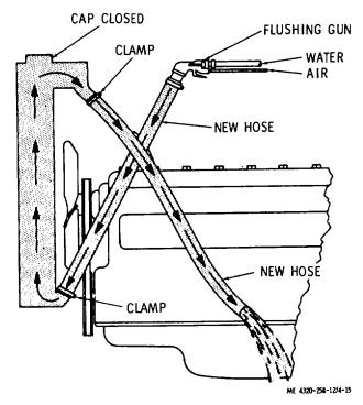
Figure 4-15. Reverse-flushing the radiator.
