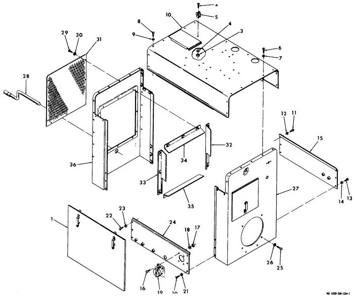
Figure 4-7. Engine housing, exploded view
