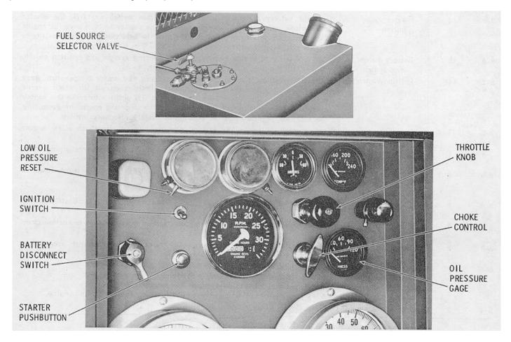
STEP 1. PLACE FUEL SOURCE SELECTOR VALVE TO TANK OR AUXILIARY, WHICHEVER IS APPLICABLE.
