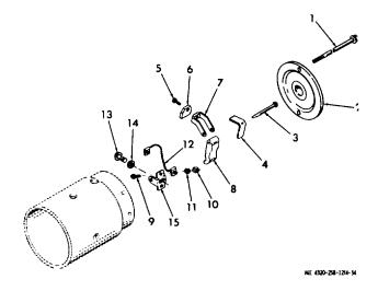
Thru bolt 1. 8. Insulated brush Commutator end holder frame 9. Brush lead screw Support pin 10. Nut Brush spring 11. Lock washer Brush screw 5. 12. Grounded brush lead Brush 13. Brush support screw 6. 7. Grounded brush 14. Washer
