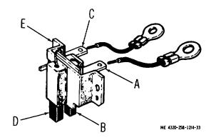
Figure 4-33. Alternator brush assembly, showing continuity paths.
