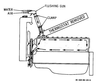
Figure 4-16. Reverse-flushing tee engine block.
