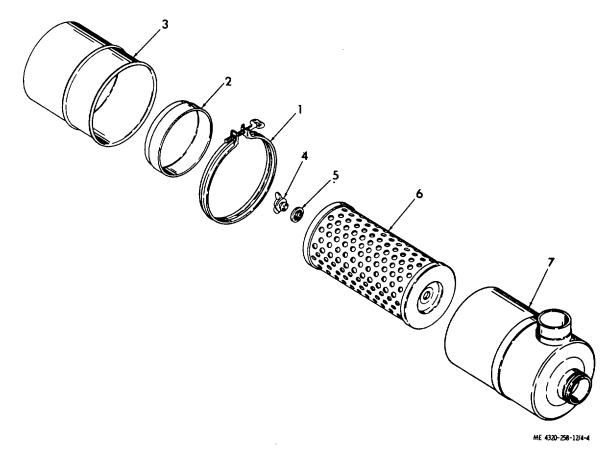
Figure 4-4. Air cleaner, exploded view.
