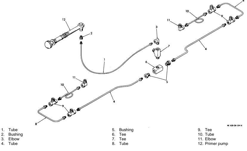
Figure 4-14. Primer pump, lines, and fittings, exploded view.
