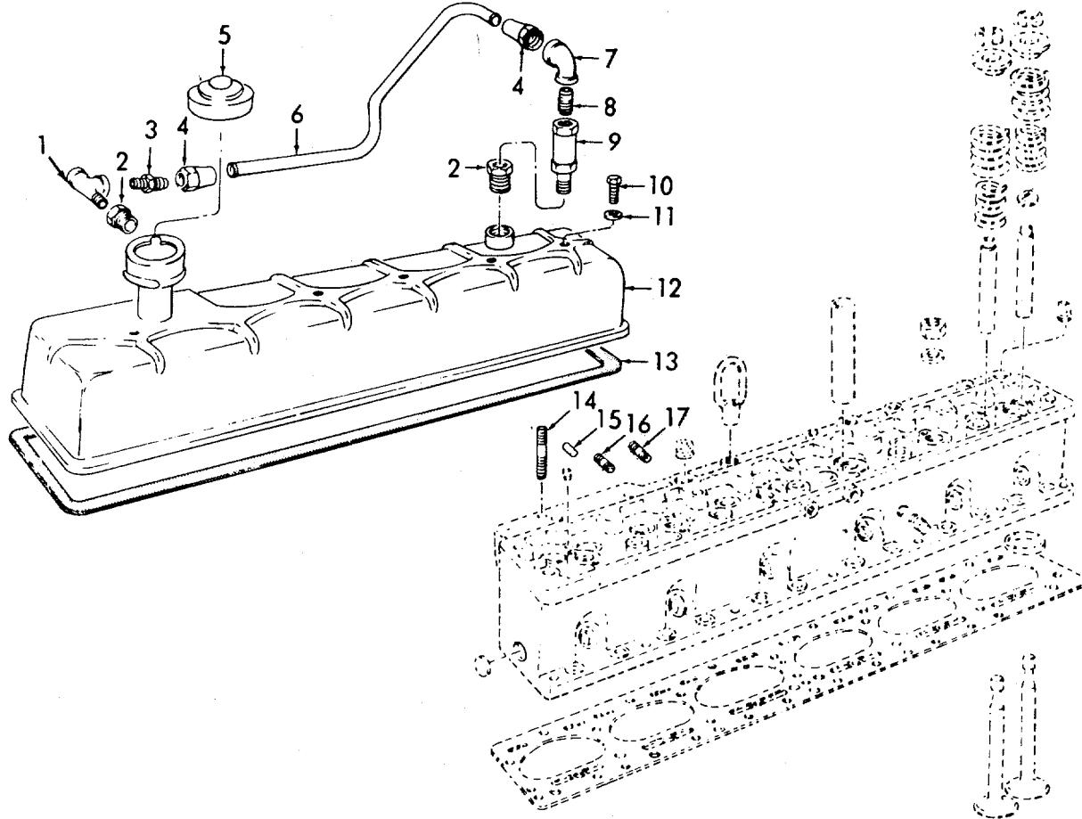
**Figure 2. Cylinder Head Cover.
