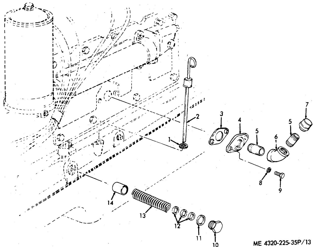
**Figure 5. Oil Relief Valve, Filler and Gage.
