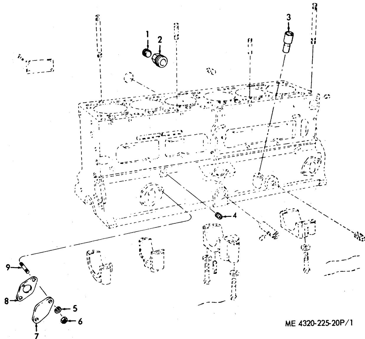
**Figure 1. Fuel Pump Hole Cover and Plugs.**
