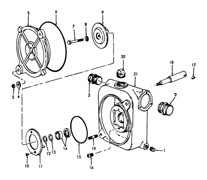
Figure 4-3. Pump, disassembly and reassembly.
