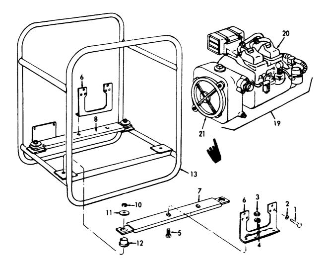
Figure D-1 Engine Assembly
