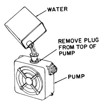
Figure 2-3. Priming the pump.
