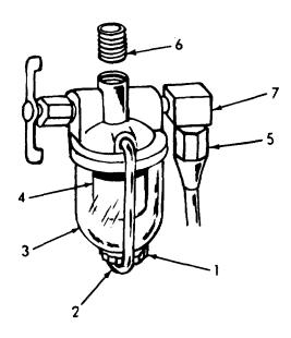
Figure 4-2. Fuel line and filter removal.
