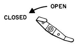
2 - Turn Fuel Shut off valve to OPEN.
