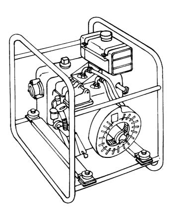
Figure 1-1. Centrifugal pump
