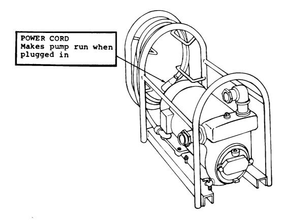
Figure 2-2. Operating Controls (Electric Motor Driven Pump).
