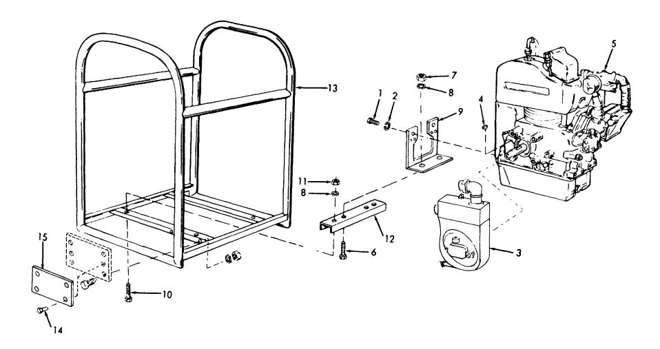
Figure D-1. Engine, Support and Carrying Frame.
