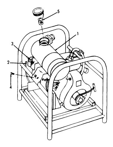
Figure 4-1. Fuel Tank Removal.
