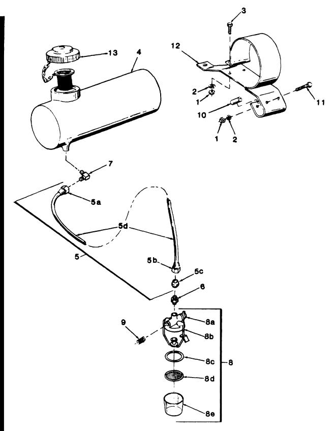
Figure D-2. Fuel Tank Lines and Fittings
