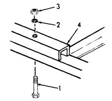
Figure 4-3. Channel Removal.
