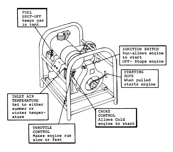
Figure 2-1. Operating Controls (Gasoline Engine Driven Pump)
