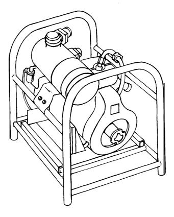
Figure 1-1. Centrifugal Pump (Gasoline Engine Powered)
