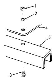
Figure 4-6. Electric Motor Removal.
