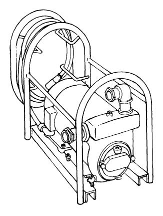
Figure 1-2. Centrifugal Pump (Electric Motor Powered Typical)
