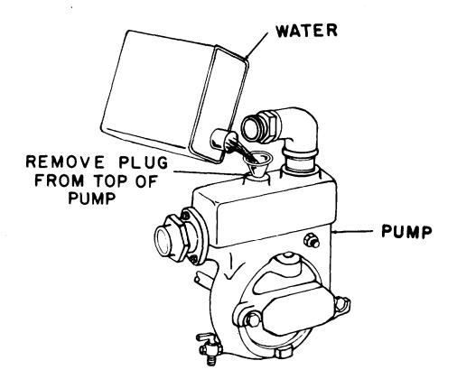
Figure 2-4. Priming the pump.
