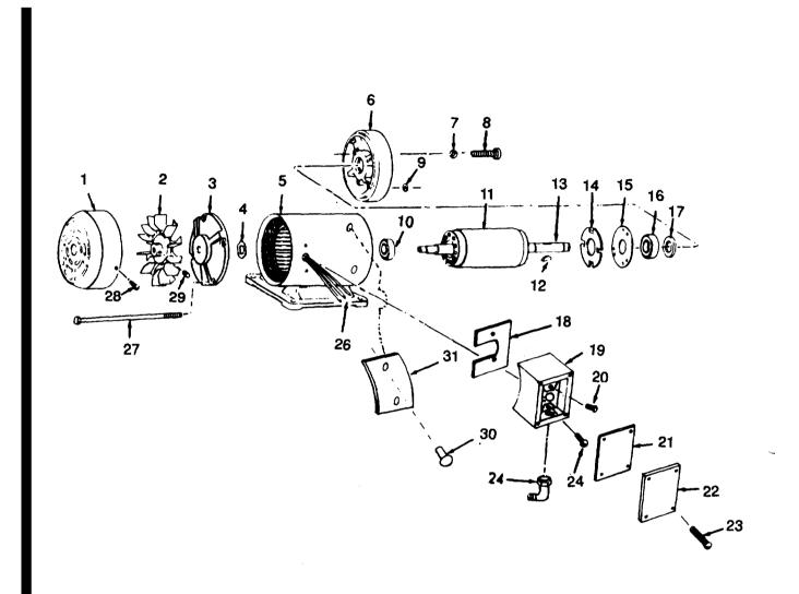
Figure D-5. Electric Motor.
