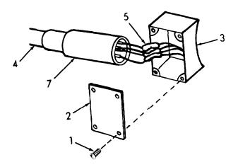
Figure 4-5. Power Cable Replacement (Electric Motor Driven Pump).
