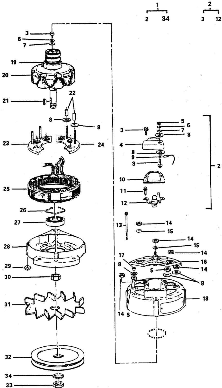
Figure 6. Alternator Assembly.
