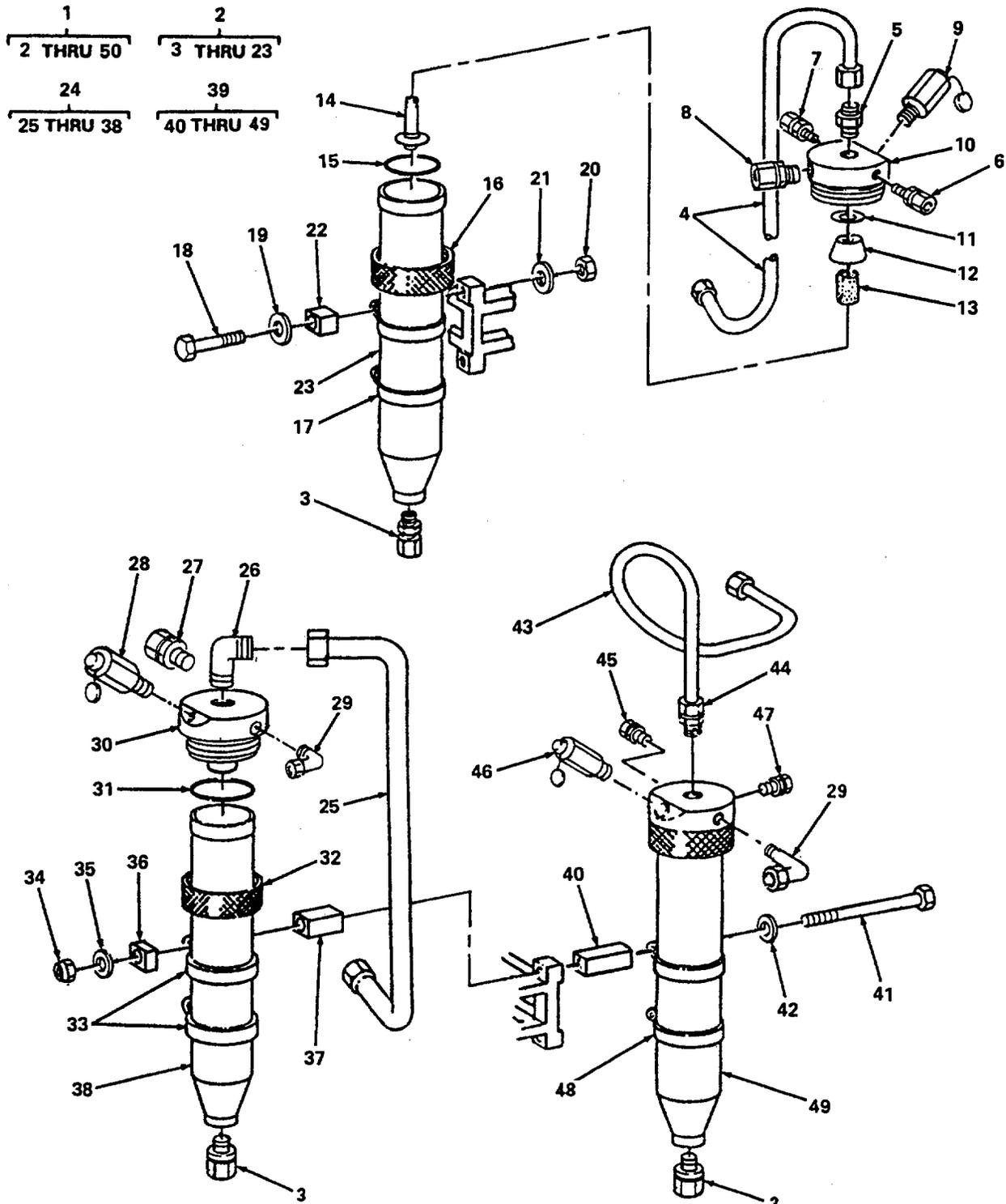
Figure 40. Compressor Interfilter and Safety Valves.
