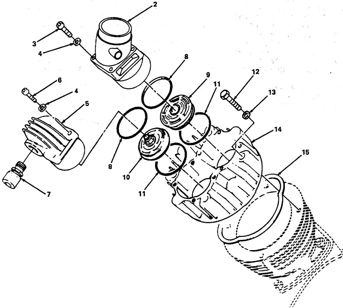
Figure 33. Compressor First Stage Valve and Head Assembly.
