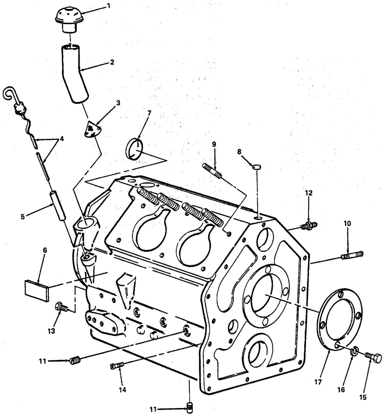
Figure 26. Crankcase Assembly.
