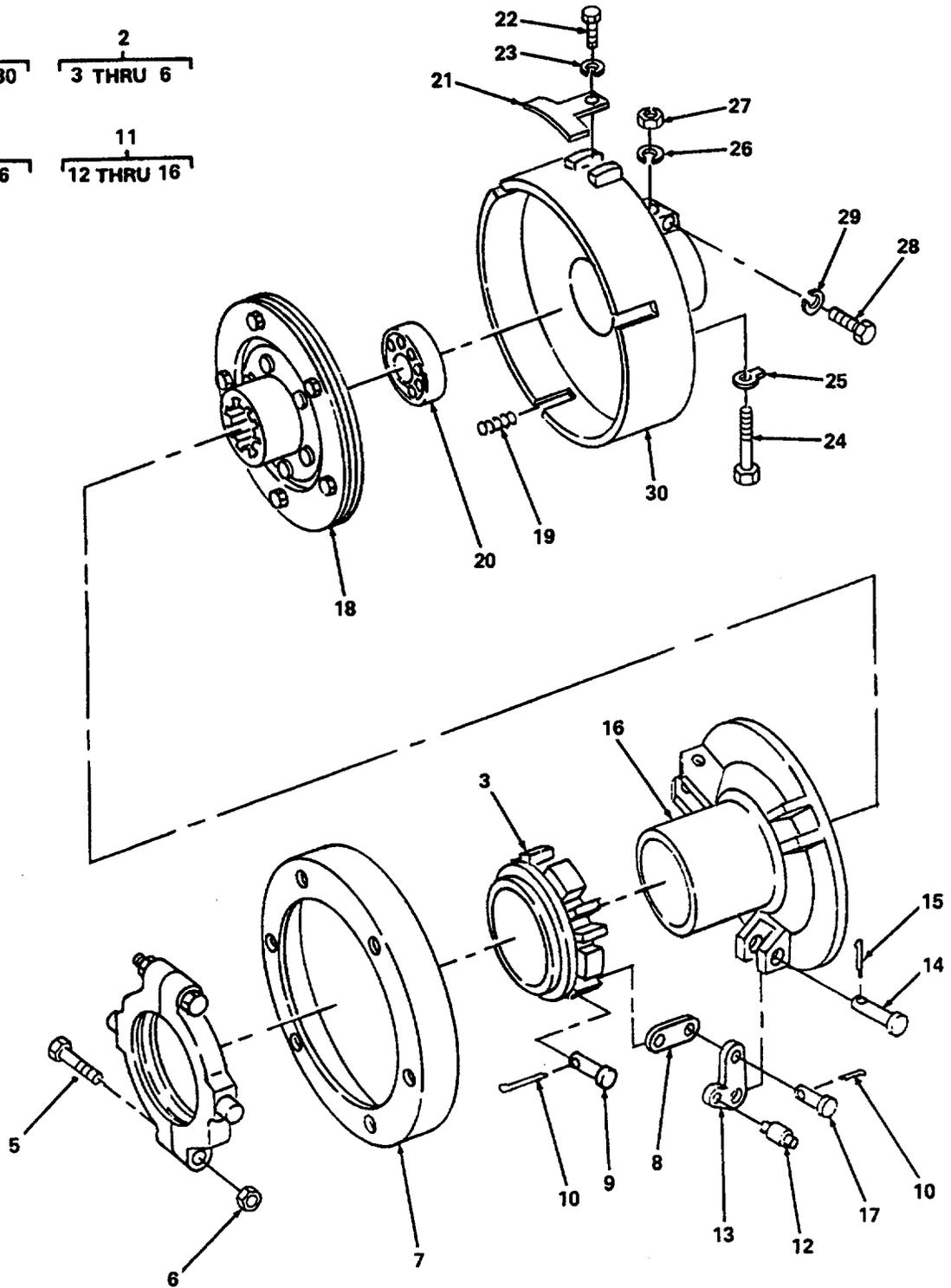
Figure 31. Clutch Assembly.
