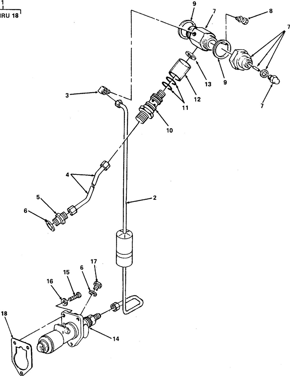
Figure 39. Compressor Lubricating Oil Pump.
