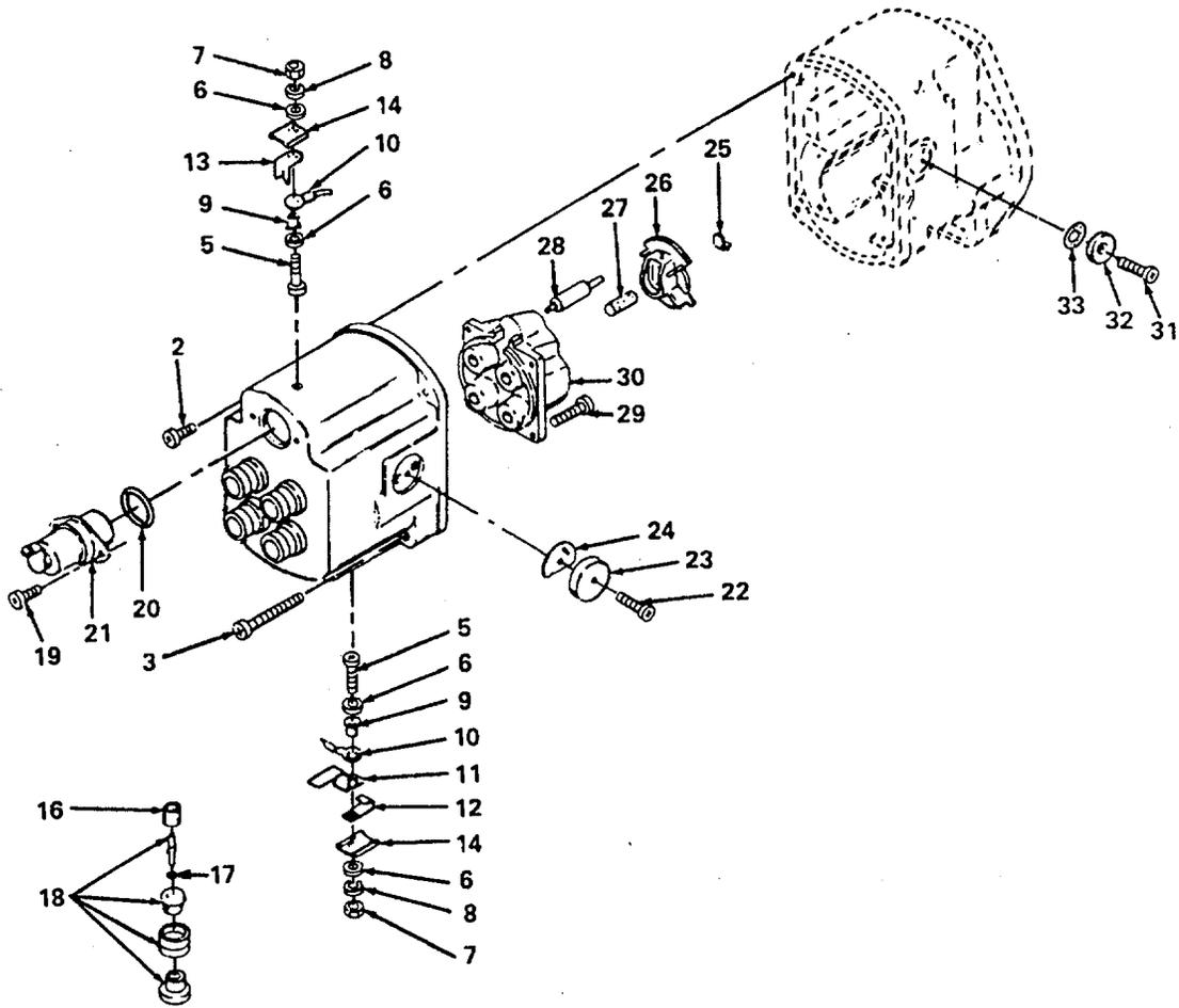
Figure 10. Magneto (Sheet 1 of 2).
