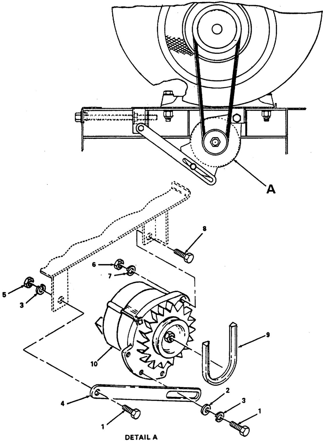
Figure 5. Alternator Mounting.
