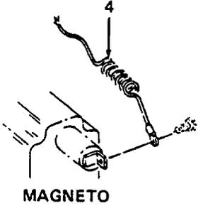
Figure 16. High Temperature Switch Assembly.
