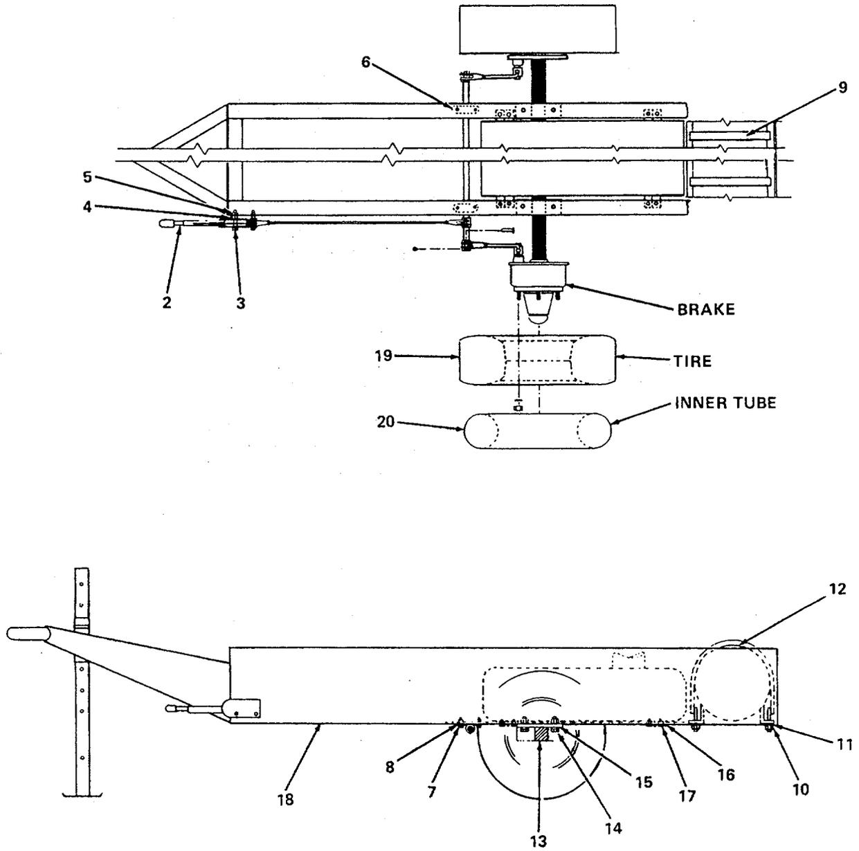
Figure 50. Chassis Assembly.
