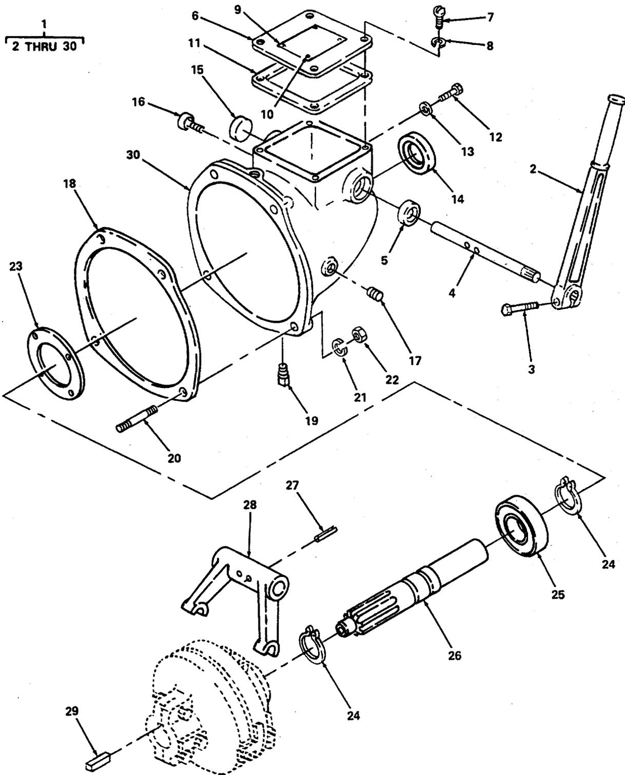
Figure 30. Clutch Take-Off Assembly.
