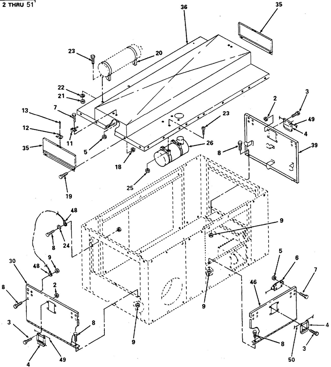
Figure 3. Enclosure Assembly (Sheet 1 of 2).
