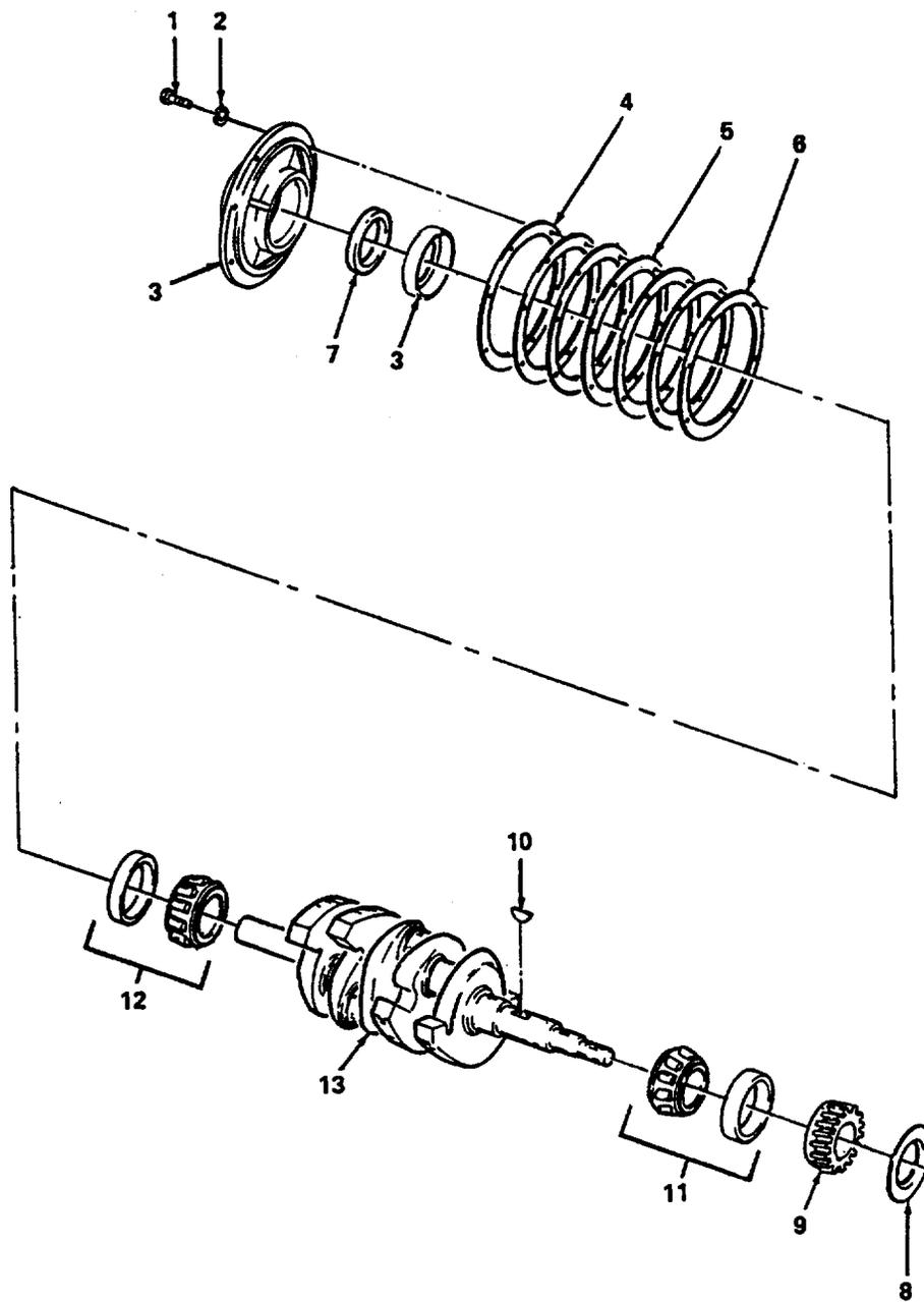
Figure 25. Crankshaft Assembly.
