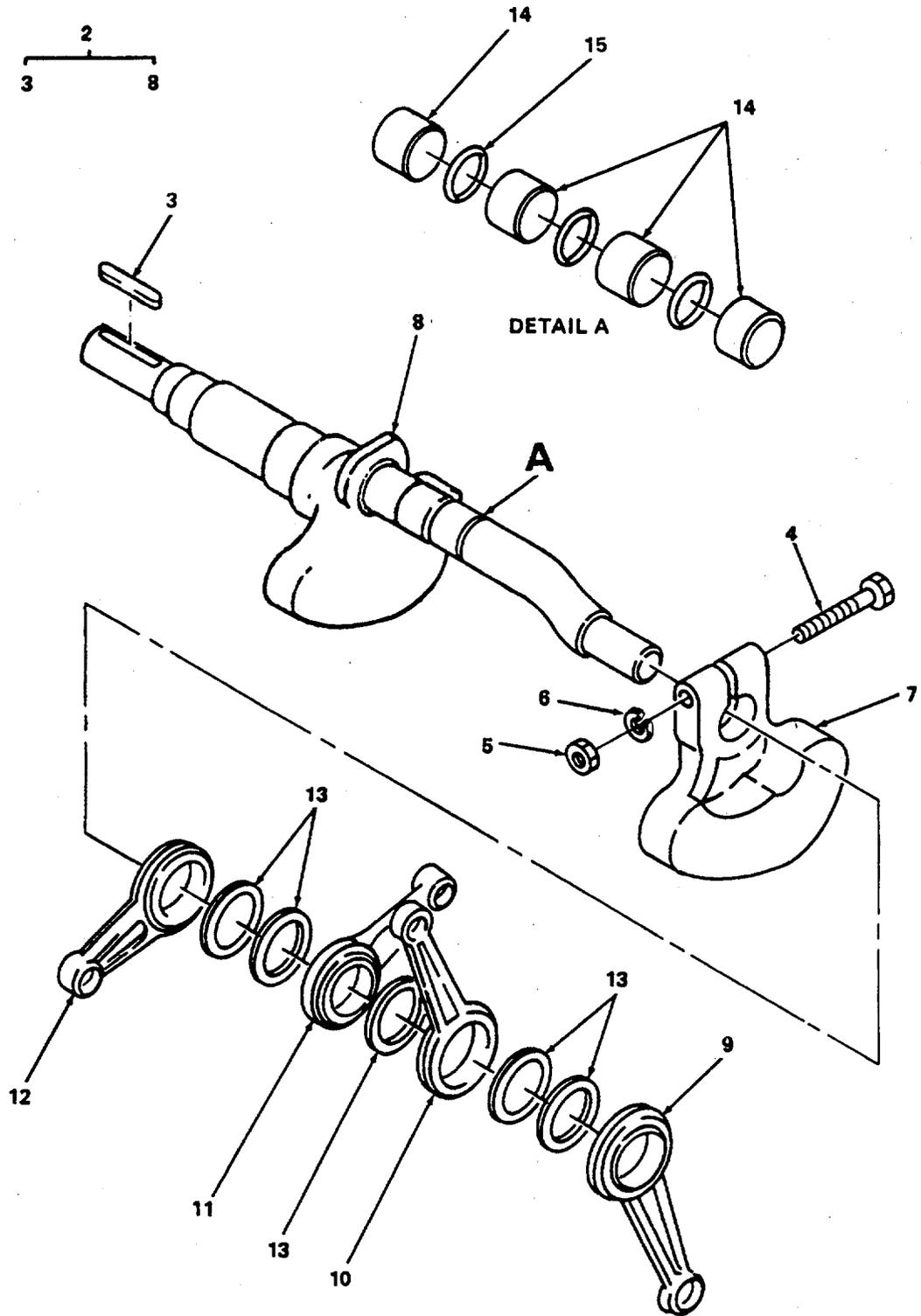
Figure 38. Crankcase and Connecting Rods.
