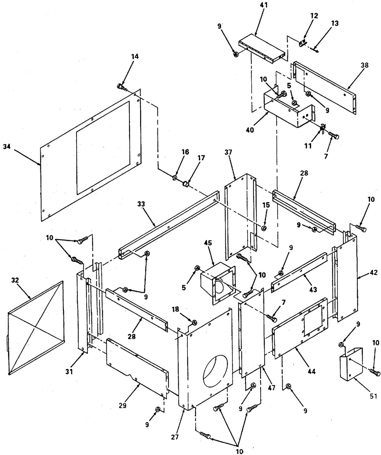
Figure 3. Enclosure Assembly (Sheet 2 of 2).
