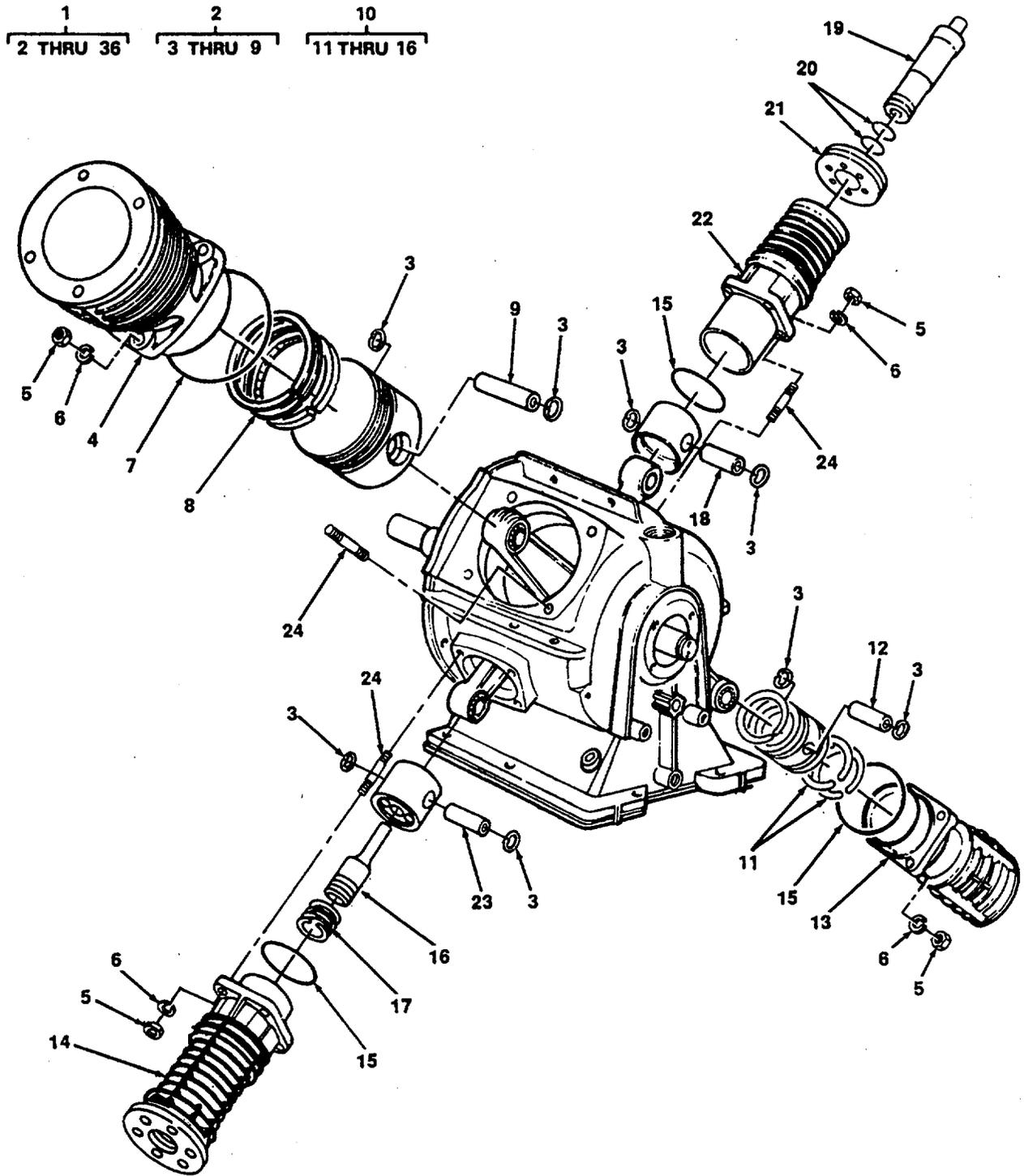
Figure 35. Compressor Pistons and Cylinders.
