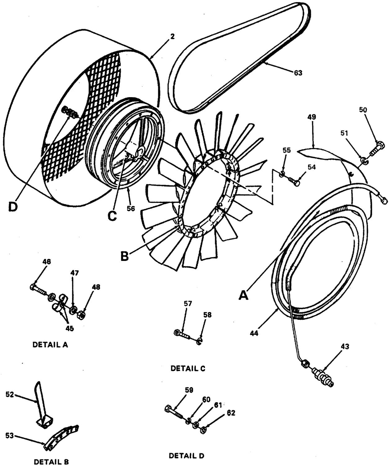
Figure 32. Compressor Flywheel and Cooler (Sheet 2 of 2).
