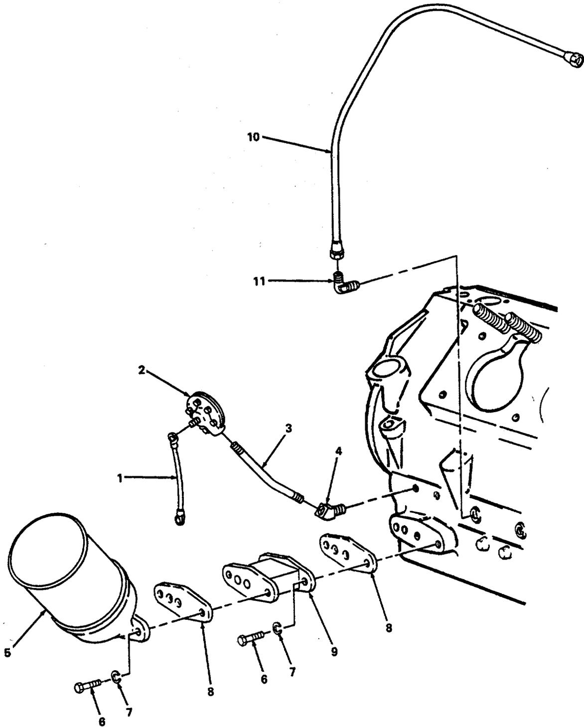
Figure 27. Oil Filter and Mounting.
