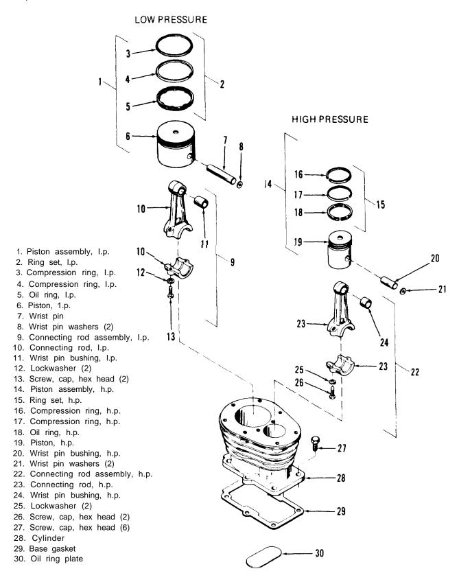
Figure 6-1. Cylinder head, pistons and connecting rod.
