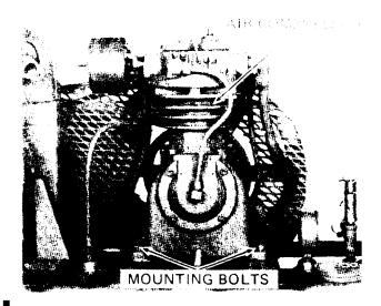
(4) Inspect the unloader and safety relief valve for loose mounting.
