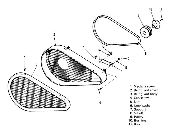
Figure 4-2. Belt guard, removal and installation.
