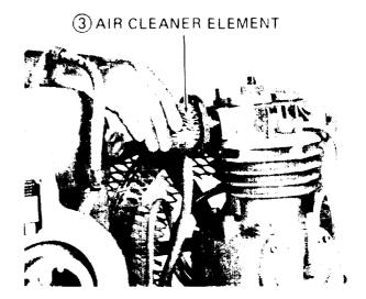
c. Lift out air cleaner element (3) and check for dirt. Service the air cleaner.
