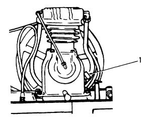
Oil level gage Indicates oil level in the crankcase
