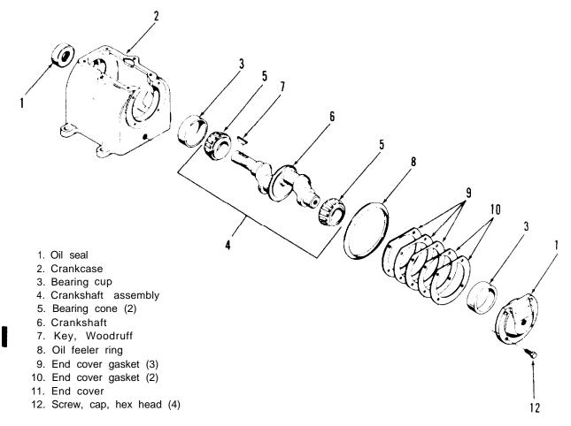
Figure 6-2. Crankshaft and crankcase.
