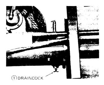
b. Keep all fittings connected to the air receiver tank tight. Check for leaks with soapy water with pressure in air receiver. Check welds on air receiver tank with soapy water.
