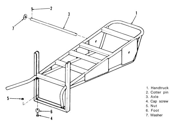
Figure 4-7. Handtruck assembly, disassembly and reassembly.
