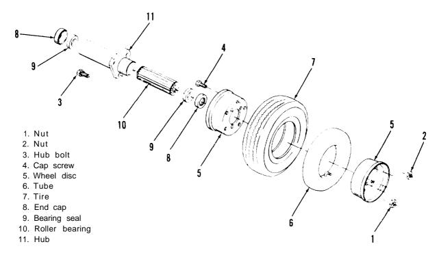
Figure 4-8. Wheel assembly, disassembly and reassembly.
