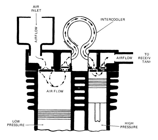
Figure 1-3. Typical two stage compressor.
