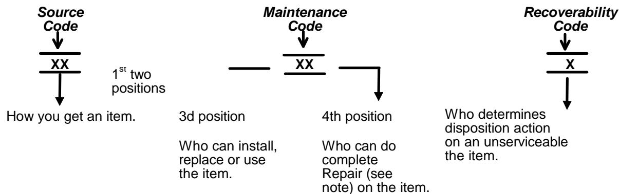
\*Complete Repair: Maintenance capacity, capability, and authority to perform all corrective maintenance tasks of the "Repair" function in a use/user environment in order to restore serviceability to a failed item.
