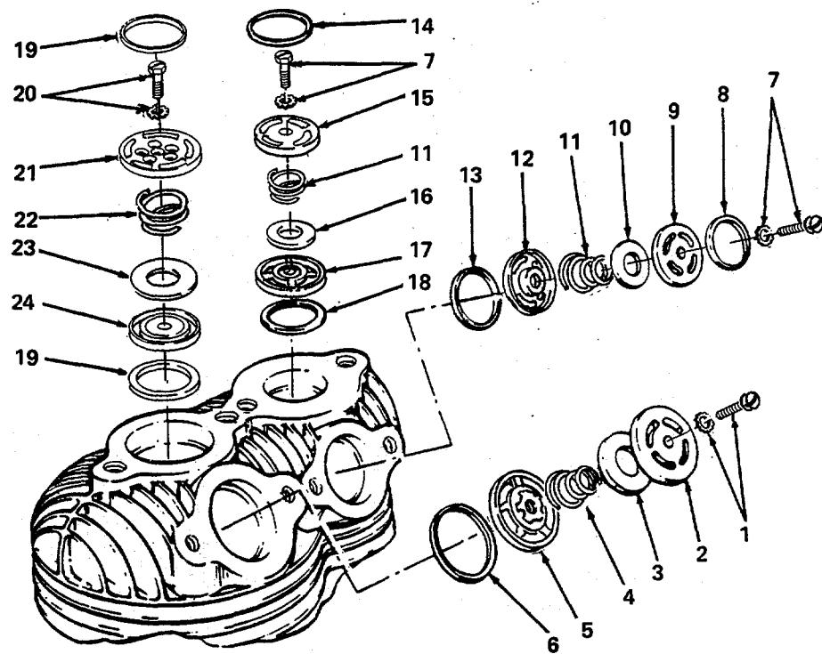
Figure 7. Valve Assembly.
