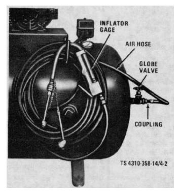
Figure 4-2. Air hose assembly, removal points
