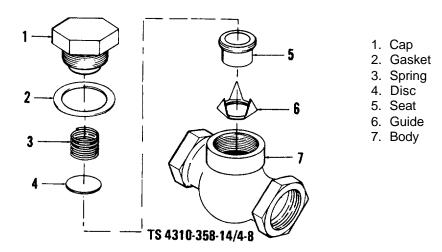
Figure 4-8. Check valve exploded view.
