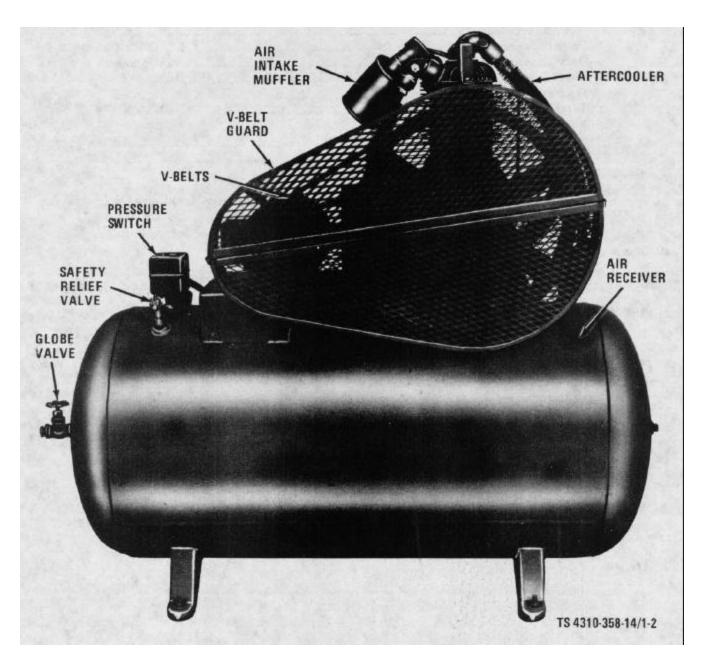
Figure 1-2. Air Compressor, left side view.
