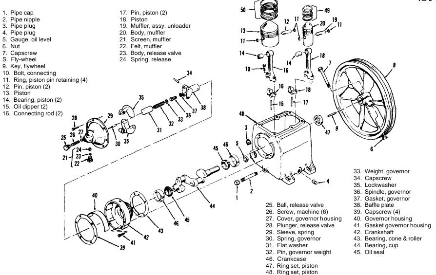
Figure 5-9. Crankcase, crankshaft, pistons, connecting rods and related assemblies, exploded view.
