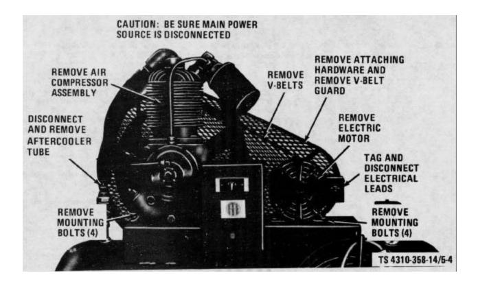
Figure 5-4. Electric motor and compressor, cleaning, v-belt removal and installation
