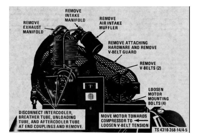
Figure 4-5. Compressor components and v-belt drive.
