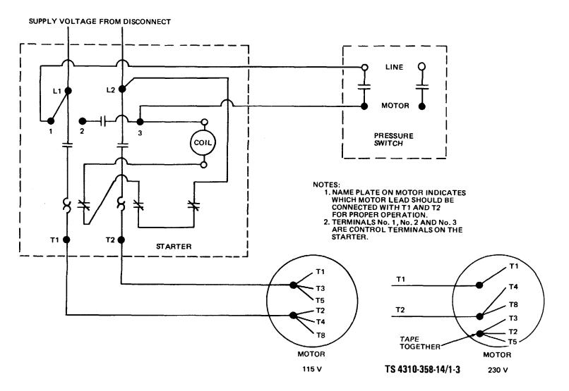
Figure 1-3. Wiring diagram.
