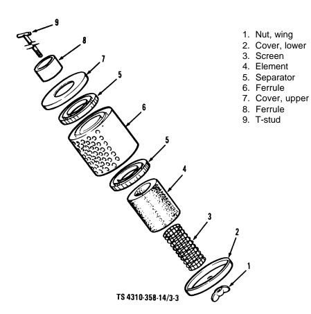
Figure 3-3. Air intake muffler
