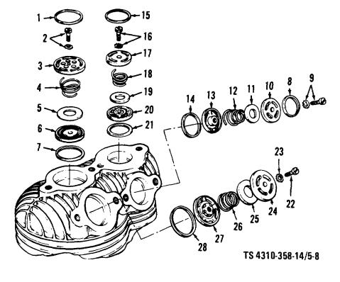
Figure 5-8. Compressor valve assemblies, disassembly and reassembly.
