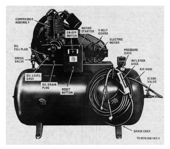
Figure 1-1. Air Compressor, right side view.
