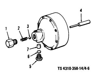
Figure 4-6. Compressor release valve assembly, removal and installation
