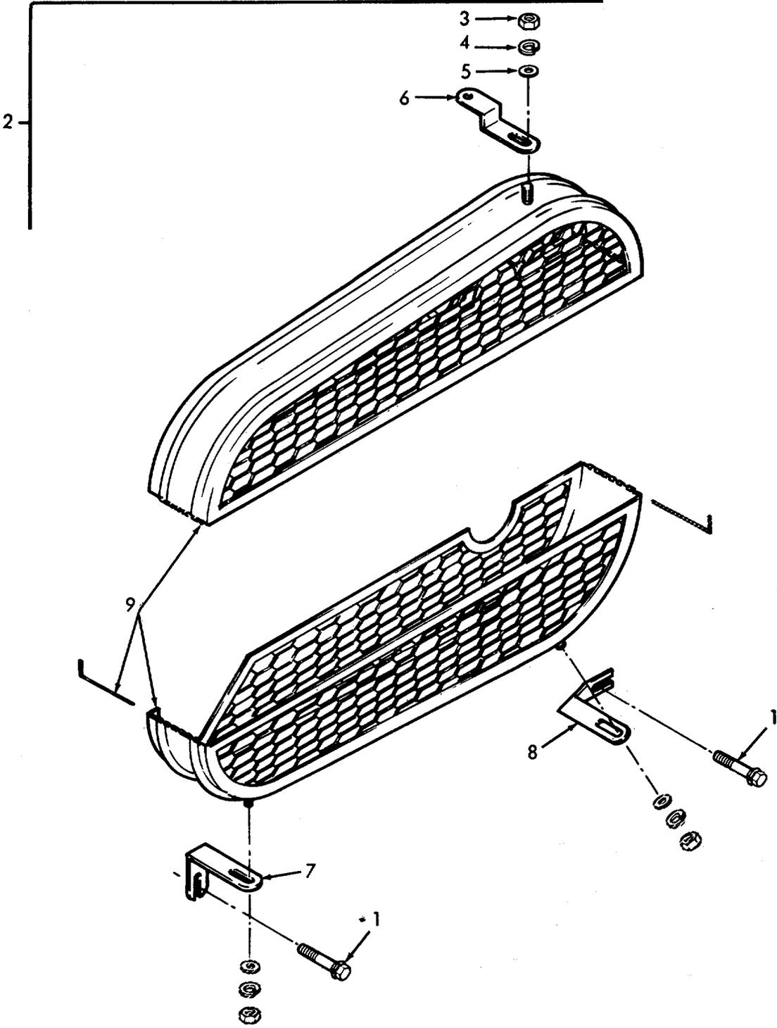
Figure 1. Belt guard shell and brackets.
