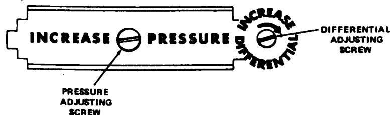
Figure 9. Pressure adjusting and differential screws.
