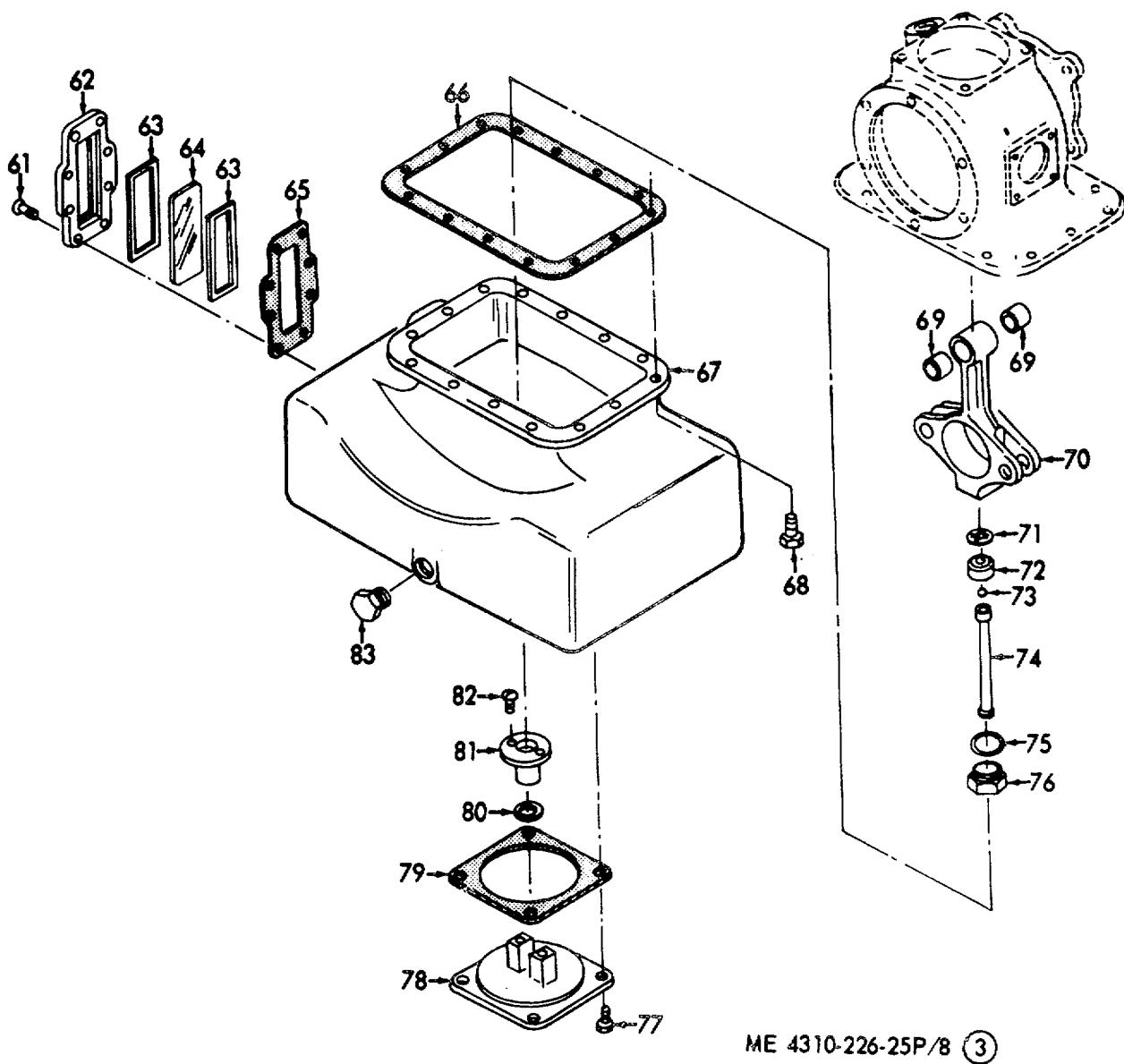
Figure No. 8 (3). Crankcase, Cylinder Piston And Head
