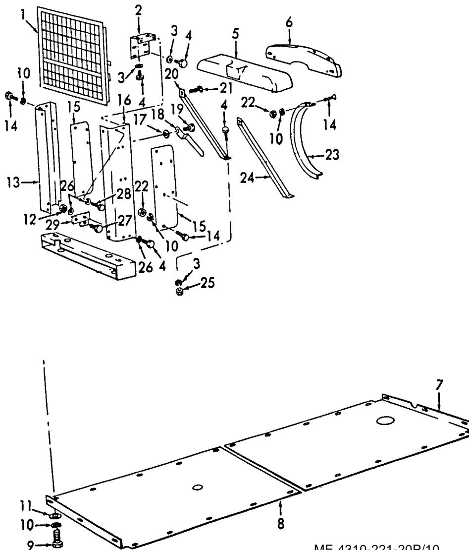
Figure 10. Radiator Guard and Braces.
