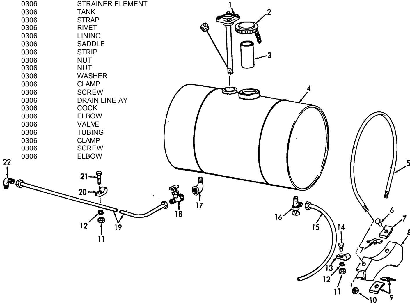
Figure 7. Gas Tanks and Lines.
