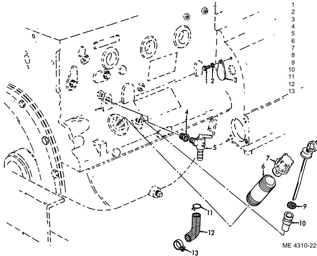
Figure 1. Oil Filler Cap and Gage.
