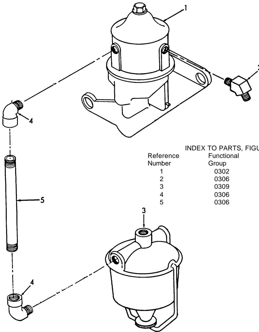
*Figure 31. Strainer and Fuel Pump.*
