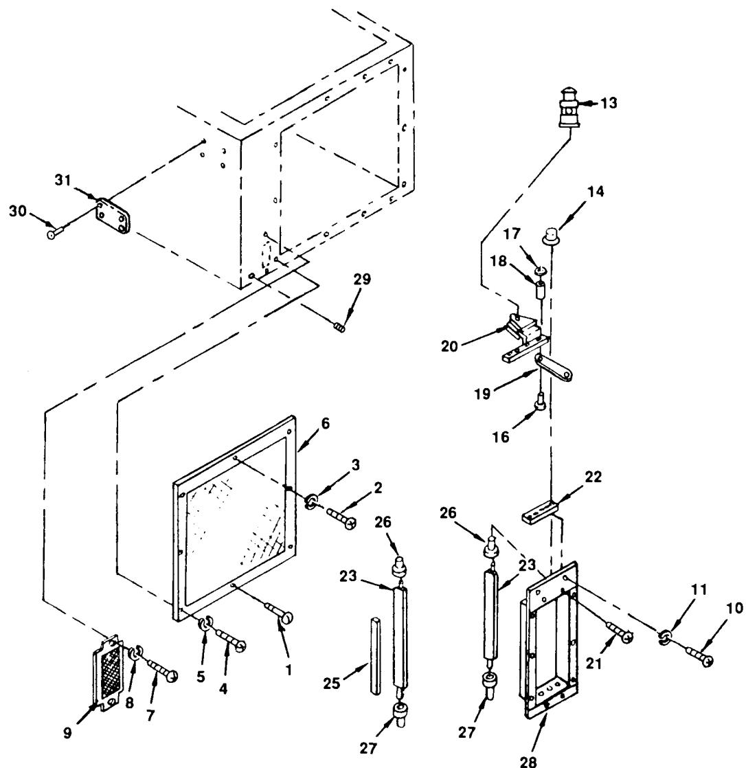
Figure 3. Side and Rear Guards, Louvers, and Instruction Plate.
