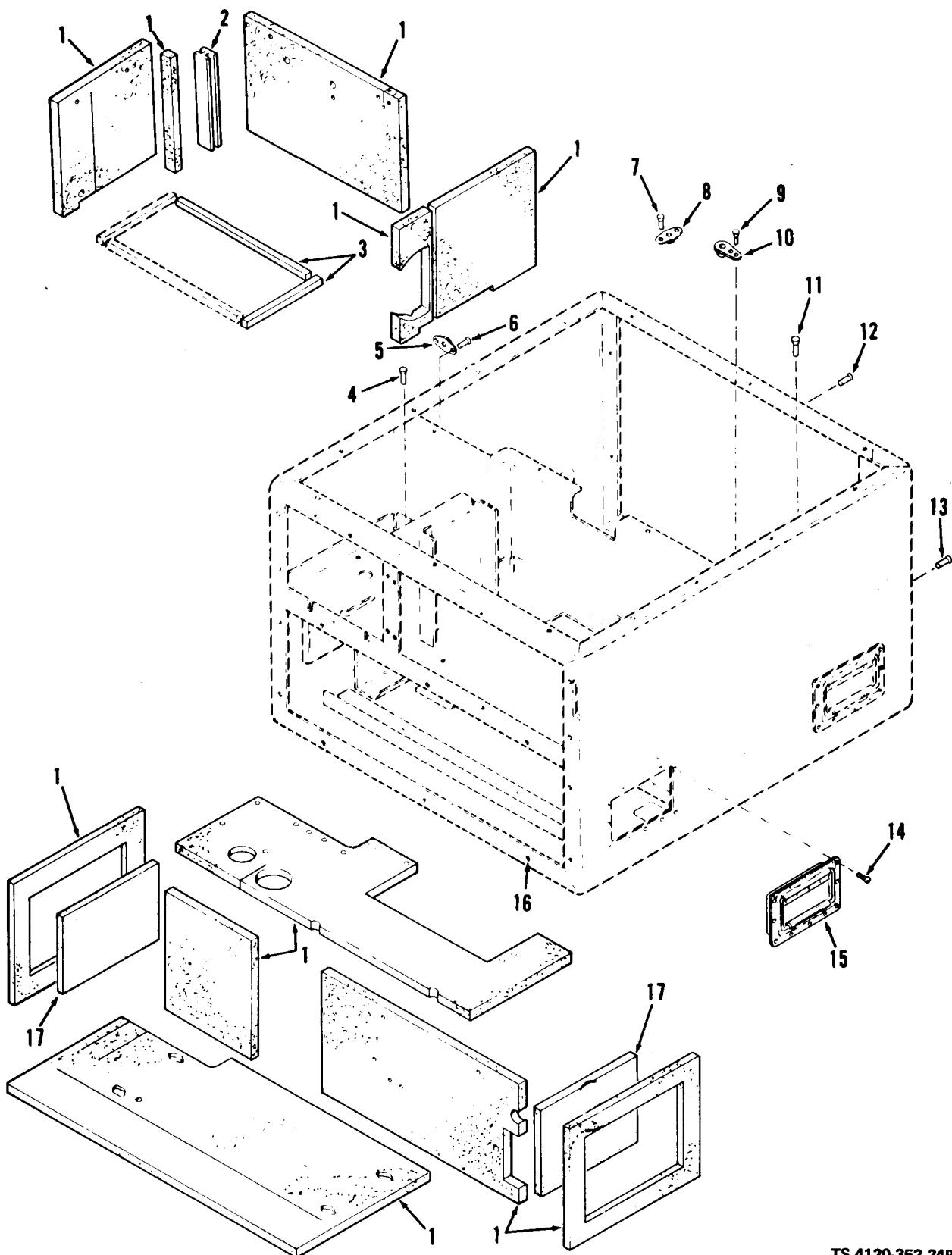
**Figure 2. Frame and Casing – Housing Assembly**
