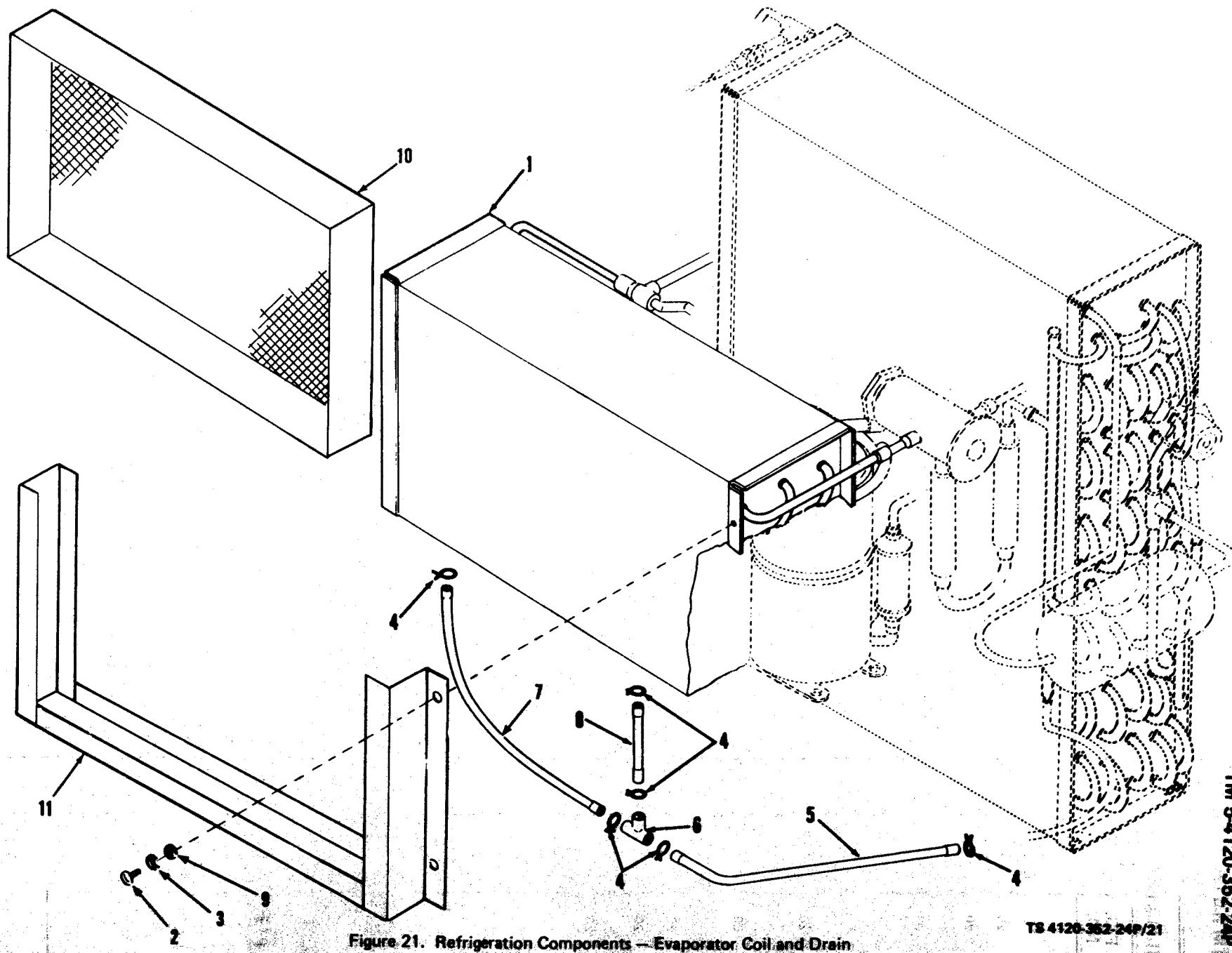
Figure 21. Refrigeration Components — Evaporator Coil and Drain
