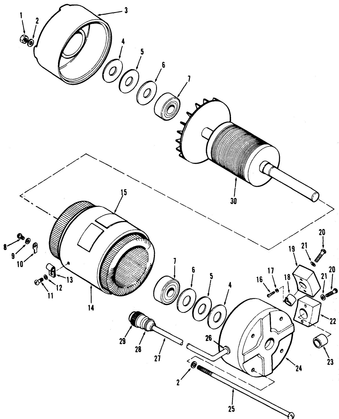
Figure 15. Electric Motors – Condenser and Evaporator Fans
