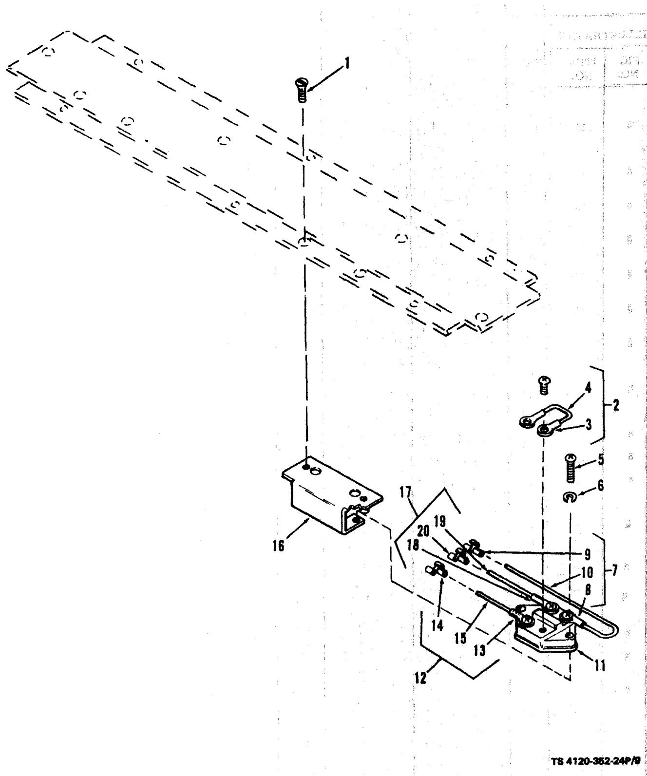
Figure 9. Starting and Protective Devices - Heater Thermostatic Switch
