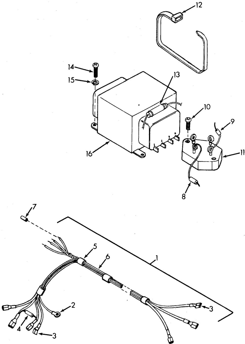
Figure 12. Transformer and Rectifier Assembly
