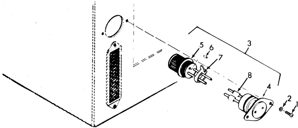
**Figure 13. Condenser Fan Thermostatic Switch**
