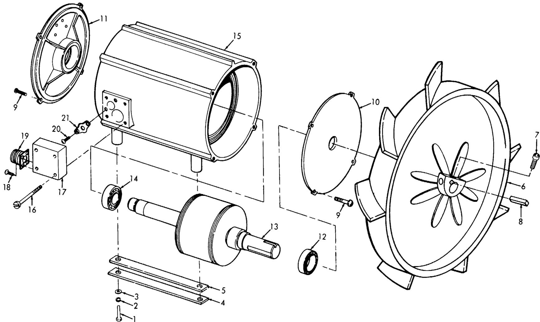
Figure 13. Condenser Fan and Motor
