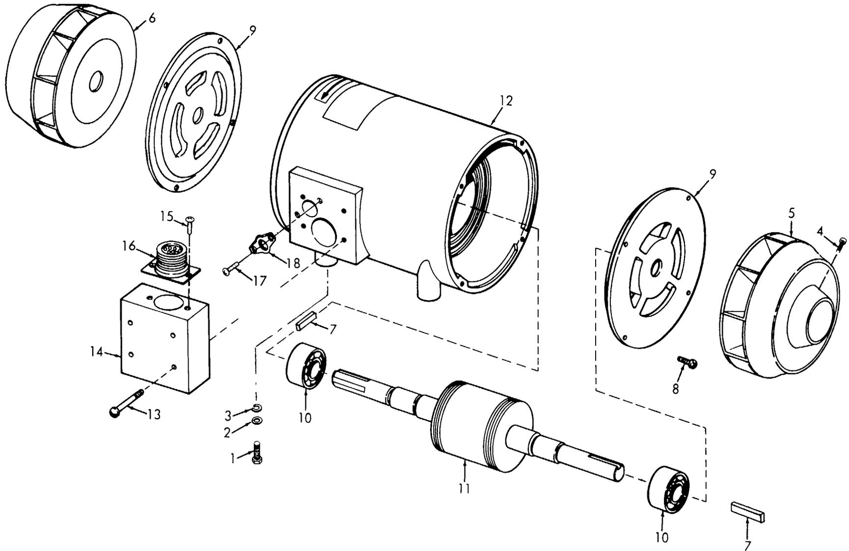
Figure 14. Evaporator Fan and Motor
