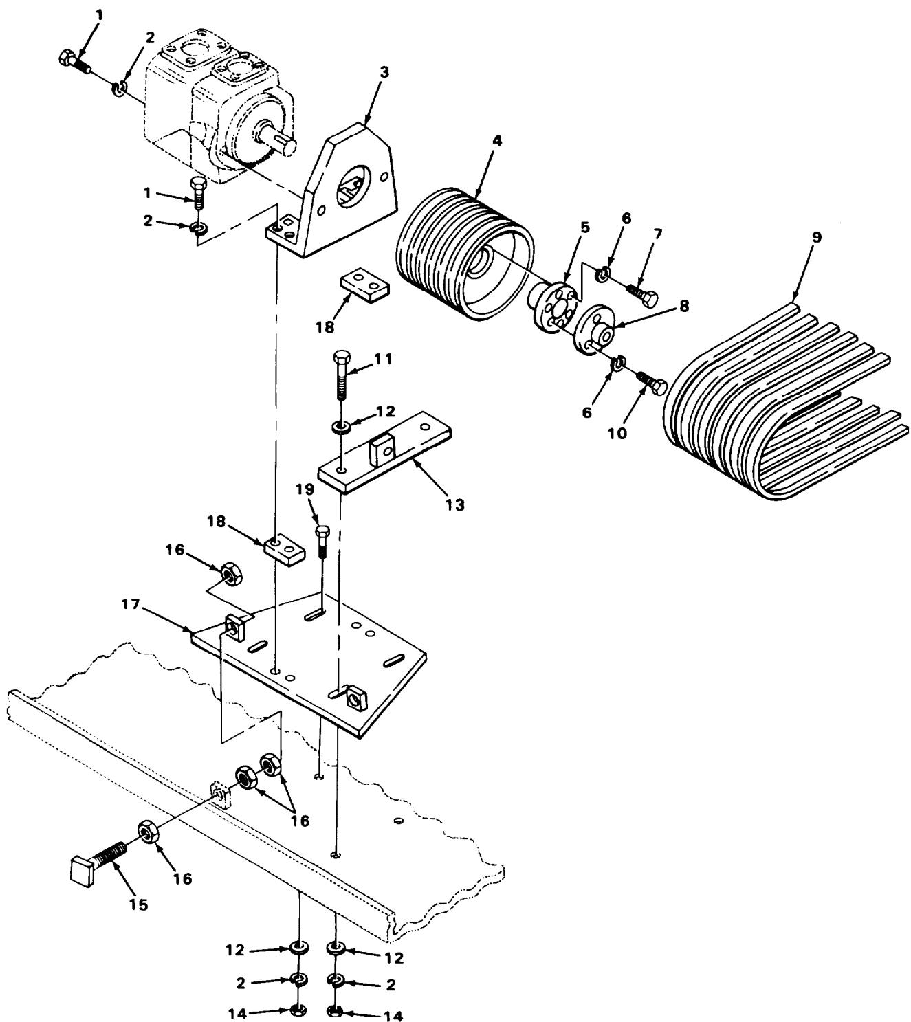
FIGURE 8. HYDRAULIC OIL PUMP MOUNTING AND RELATED PARTS.
