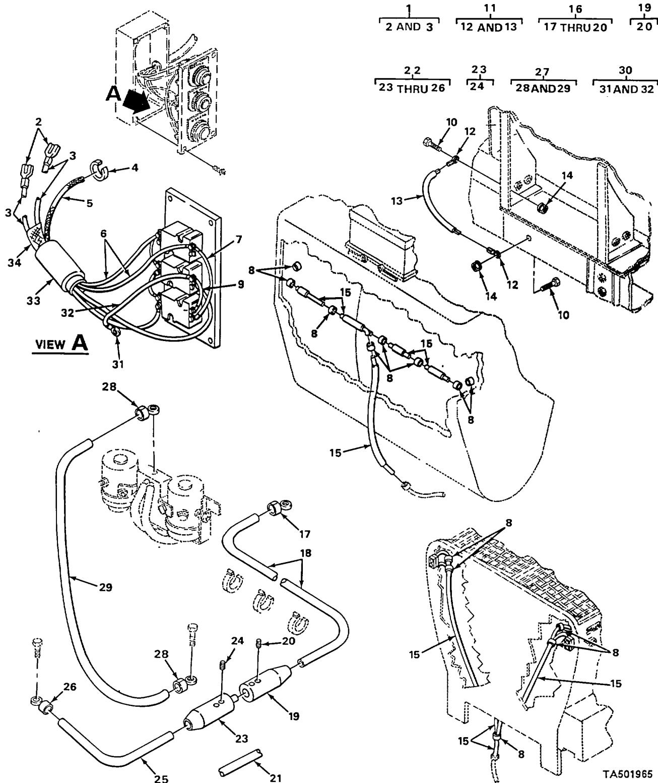
*FIGURE 3. CHASSIS WIRING.*
