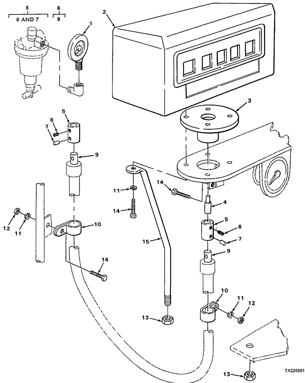
FIGURE 21. LIQUID ADMIXTURE PRESSURE GAGE AND CEMENT FEEDER.
