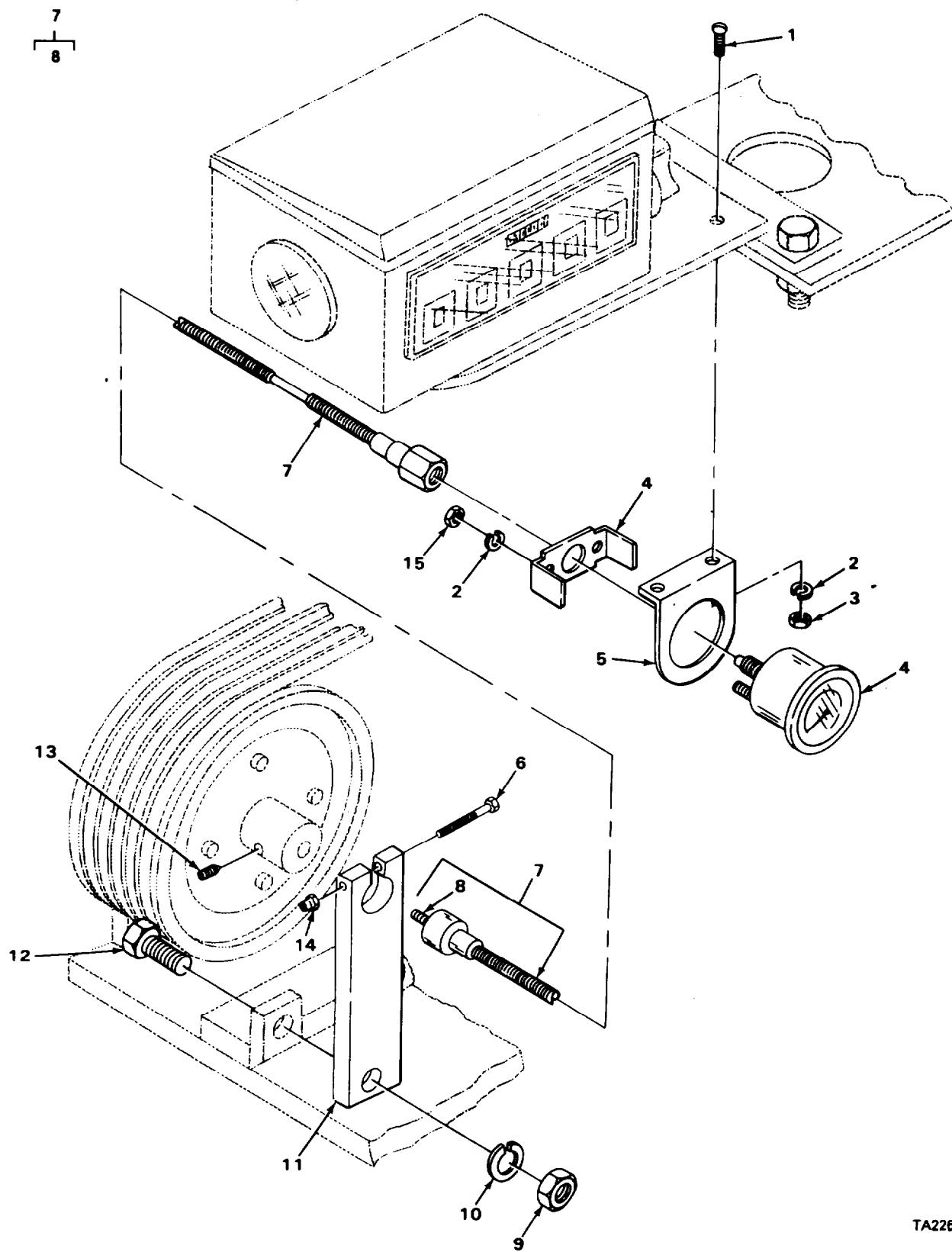
FIGURE 20. TACHOMETER.
