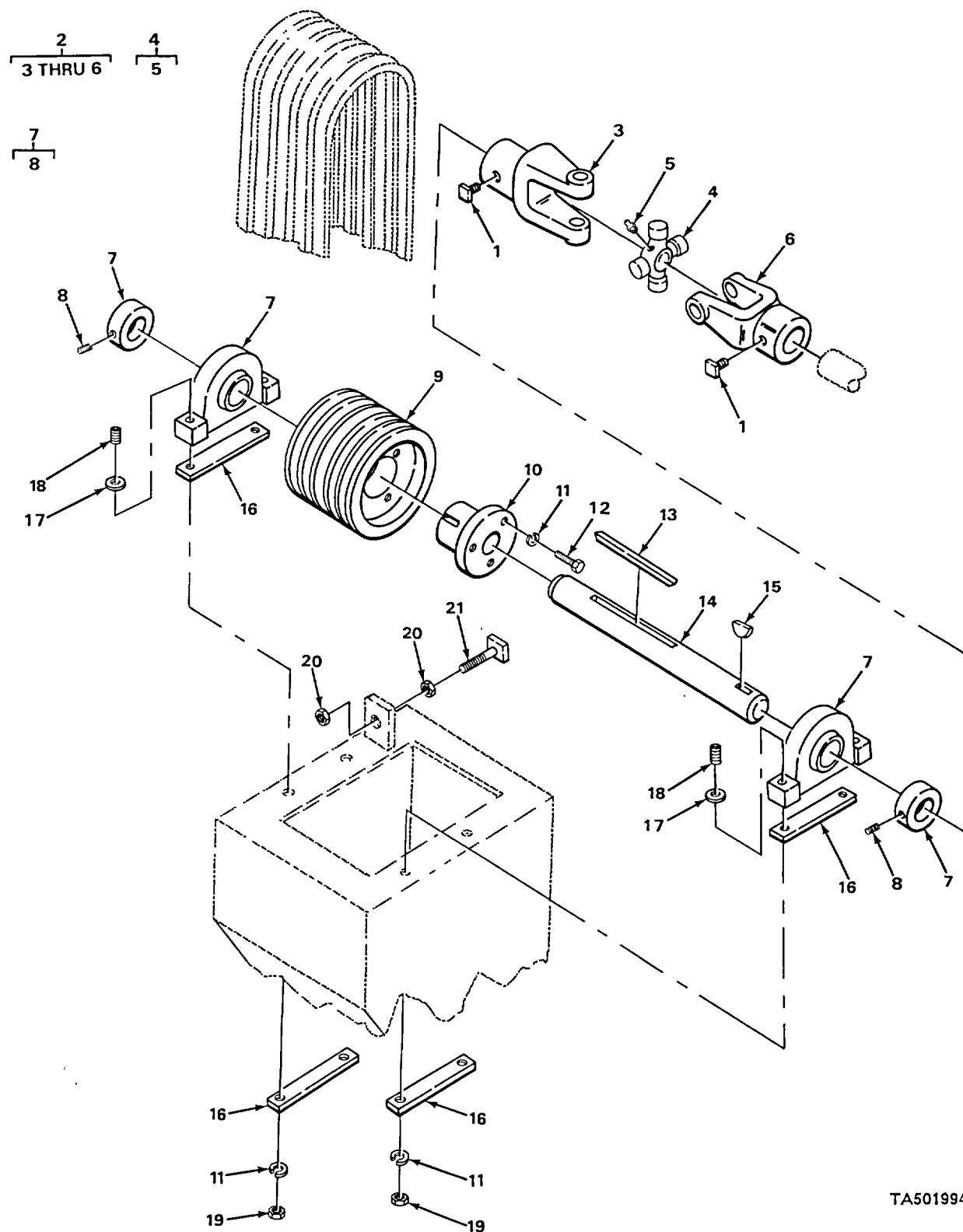
FIGURE 43. MAIN DRIVE SYSTEM, PTO BELTS SHAFT.
