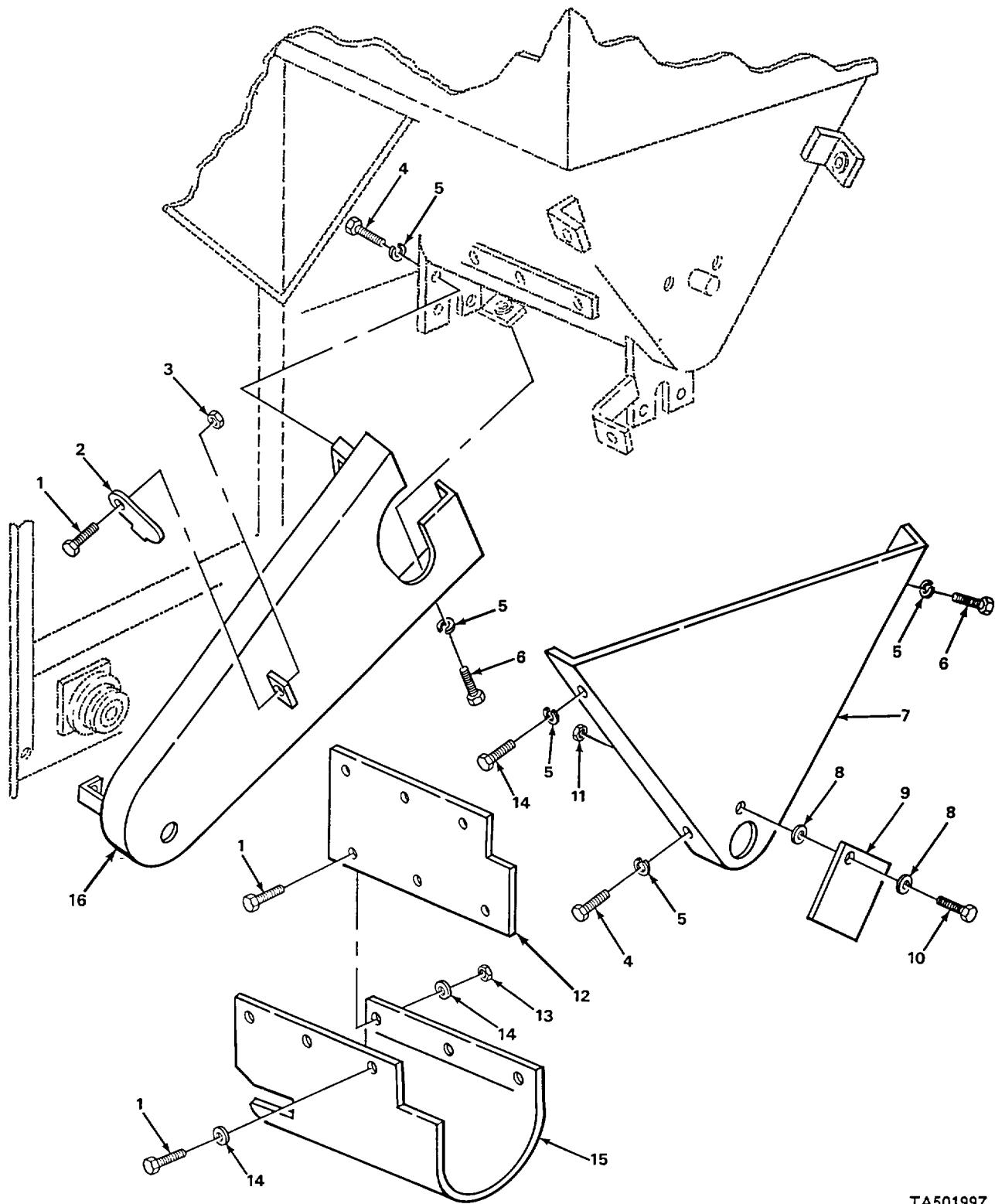
*FIGURE 47. MAIN DRIVE SYSTEM GUARDS, CEMENT BIN.*
