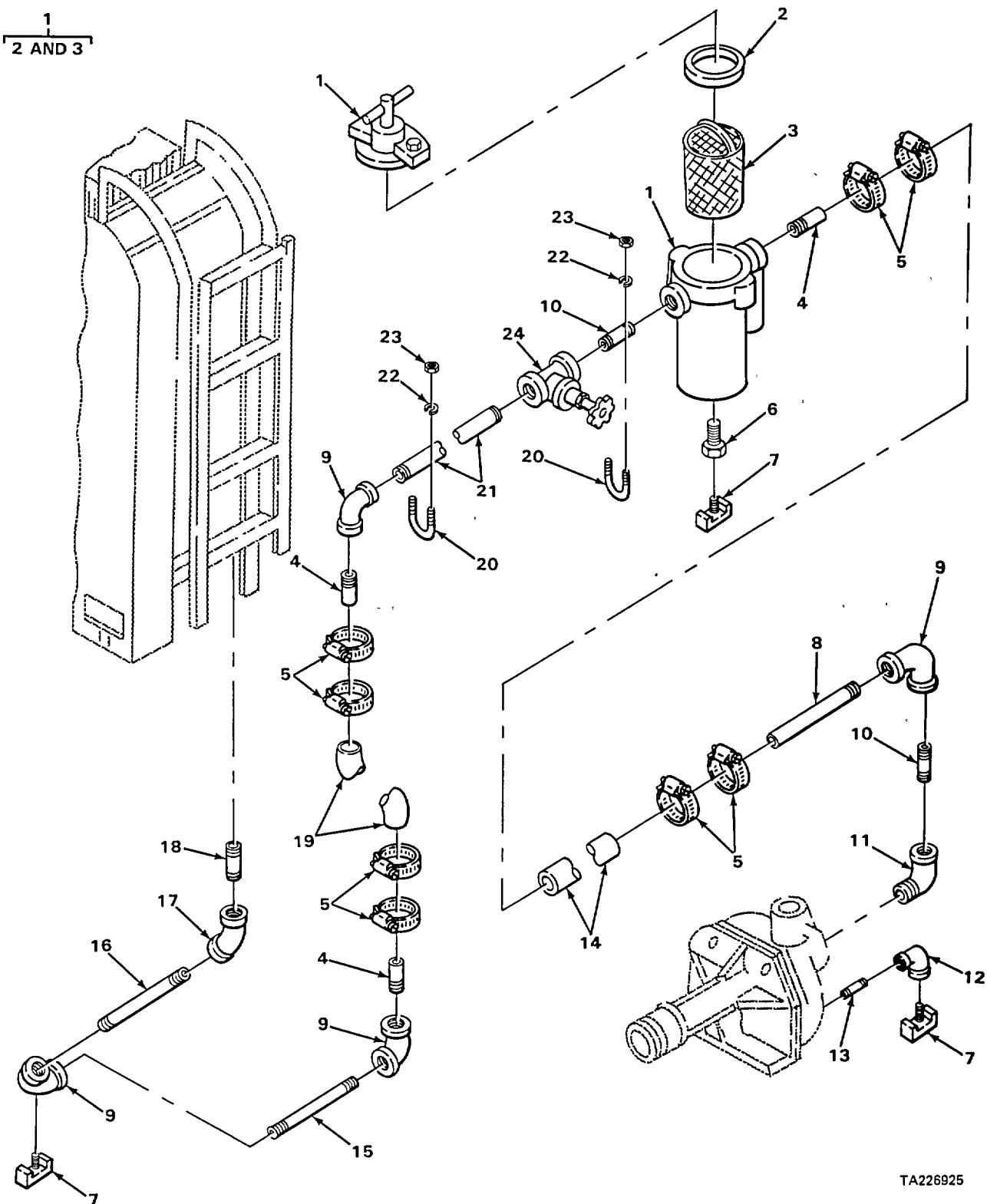
FIGURE 65. WATER SYSTEM LINES, TANK TO PUMP.
