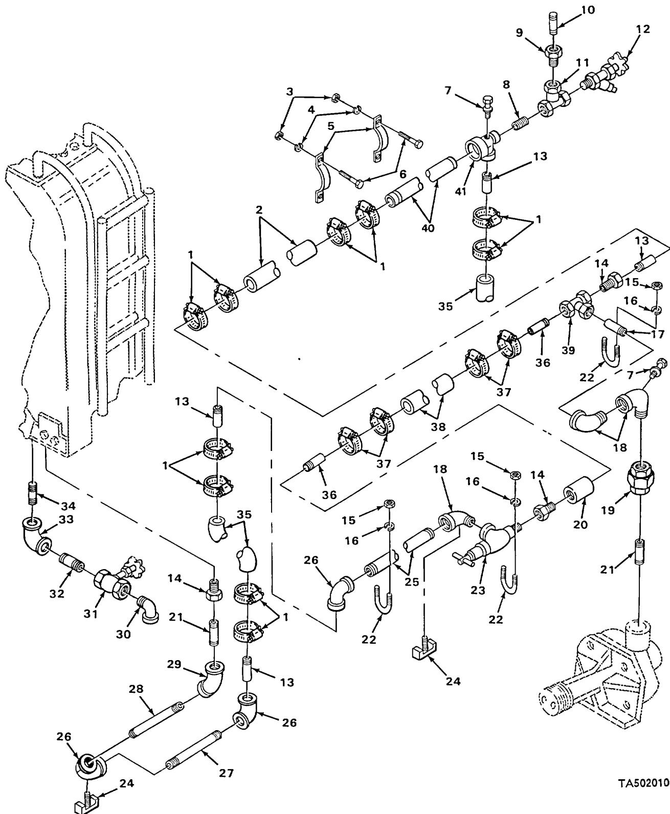
FIGURE 66. WATER SYSTEM RETURN LINES, PUMP TO TANK.
