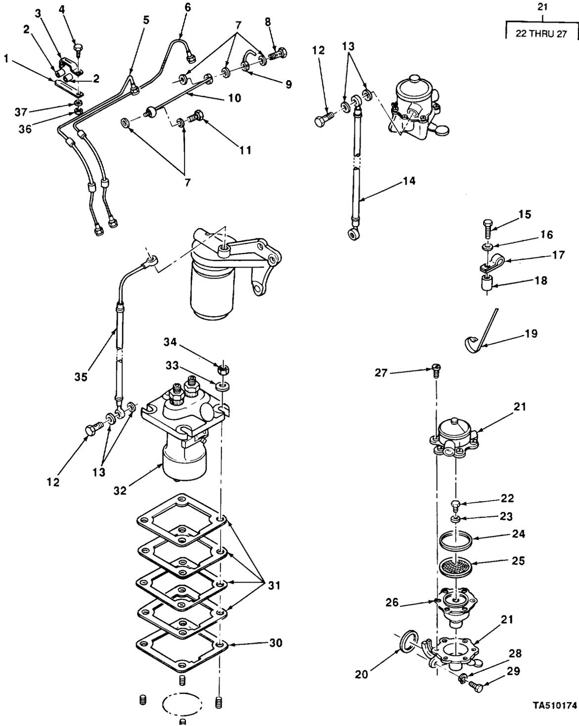
FIGURE 16. FUEL PUMPS AND LINES.
