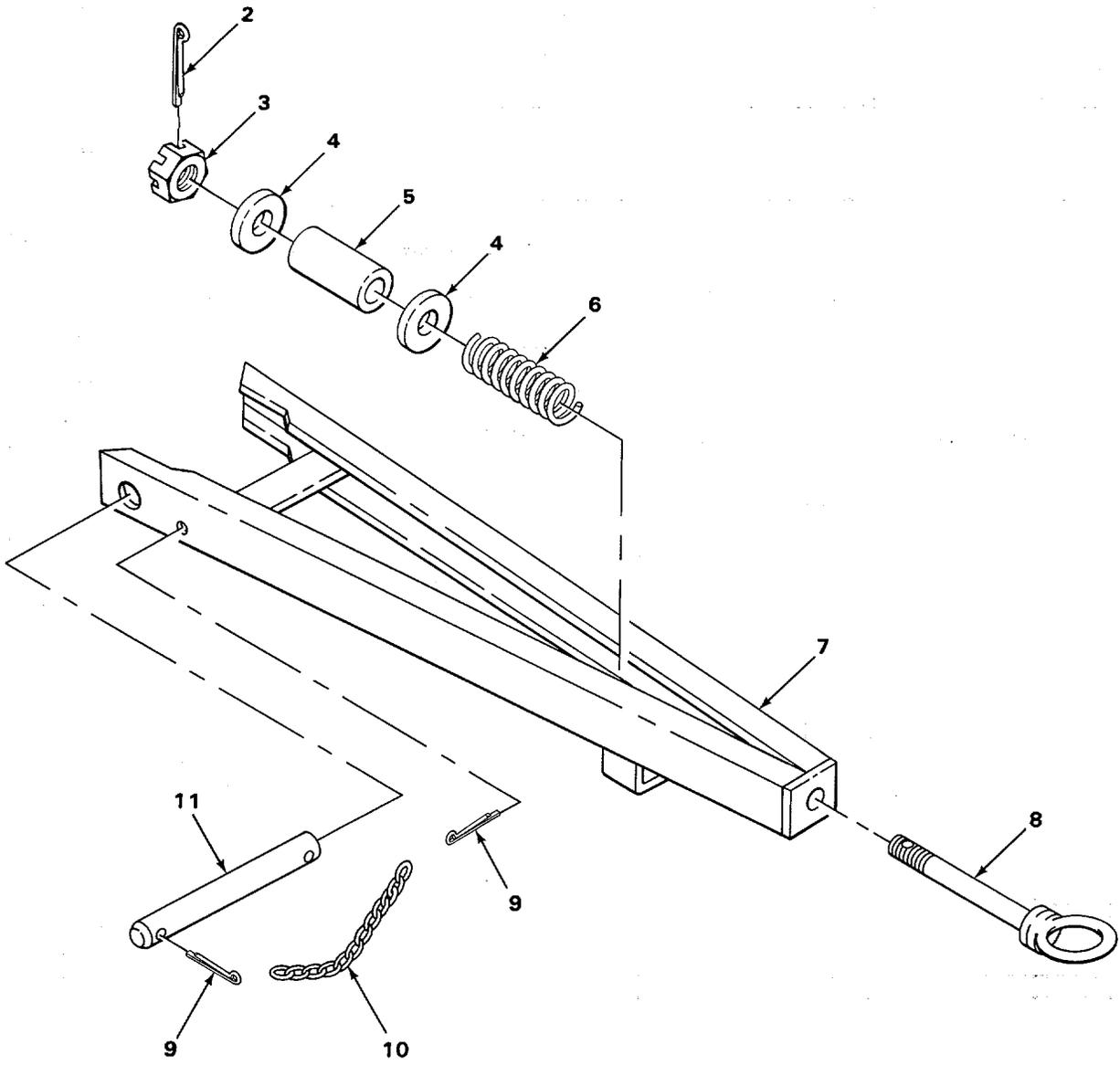
FIGURE 47. TOWING ATTACHMENTS.
