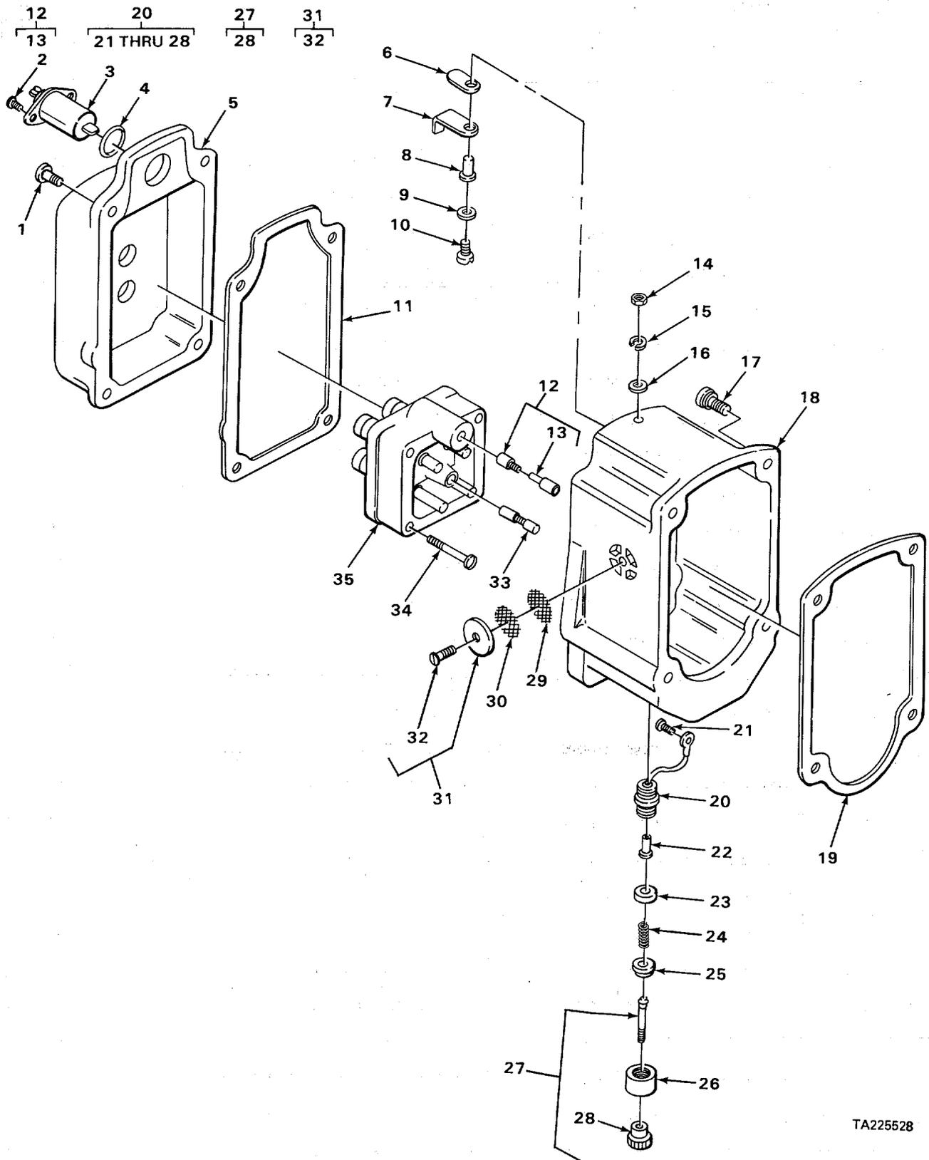
FIGURE 33. MAGNETO ASSEMBLY.
