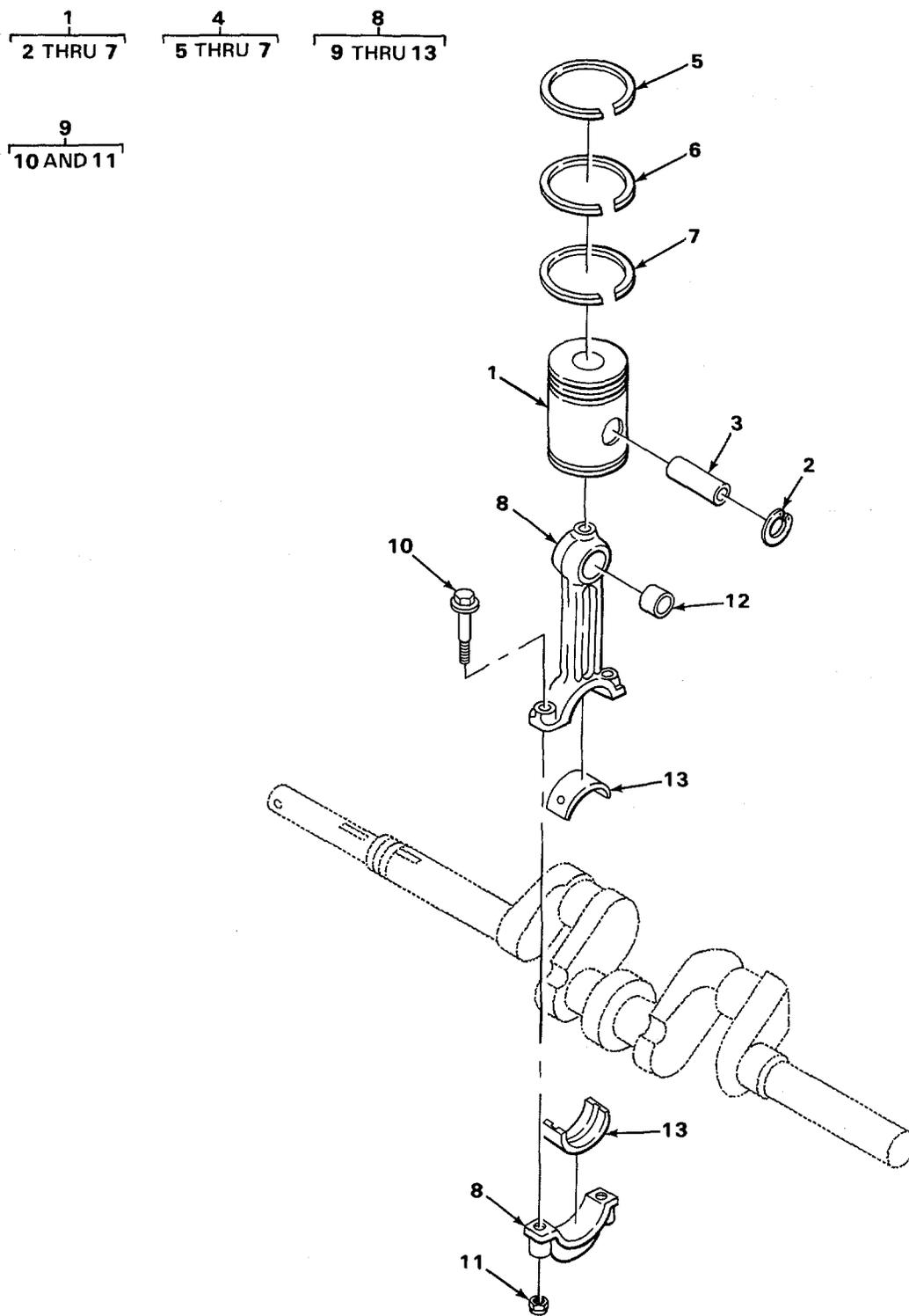
FIGURE 6. PISTON AND CONNECTING ROD.
