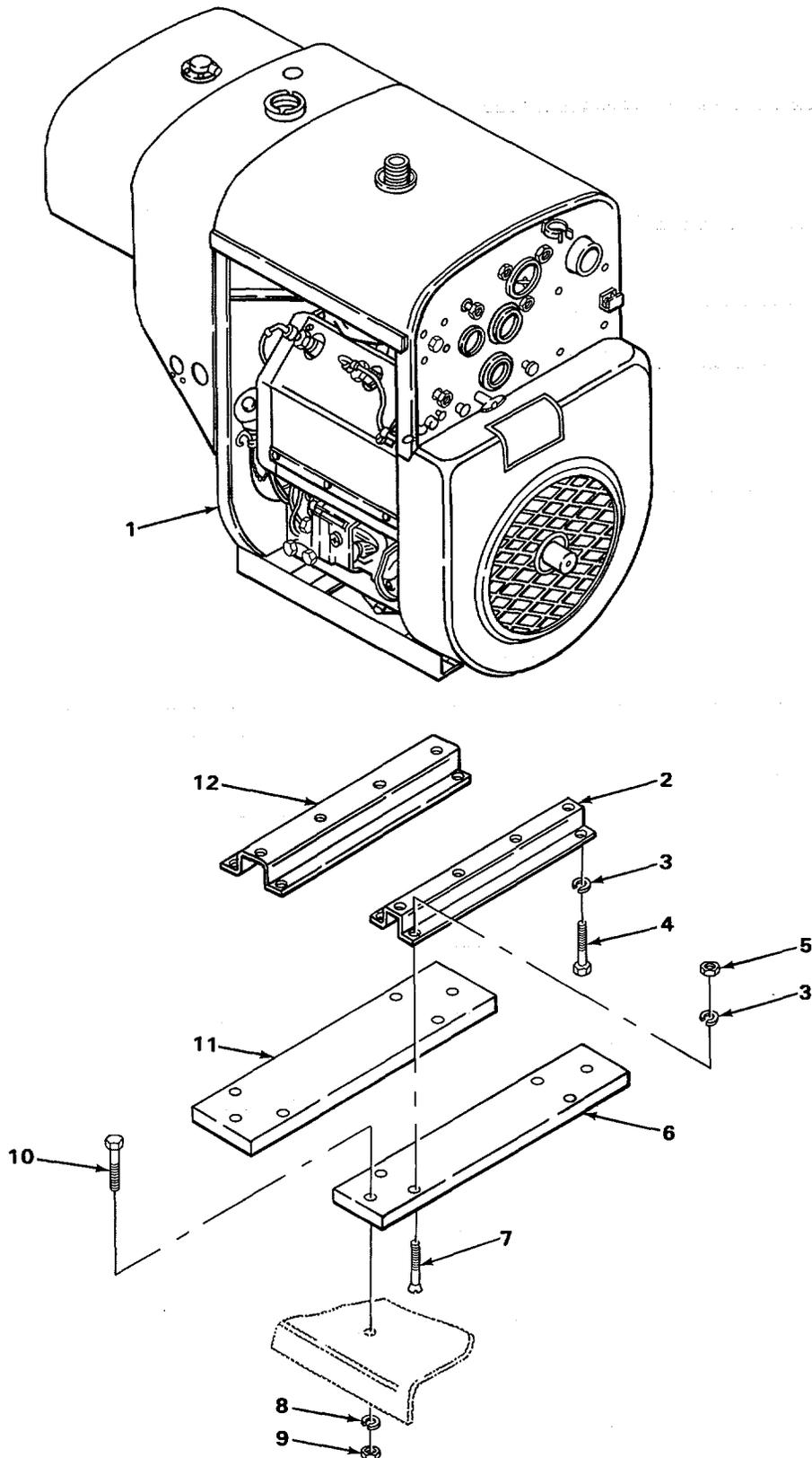
FIGURE 1. ENGINE AND MOUNTING HARDWARE.
