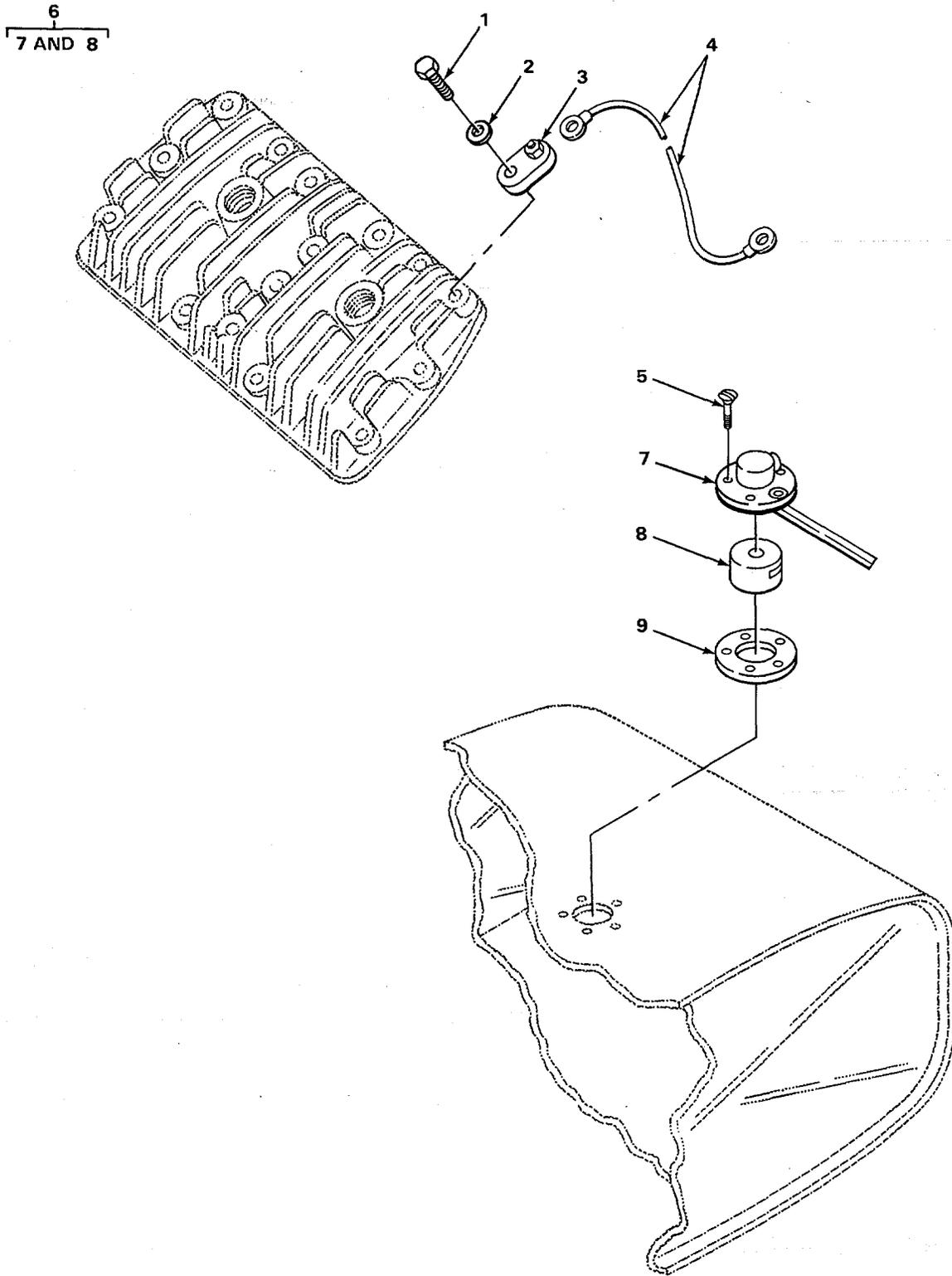
FIGURE 36. HI TEMPERATURE AND FUEL SENDING UNITS.
