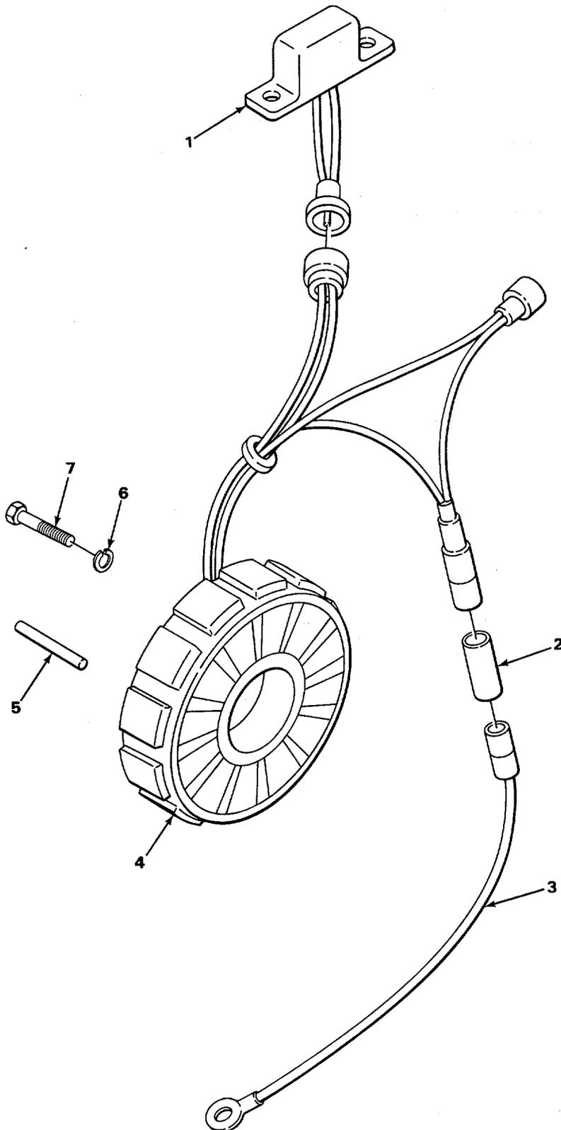
FIGURE 28. ALTERNATOR ASSEMBLY.
