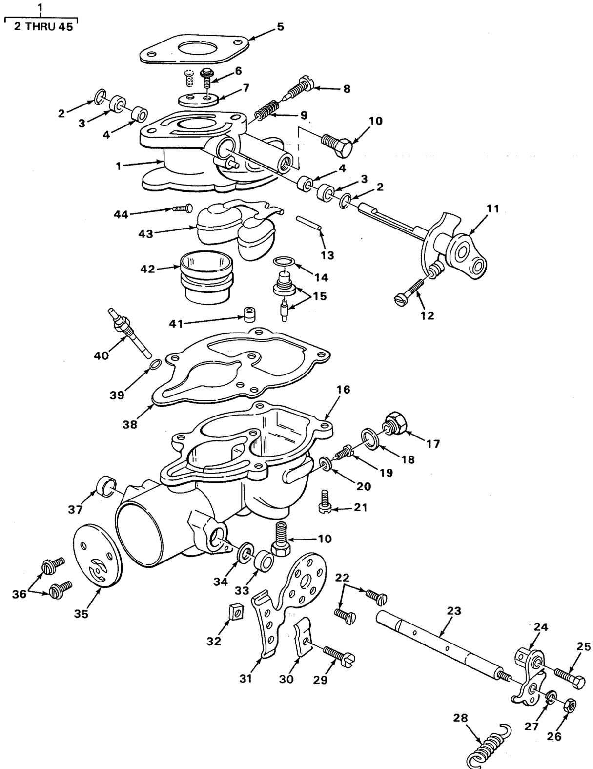
FIGURE 16. CARBURETOR ASSEMBLY.
