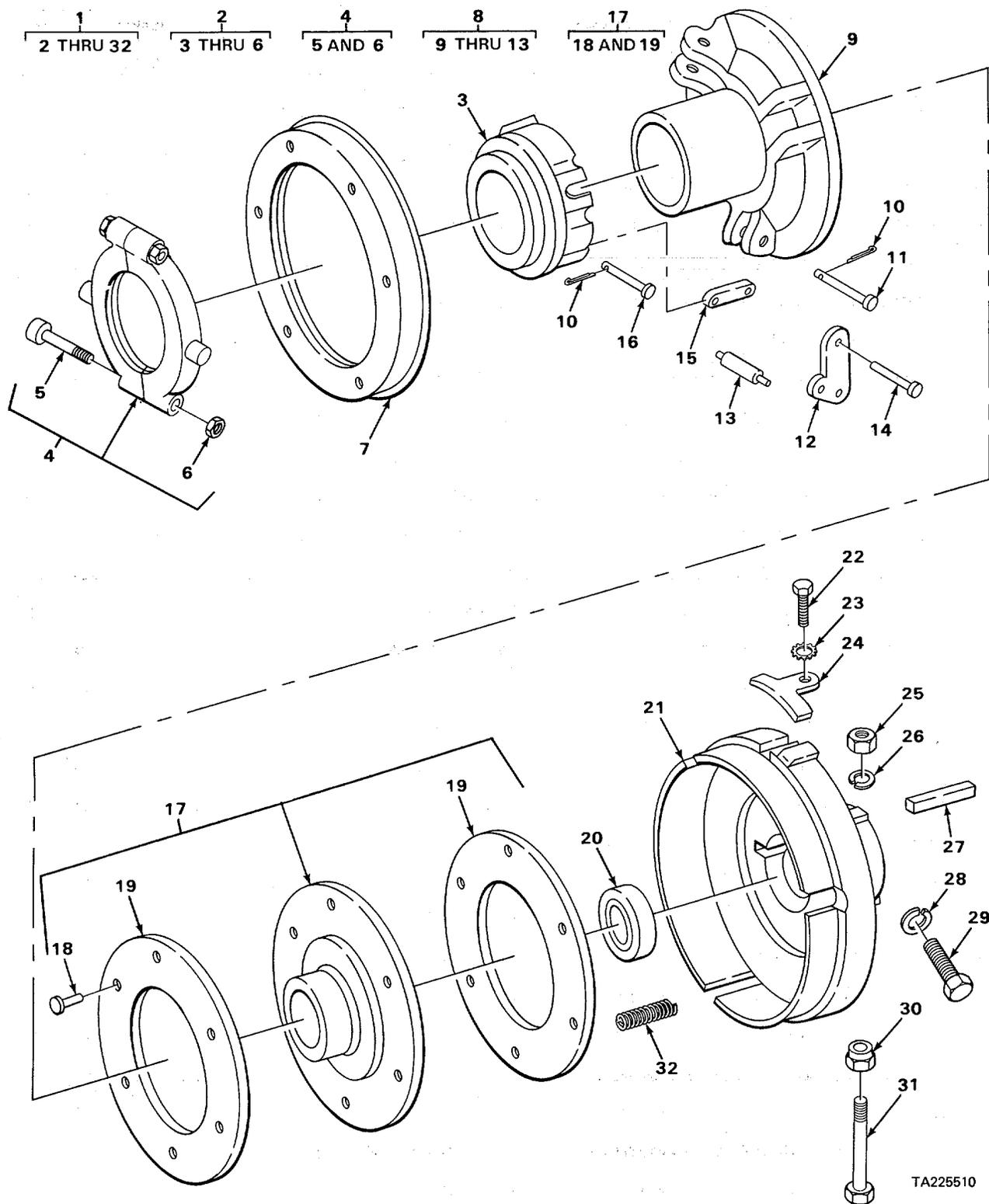
FIGURE 15. CLUTCH ASSEMBLY.
