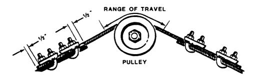
(1) Make a loop at the end of one cable, thread the other cable end through the loop, and make another loop. Secure both loops as shown.
