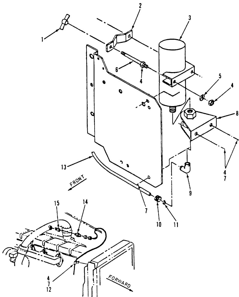
Figure 293. Ether Start Installation
