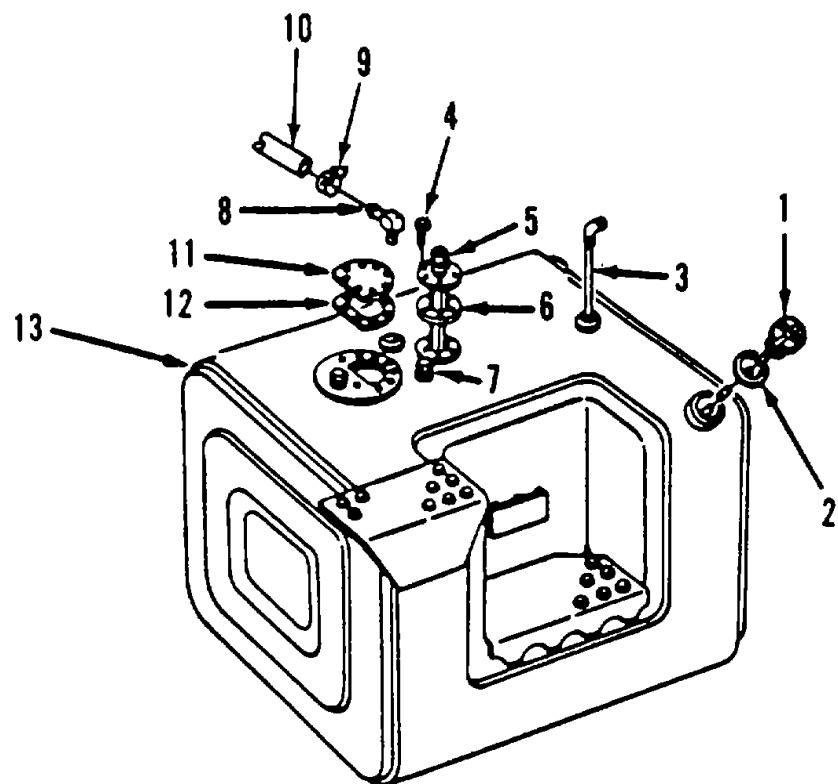
Figure 357. Fuel Tank Assembly
