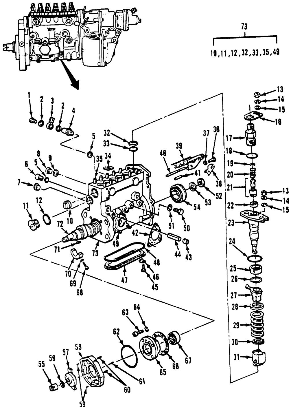
Figure 304. Fuel Injection Pump
