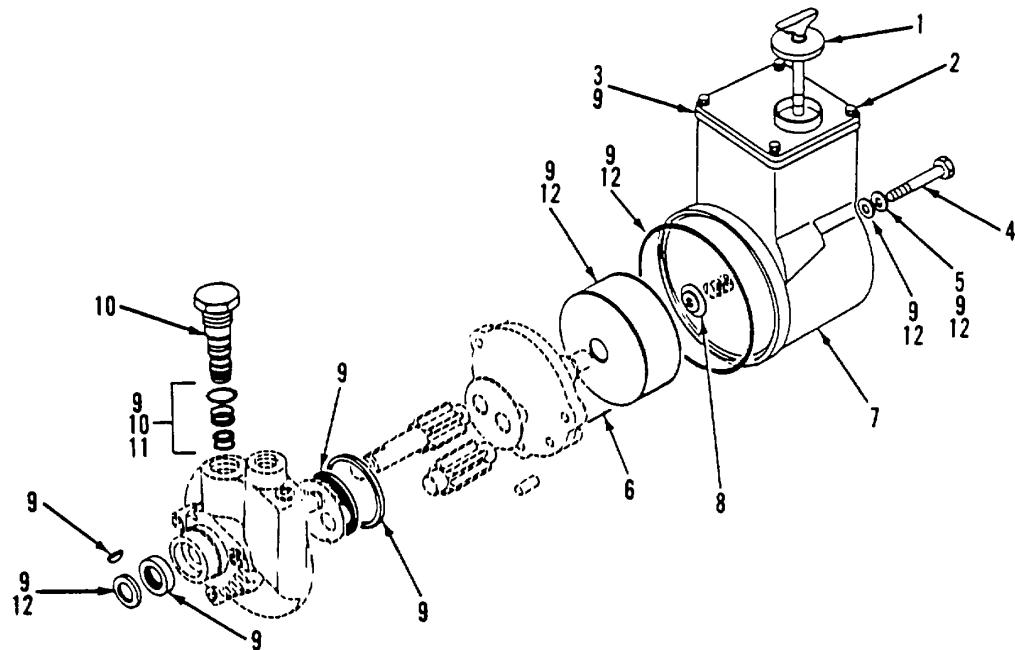
Figure 286. Steering Pump Assembly
