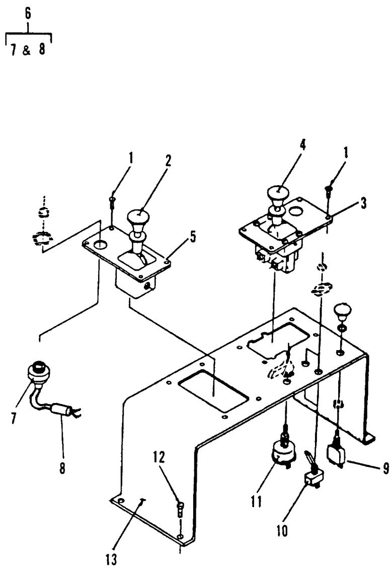
Figure 269. Control Console Assembly
