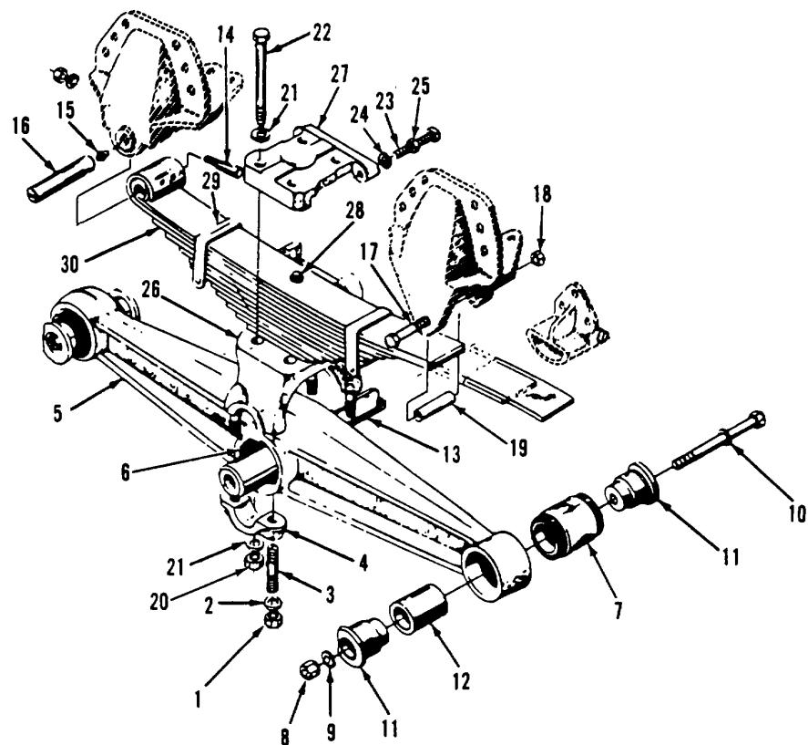
Figure 353. Rear Suspension (Sheet 1 of 2)
