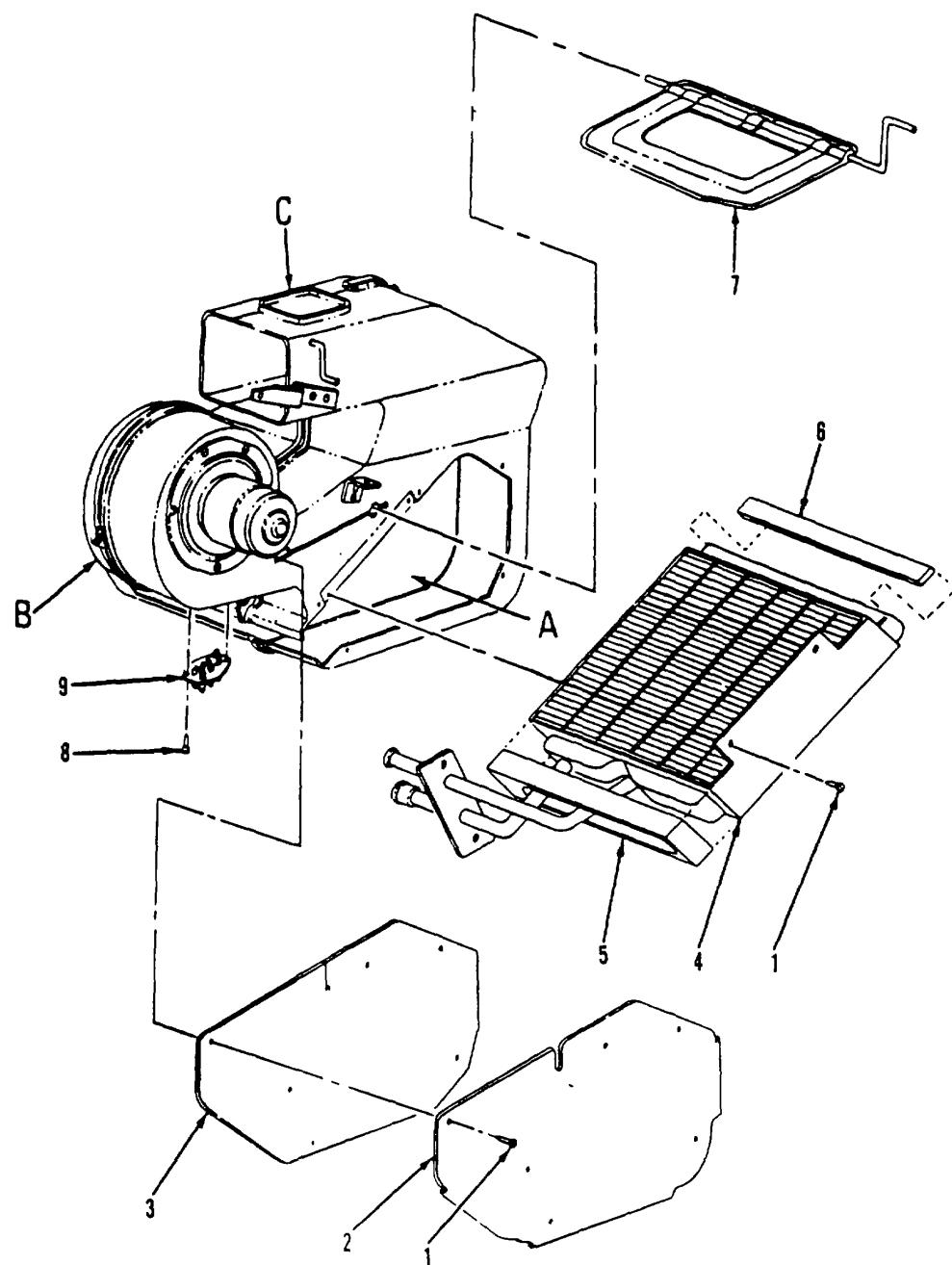
Figure 262. Heater Assembly (Sheet 1 of 2)
