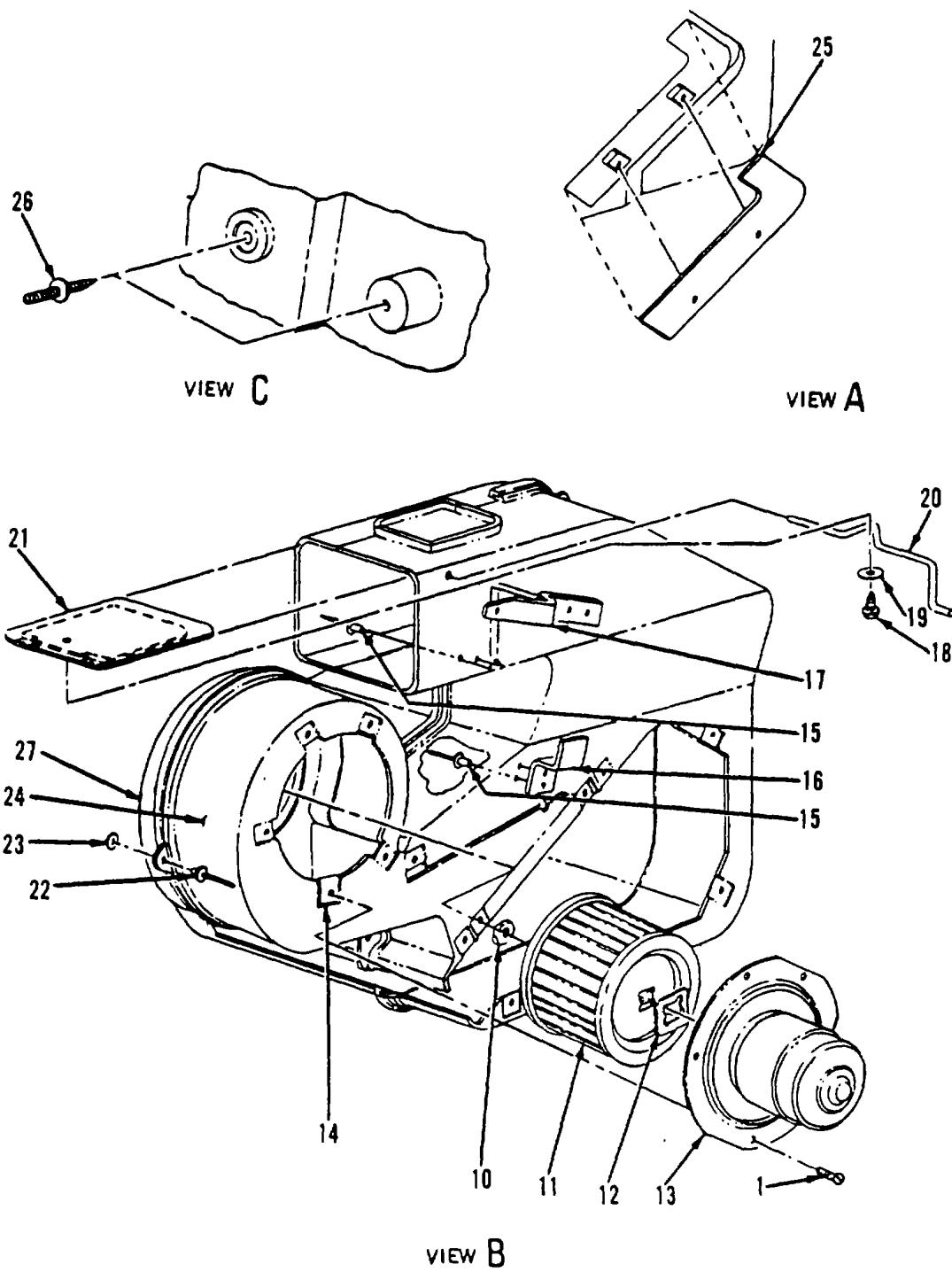
Figure 262. Heater Assembly (Sheet 2 of 2)
