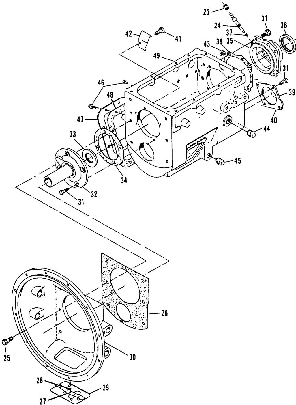
Figure 327. Transmission Assembly (Sheet 2 of 3)
