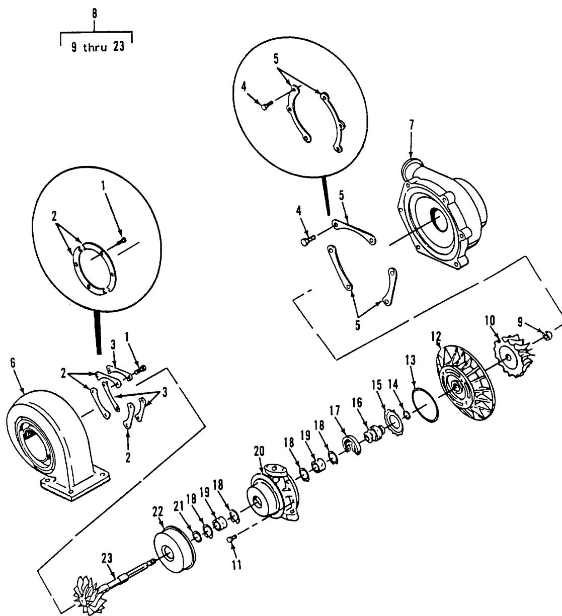
Figure 295. Turbocharger Assembly
