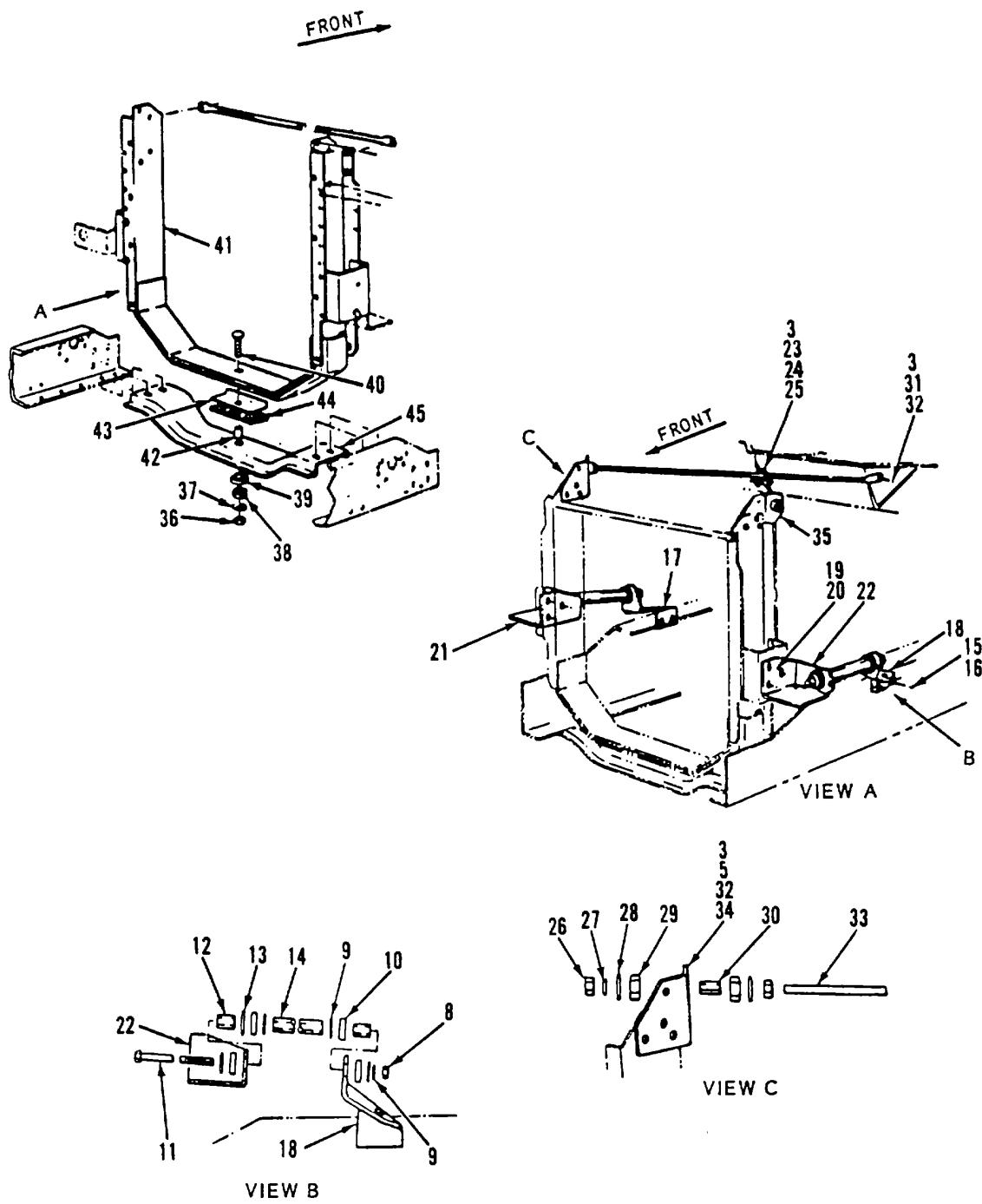
Figure 283. Radiator Installation (Sheet 2 of 2)
