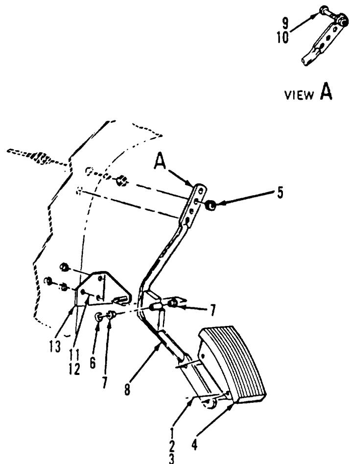
Figure 274. Accelerator Control
