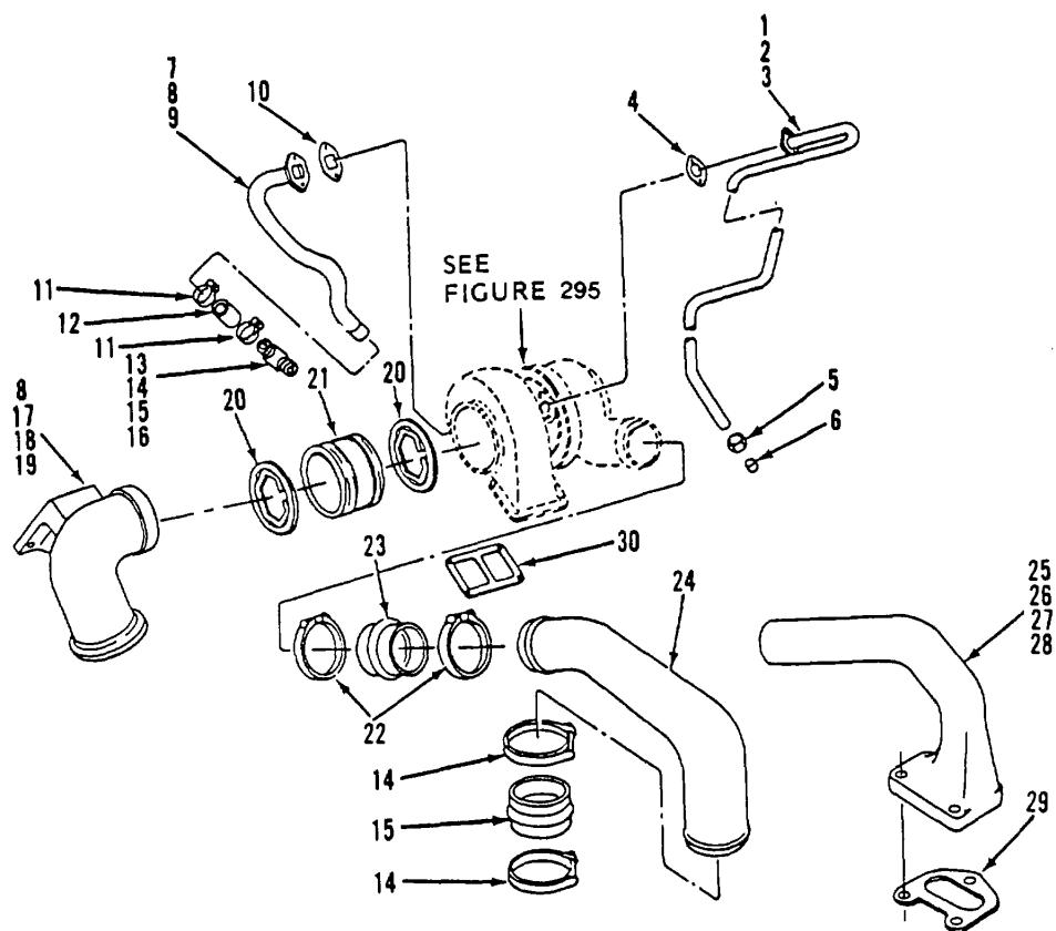
Figure 294. Turbocharger Piping
