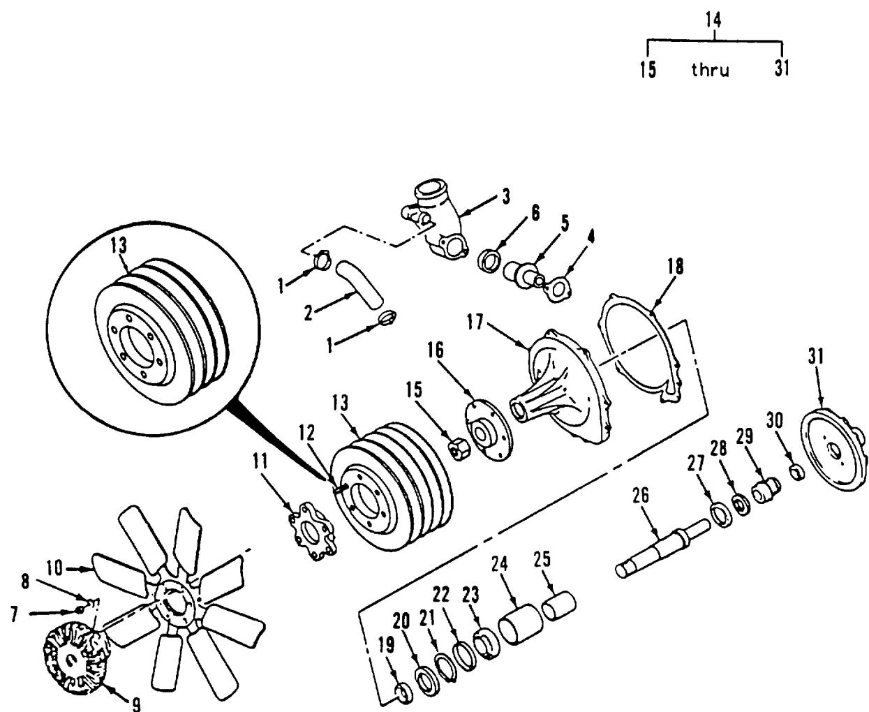
Figure 310. Water Pump and Fan Drive
