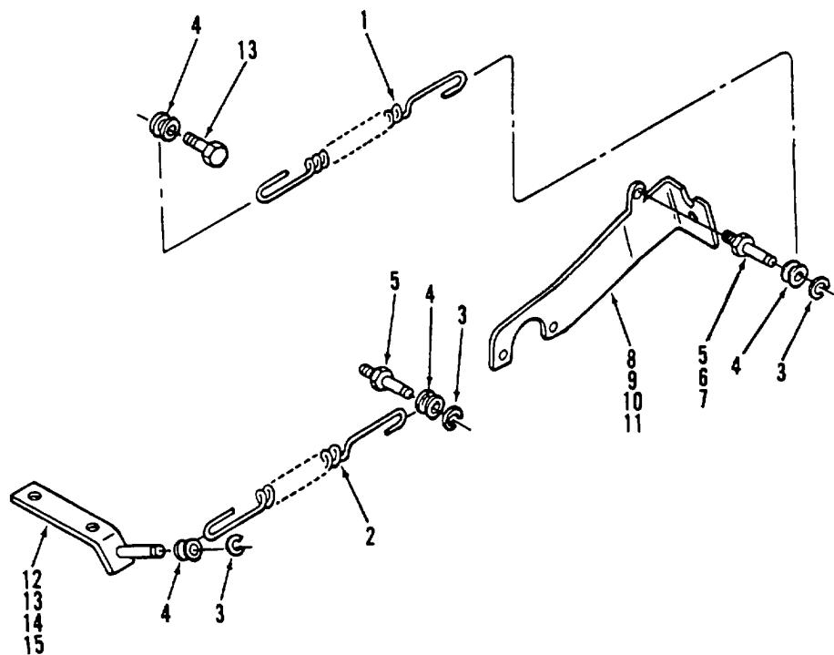
Figure 298. Fuel Pump Linkage
