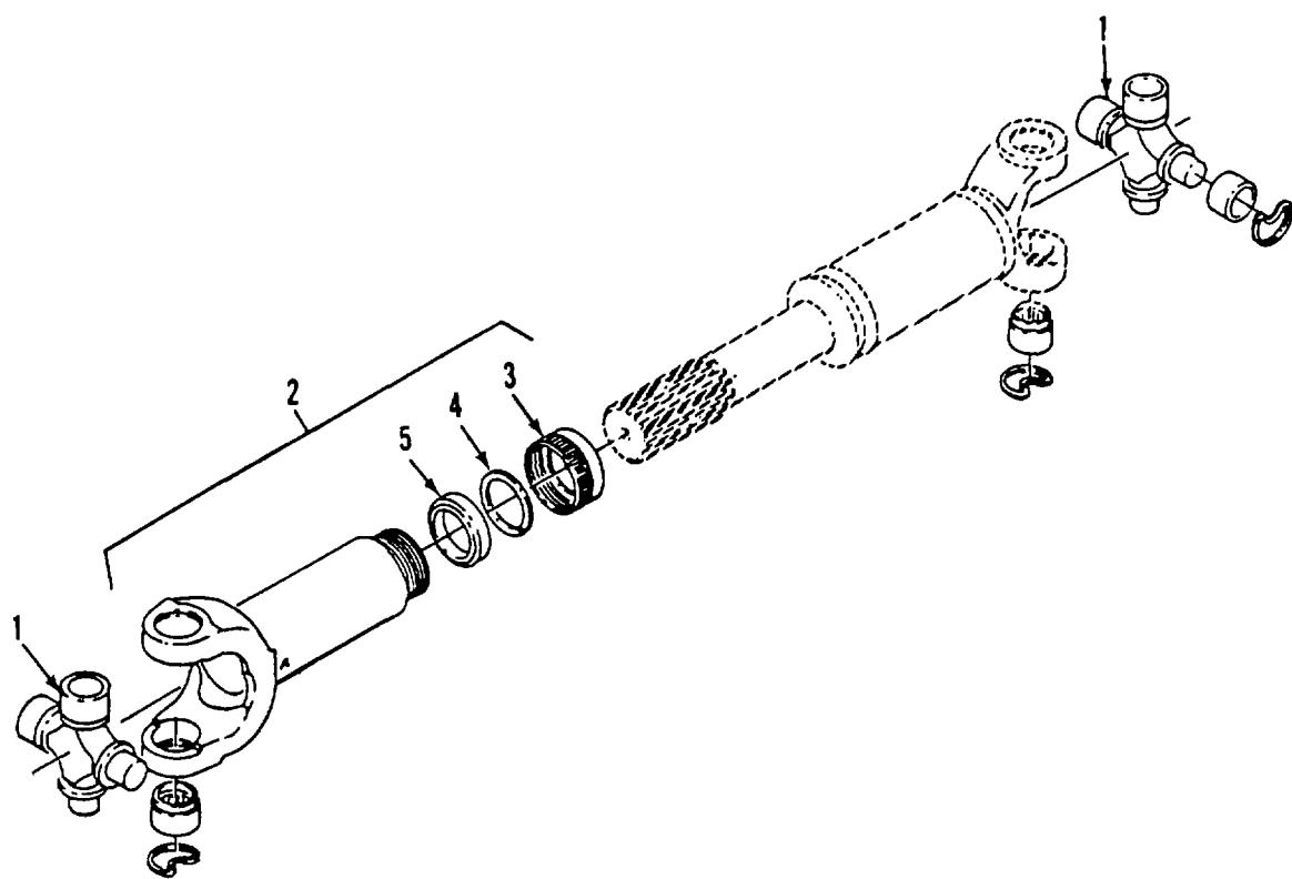
Figure 329. Driveshaft - Transfer Case to Front Axle
