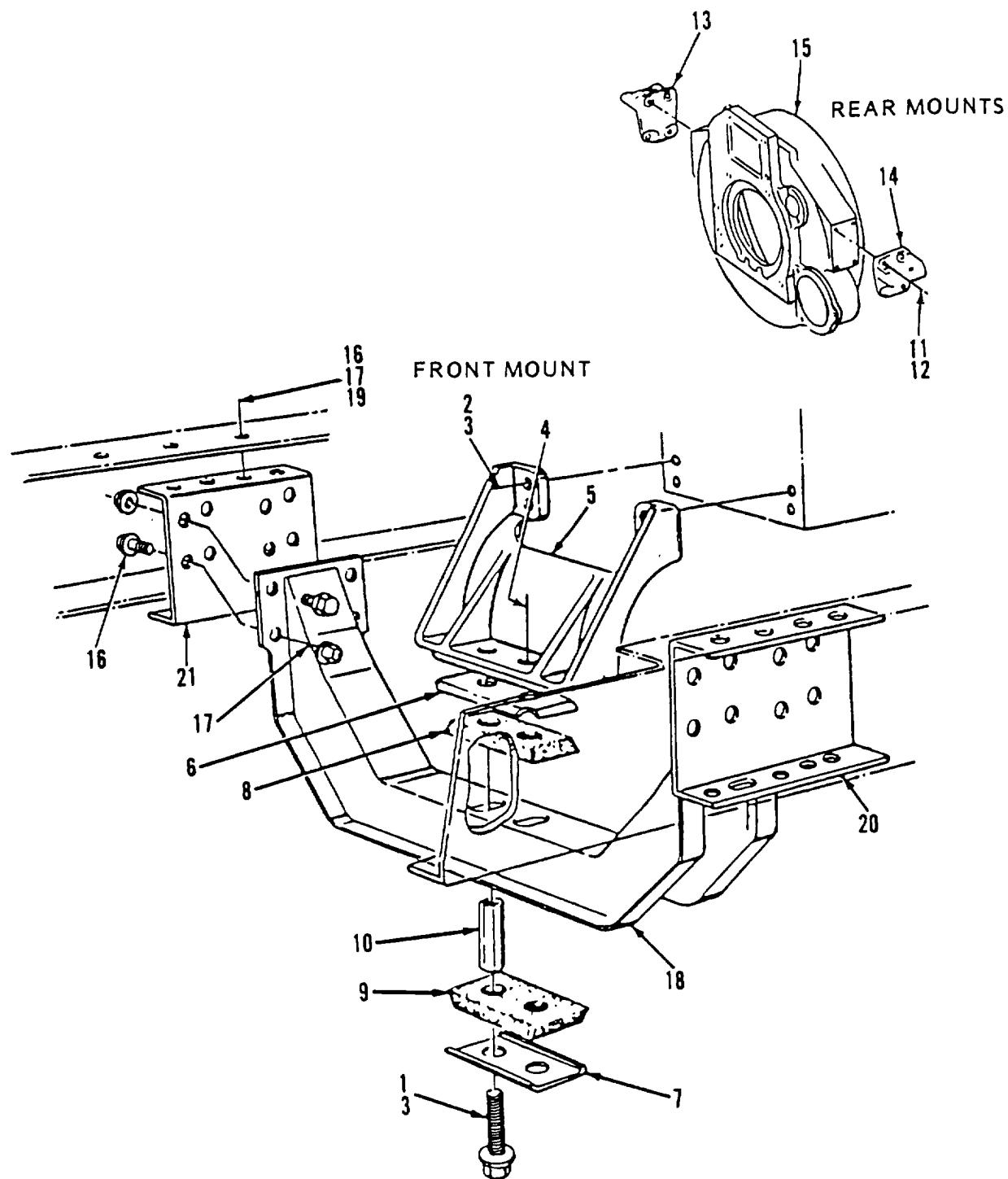
Figure 309. Engine Mounting
