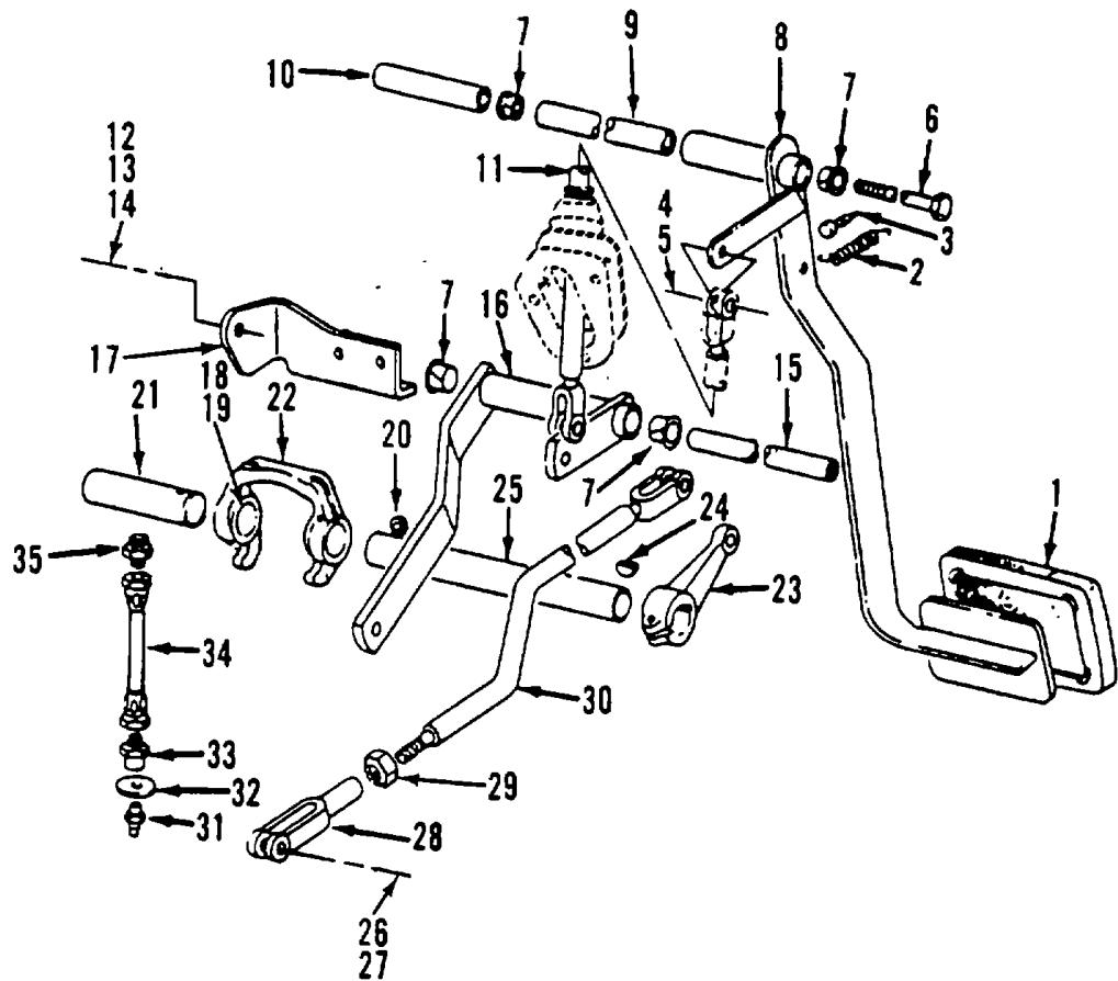
Figure 273. Clutch Control
