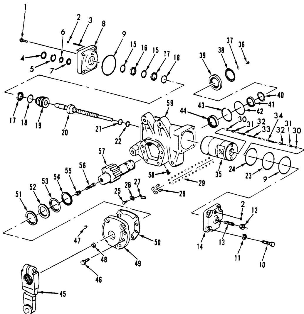
Figure 279. Steering Gear
