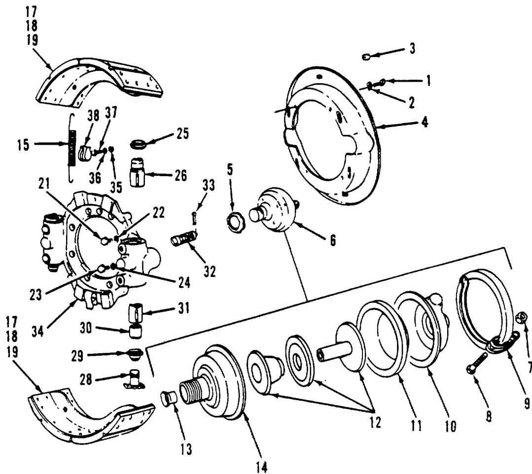
Figure 343. Left Front Brake Assembly
