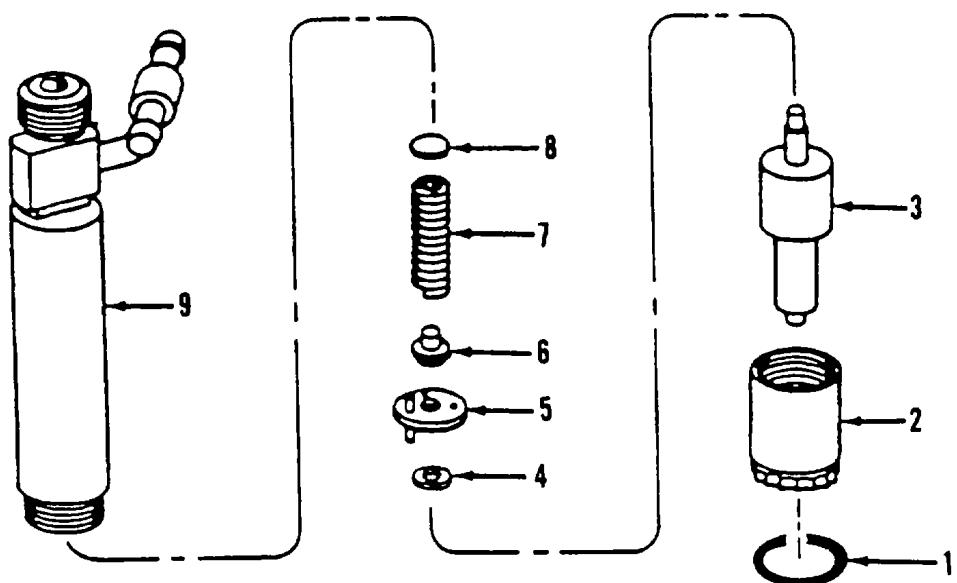
Figure 319. Fuel Injection Nozzle
