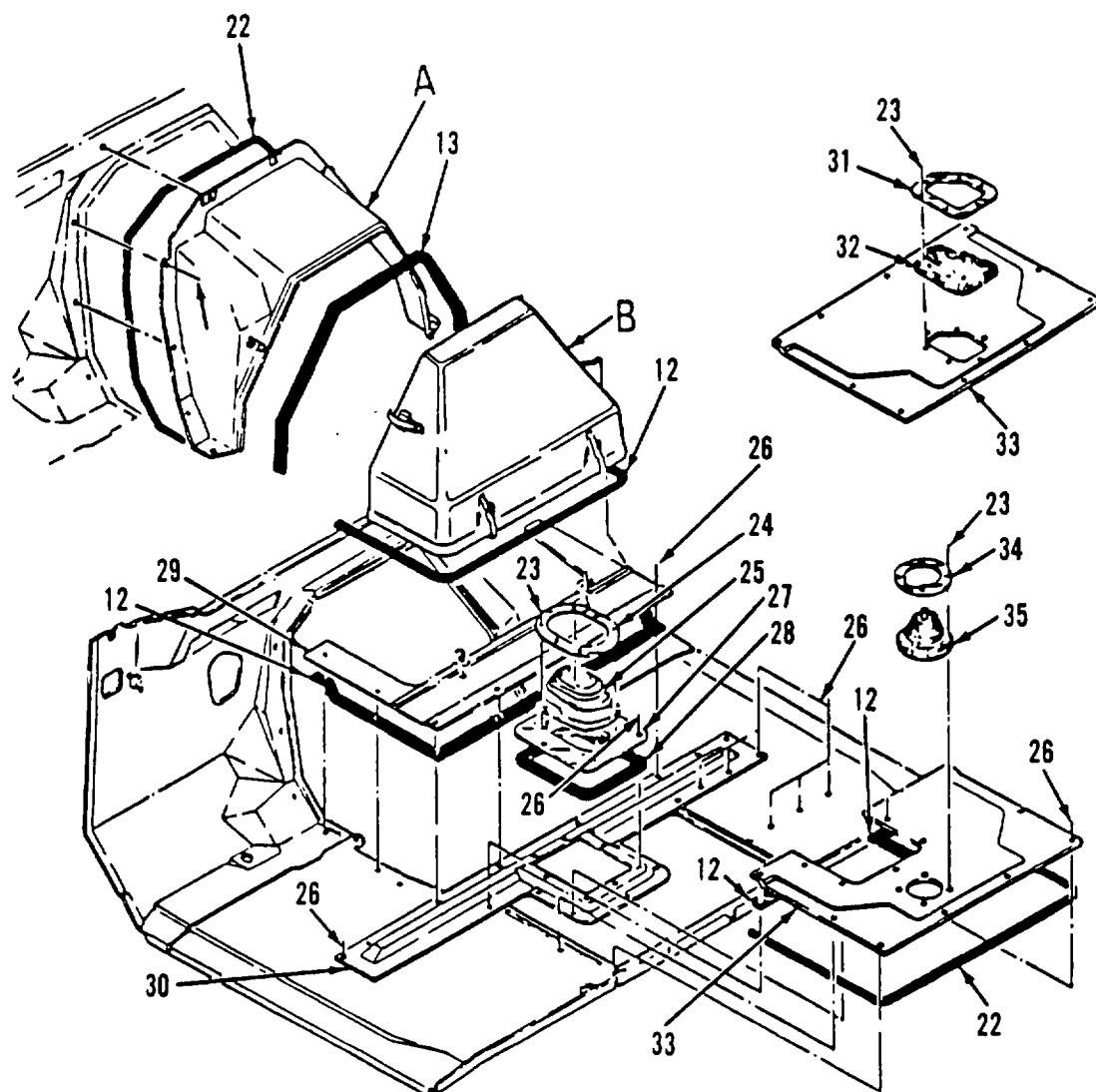
Figure 266. Engine and Transmission Cover (Sheet 1 of 2)
