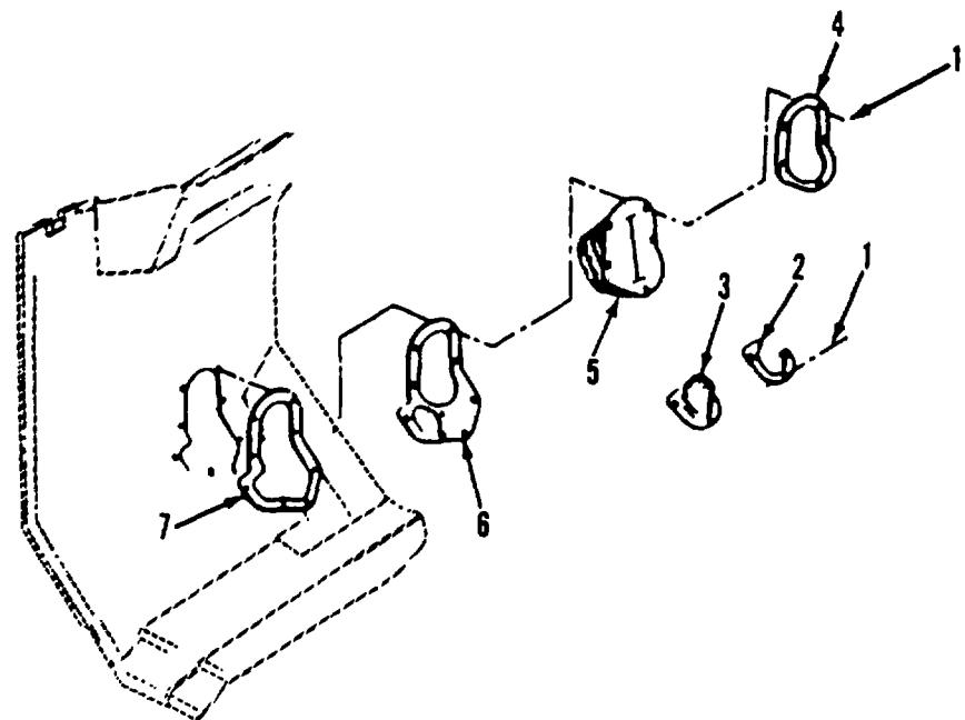
Figure 271. Steering Column and Clutch Shaft Seals
