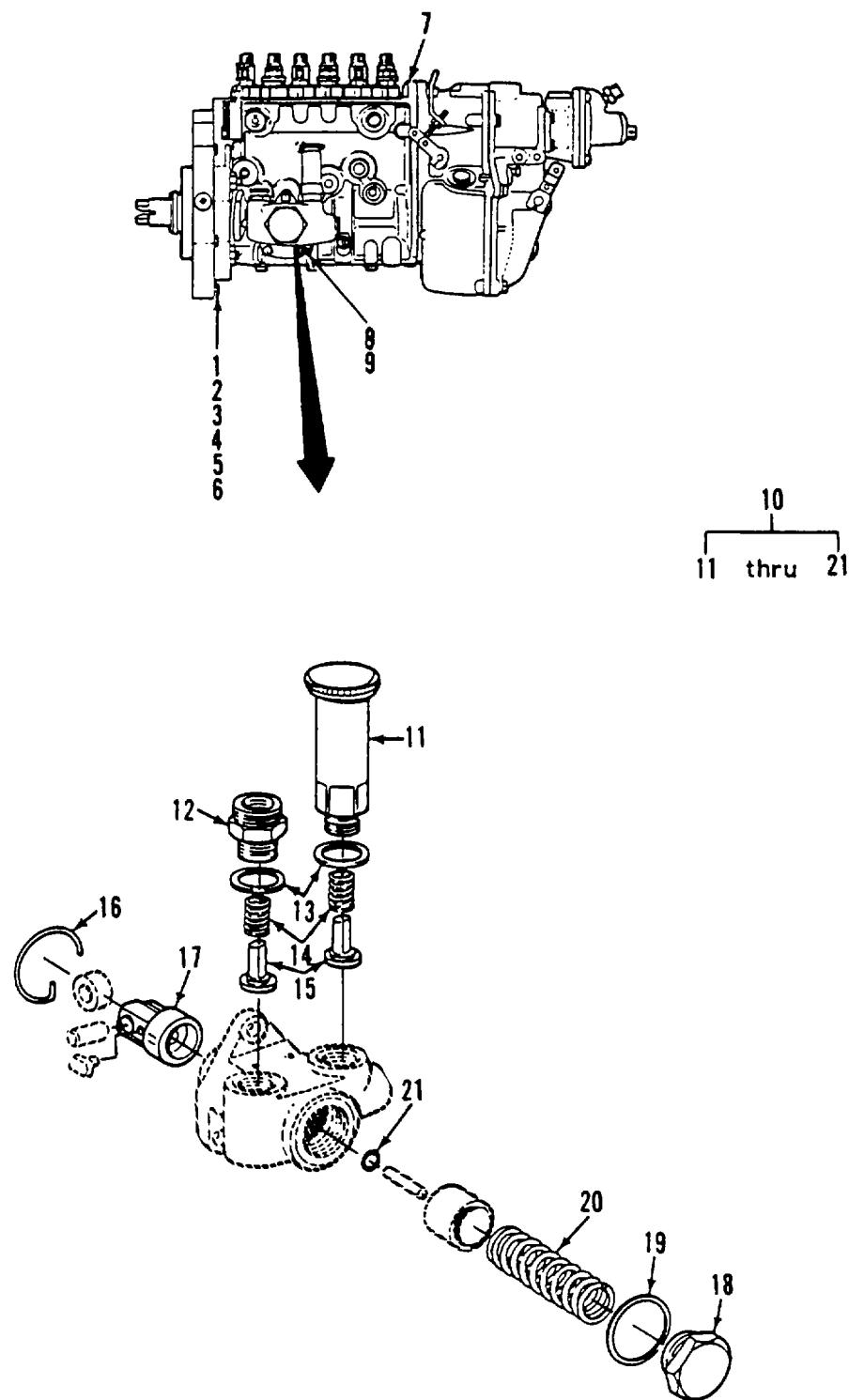
Figure 301. Injection Pump - Fuel Supply Pump
