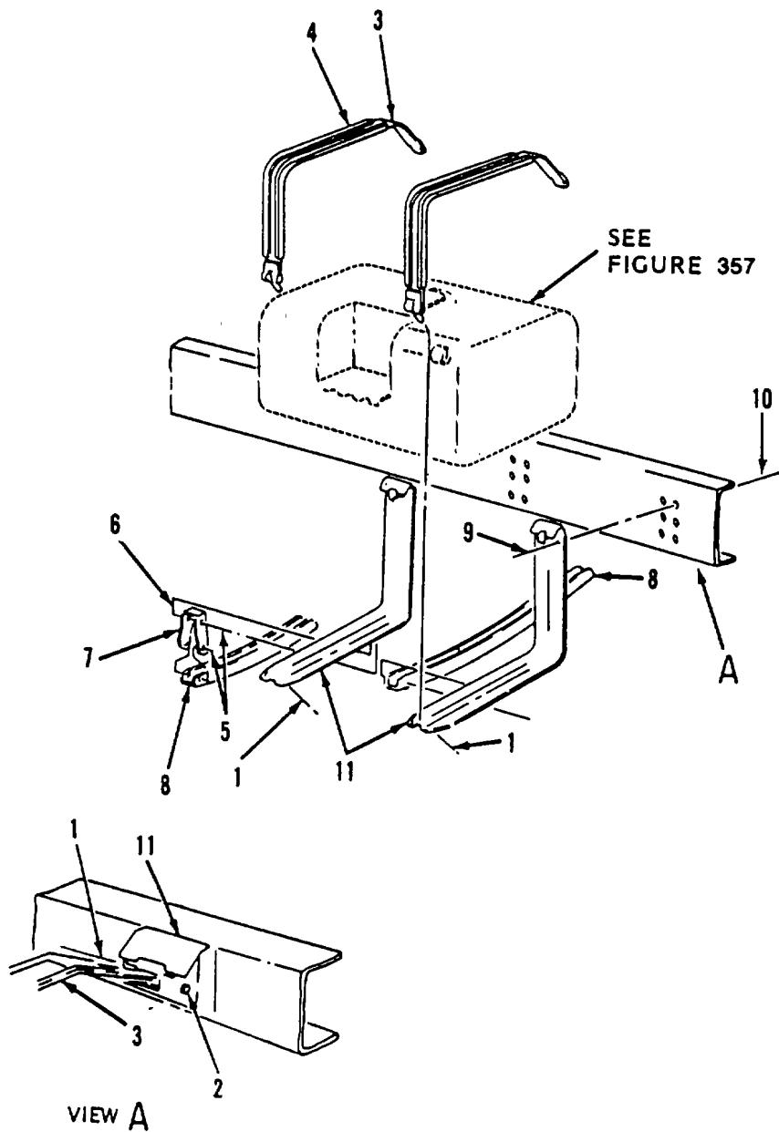
Figure 356. Fuel Tanks Installation
