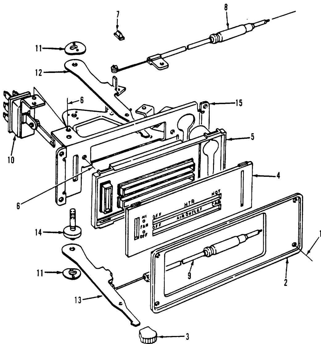
Figure 260. Heater Controls
