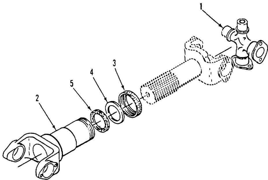
Figure 349. Driveshaft - Transfer Case to Rear Axle
