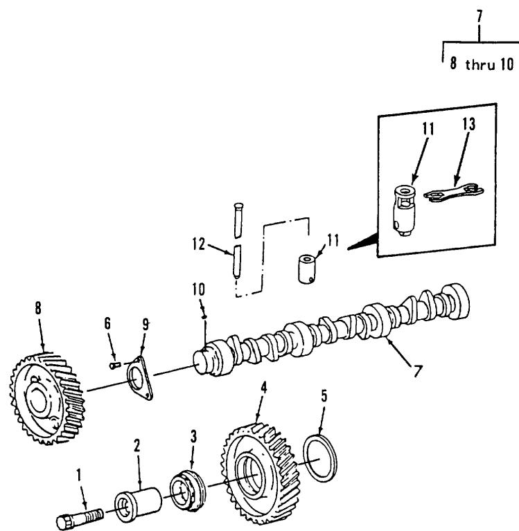
Figure 322. Camshaft and Related Parts
