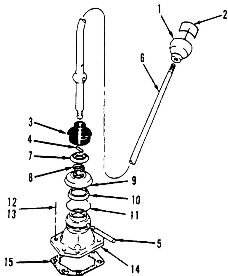
Figure 275. Transmission Control
