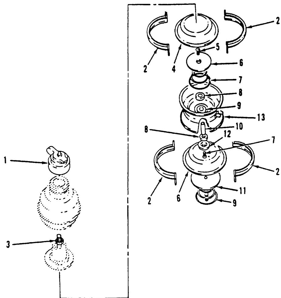
Figure 338. Air Brake Chamber - Forward Rear Axle
