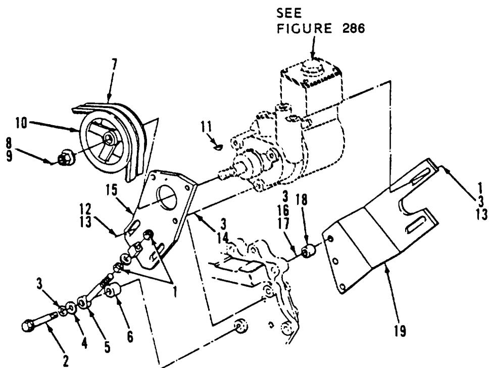
Figure 284. Steering Pump Installation
