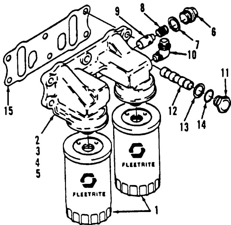
Figure 312. Oil Filter and Connection
