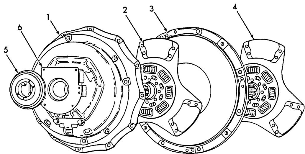
**Figure 333. Clutch Assembly**
