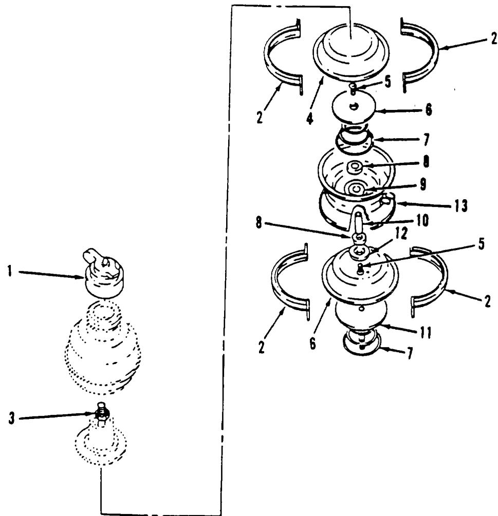
Figure 339. Air Brake Chamber - Rear Rear Axle
