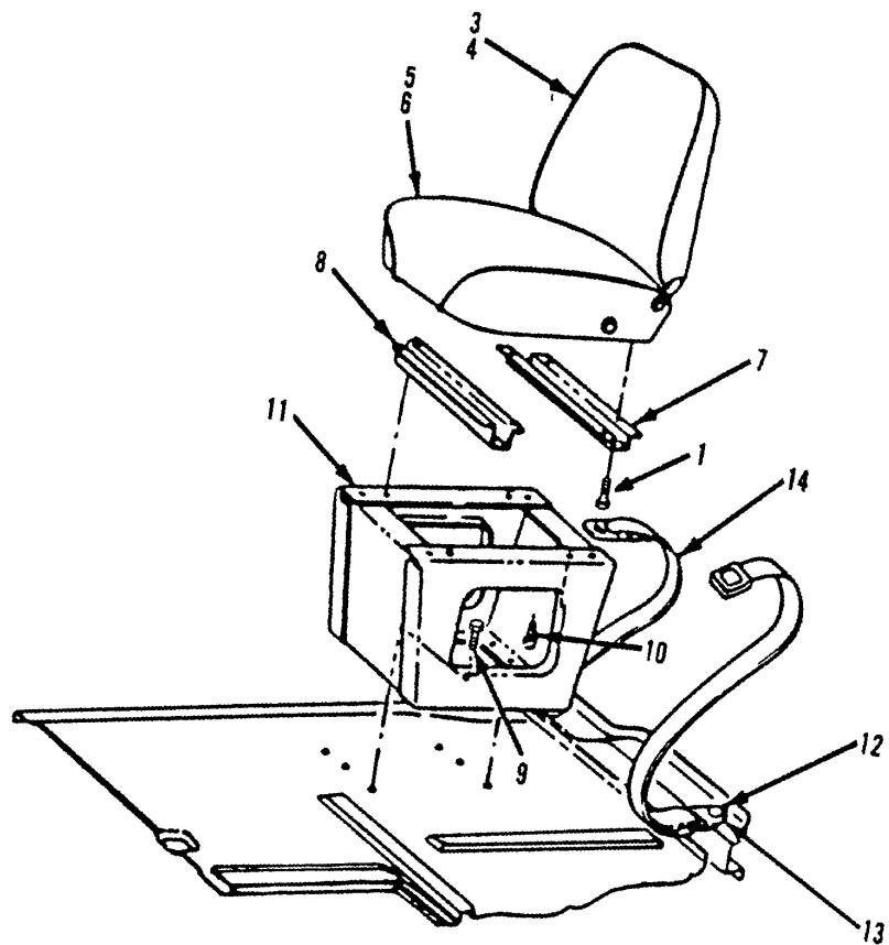
Figure 264. Passenger Seat Installation
