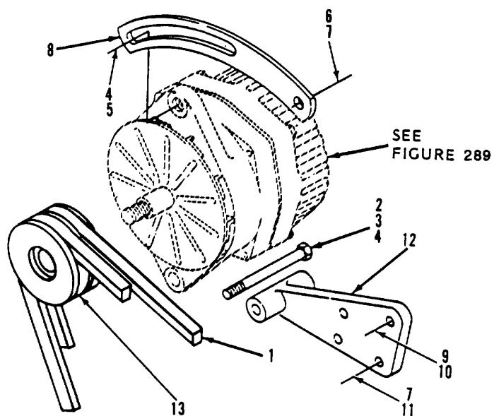
Figure 288. Alternator Mounting
