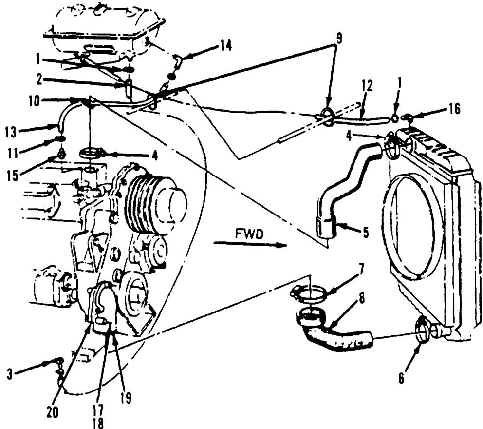
Figure 281. Radiator Hose Installation
