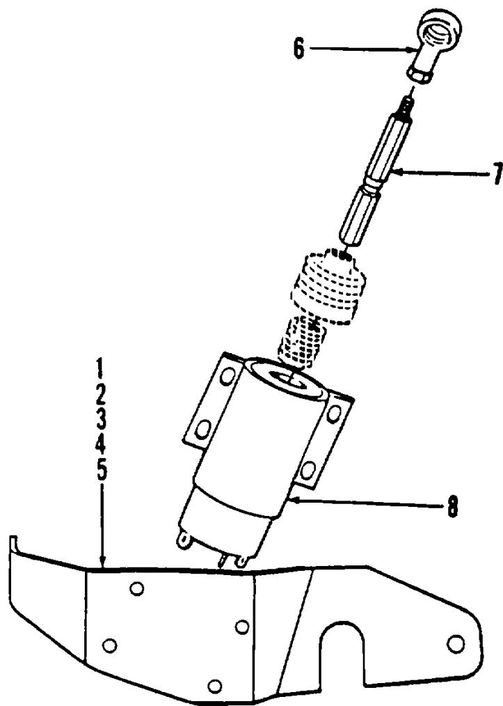
Figure 299. Fuel Pump Solenoid
