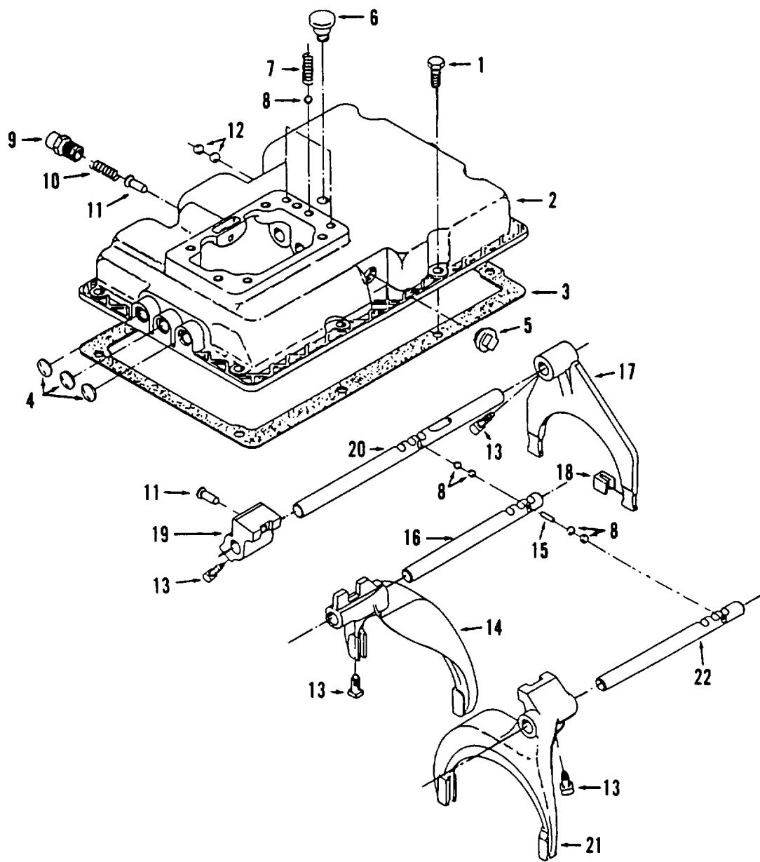
Figure 327. Transmission Assembly (Sheet 1 of 3)
