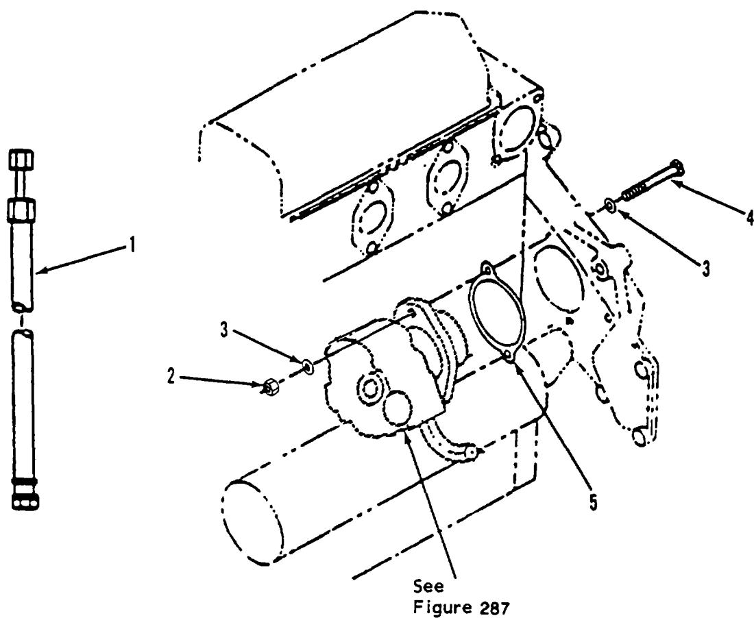
Figure 285. Steering Pump Installation
