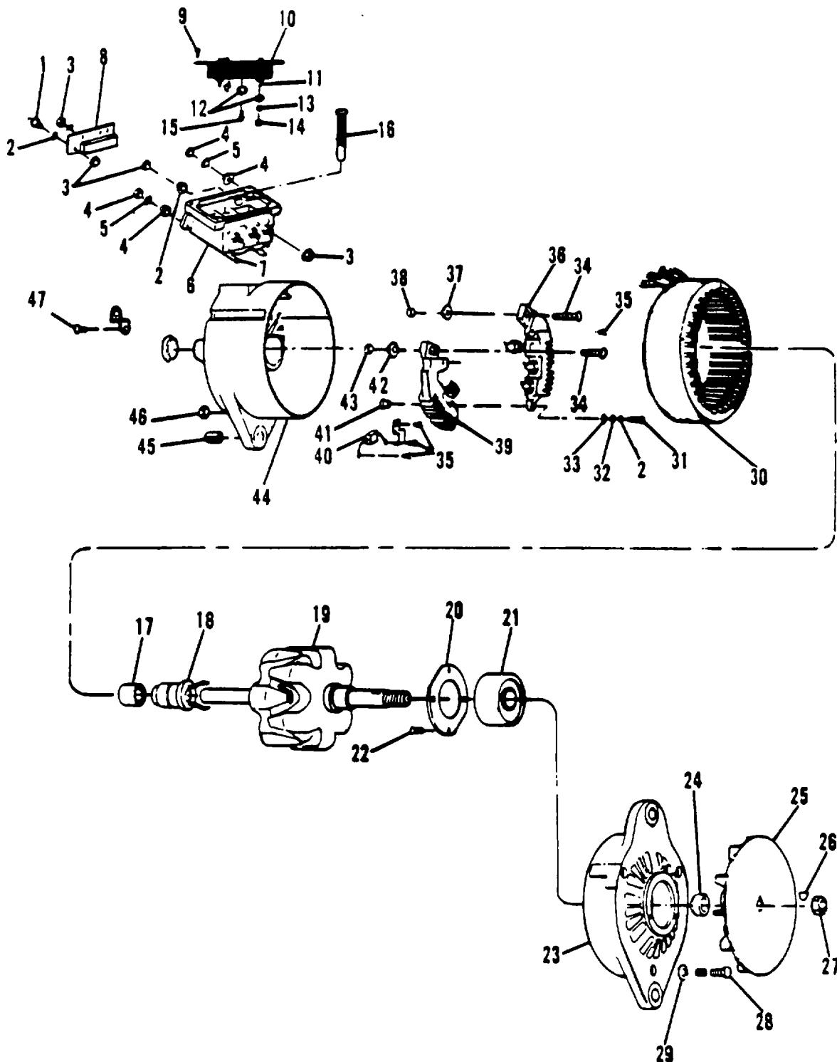
Figure 289. Alternator Assembly
