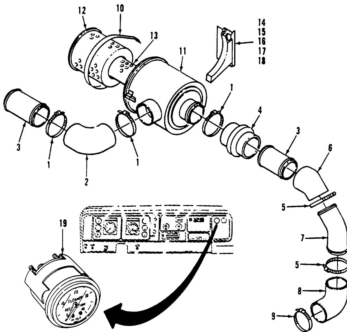
Figure 292. Air Cleaner and Mounting
