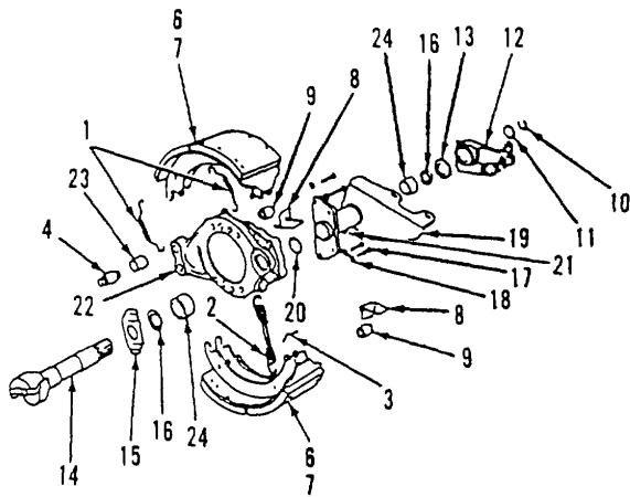
Figure 346. Right Forward Rear Brake Assembly
