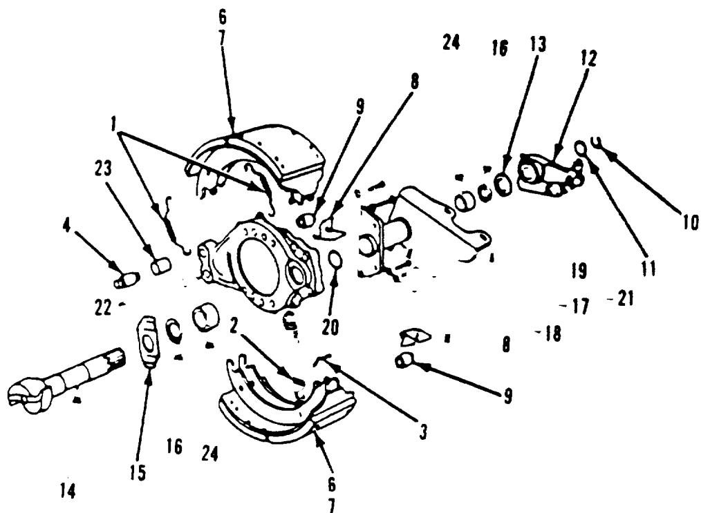
Figure 345. Left Forward Rear Brake Assembly
