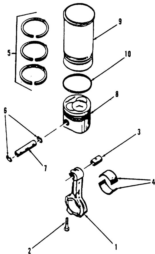
Figure 323. Piston and Connecting Rod
