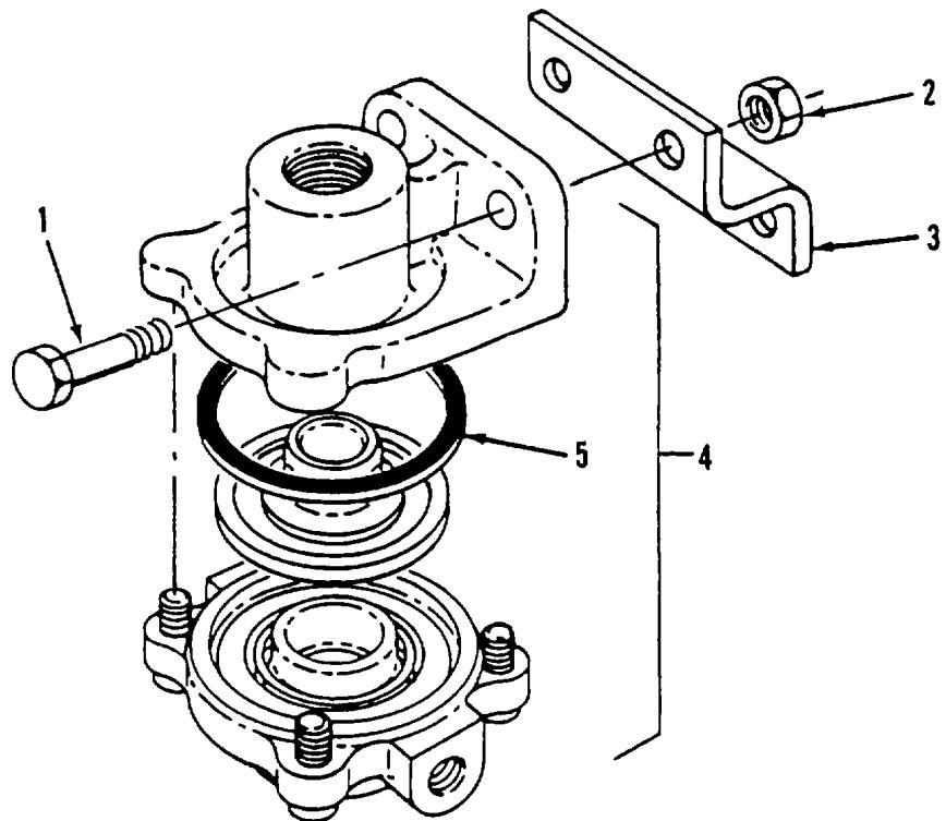
Figure 337. Quick Release Valve
