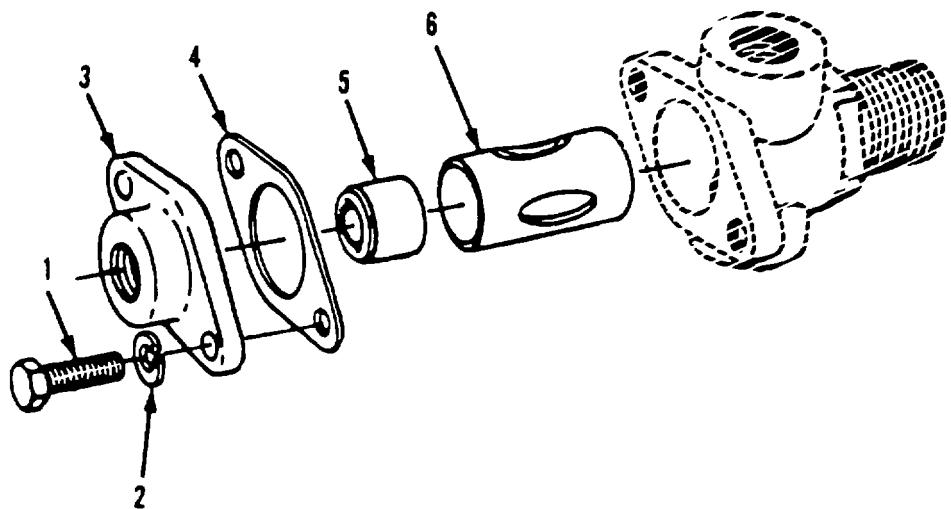
Figure 336. Double Check Valve
