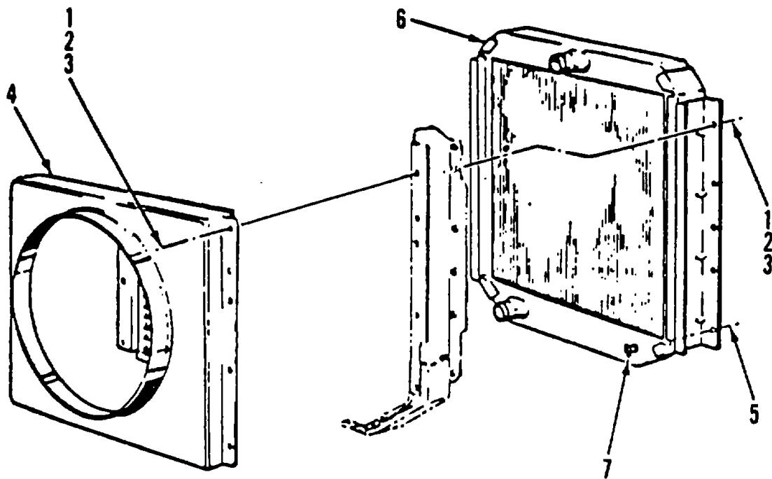
Figure 283. Radiator Installation (Sheet 1 of 2)
