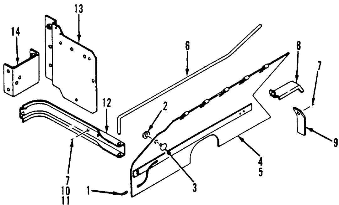
Figure 256. Splash Guard Installation
