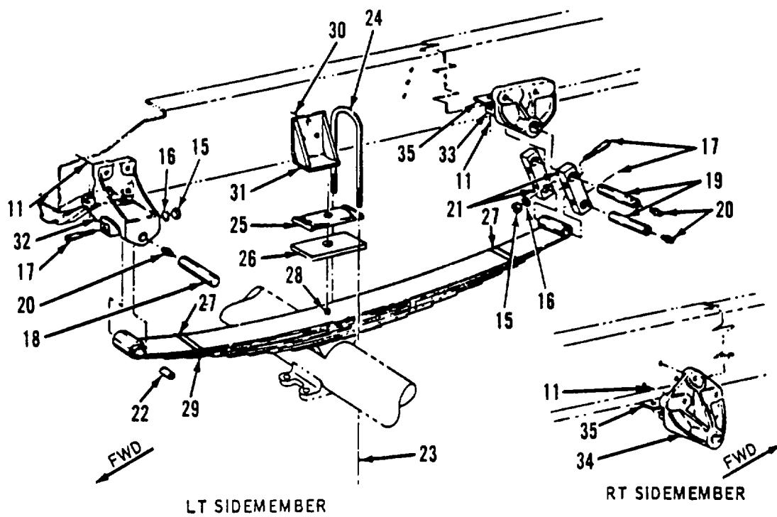
Figure 355. Front Springs and Shocks
