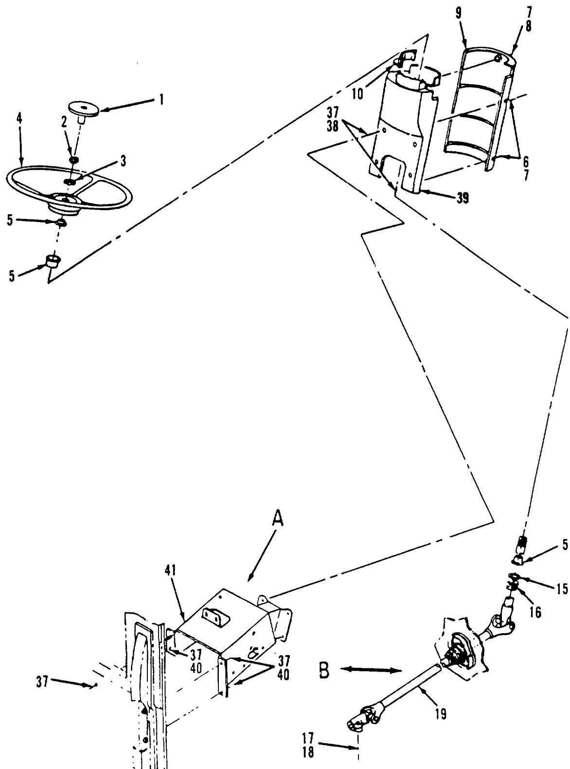
Figure 276. Steering Column Installation (Sheet 1 of 2)
