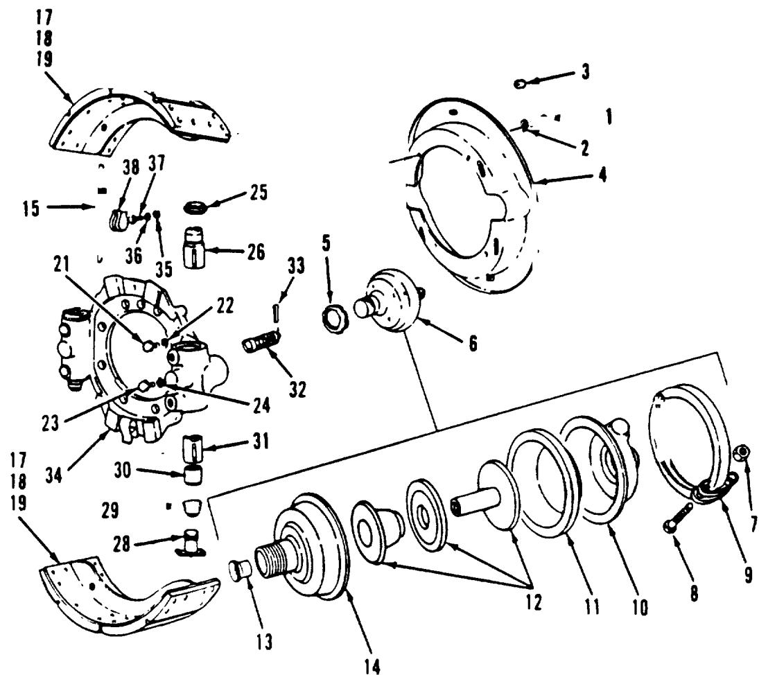
Figure 344. Right Front Brake Assembly
