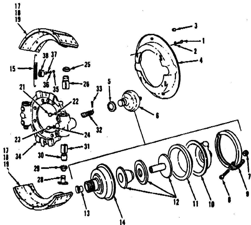
Figure 179. Right Front Brake Assembly
