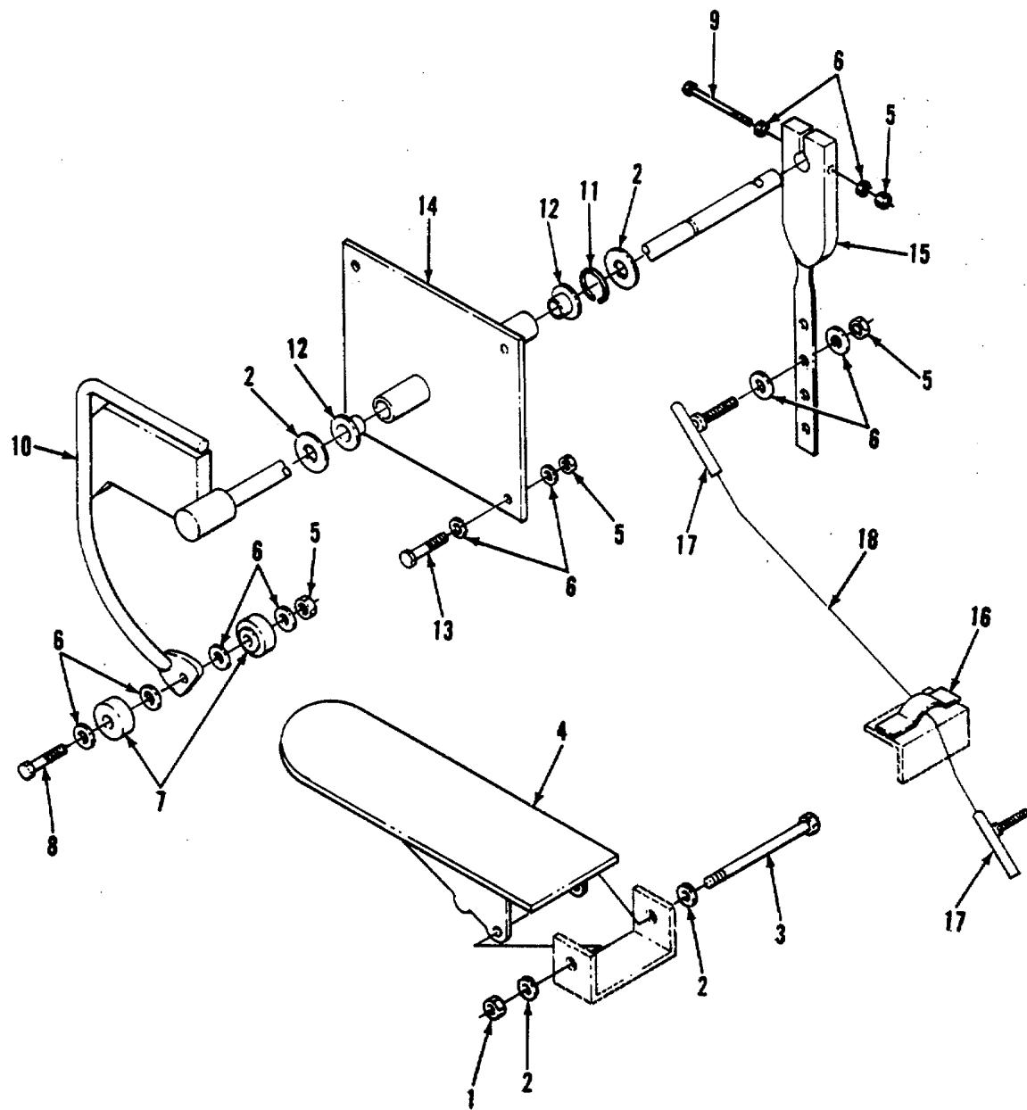
Figure 108. Accelerator Pedal Installation
