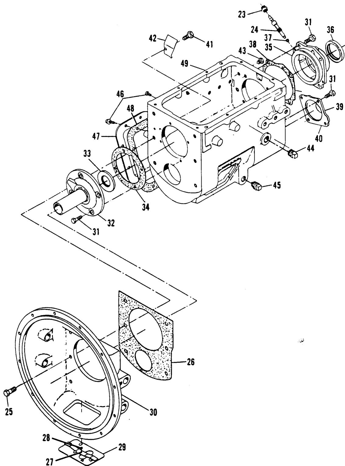
Figure 162. Transmission Assembly (Sheet 2 of 3)
