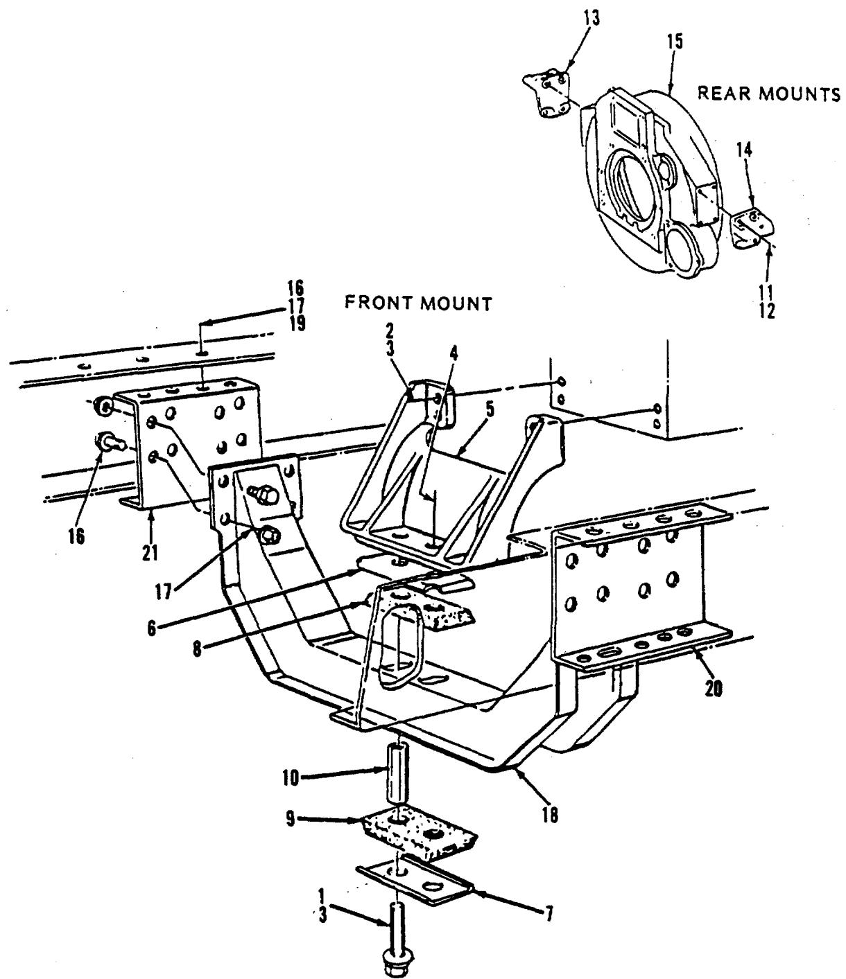
Figure 144. Engine Mounting
