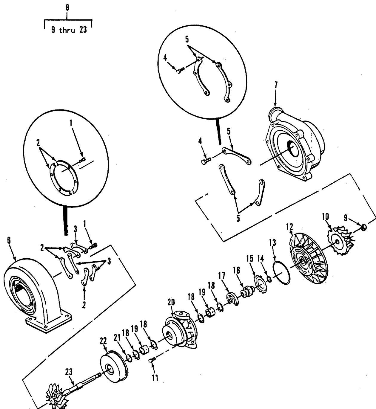
Figure 130. Turbocharger Assembly
