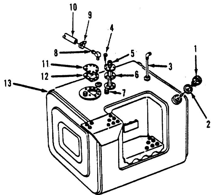
Figure 192. Fuel Tank Assembly
