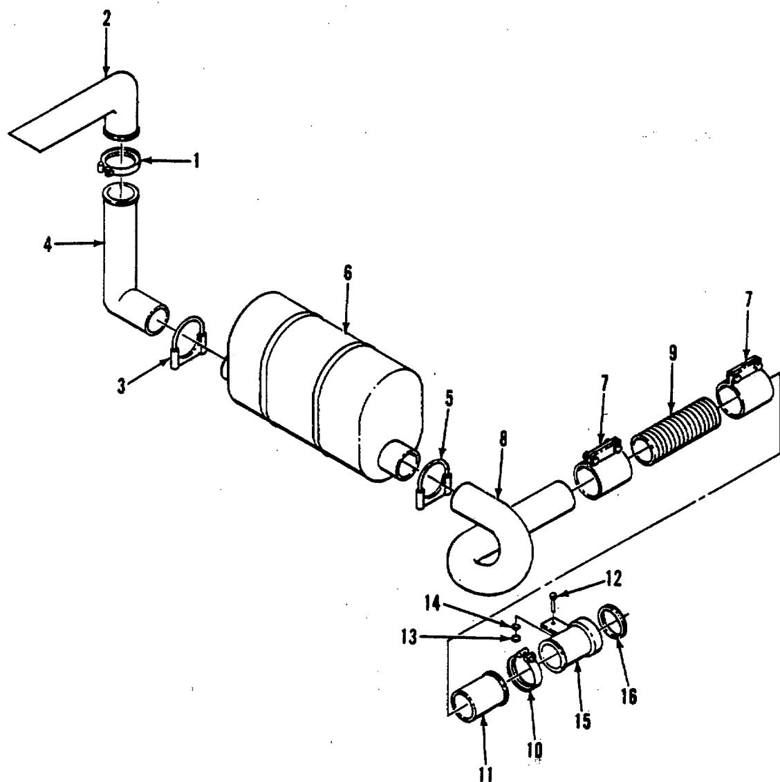
Figure 115. Exhaust System Installation
