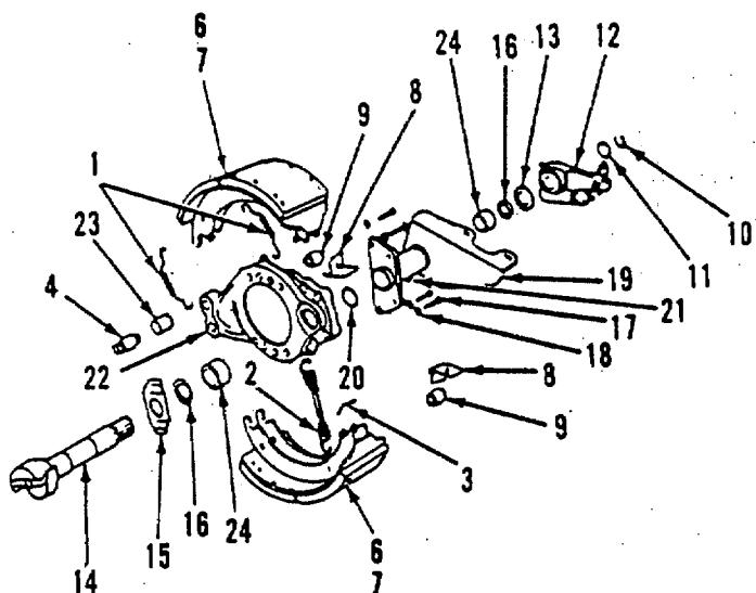
Figure 183. Right Rear Brake Assembly
