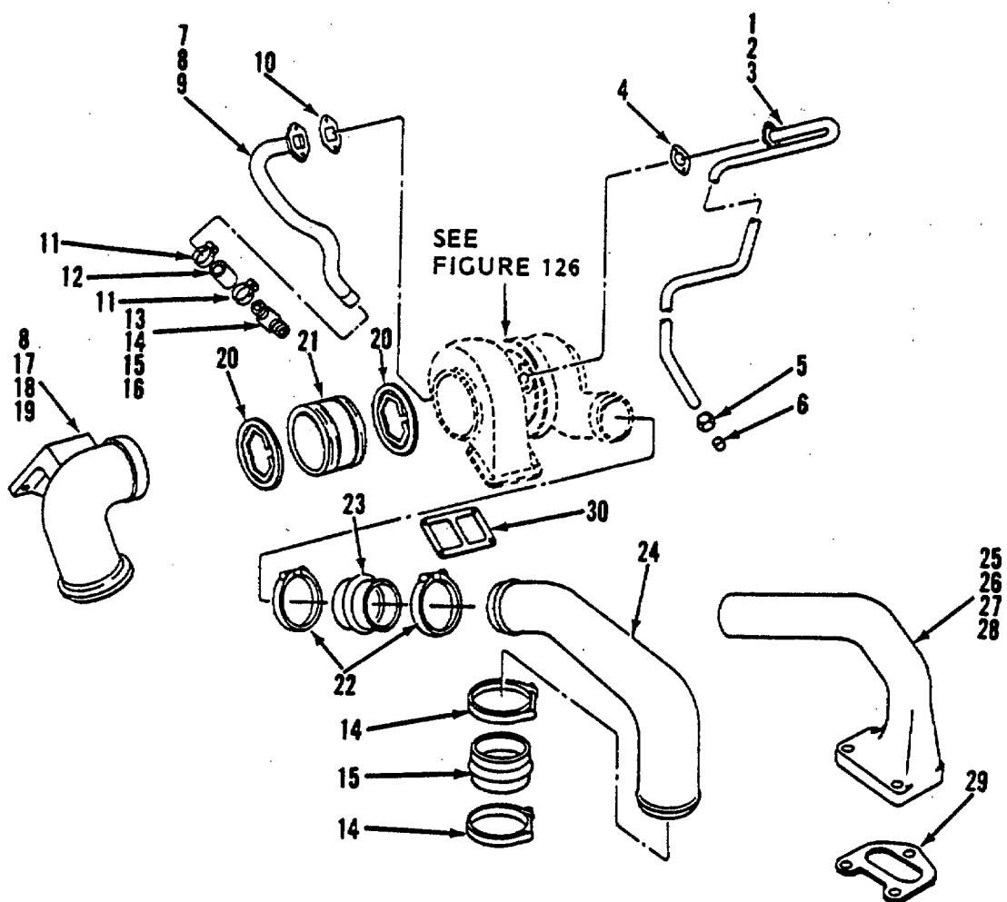
Figure 129. Turbocharger Piping
