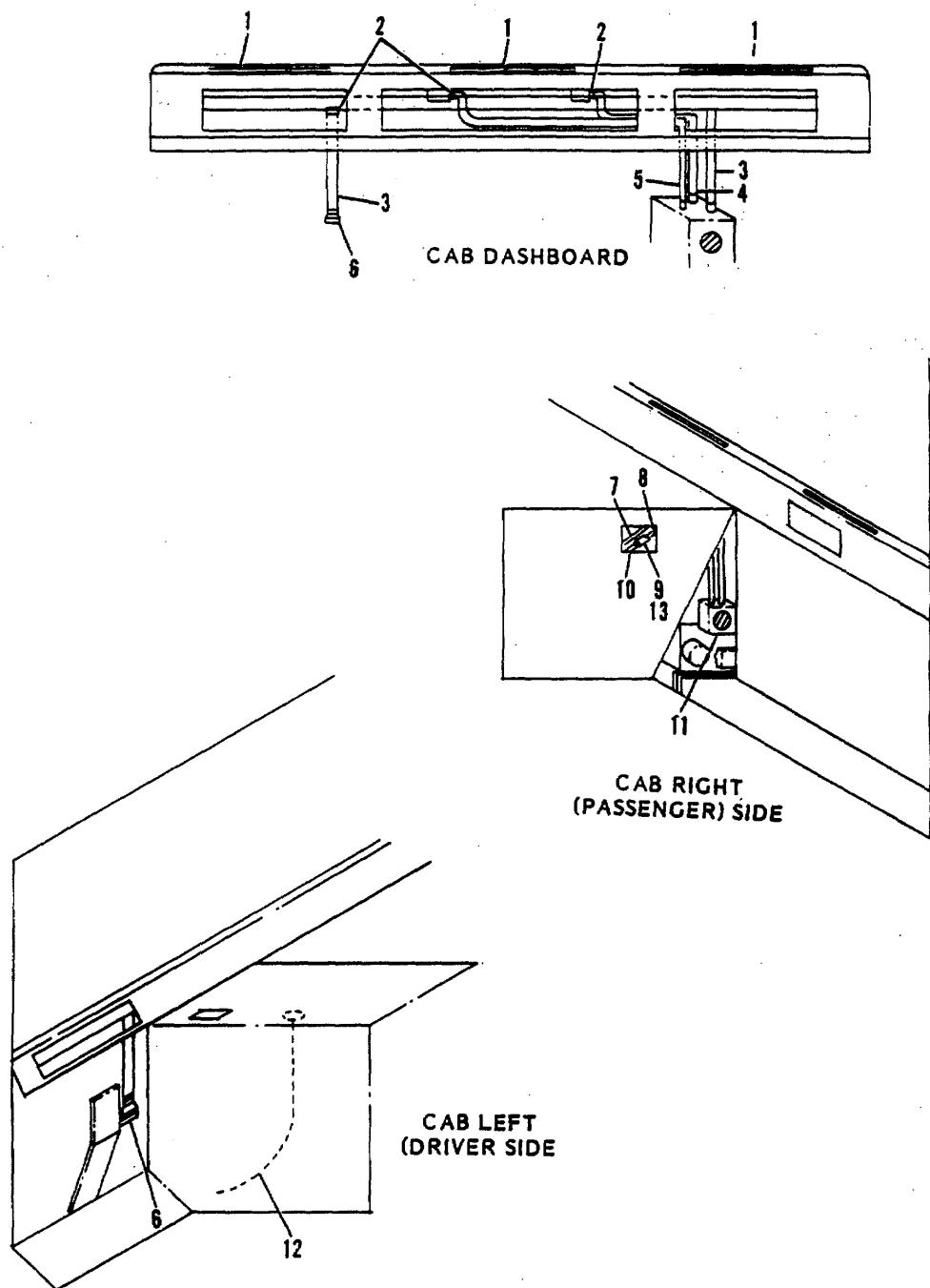
Figure 104. Heater/Defroster Connections
