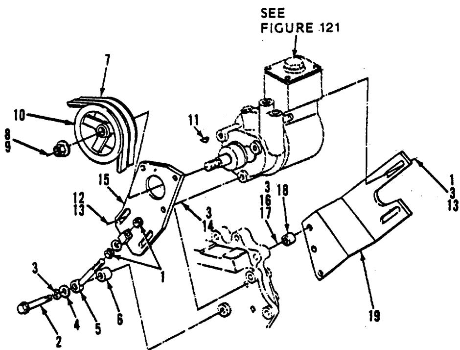
Figure 119. Steering Pump Installation
