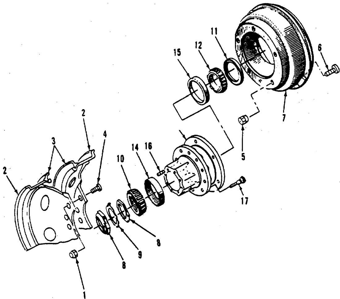
Figure 177. Rear Wheel, Hub and Drum
