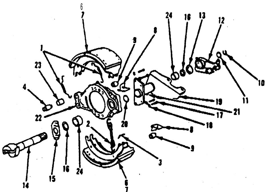
Figure 180. Left Forward Rear Brake
