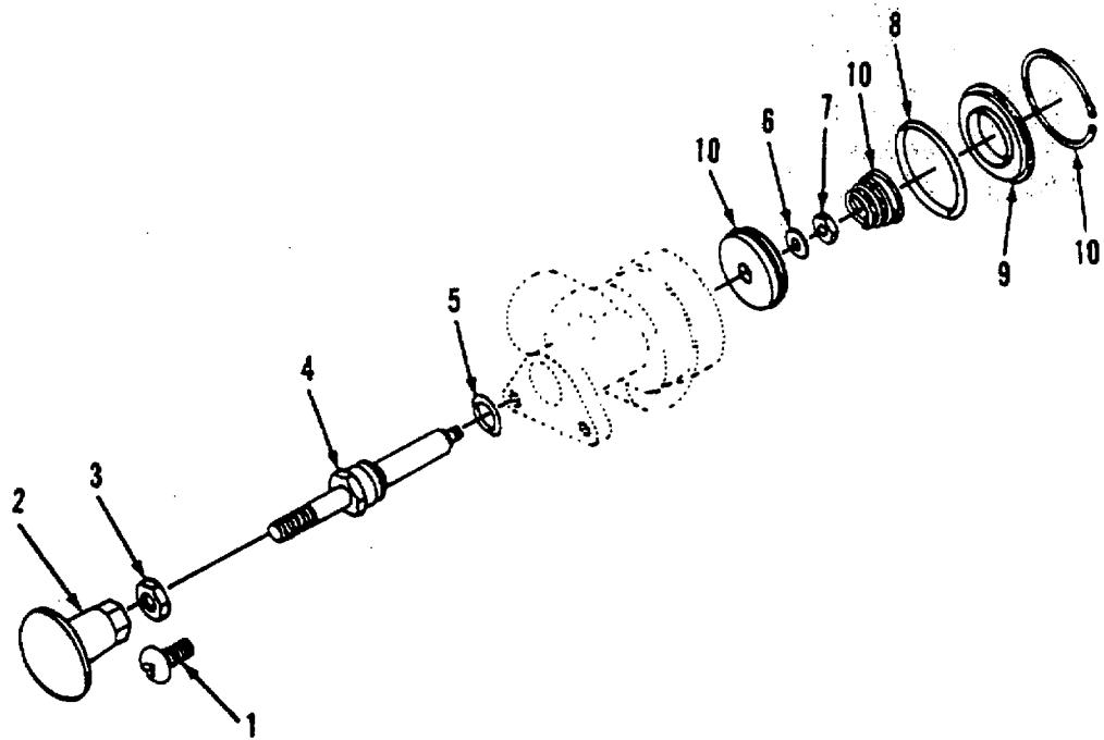
Figure 170. Parking Brake Control Valve
