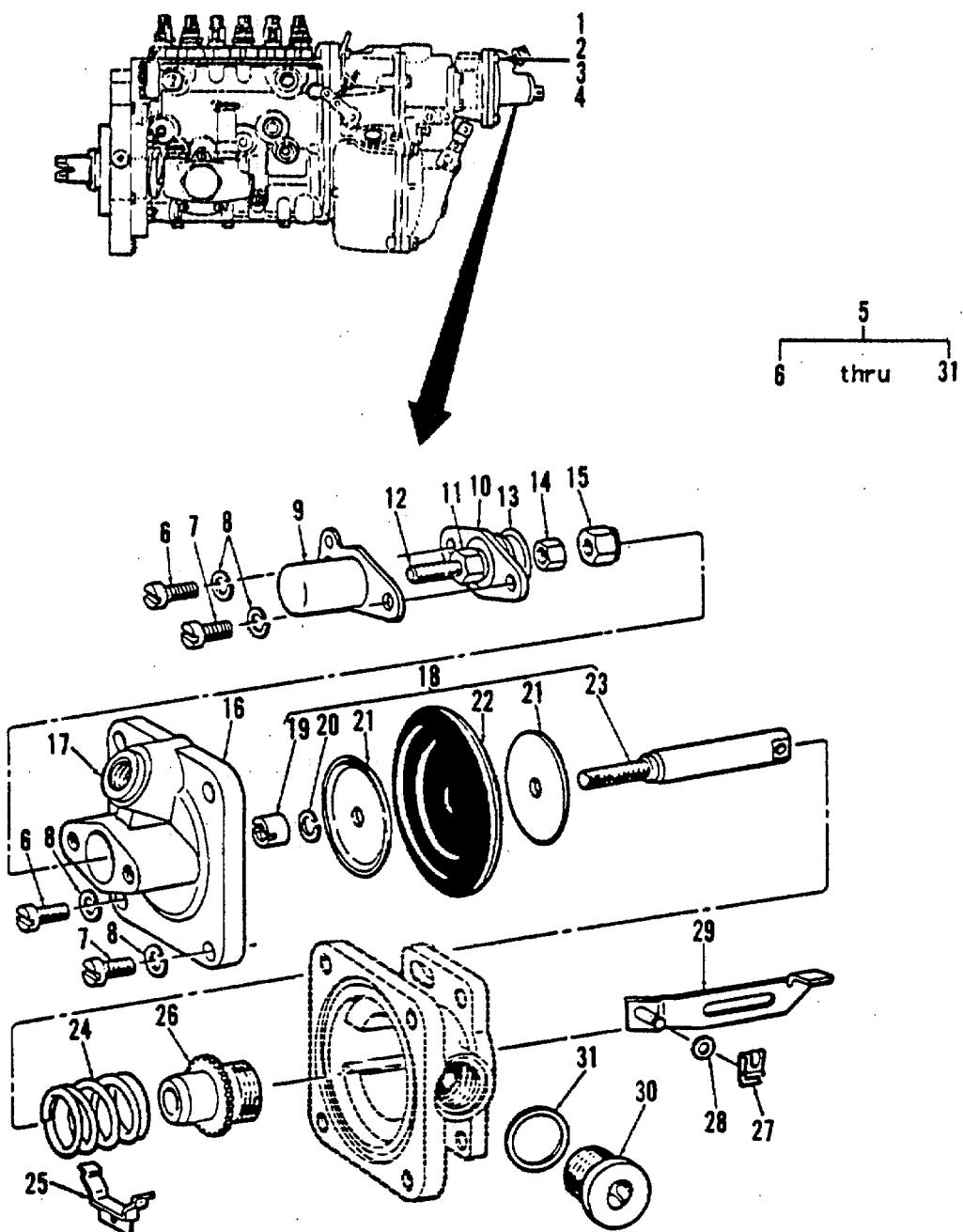
Figure 137. Fuel Injection Pump- Aneroid
