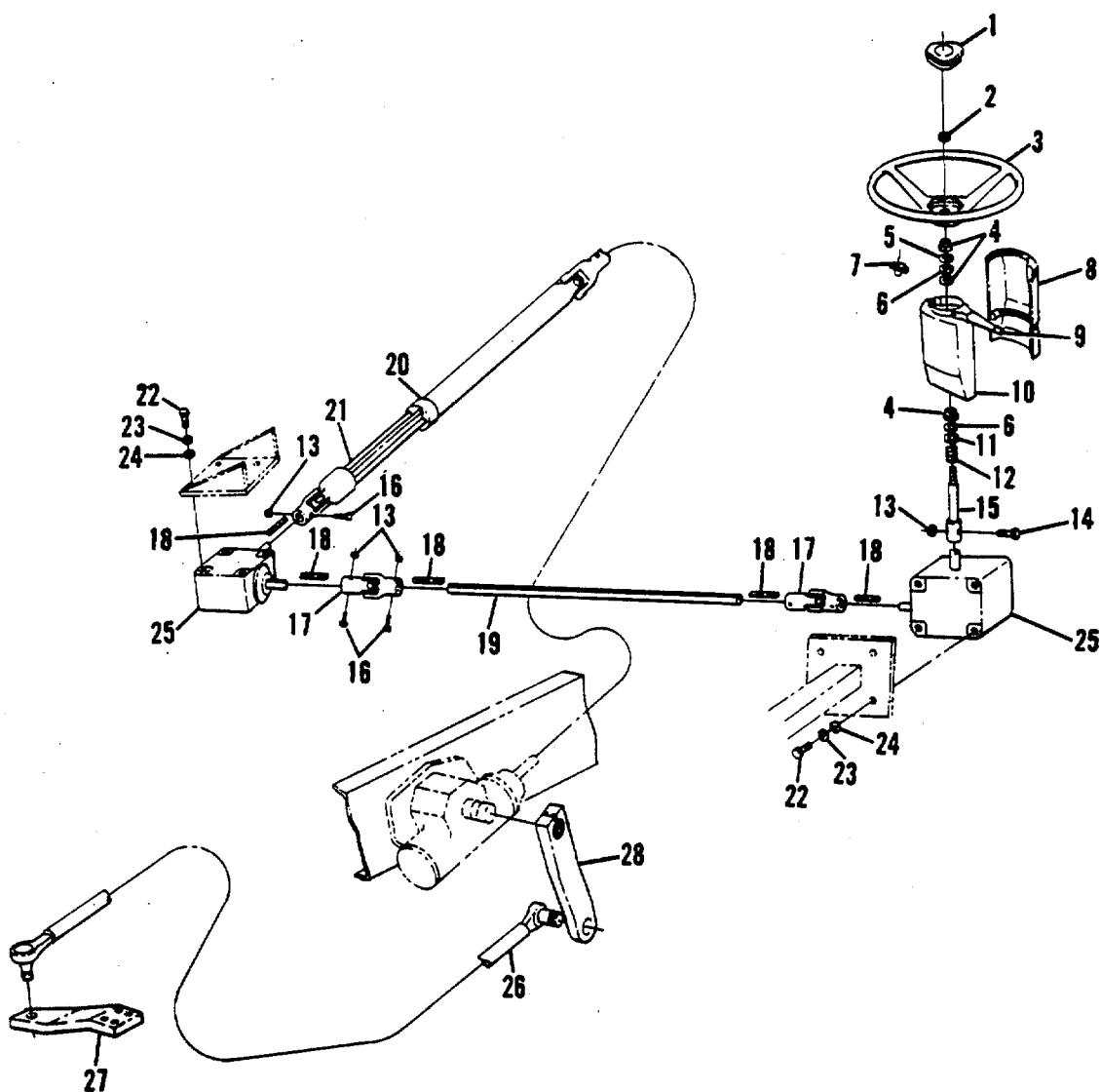
Figure 110. Steering Installation
