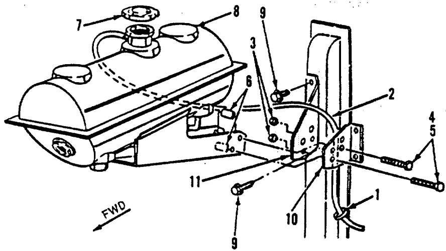
Figure 117. Deaeration Tank Installation
