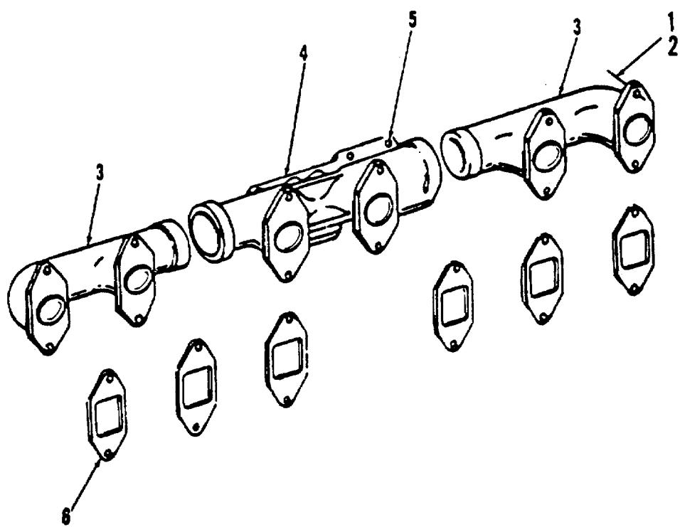
Figure 150. Exhaust Manifold
