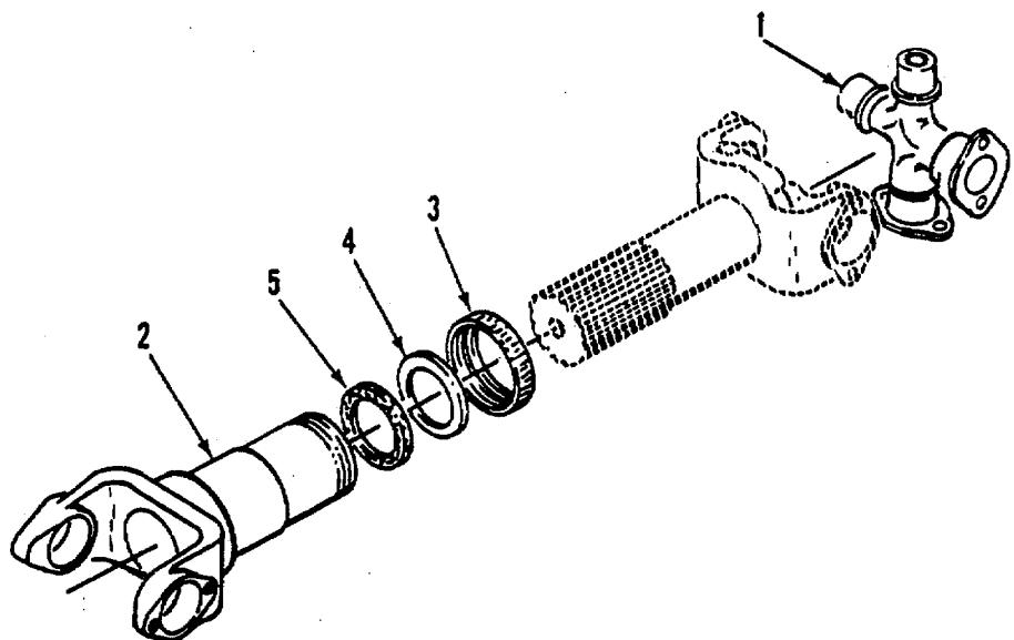
Figure 185. Driveshaft-Rear Interaxle
