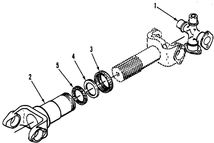
*Figure 163. Driveshaft - Transmission to Transfer Case*
