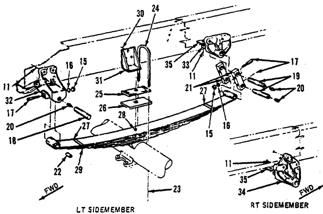
Figure 190. Front Springs and Shocks
