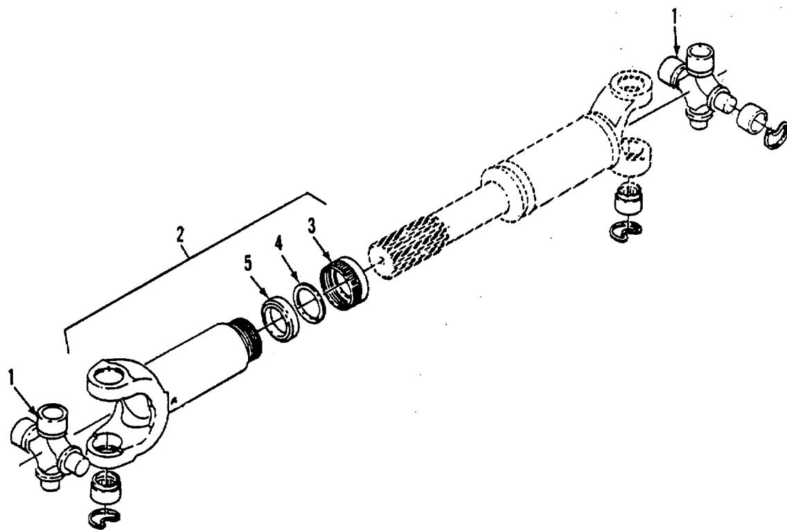
Figure 164. Driveshaft - Transfer Case to Front Axle
