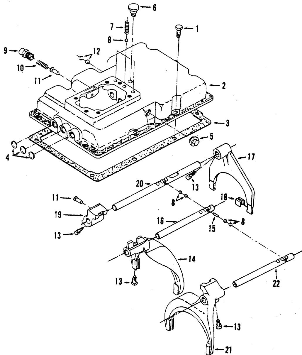
Figure 162. Transmission Assembly (Sheet 1 of 3)
