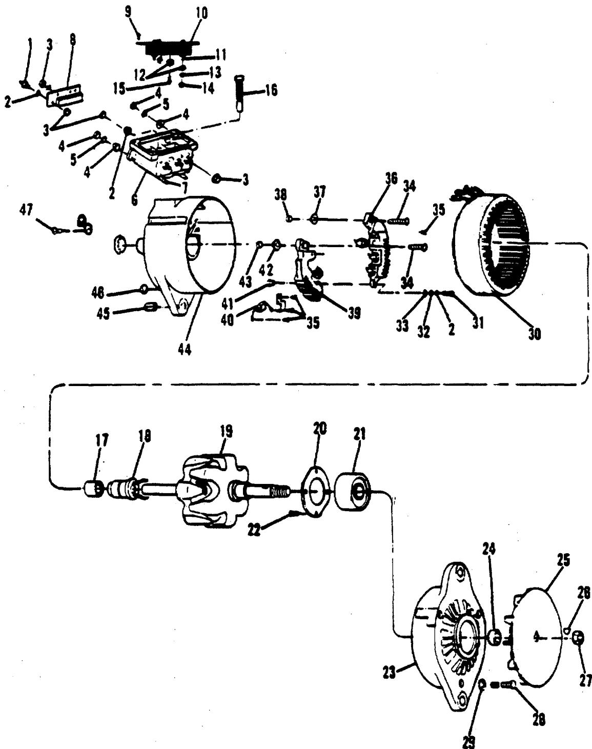
Figure 124. Alternator Assembly
