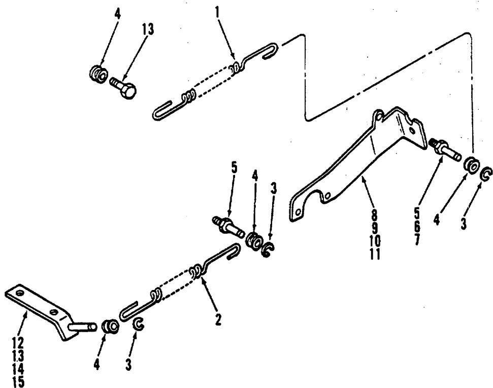
Figure 133. Fuel Pump Linkage
