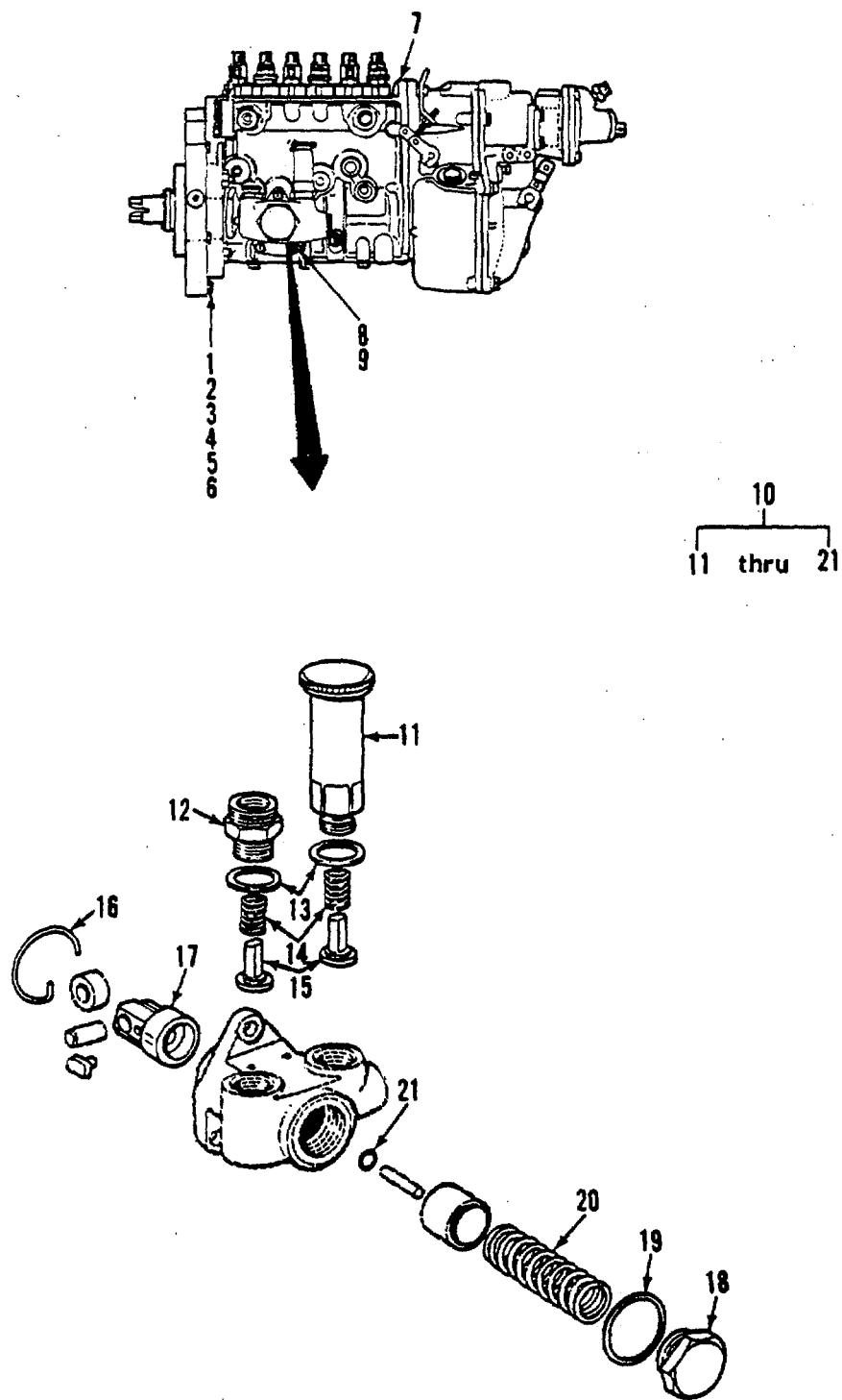
Figure 136. Fuel Injection Pump - Fuel Supply Pump
