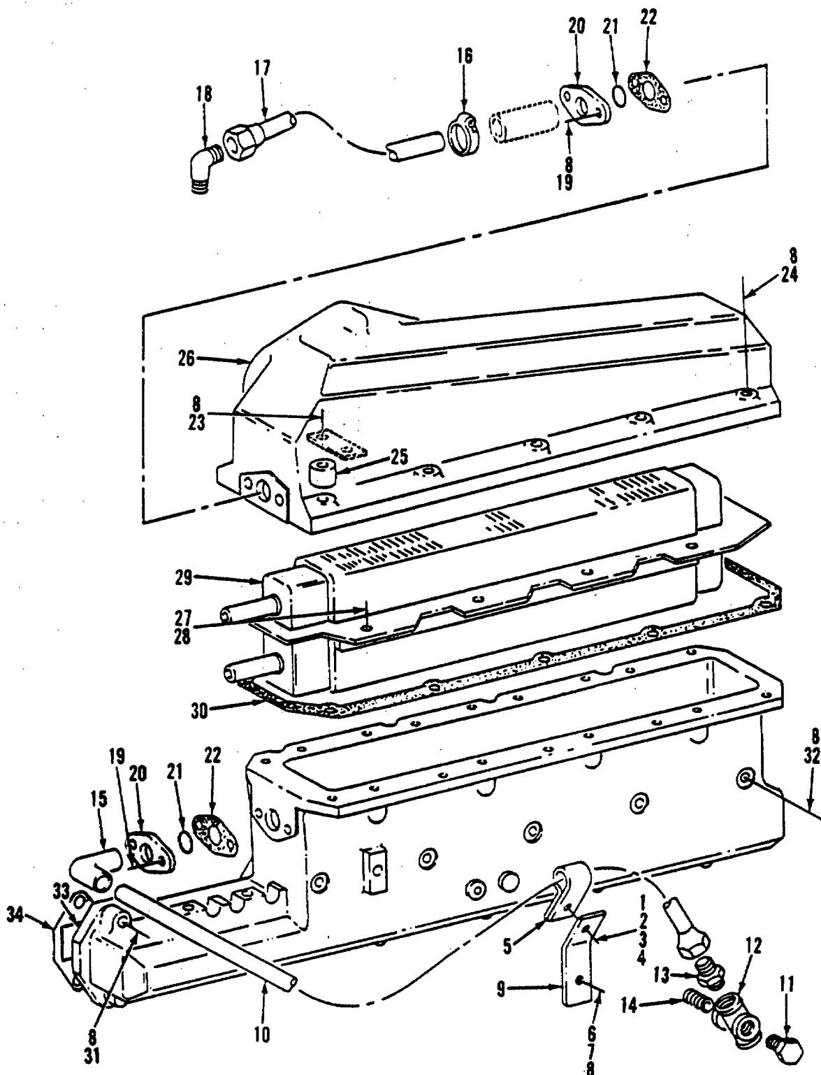
Figure 149. Intercooler Mounting and Piping
