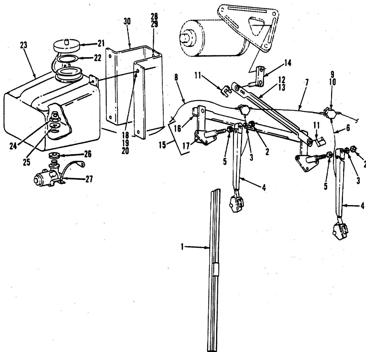
Figure 103. Windshield Wiper Installation
