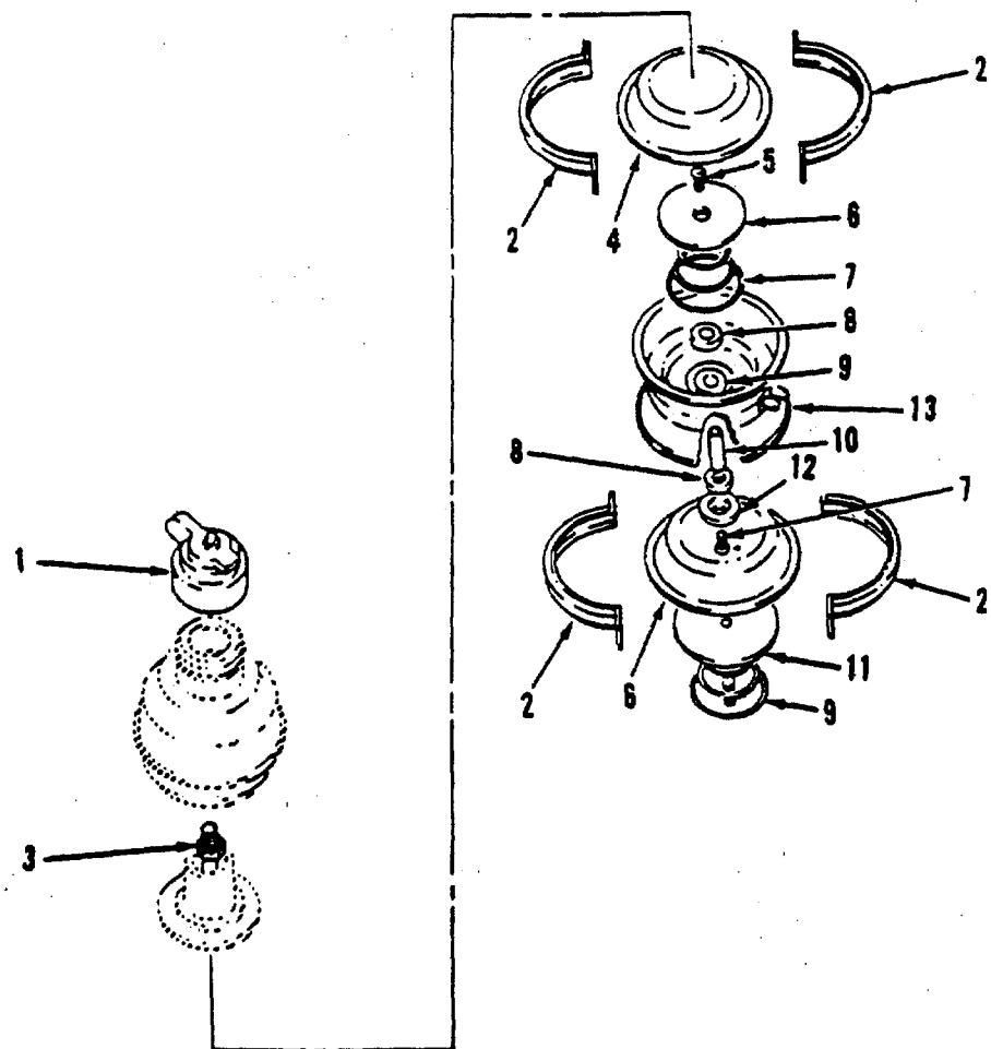
Figure 173. Air Brake Chamber - Forward Rear Axle
