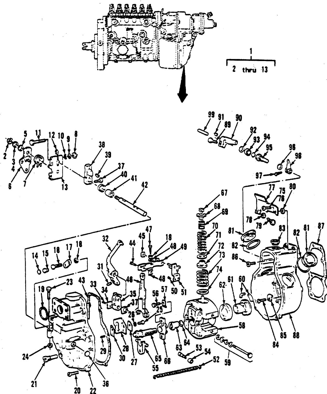
Figure 138. Fuel Injection Pump - Governor
