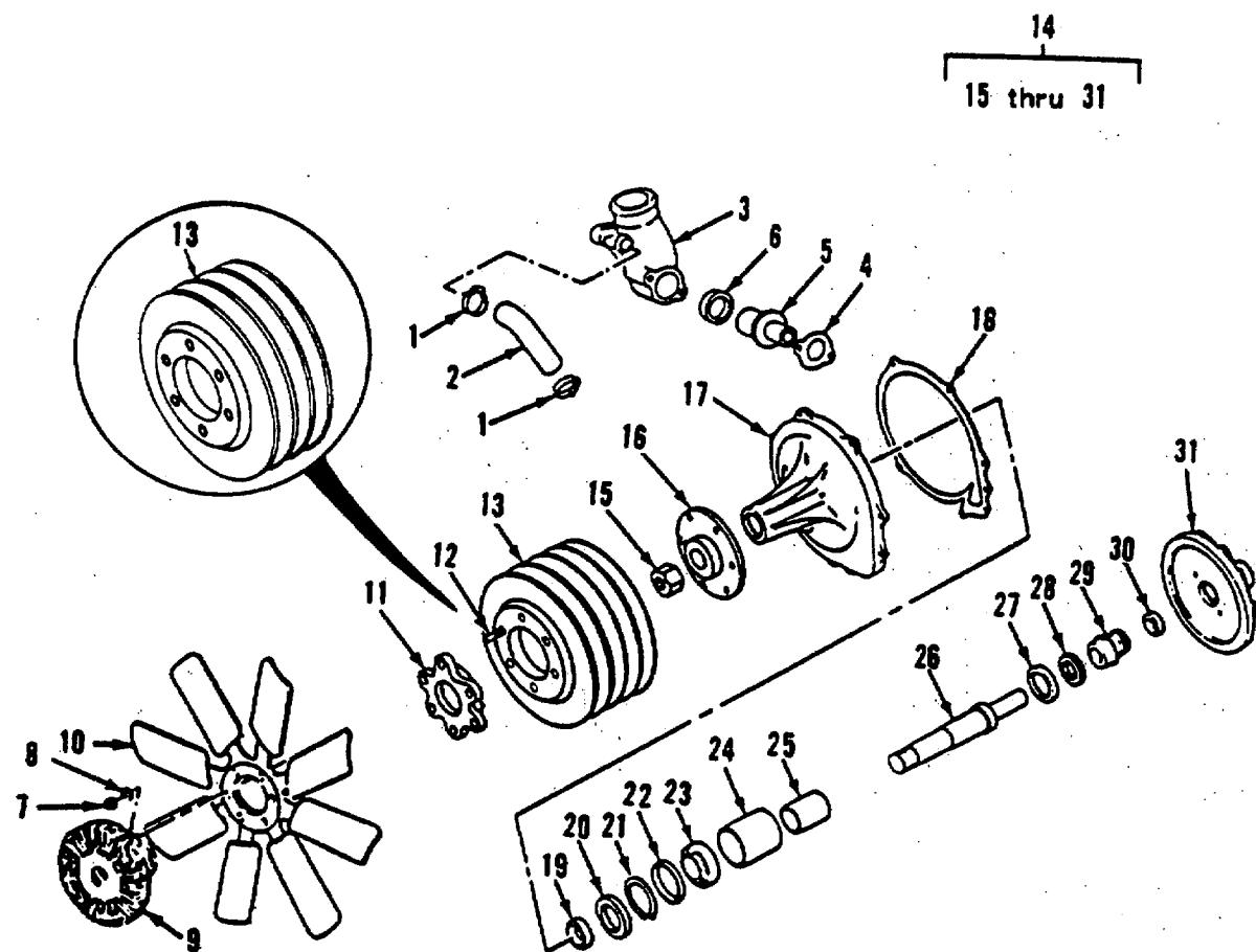
Figure 145. Water Pump and Fan Drive
