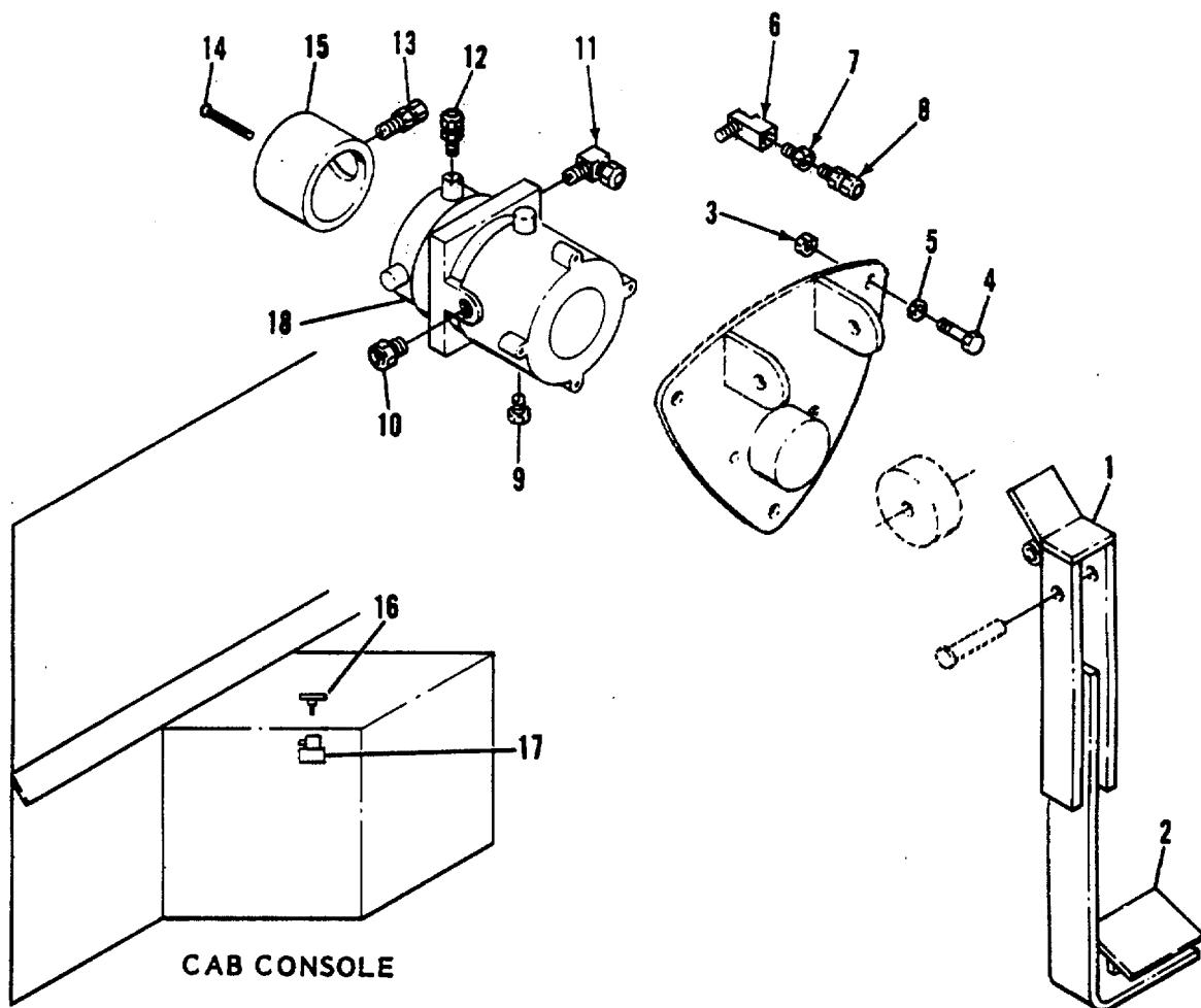
Figure 106. Brake Pedal Installation
