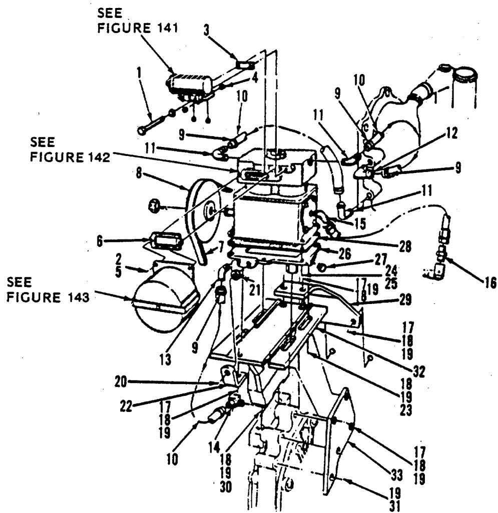
Figure 140. Air Compressor Mounting
