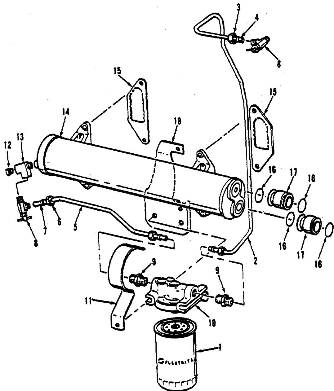
Figure 148. Oil Cooler and Coolant Filter
