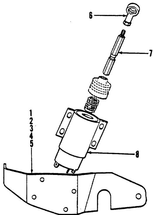
Figure 134. Fuel Pump Solenoid
