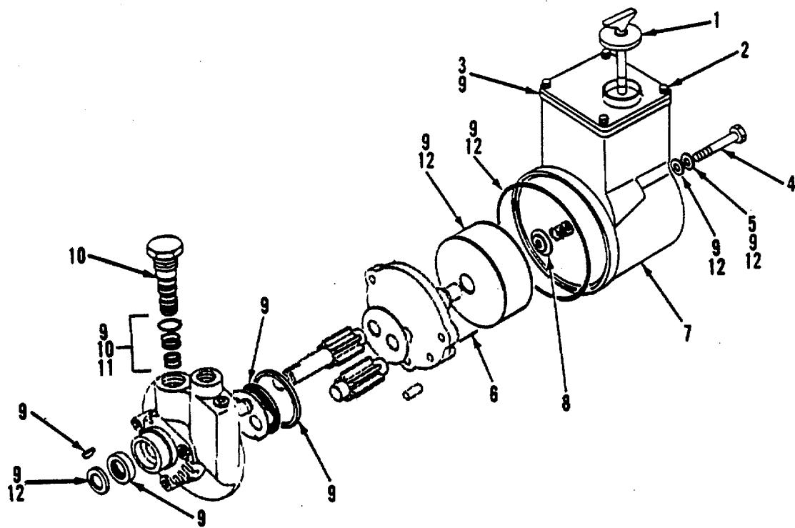
Figure 121. Steering Pump Assembly
