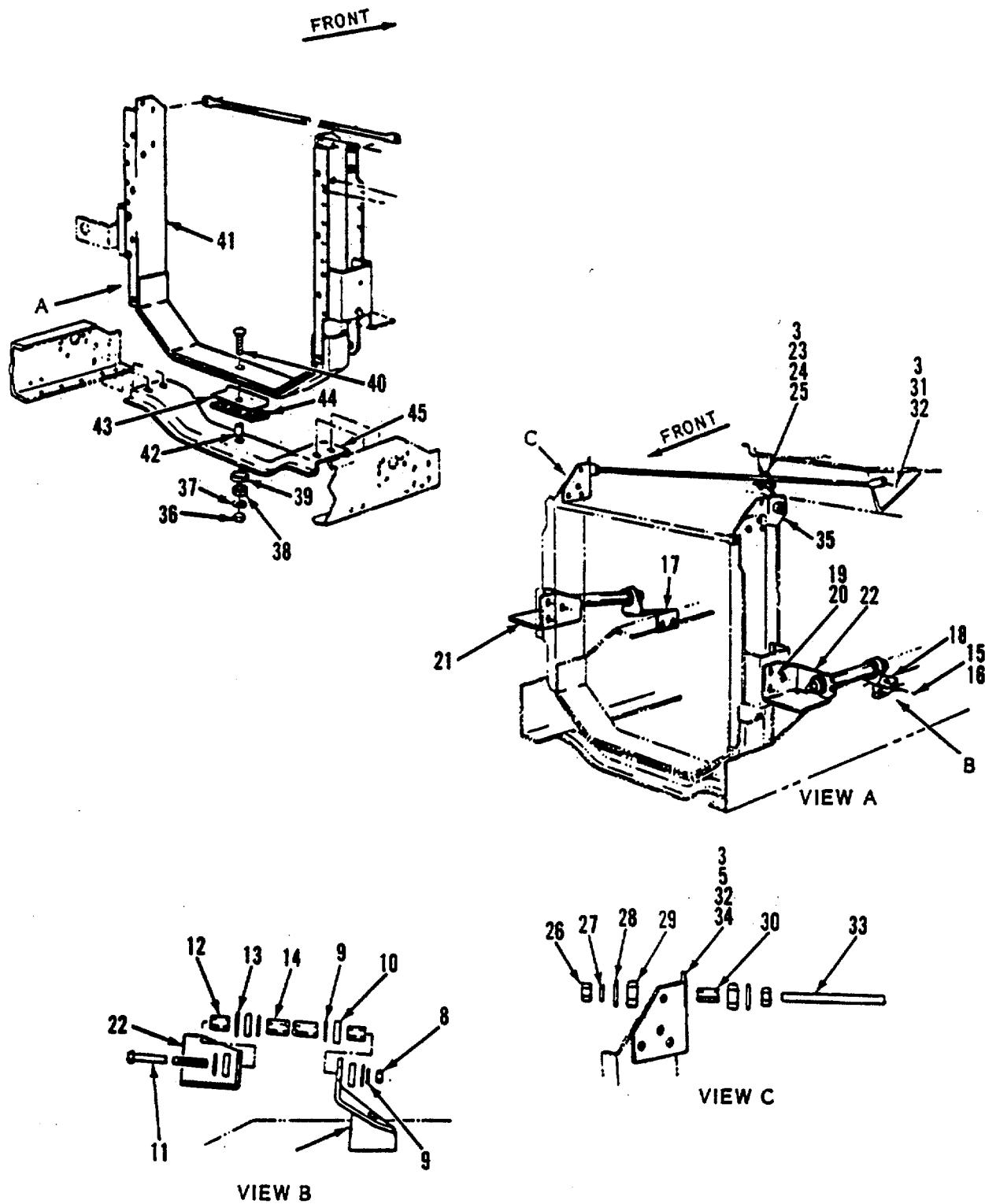
Figure 118. Radiator Installation (Sheet 2 of 2)
