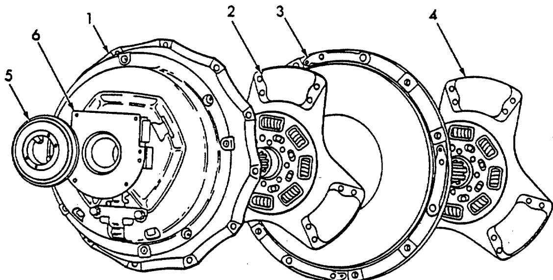
Figure 168. Clutch Assembly
