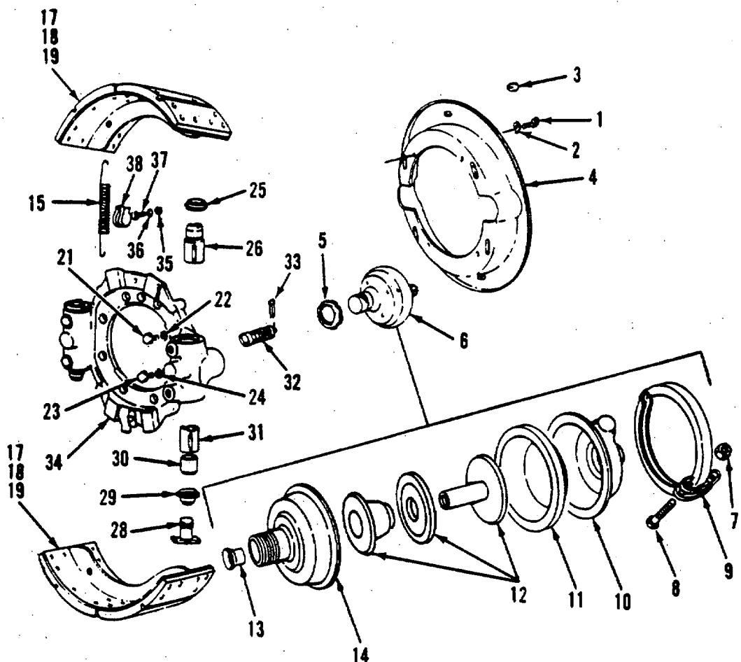
Figure 178. Left Front Brake Assembly
