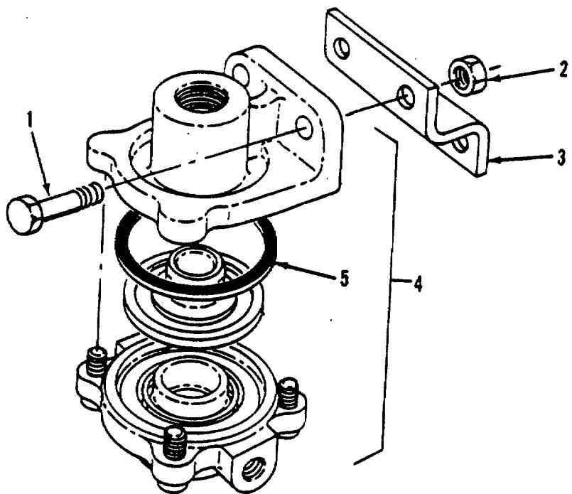
Figure 172. Quick Release Valve
