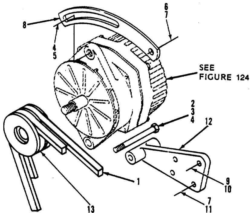
Figure 123. Alternator Mounting
