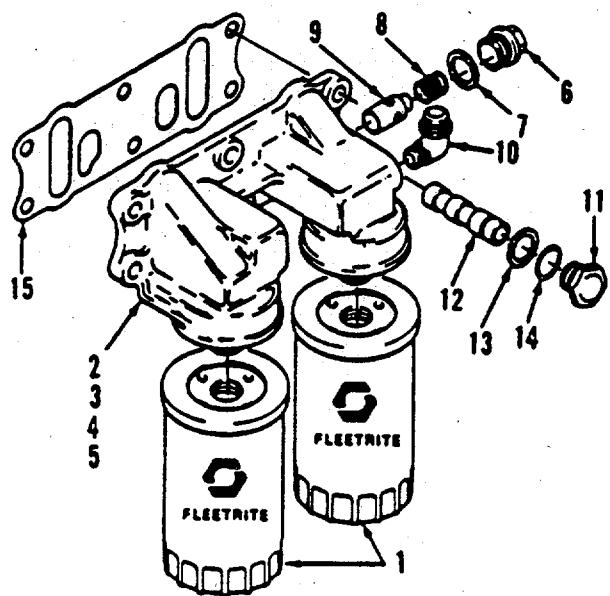
Figure 147. Oil Filter and Connection
