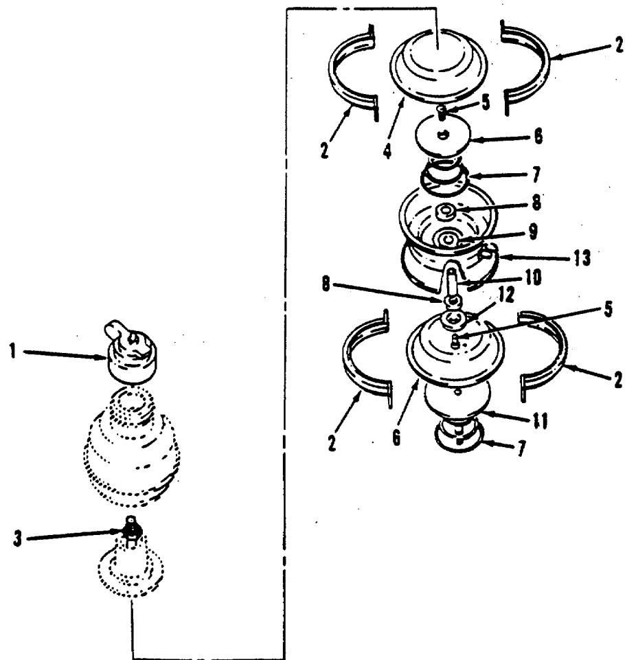
Figure 174. Air Brake Chamber - Rear Rear Axle
