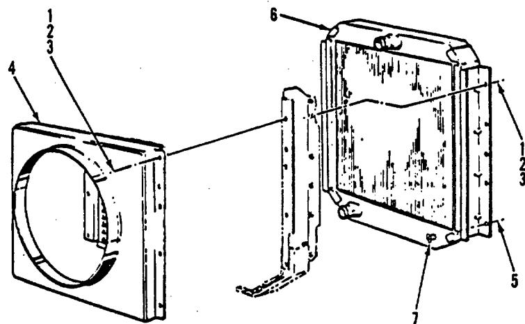
Figure 118. Radiator Installation (Sheet 1 of 2)
