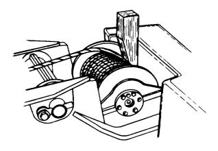
Figure 5-6 Wedge Block in Winch Drum
