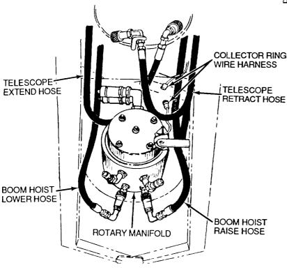
Figure 5-19 Rotary Manifold Hoses
