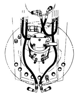
Figure 5-20 <u>Location of Boom Hoist Cylinder Hoses</u> <u>After Disconnection</u>
