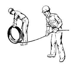
Figure 4-26. Correct Method of Uncoiling Wire Rope
