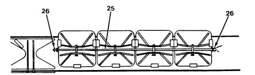
Figure 5-33 Secure Pads on Boom
