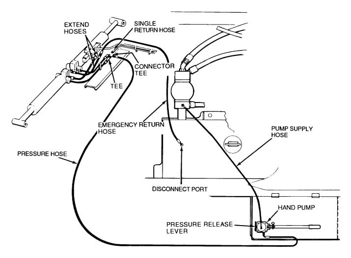
Figure 4-56. Lowering the LRT Crane off the Outriggers
