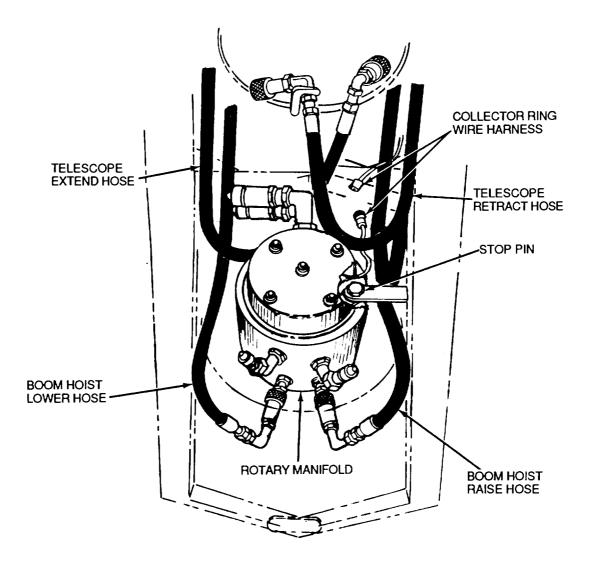
Figure 5-40 Rotary Manifold Hoses
