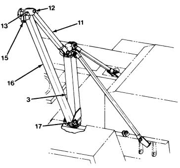
Figure 5-12. Assembling the Mast
