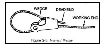
3. Seat wedge and loop just tightly enough to allow handling by attaching socket to a strong support and engaging winch to take a strain on cable.
