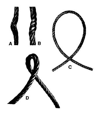
Figure 4-22. Wire Rope Kinking
