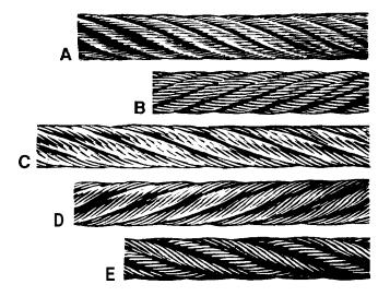
Figure 4-17. a.Right Regular Lay b. Left Regular Lay c. Right Lang Lay d. Left Lang Lay e. Right Alternate Lay.
