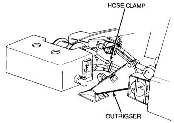
Figure 5-34 Positioning Outrigger
