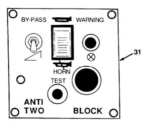
Figure 4-12. Anti-two Block Panel
