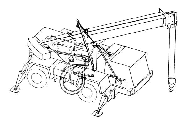
Figure 5-21 Positioning of Mast and Lifting Arm.
