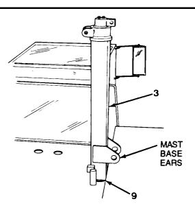
Figure 5-10. Assembling the Mast
