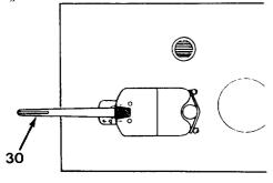
Figure 4-11. Turn Signal Lever
