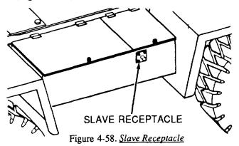
If slave starting, make sure when connecting slave start cables that ignition switch is OFF, transmission is in neutral and parking brake is applied.
