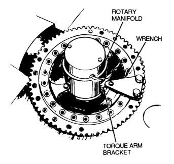
Figure 5-32 Rear Axle Oscillation
