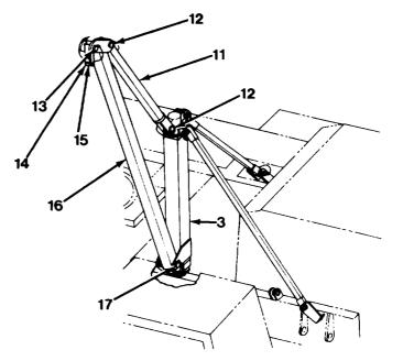
Figure 5-31 Assembling the Mast
