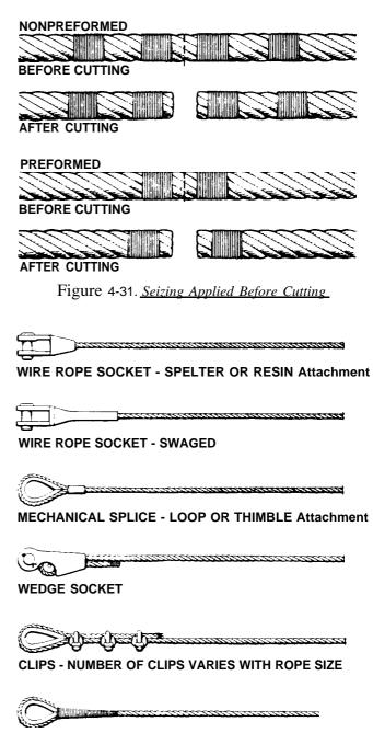
Figure 4-32. End Fittings and Attachments
