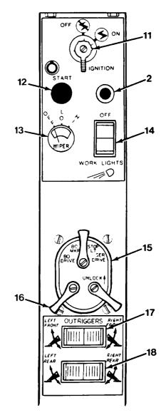
Figure 4-3. Slide Sloping Dash Panel
