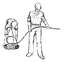
Figure 4-27. Incorrect Method of Unreeling Wire Rope
