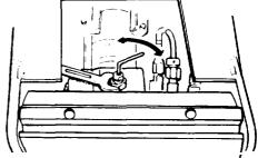
Figure 4-54. Holding Valve (Adjusting Screw)
