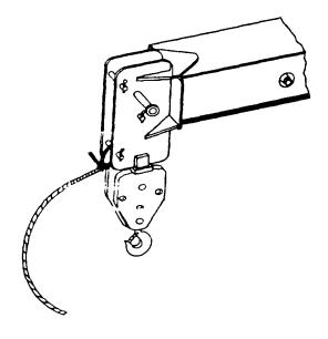
Figure 5-24 Attached Tether Rope
