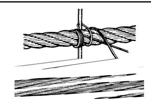
Figure 4-29. Seizing Wire Rope - Method A
