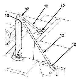
Figure 5-11A. Installing the Truss Rods
