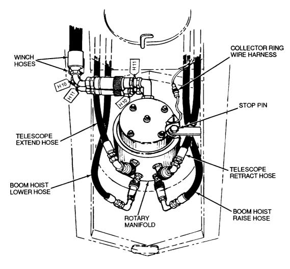
Figure 5-13. Rotary Manifold Hoses
