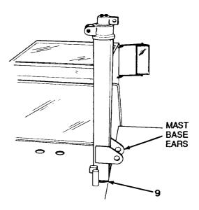
Figure 5-10. Assembling the Mast
