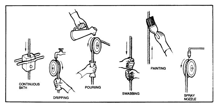
Figure B-1. Methods of Applying Lubrication
