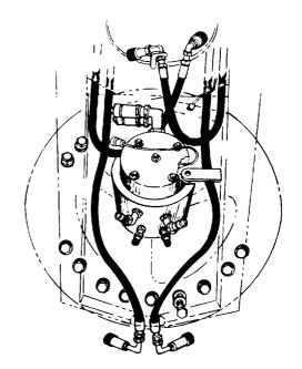
Figure 5-20 Location of Boom Hoist Cylinder Hoses After Disconnection
