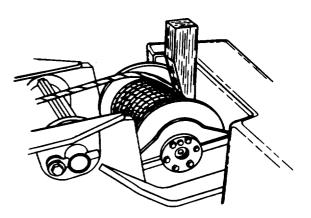
Figure 5-6. Wedge Block in Winch Drum
