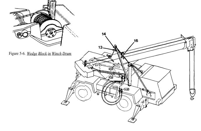
Figure 5-39 Lifting the Upperstructure
