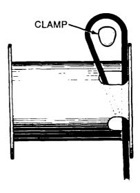
Figure 2-6. Securing Cable on Winch
