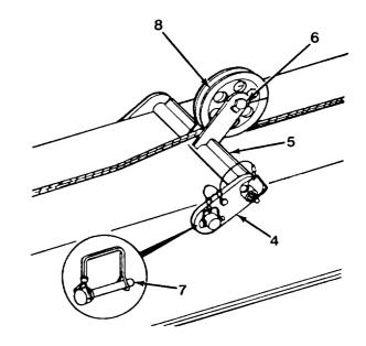
Figure 5-8. Installing Sheaves
