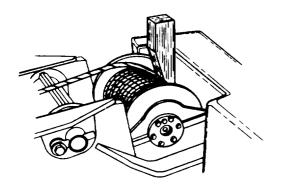
Figure 5-6. Wedge Block in Winch Drum
