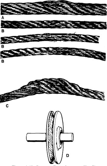
Figure 4-49. Damage From Incorrect Handling
