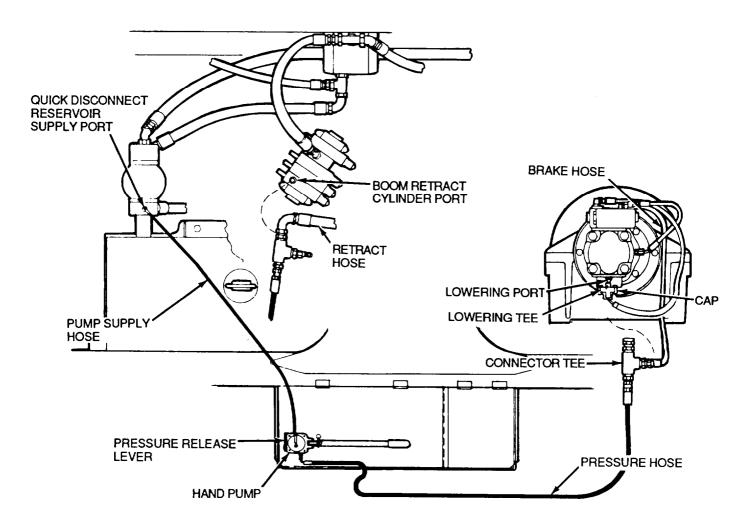
Figure 4-53. Quick Disconnect on Supply Hose
