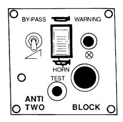
Figure 5-9. Anti-Two Block Panel
