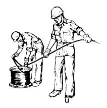
Figure 4-28. Incorrect Method of Uncoiling Wire Rope
