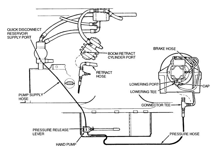
Figure 4-53. Quick Disconnect on Supply Hose
