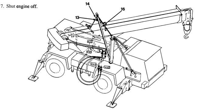
Figure 5-22 Lifting the Upperstructure
