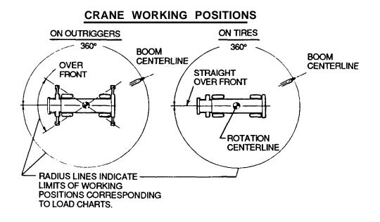
Figure 1-7. Working Area Diagram
