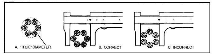
Figure 4-21. How to Measure (or caliper) a Wire Rope
