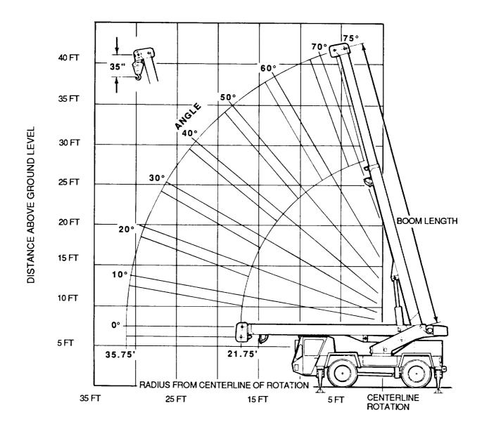
Figure 1-6. Radius from Centerline of Rotation
