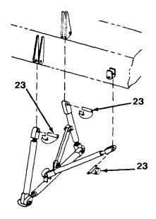
Figure 5-37 Boom Support Removal
