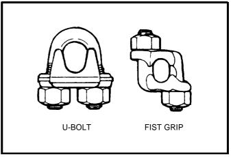
Figure 4-34. Basic Designs of Wire Rope Clips
