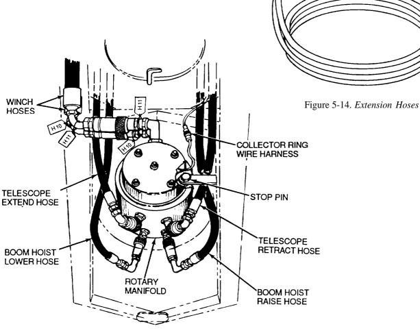
Figure 5-13. Rotary Manifold Hoses
