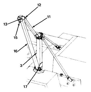
Figure 5-12. Assembling the Mast
