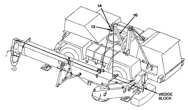
Figure 5-36 Preparing Upperstructure for Lift
