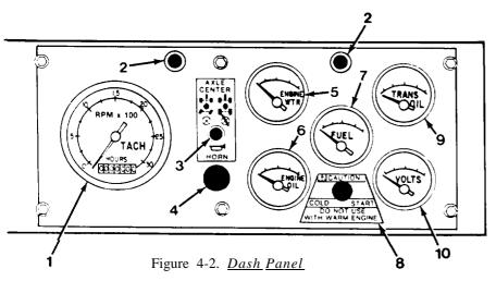
1. **Tachometer/Hour Meter** indicates engine rpm (normal idle 800 rpm; governed 2,950 rpm) and operating hours of engine (Figure 4-2).
