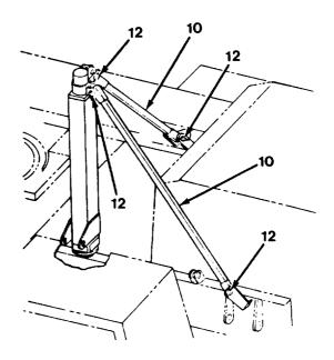
Figure 5-11A. Installing the Truss Rods
