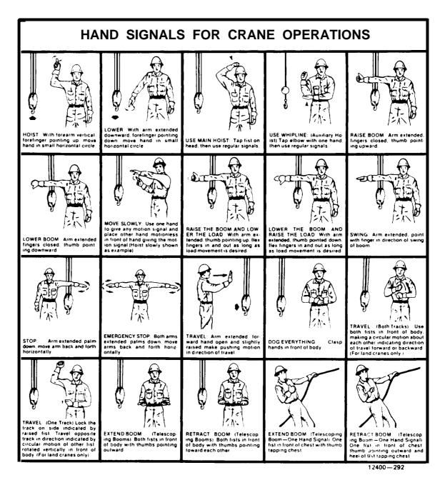
Figure 4-16. Hand Signals for Crane Operation
