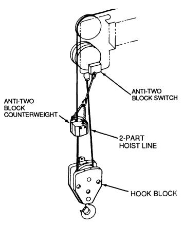
Figure 5-2. <u>Anti-Two Block Counterweight. Switch and</u> <u>Hook Block</u>
