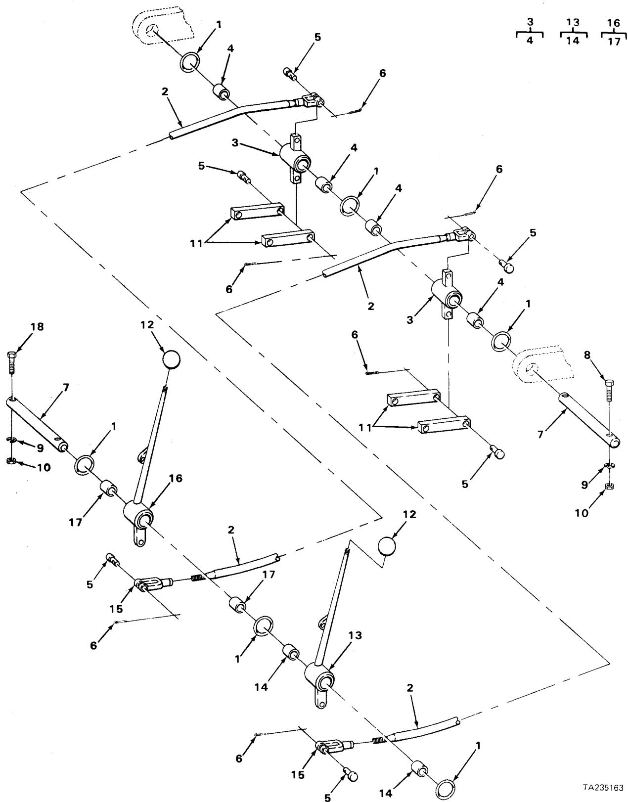
FIGURE 59. VALVE CONTROL LINKAGE (2 SPOOL)
