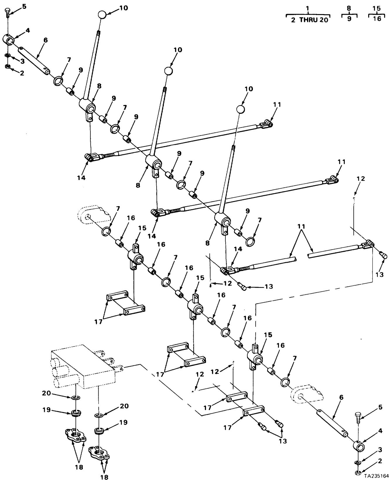
FIGURE 60. VALVE CONTROL LINKAGE (3 SPOOL)
