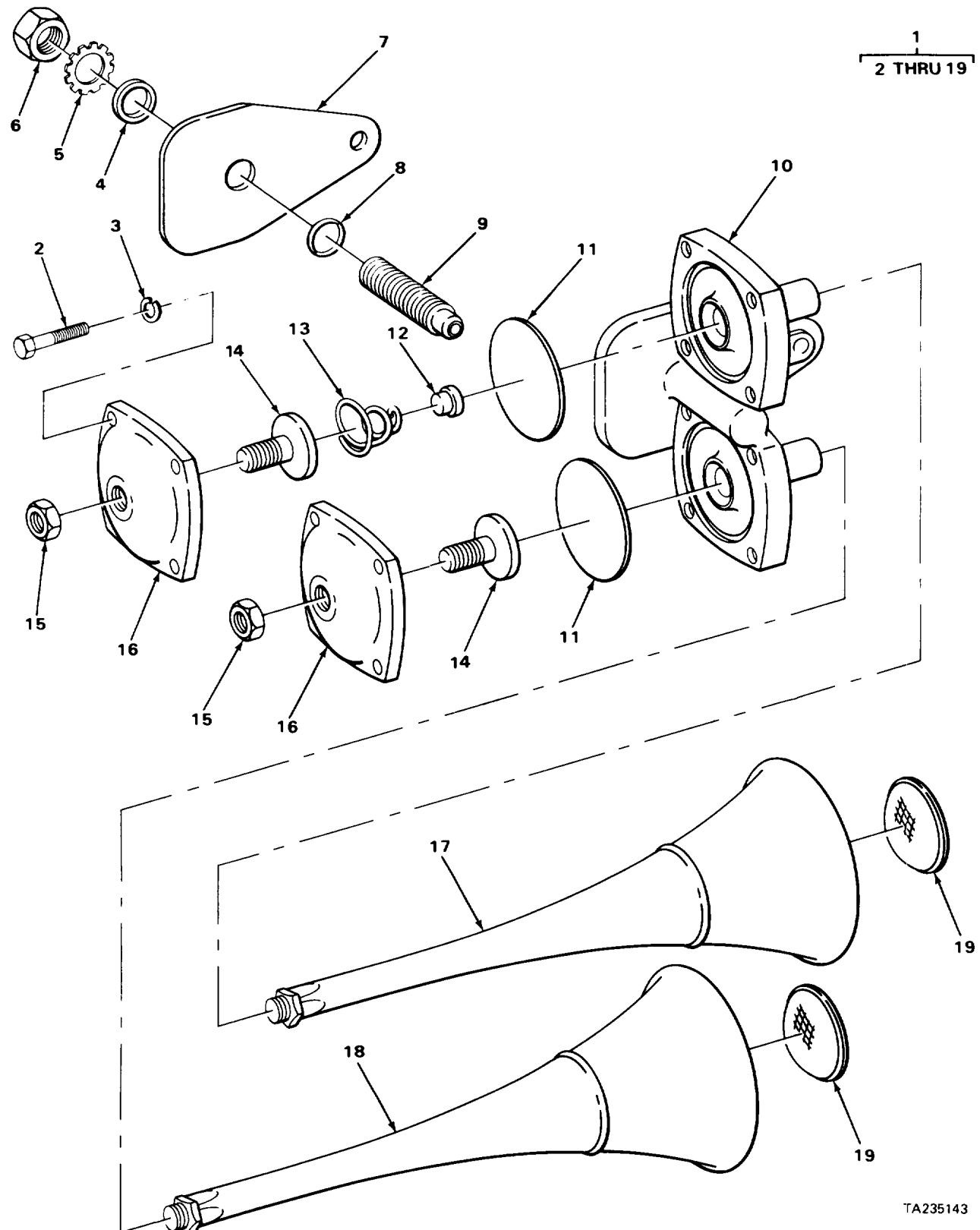
FIGURE 51. AIR HORN ASSEMBLY
