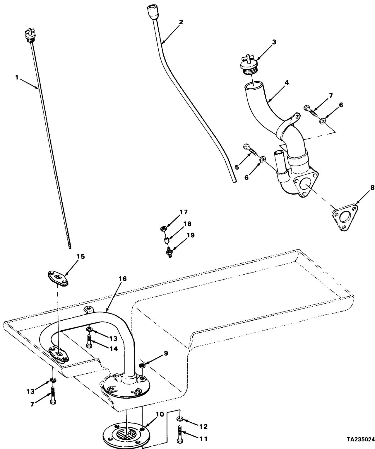
FIGURE 2A. OIL GAGE, FILLER PIPE, LUBRICATING SUCTION PIPING AND RELATED PARTS.
