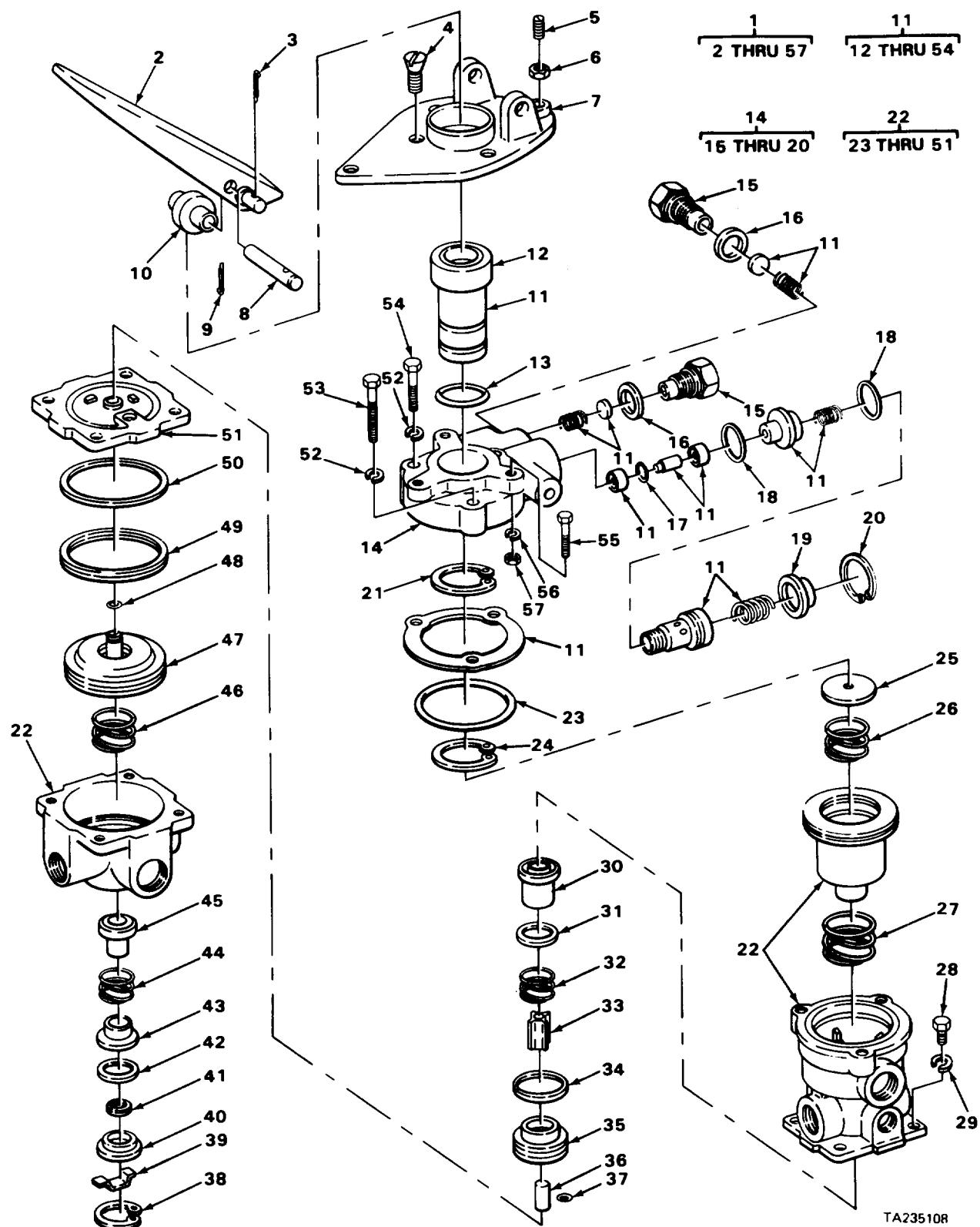
FIGURE 37. TREADLE VALVE LEFT HAND
