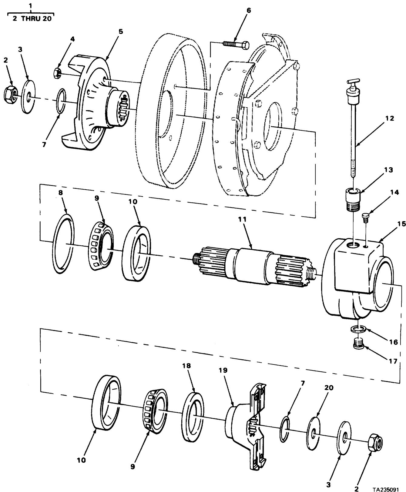
FIGURE 32. TRANSFER DRIVE ASSEMBLY
