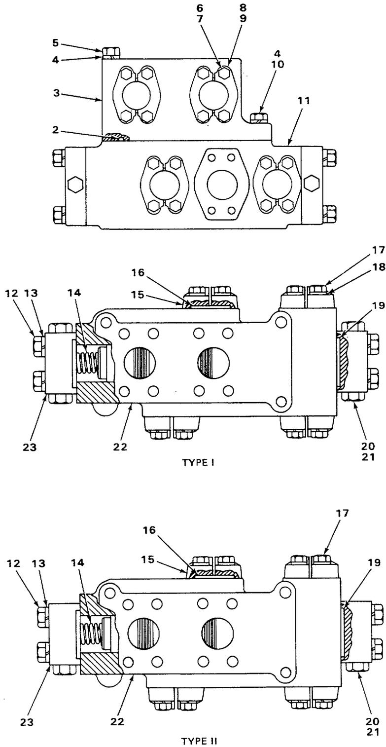
FIGURE 91. SELECTOR VALVE (TYPES 1 AND 2).
