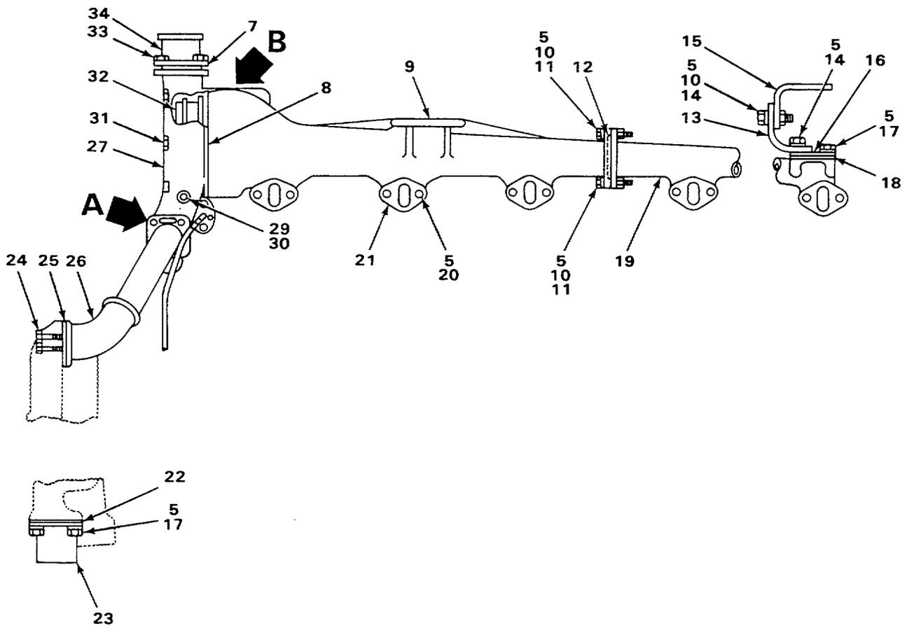
FIGURE 23. WATER MANIFOLD.
