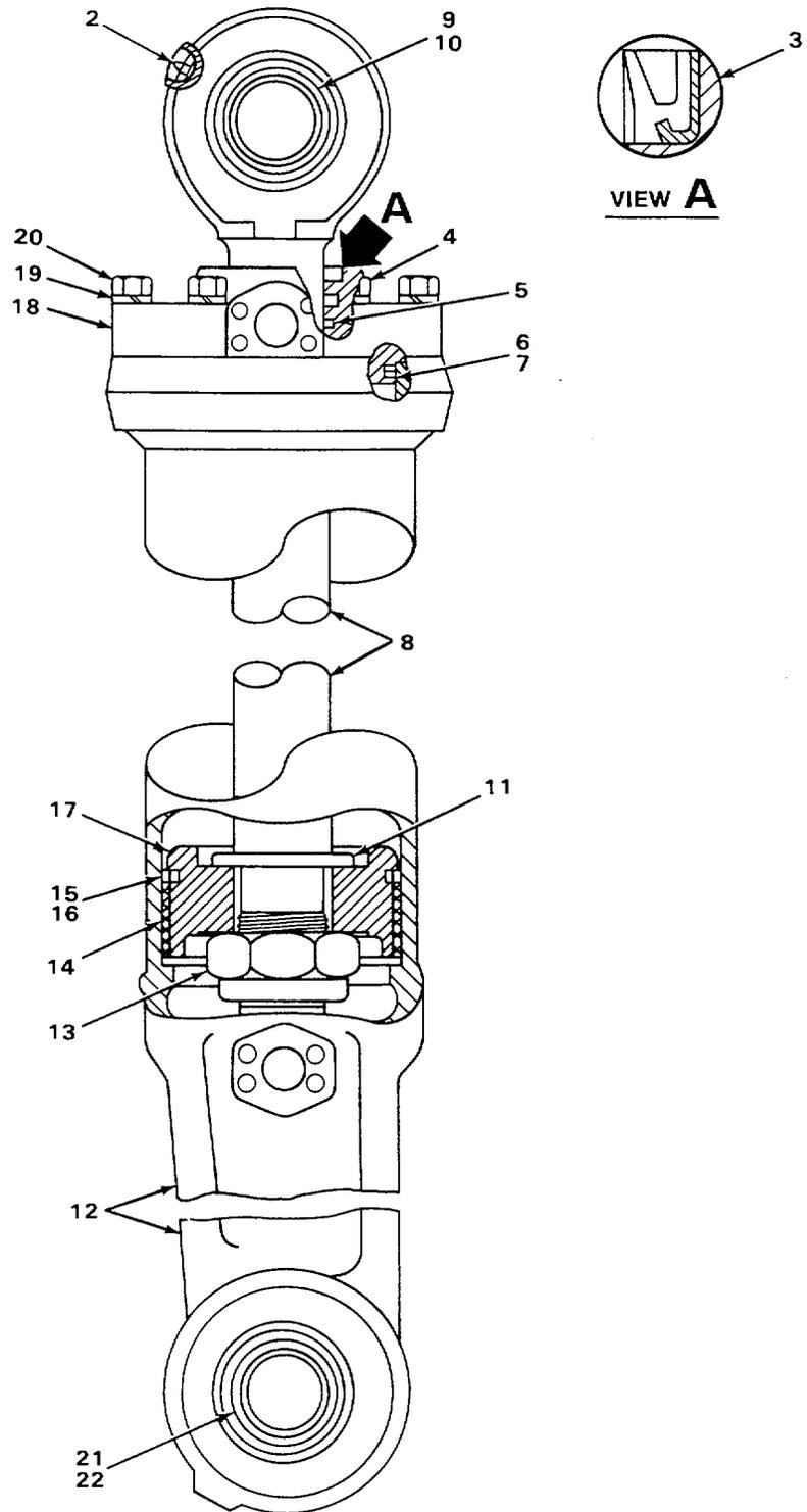
FIGURE 108. RIPPER CYLINDER, CENTER.
