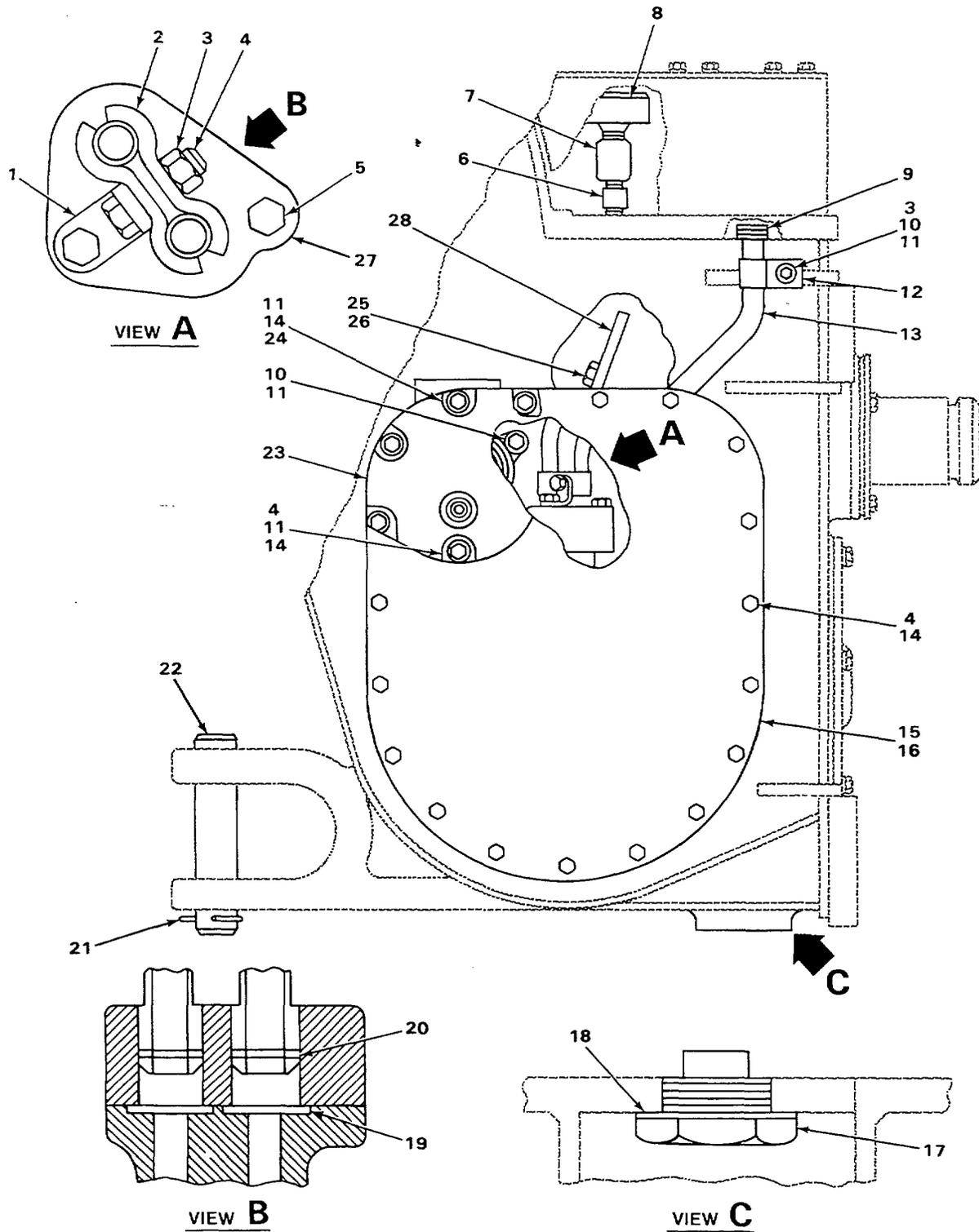
FIGURE 80. WINCH FILTER RELATED PARTS.
