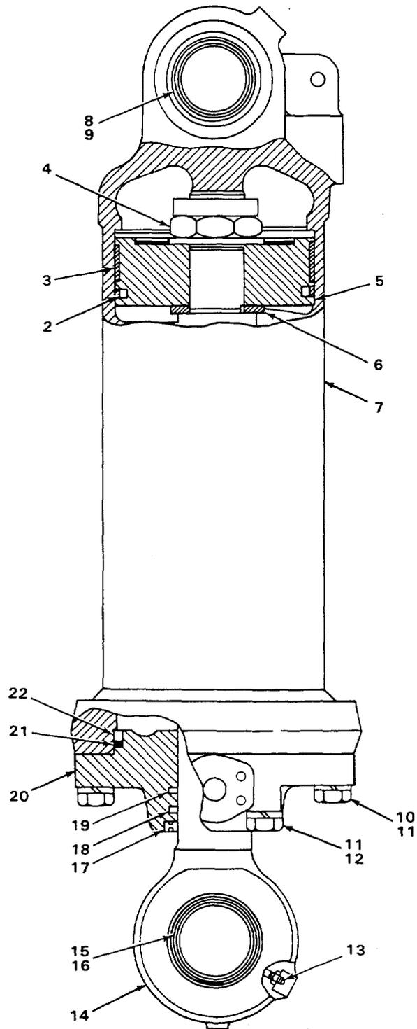
FIGURE 107. RIPPER CYLINDER, LEFT AND RIGHT.
