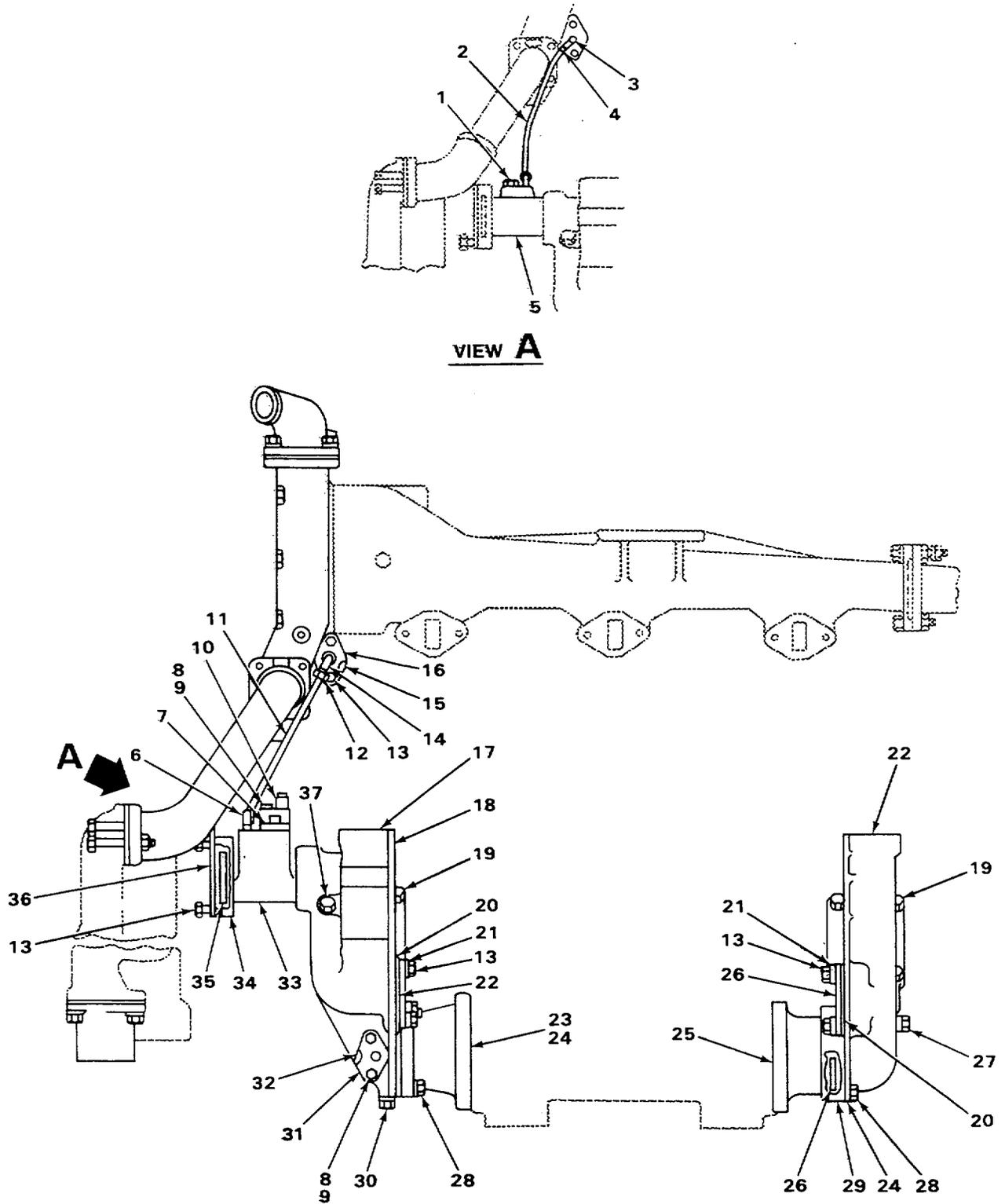
FIGURE 24. WATER MANIFOLD LINES AND RELATED PARTS.
