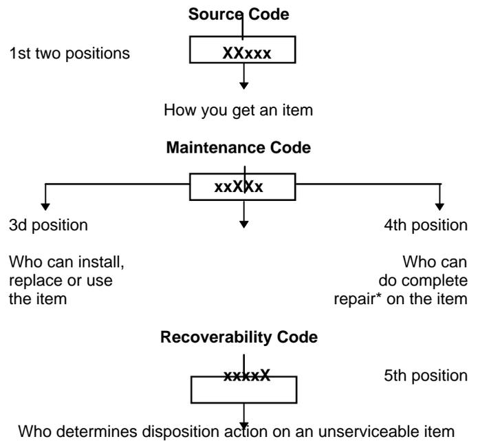
\*Complete Repair: Maintenance capacity, capability, and authority to perform all corrective maintenance tasks of the "Repair" function in a use/user environment in order to restore serviceability to a failed item.
