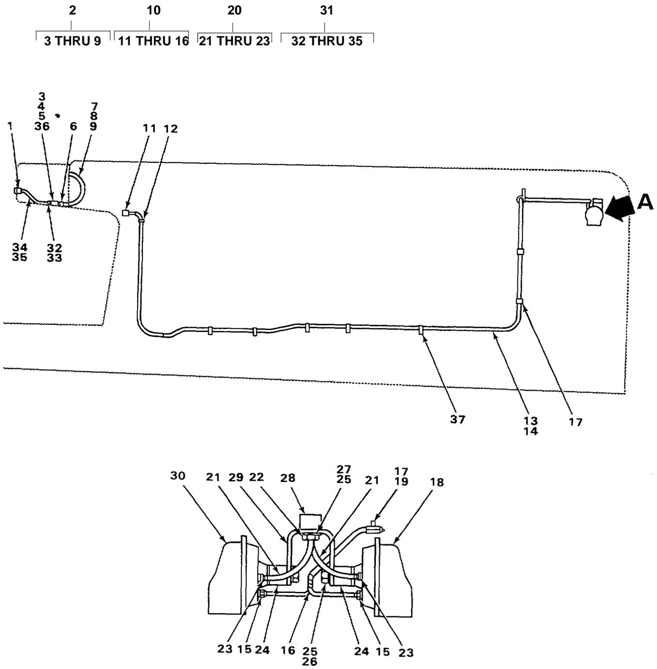
FIGURE 43. CENTER MOUNTED ELECTRIC HORN.
