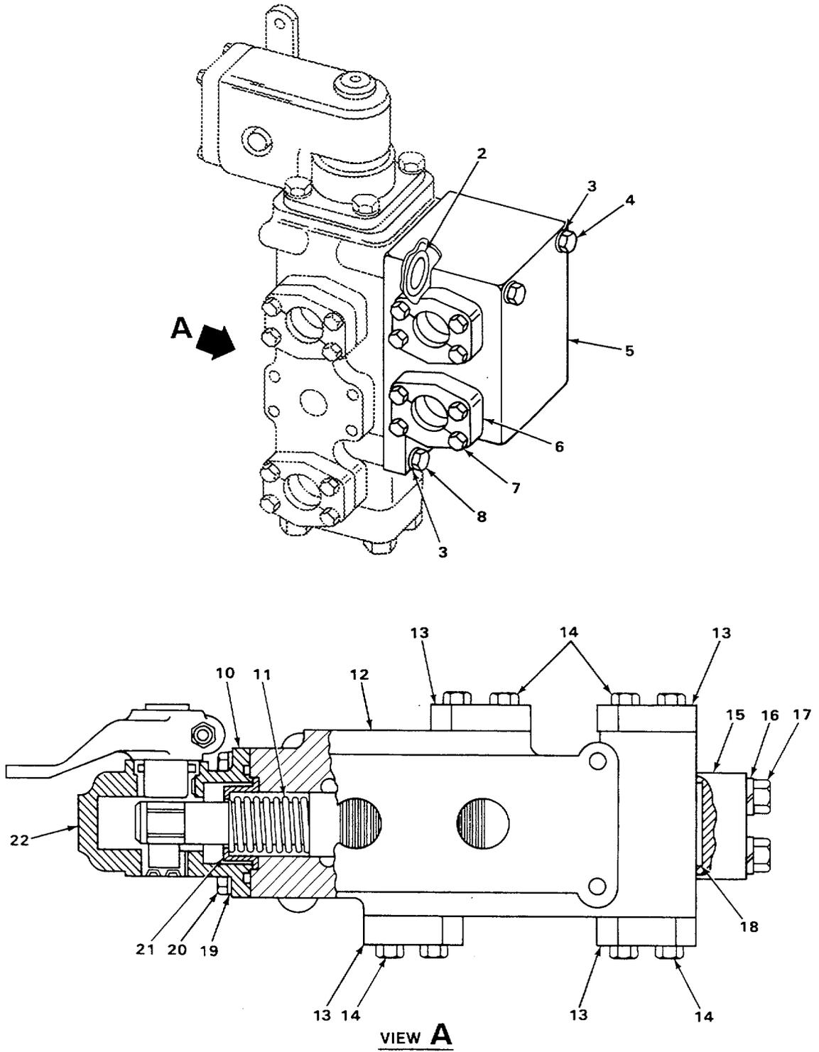
FIGURE 88. RIPPER SELECTOR VALVE.
