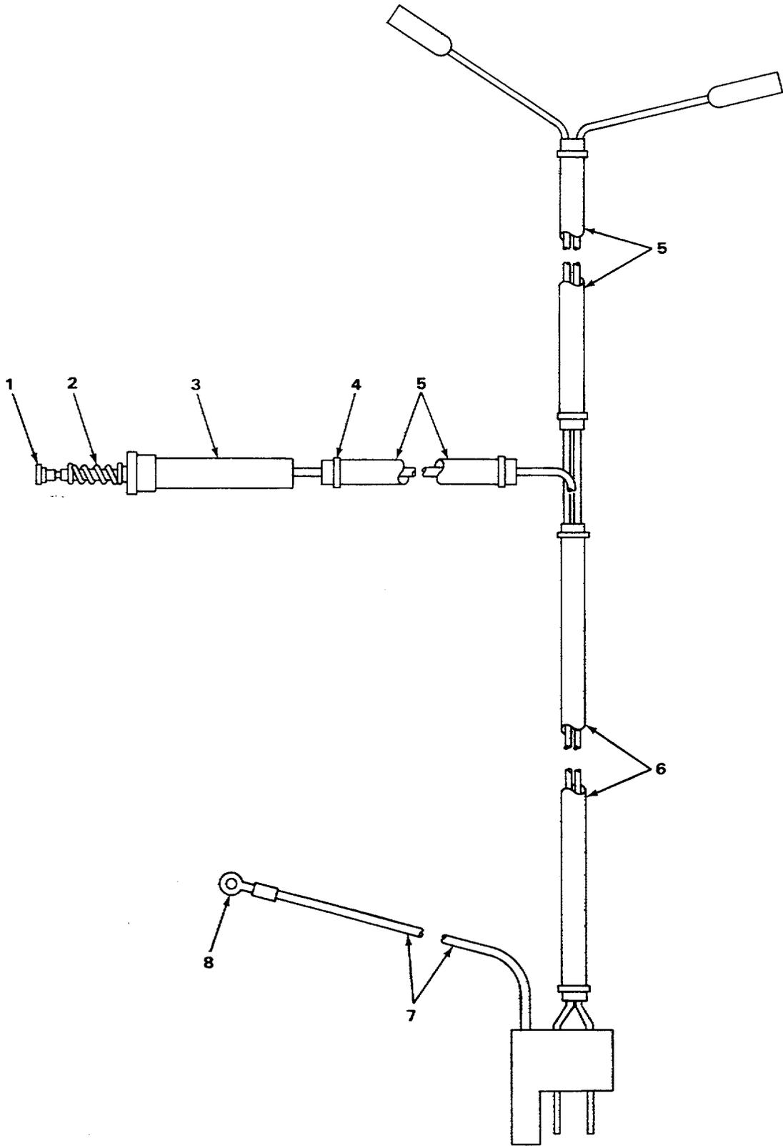
FIGURE 35. BACKUP WARNING ALARM HARNESS.
