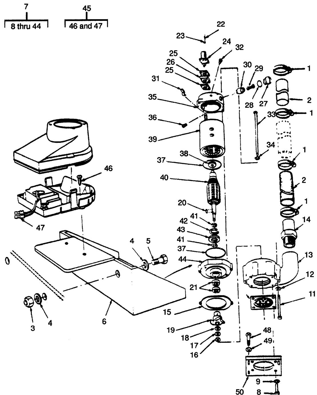
Figure 75. Electric Bilge Pump Assembly and Bilge Level Warning Switch.
