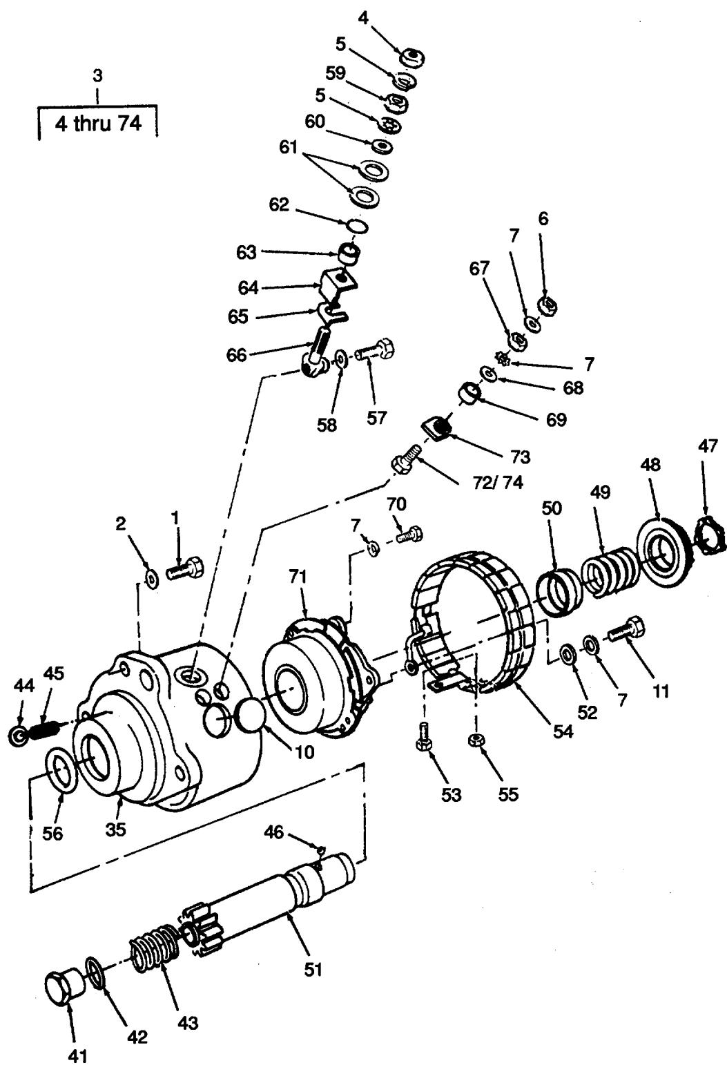
Figure 55. Starter Motor ( Sheet 1 of 2 ).
