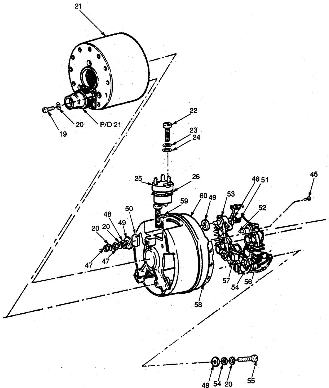
Figure 44. AC5 Alternator and Support Bracket (Sheet 2 of 3).
