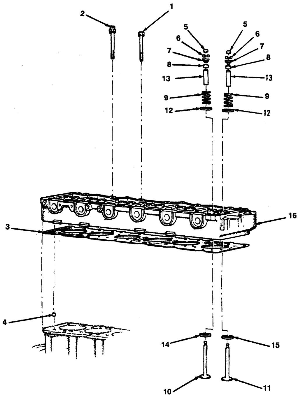
Figure 61. Cylinder Head Assembly.
