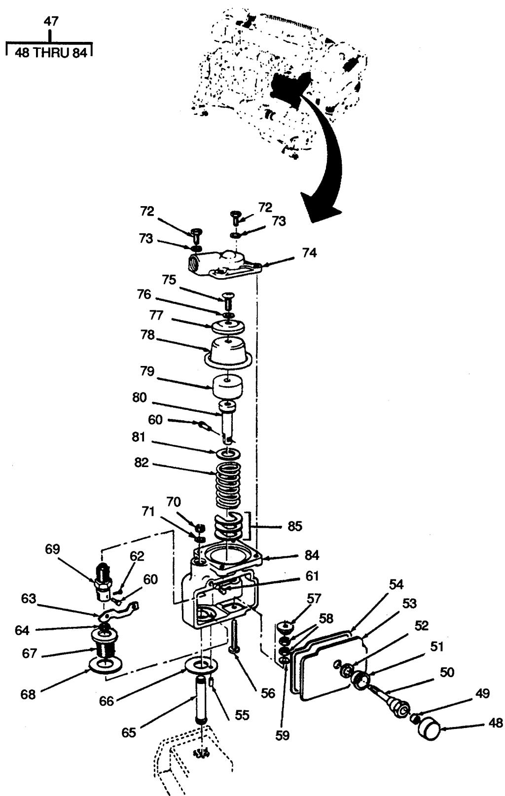
Figure 58. Injector Pump Assembly (Sheet 2 of 6).
