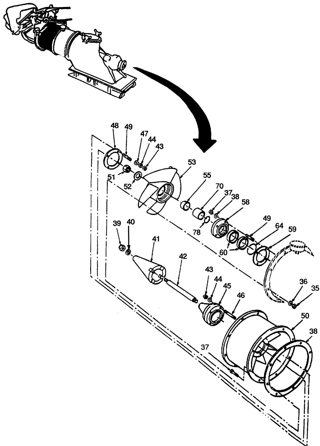
Figure 71. Hydro jet Assembly (Sheet 3 of 5)
