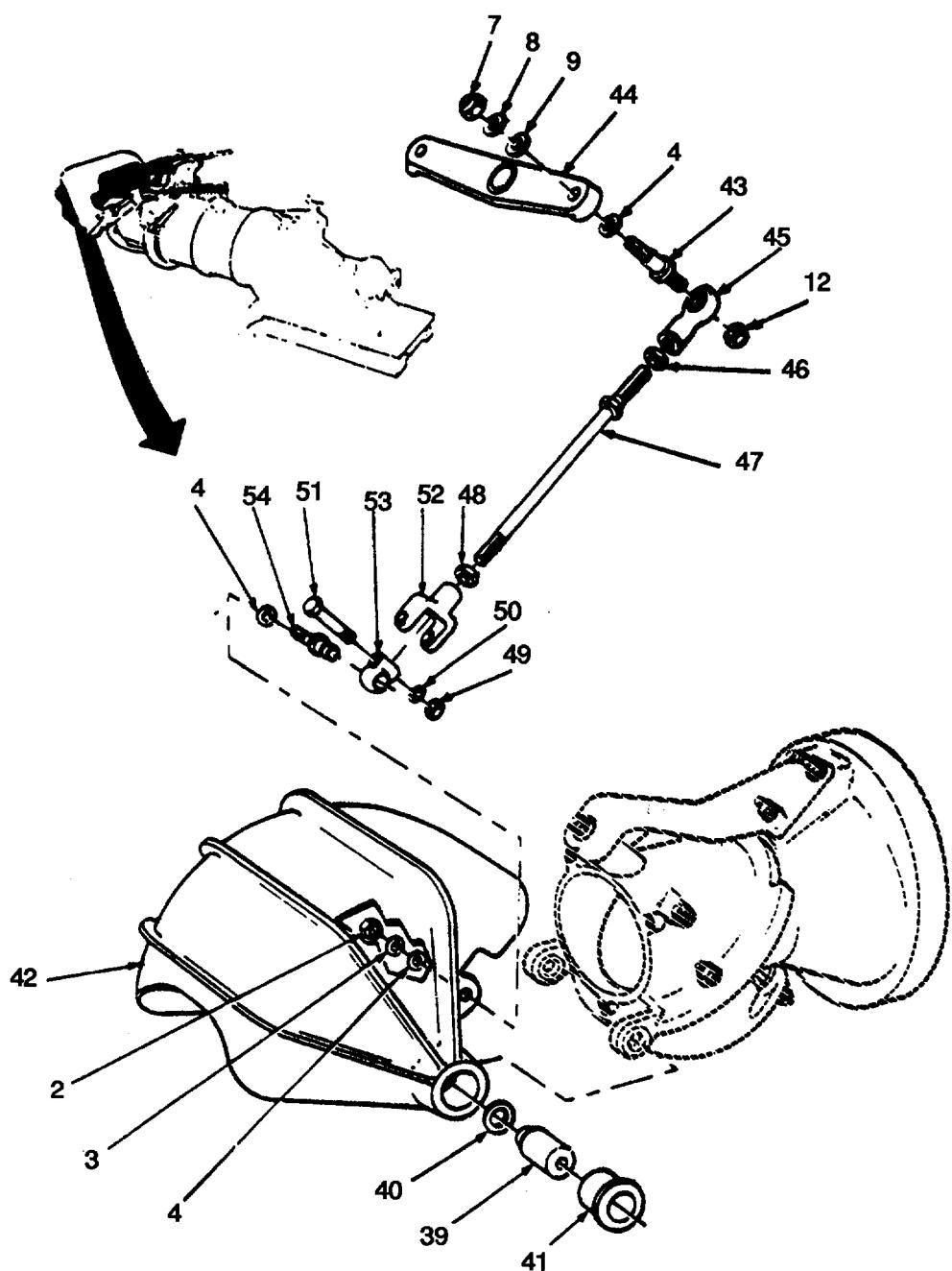
Figure 72. Hydro Jet Unit, steering Assembly (Sheet 3 of 6).
