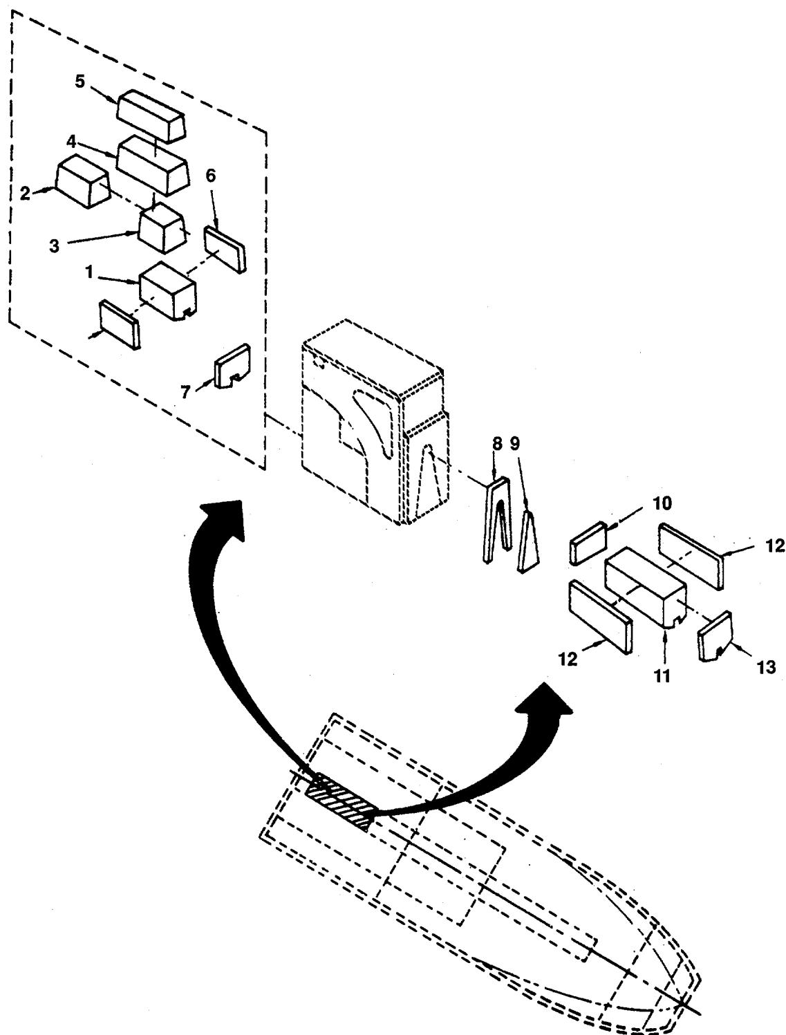
Figure 82. Buoyancy Blocks MK-2 (Sheet 1 of 7).
