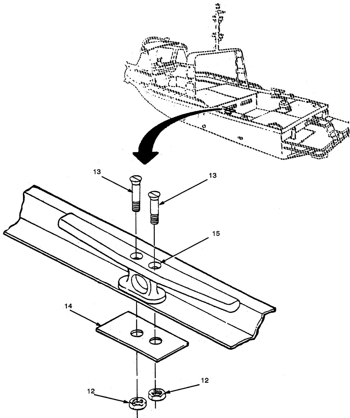
Figure 84. Diving Platform , Hinged Flap. (Sheet 2 of 2)
