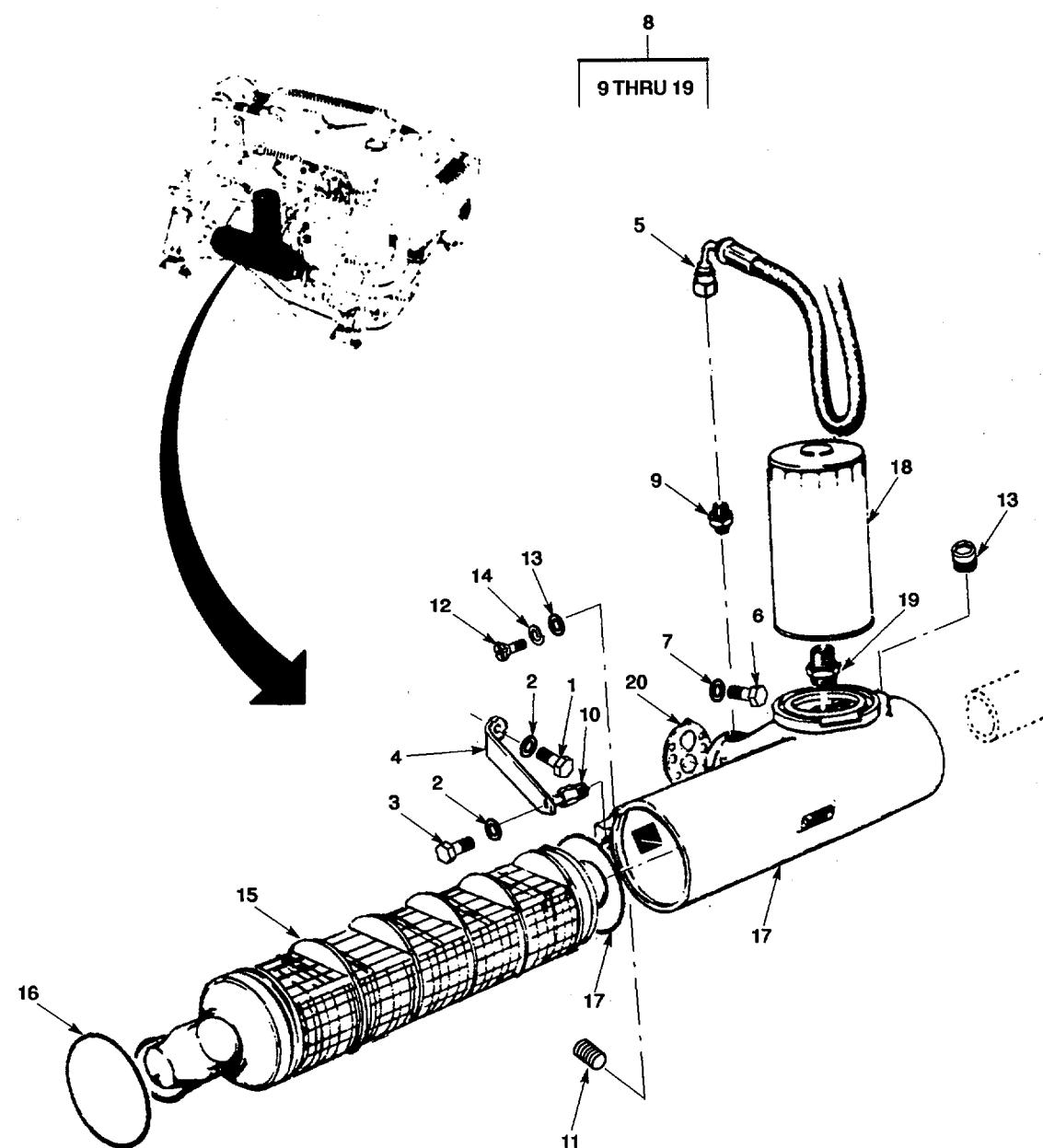
Figure 37. Oil Cooler and Oil Filter.
