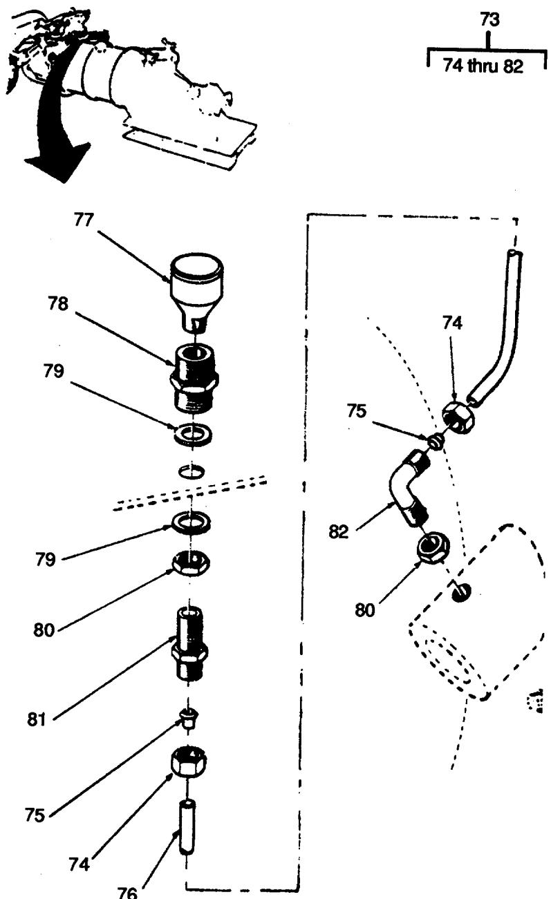
Figure 72. Hydro Jet Unit, Steering Assembly (Sheet 6 of 6).
