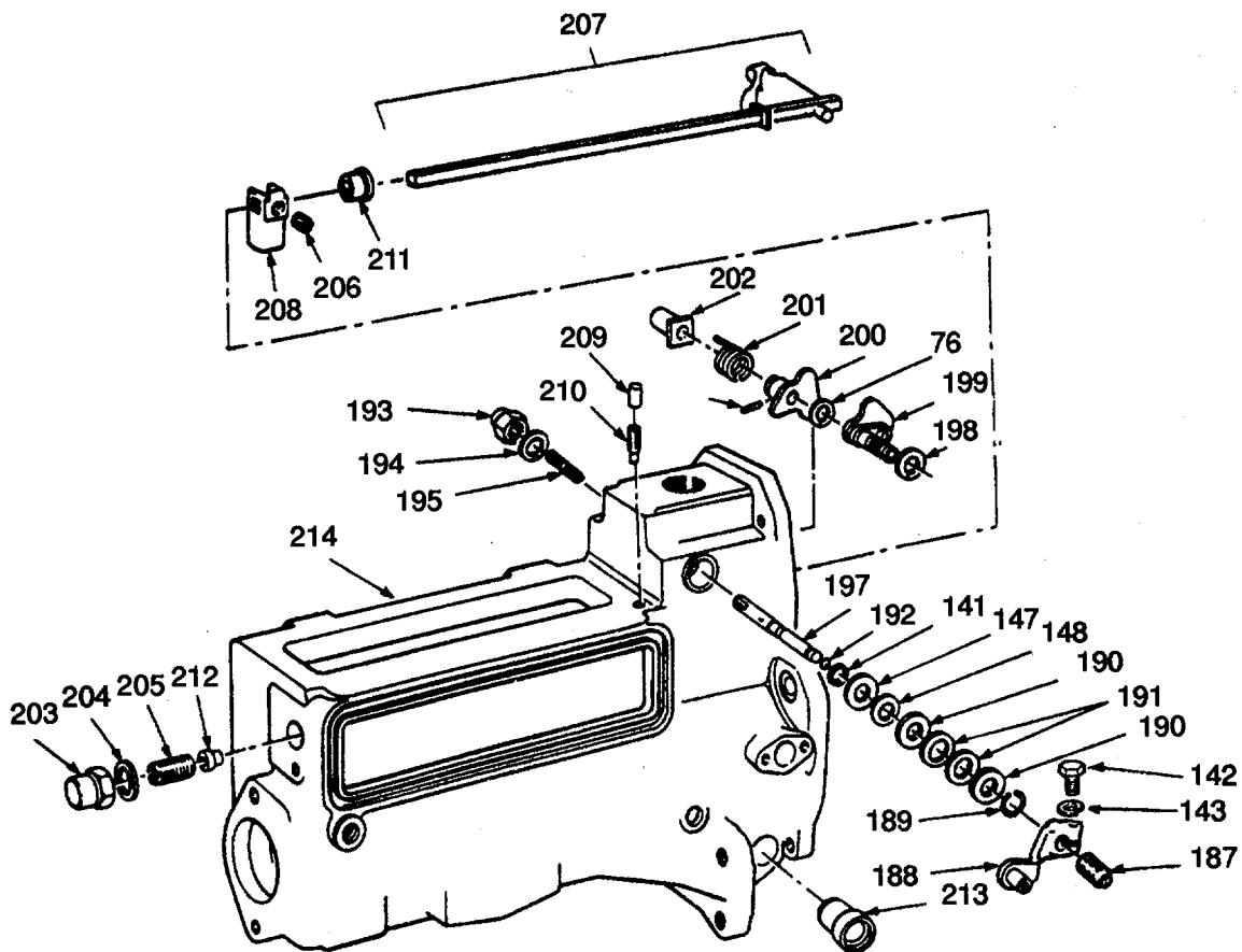
Figure 58. Injector Pump Assembly (Sheet 6 of 6).
