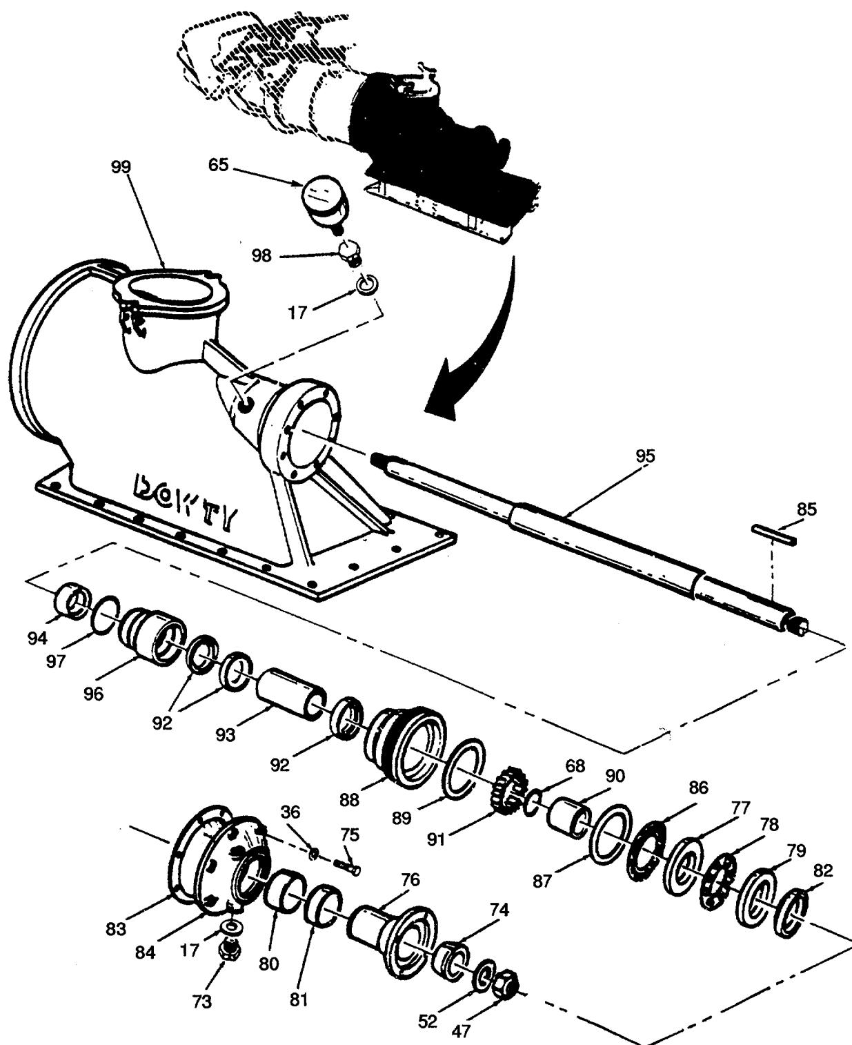
Figure 71. Hydro - Jet Assembly (Sheet 5 of 5).
