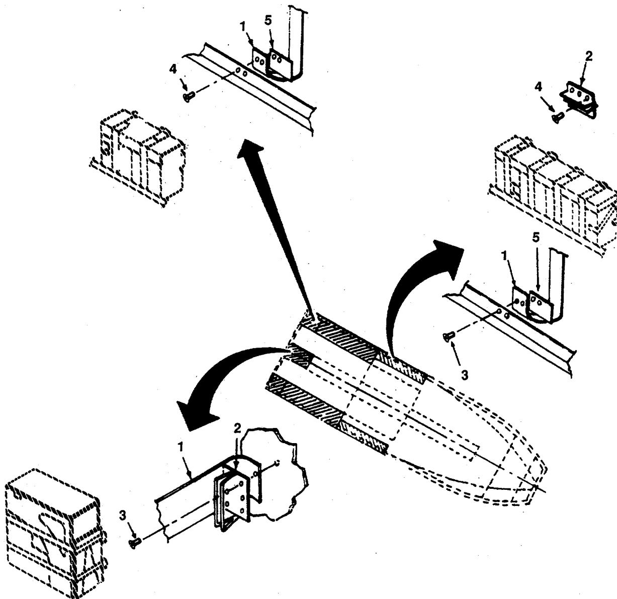
Figure 81. Anchoring Buoyancy Blocks MK-2.
