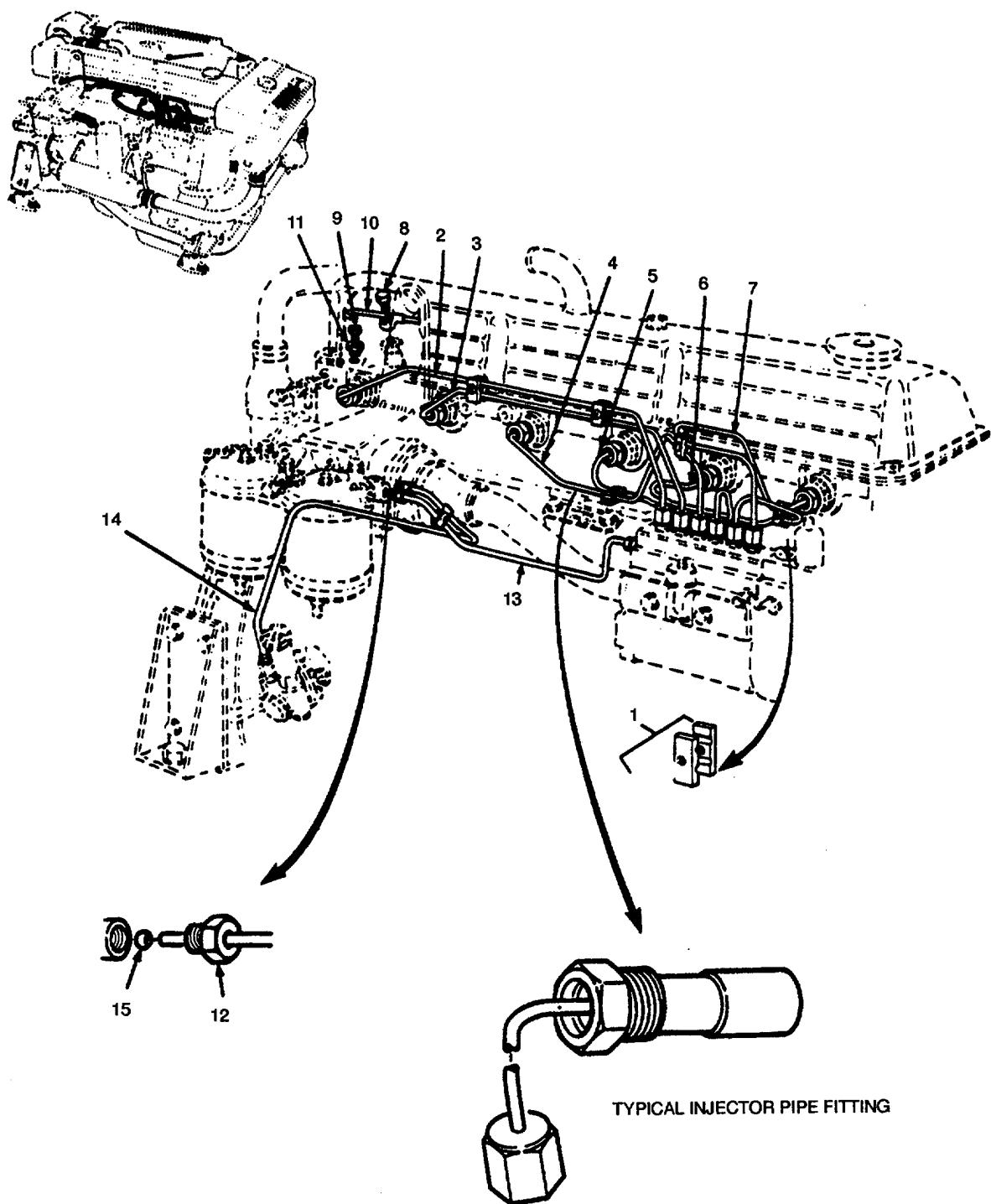
Figure 59. Injector Lines and Fittings.
