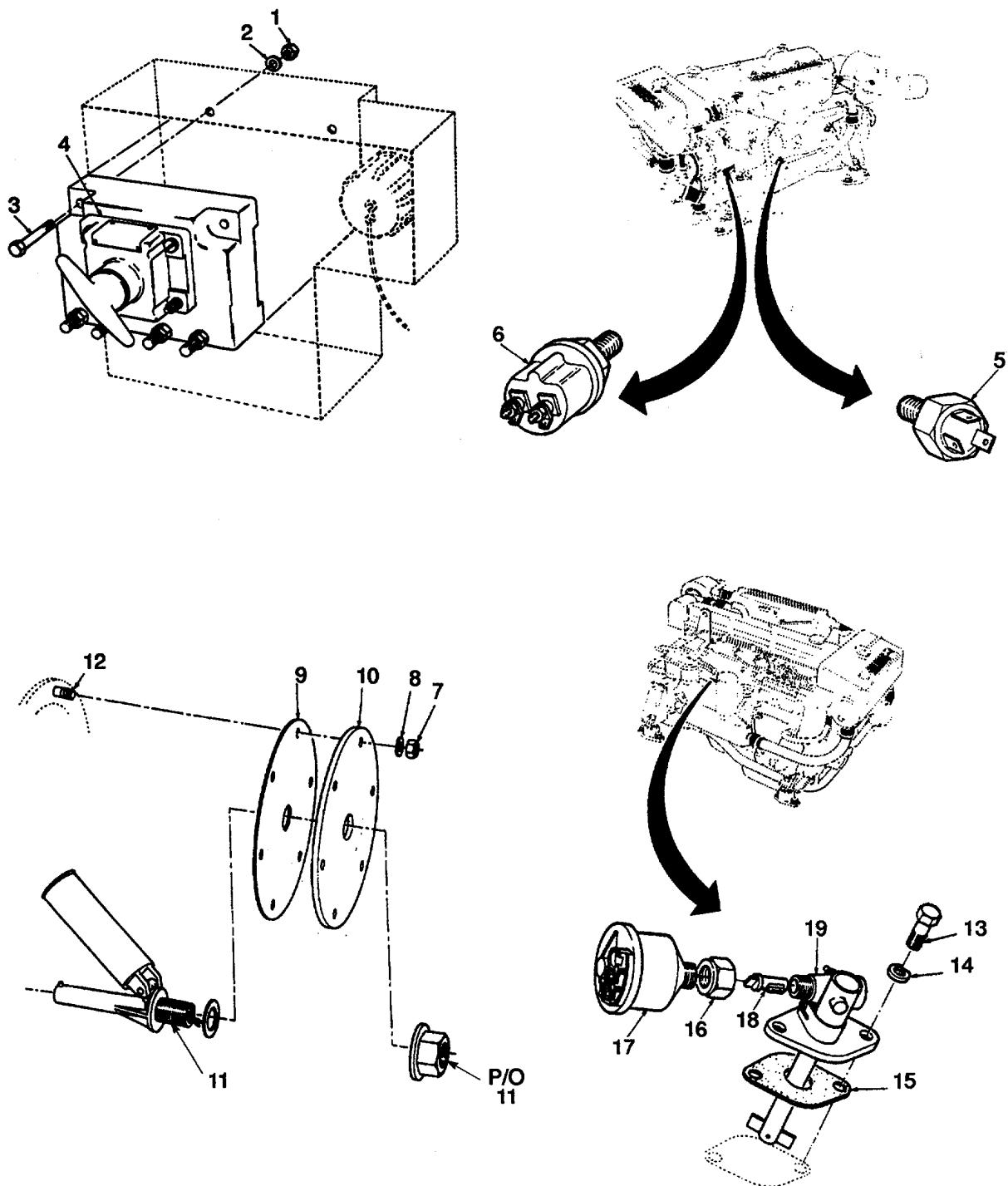
Figure 47. Master Switch, Oil Pressure, Fuel Level
