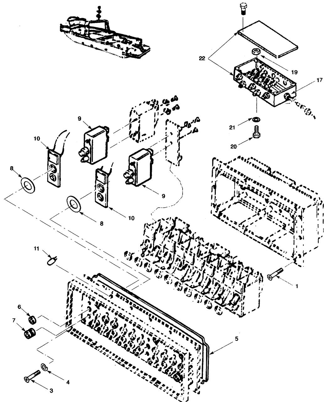
Figure 21. Switch Panel Configuration (Sheet 2 of 2).
