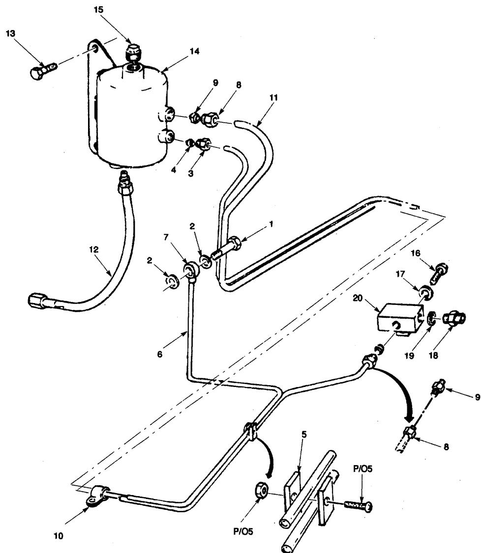
Figure 25. Thermostat Reservoir.
