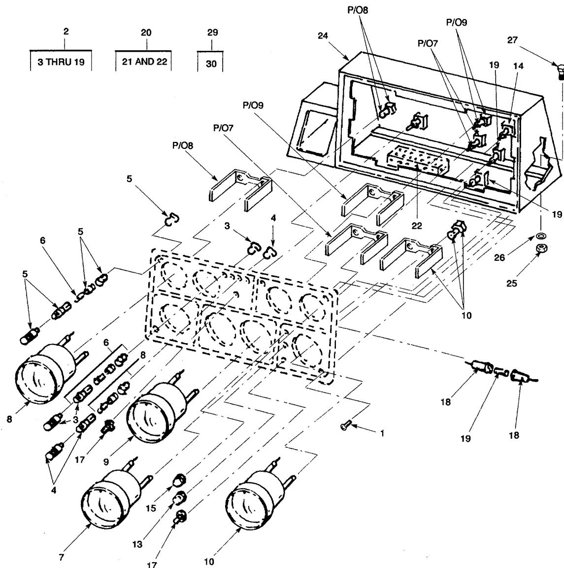
Figure 20. Instrument Panel and Warning Lights (Sheet 1 of 2).
