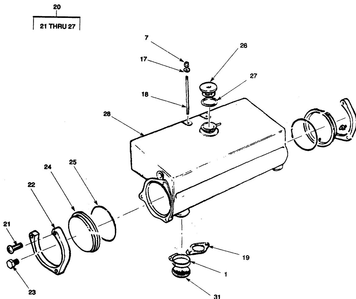
Figure 35. Heat Exchange/Header Tank (Sheet 2 of 2).
