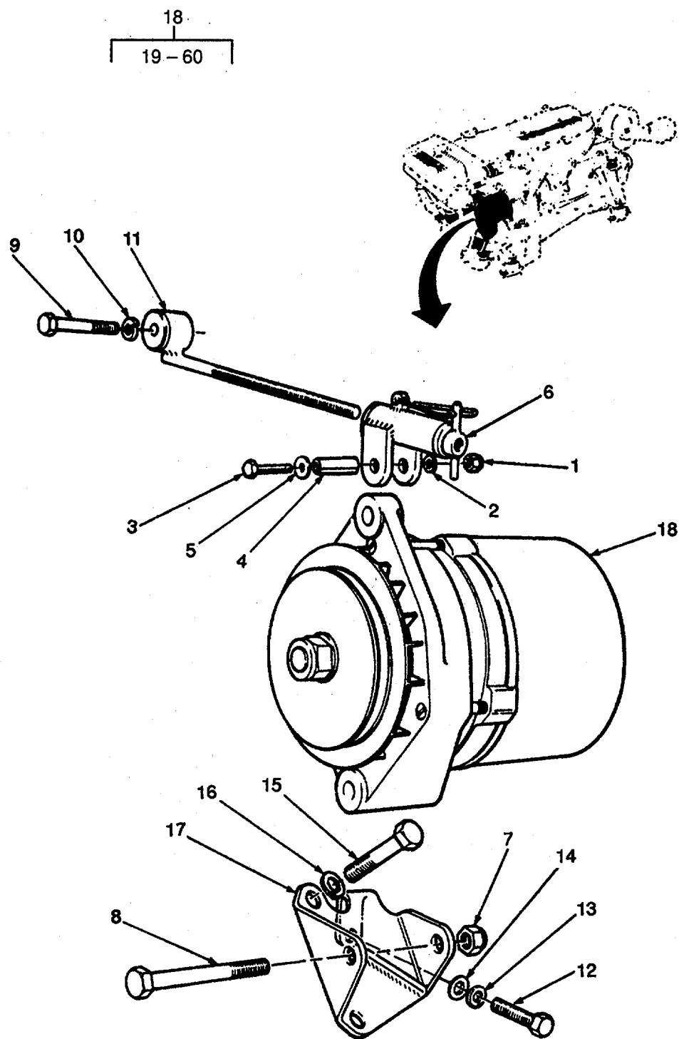
Figure 44. AC5 Alternator and Support Bracket (Sheet 1 of 3).
