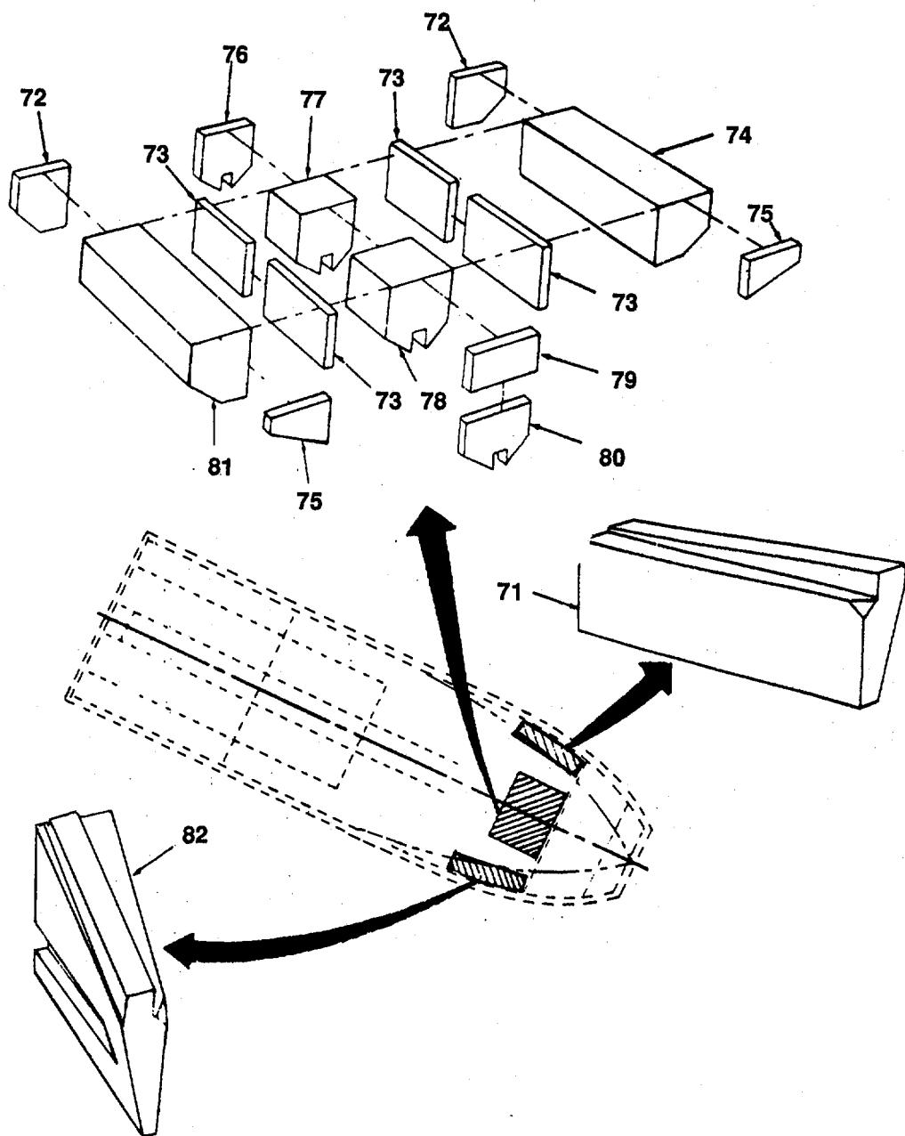
Figure 82. Buoyancy Blocks MK-2 (Sheet 6 of 7).
