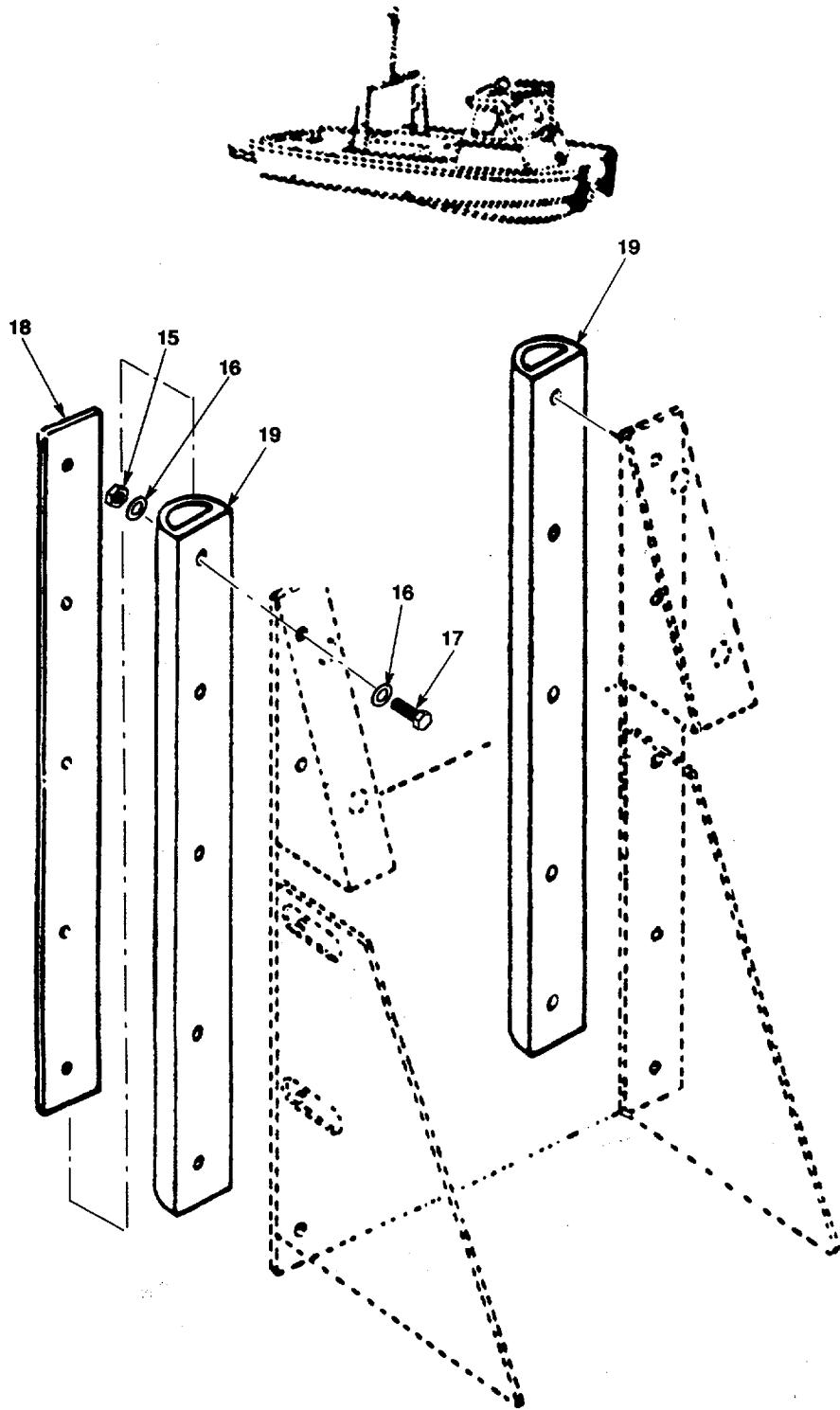
Figure 7. Pushing Knee MK-2 Configuration (Sheet 2 of 2).
