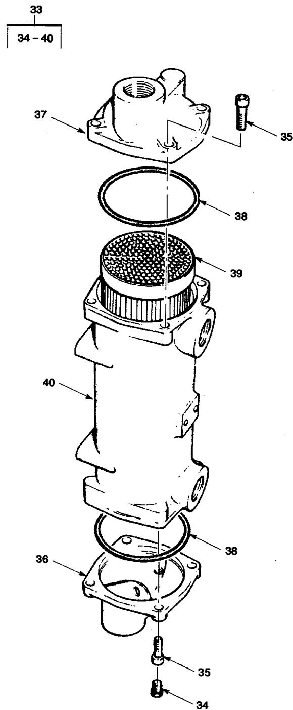
Figure 32. Raw Water (Sheet 3 of 3).
