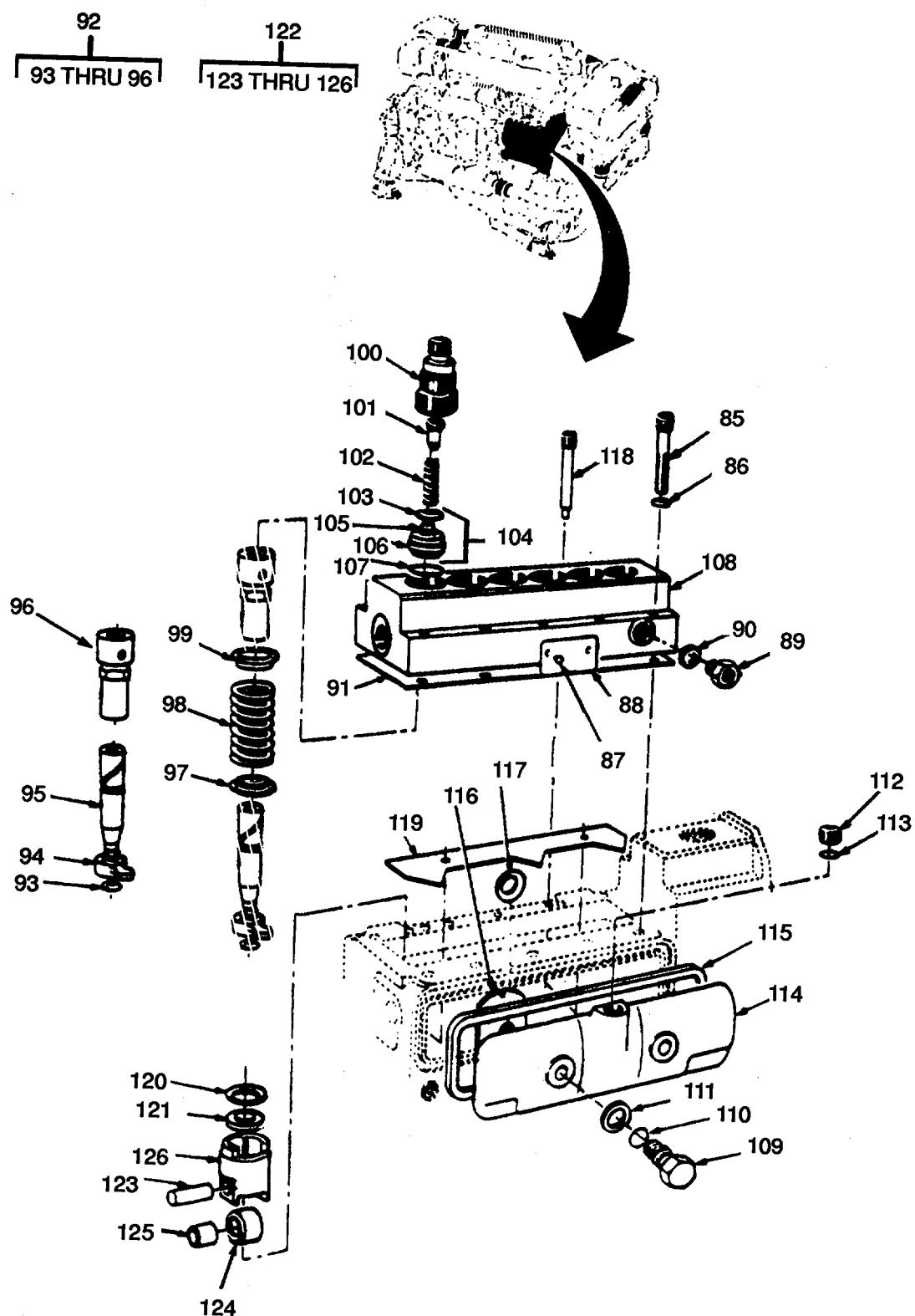
Figure 58. Injector Pump Assembly (Sheet 3 of 6)
