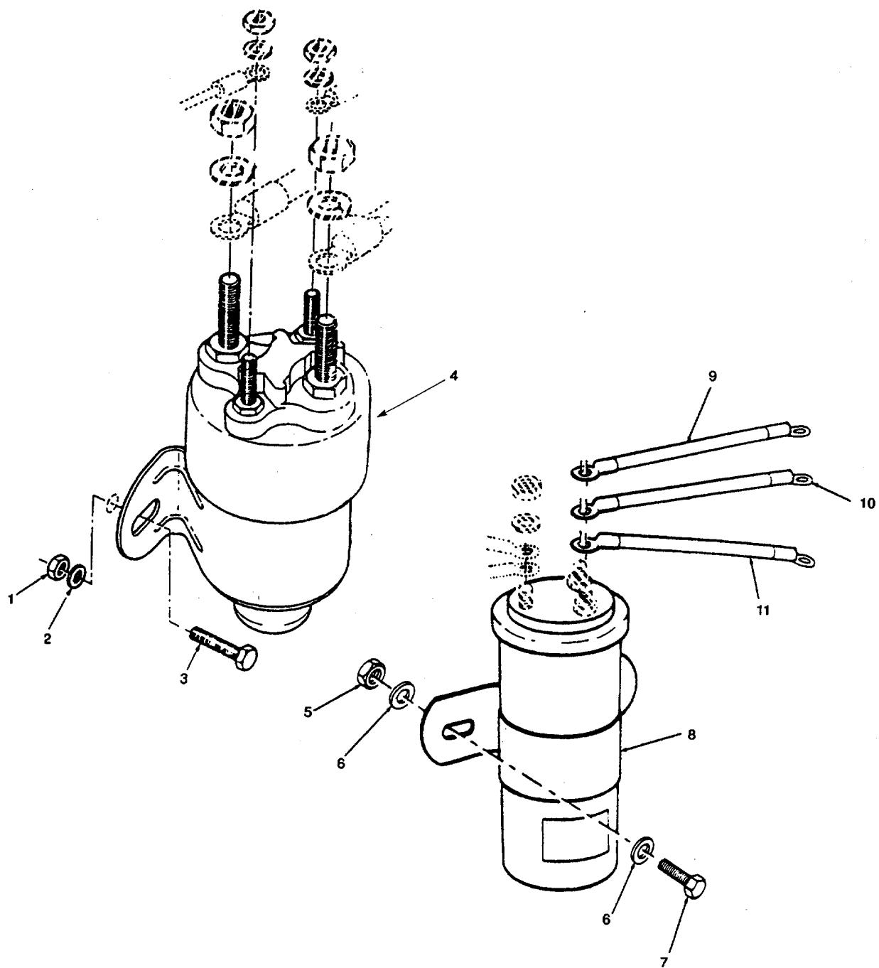
Figure 51. Blocking Diode & Solenoid
