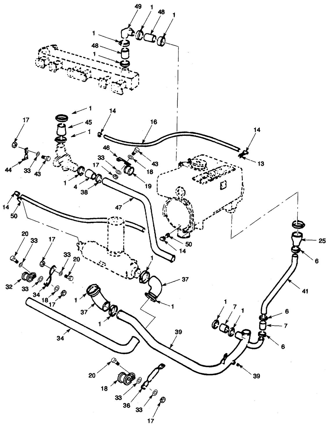
Figure 33. Intercooler System (Sheet 3 of 4).
