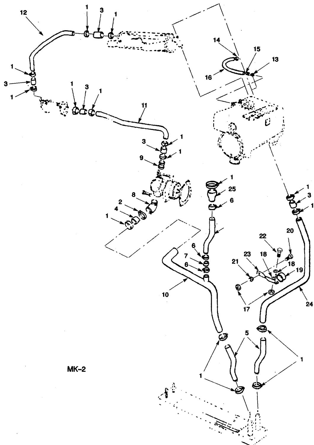
Figure 33. Intercooler System (Sheet 1 of 4).
