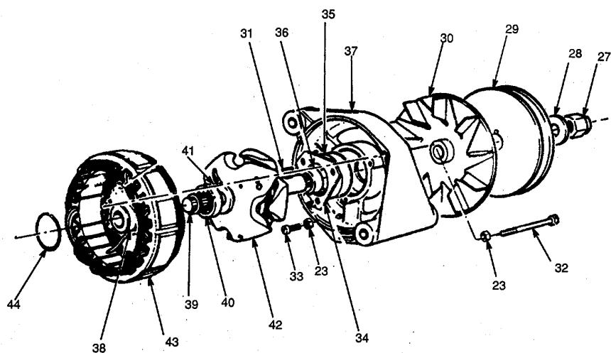
Figure 44. AC5 Alternator and Support Bracket (Sheet 3 of 3).
