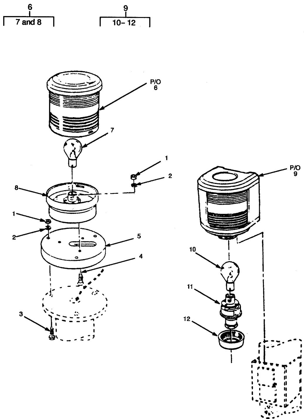
Figure 45. Navigation Lights MK-1 (Sheet 1 of 2).
