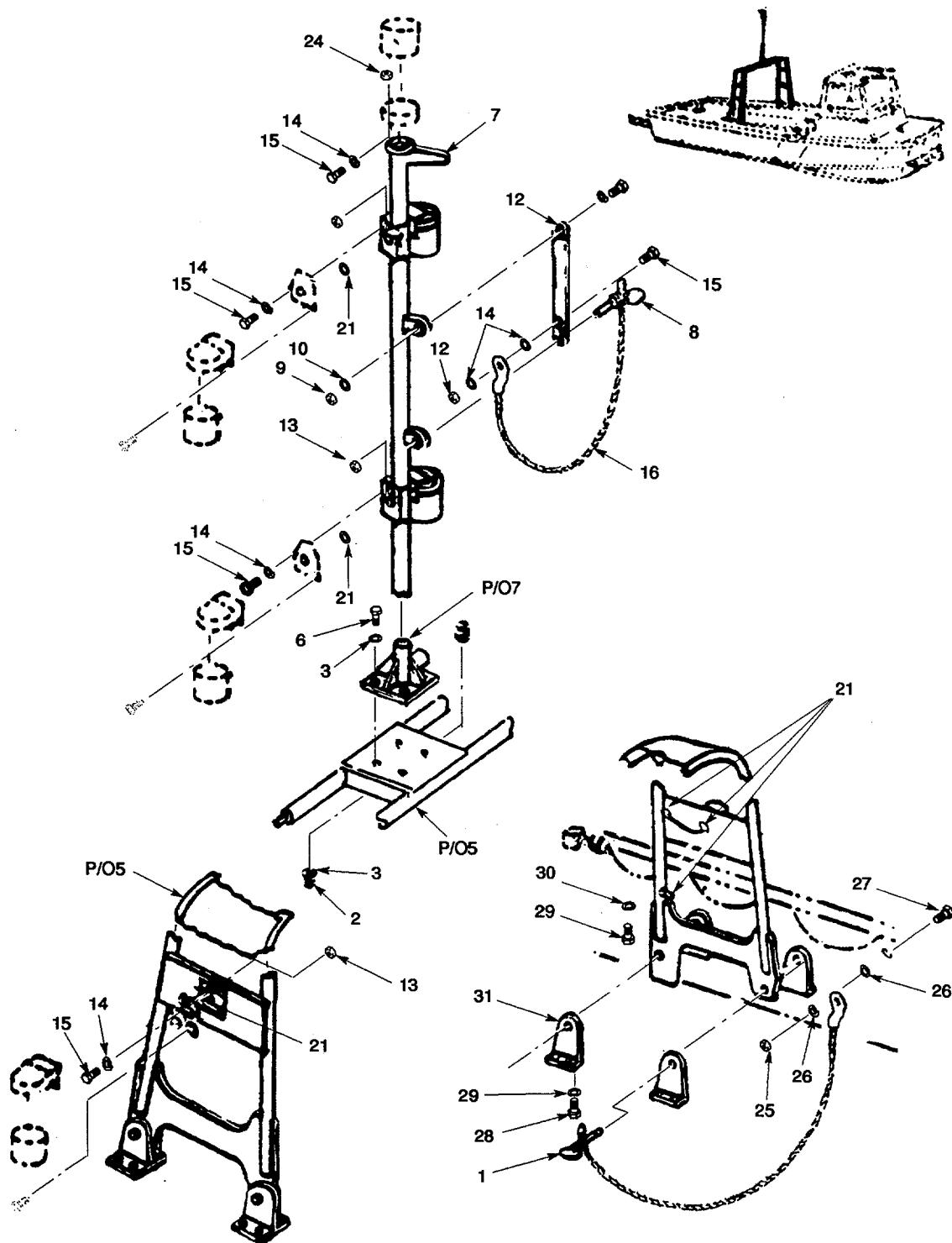
Figure 1. Mast Assembly with Wiring MK-2 (Sheet 2 of 2).
