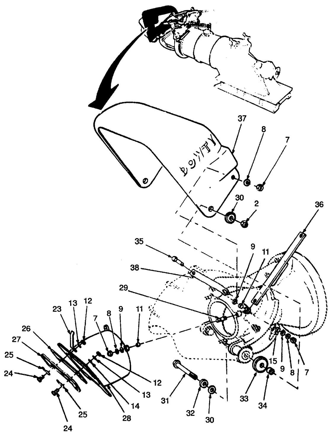
Figure 72. Hydro Jet Unit, Steering Assembly (Sheet 2 of 6).
