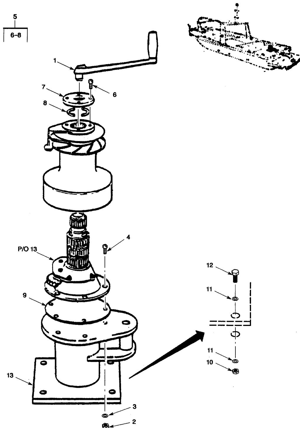
Figure 6. Capstan and Tow Hook (Sheet 1 of 3).
