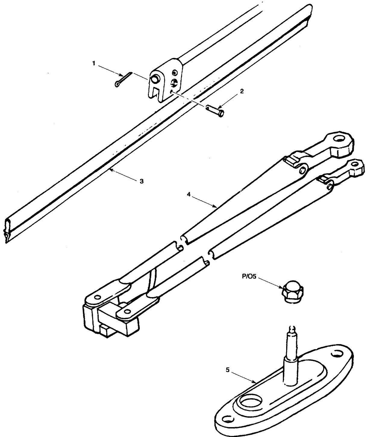
Figure 3. Windshield Wiper Blade.
