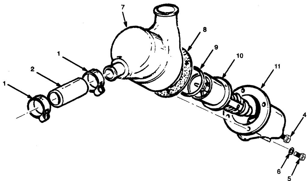
Figure 36. Thermostat Assembly.
