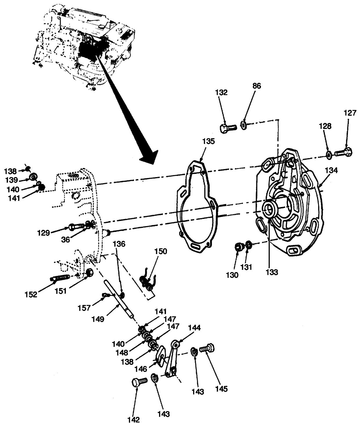
Figure 58. Injector Pump Assembly (Sheet 4 of 6).
