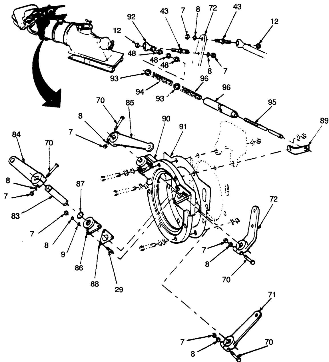
Figure 72. Hydro Jet Unit, Steering Assembly (Sheet 5 of 6).
