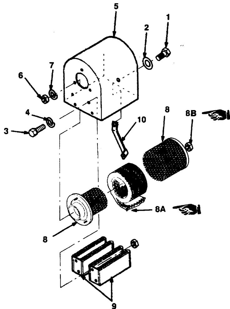
Figure 54. Air Filter Cover, Filter Element and Silencer.
