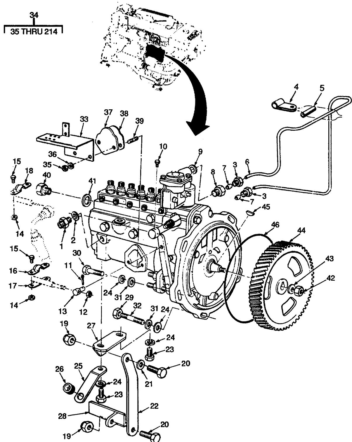
Figure 58. Injector Pump Assembly (Sheet 1 of 6).
