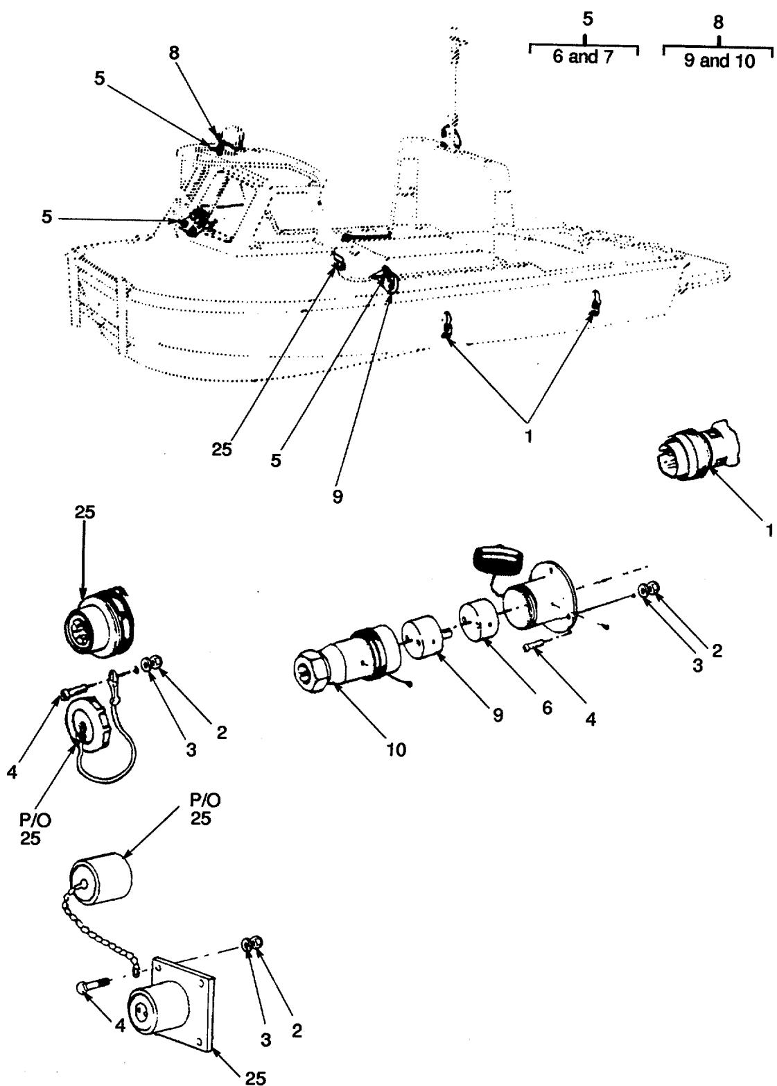
Figure 50. Plugs and Sockets (Sheet 1 of 2).
