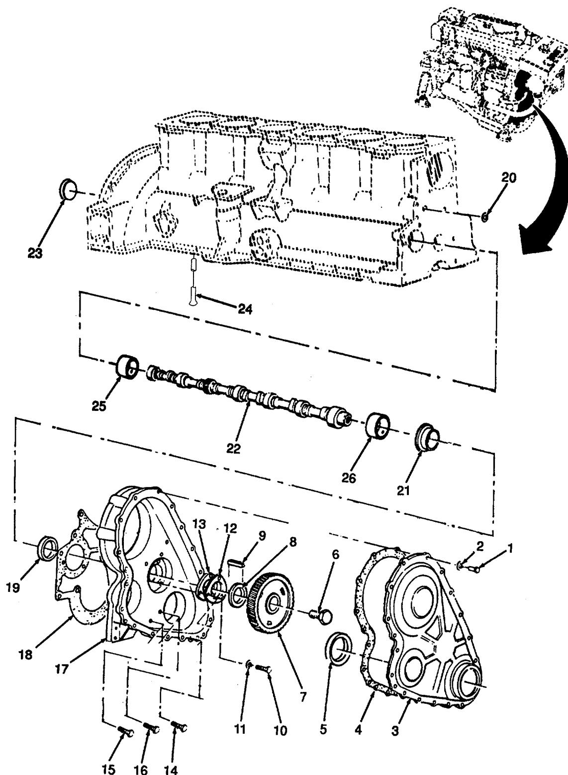
Figure 65. Camshaft Assembly.
