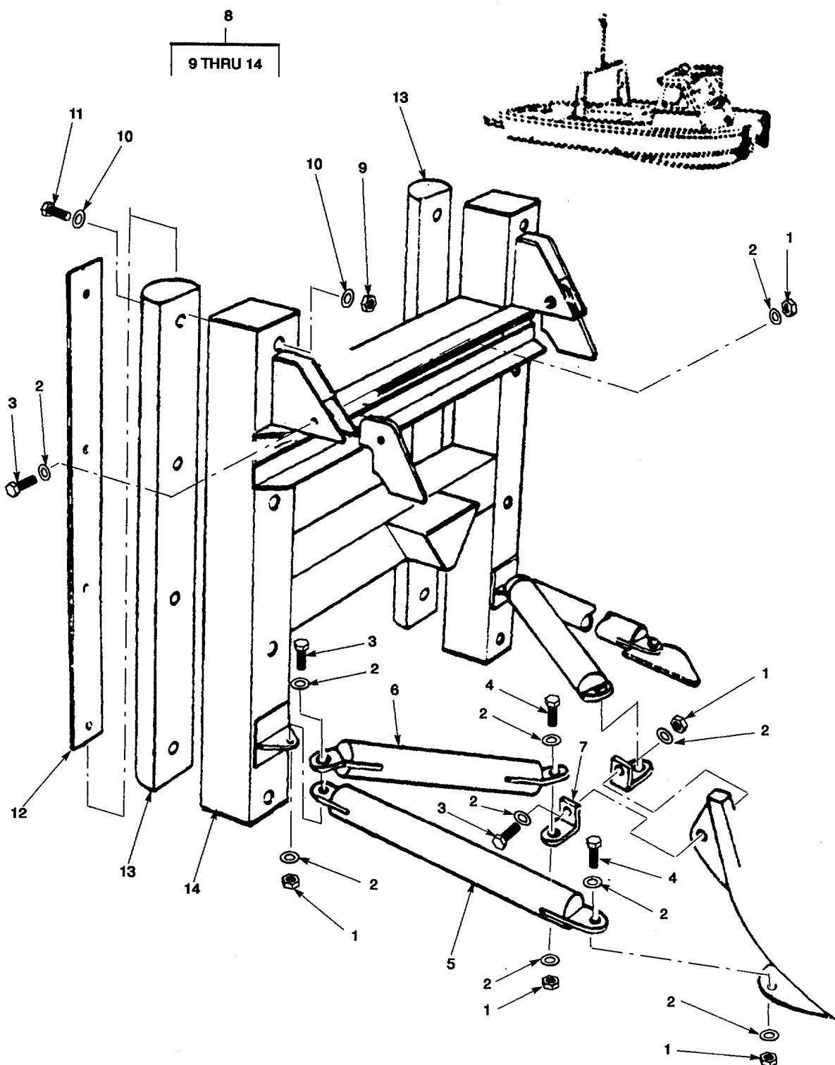
Figure 7. Pushing Knee MK-1 Configuration (Sheet 1 of 2).
