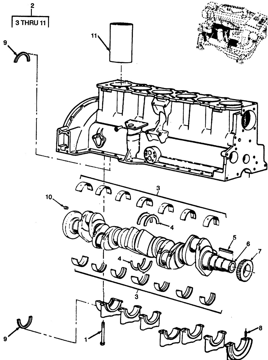
Figure 66. Crankshaft, Main Bearings, Engine Block and Liners.
