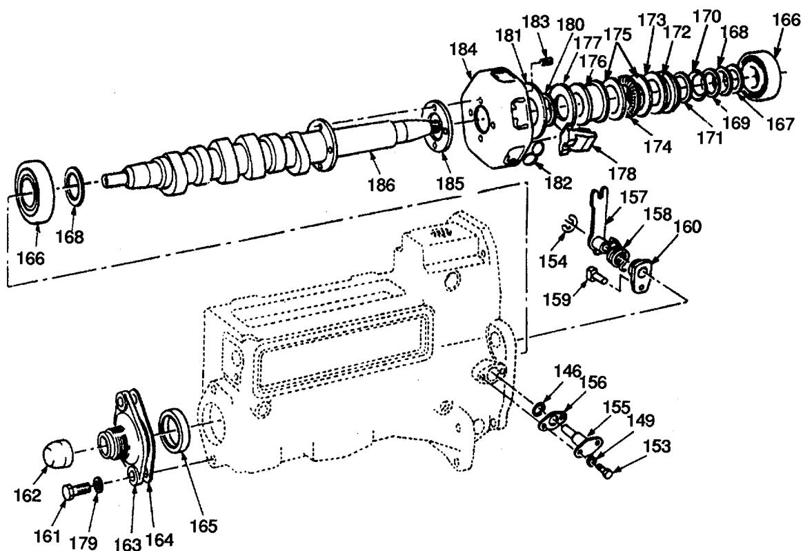
Figure 58. Injector Pump Assembly (Sheet 5 of 6).
