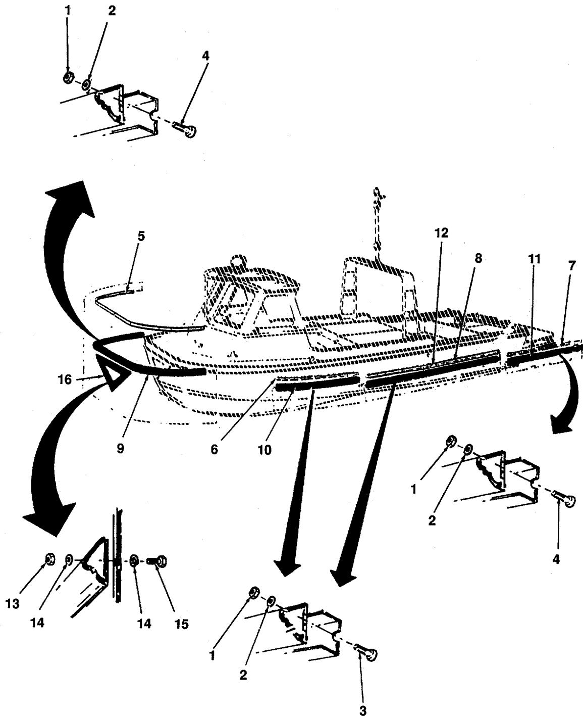
Figure 79. Fendering (Rubber Rubrail).
