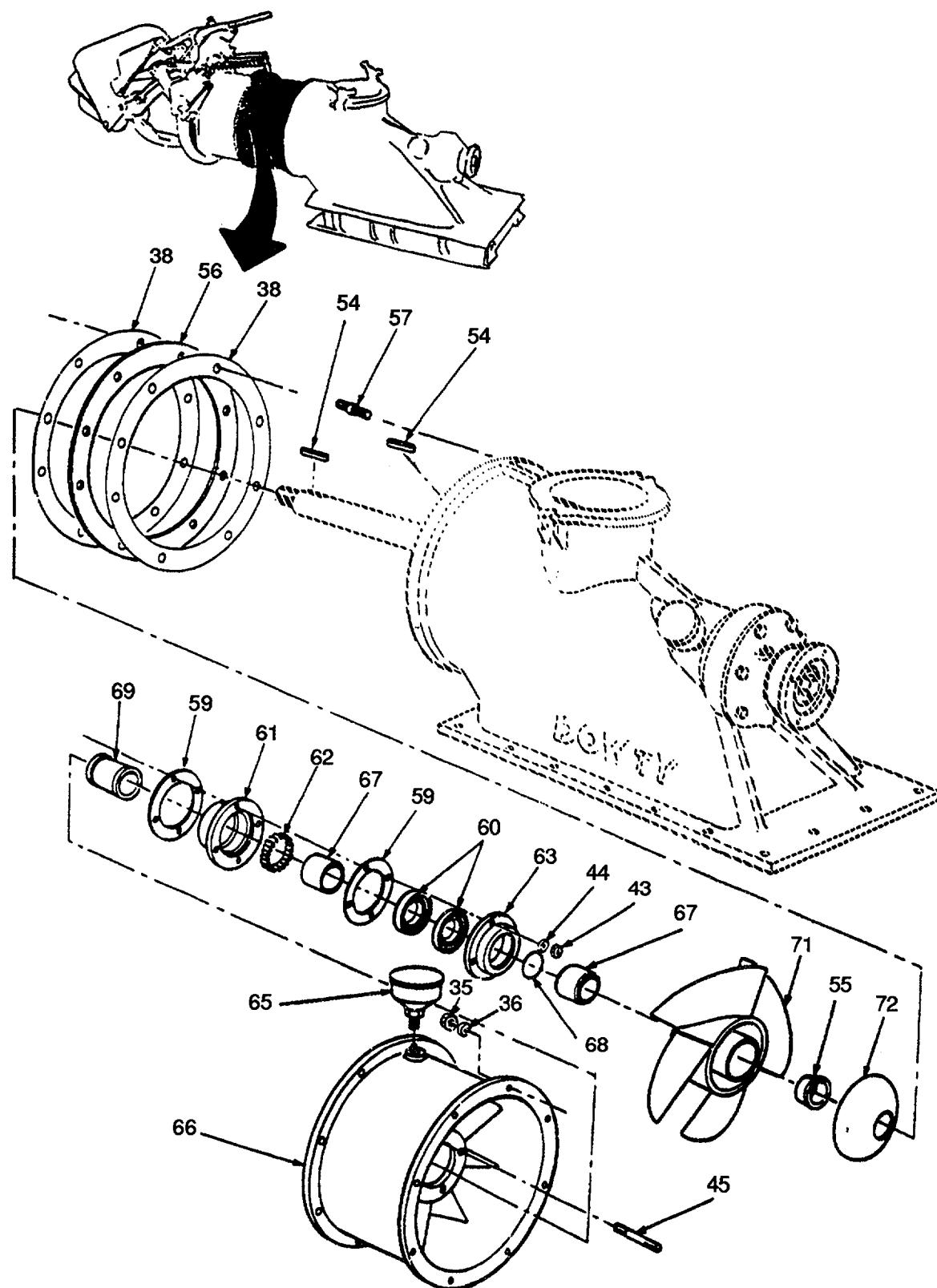
Figure 71. Hydro Jet Assembly (Sheet 4 of 5).
