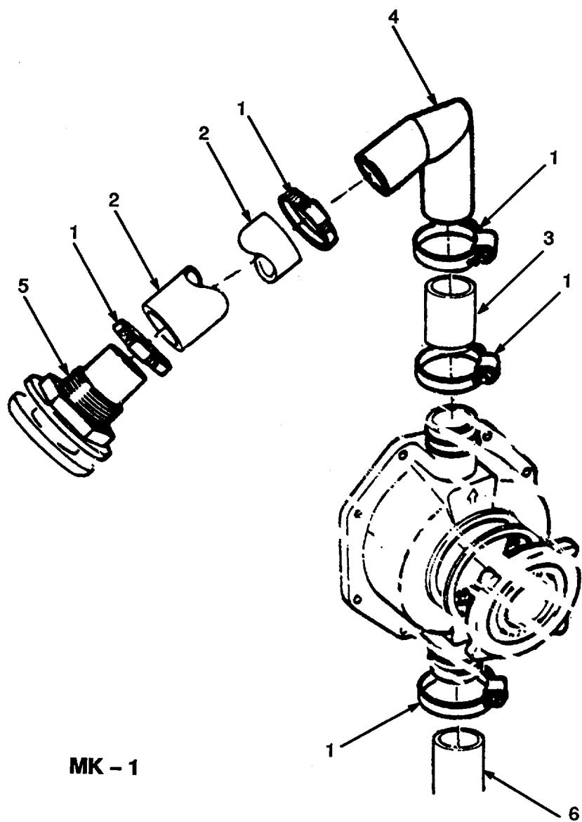
Figure 76. Hand Bilge Pump (Sheet 1 of 2).
