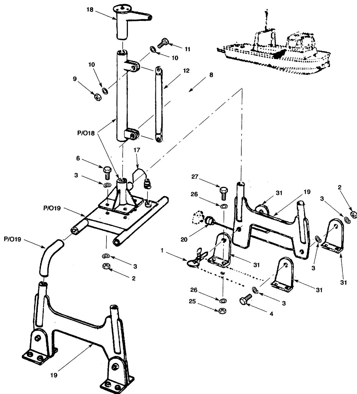
Figure 1. Mast Assembly with Wiring MK-1 (Sheet 1 of 2).
