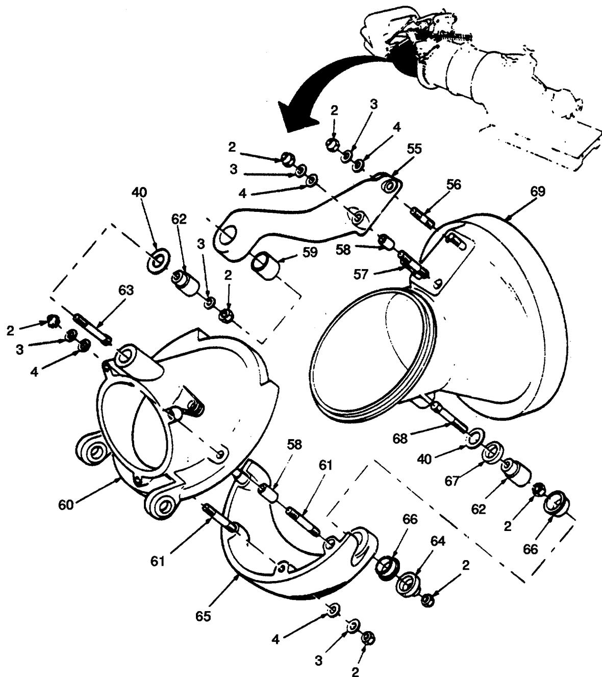
Figure 72. Hydro Jet Unit, Steering Assembly (Sheet 4 of 6).
