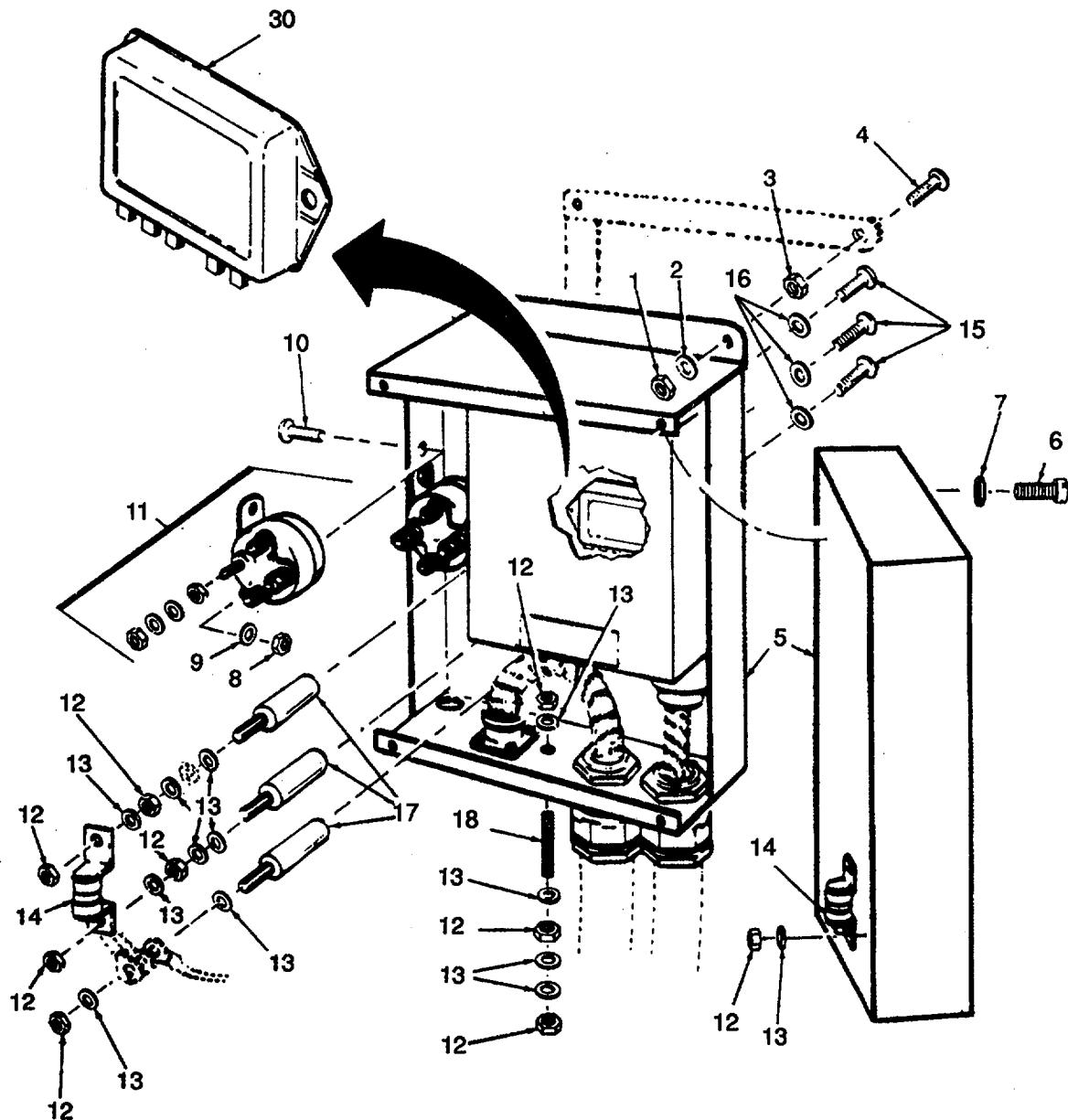
Figure 49. Screened Control Box ( Sheet 1 of 2 ).
