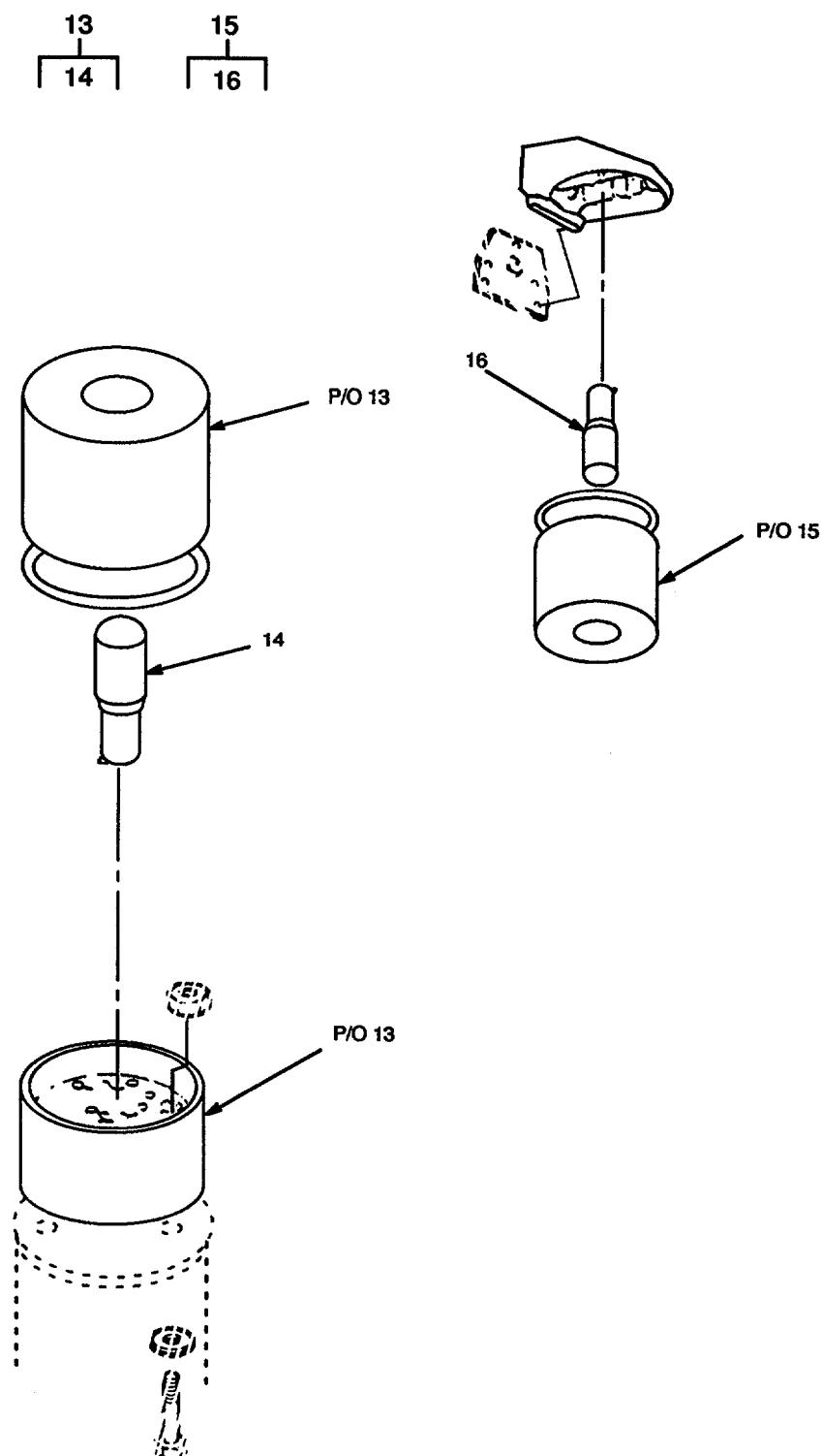
Figure 45. Navigation Lights MK-2 (Sheet 2 of 2).
