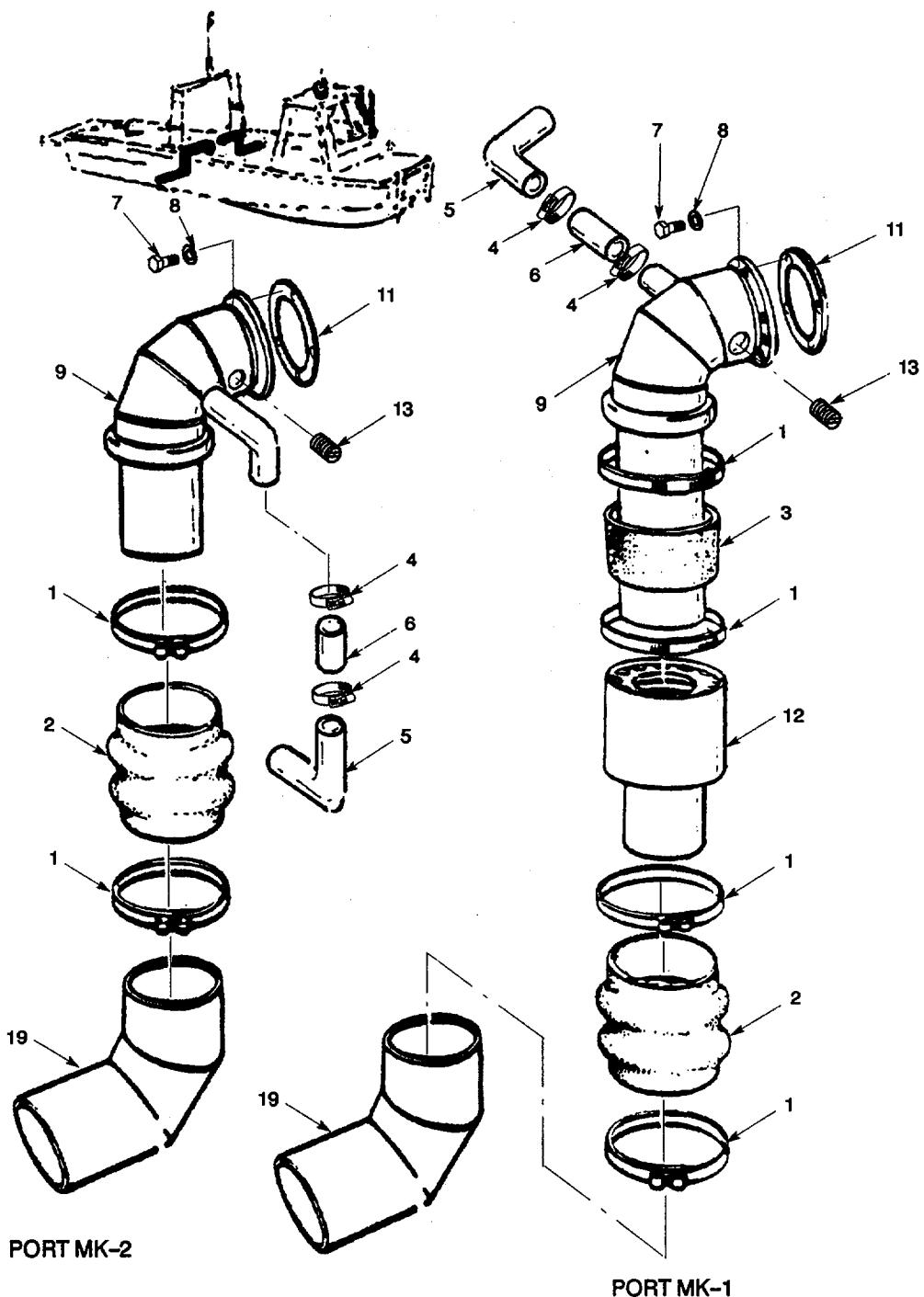
Figure 29. Exhaust Arrangement Port Engine (Sheet 1 of 2).
