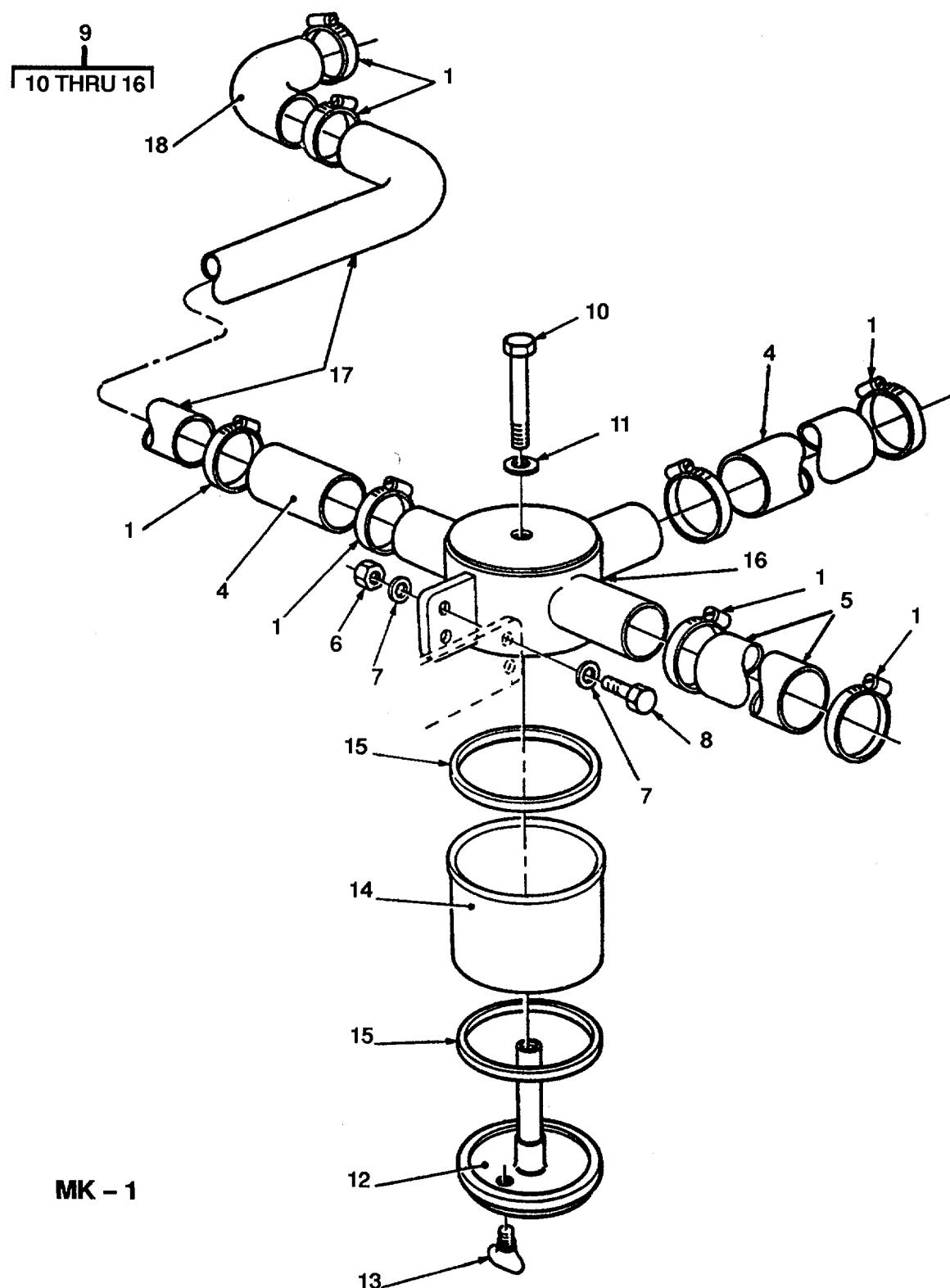
Figure 68. Engine Breather Water Trap Assembly (Sheet 2 of 2).
