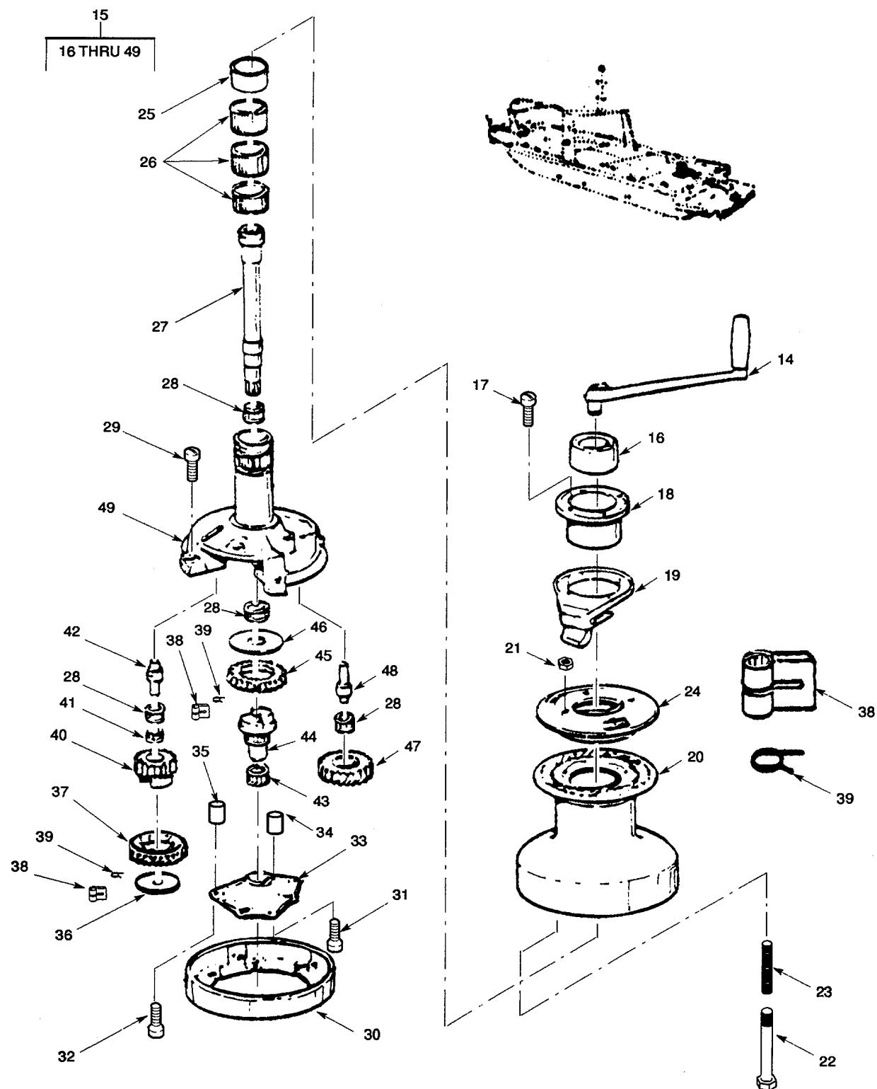
Figure 6. Capstan and Tow Hook MK-2 (Sheet 2 of 3)
