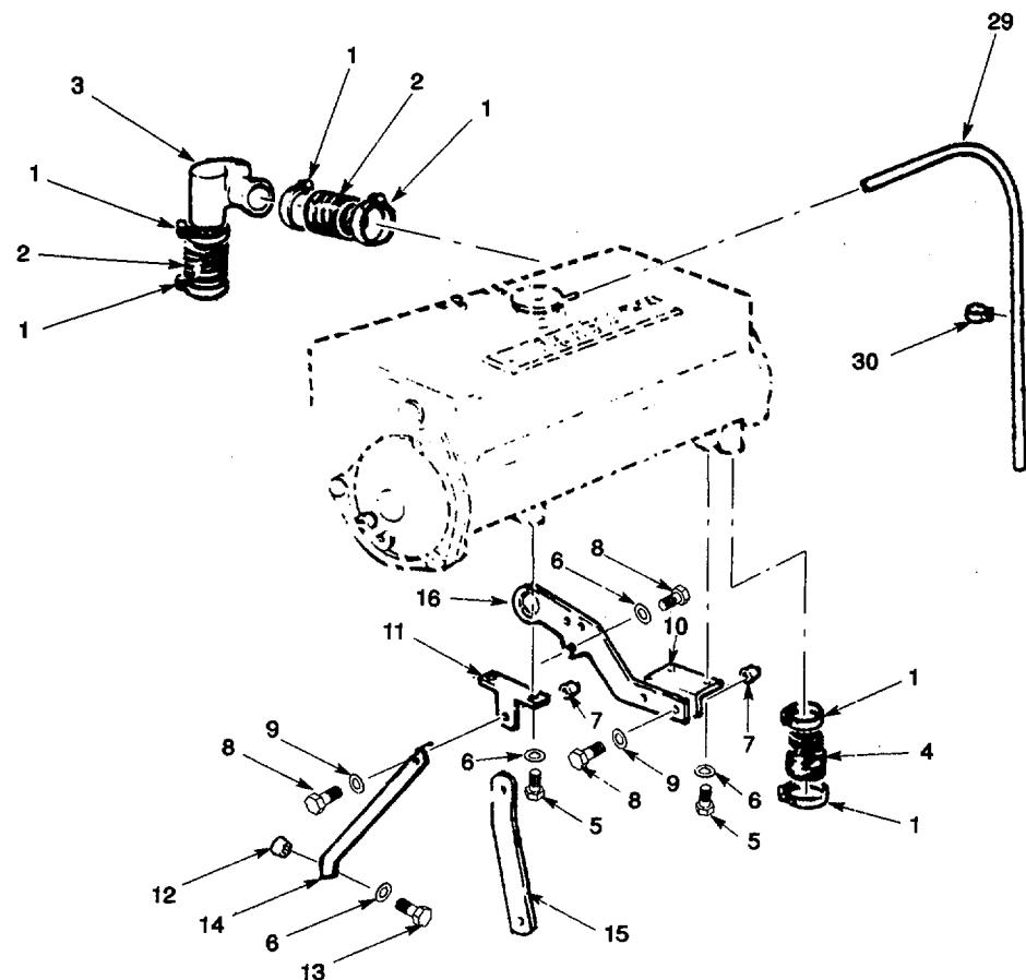
Figure 35. Heat Exchanger/Heater Tank (Sheet 1 of 2).
