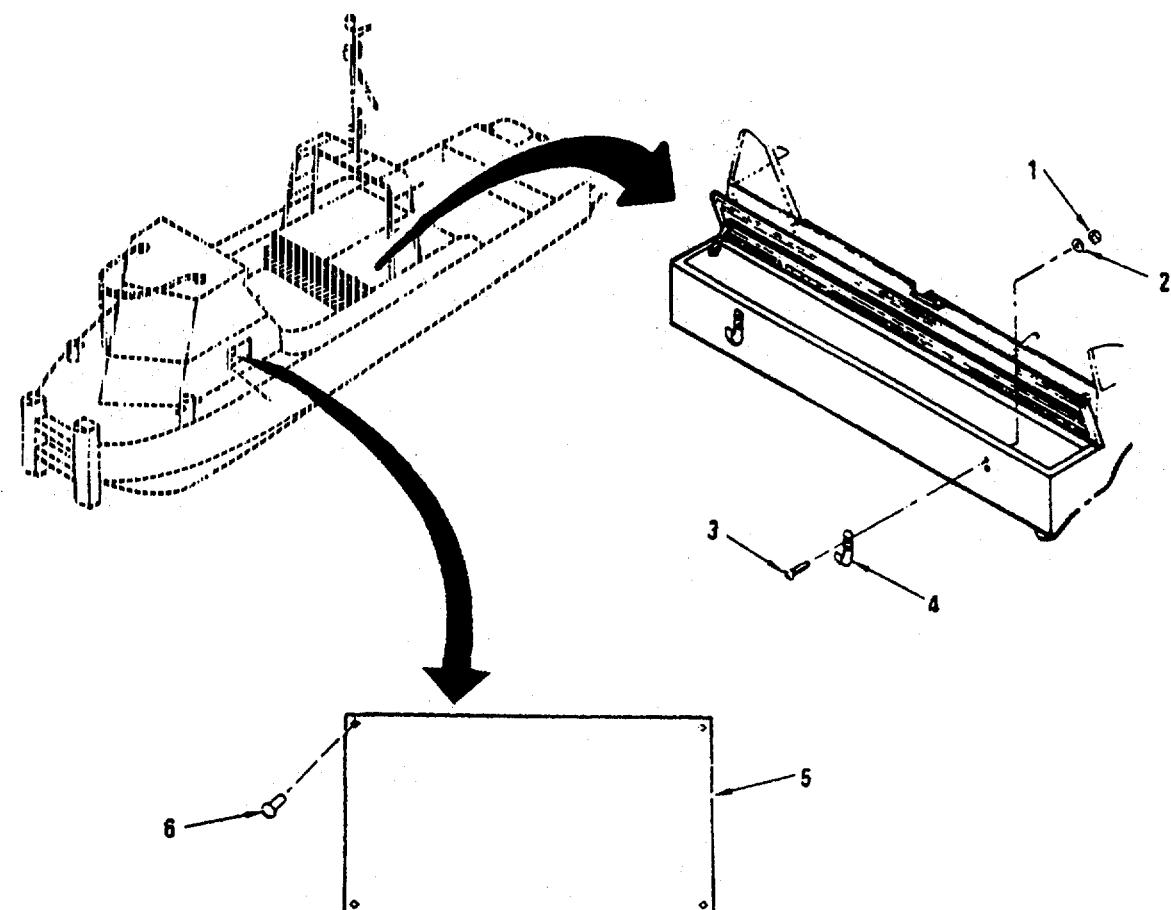
Figure 85. Boat Hook Holder and identification Plate MK-2.
