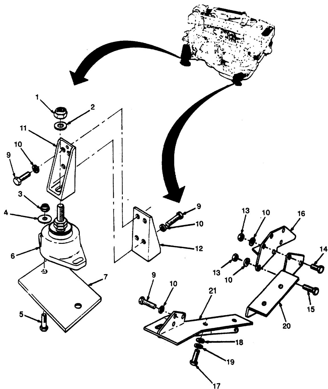
Figure 52. Engine, Mounts, and Brackets (Sheets 1 of 2).
