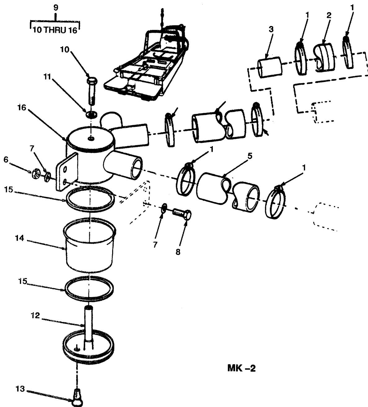
Figure 68. Engine Breather Water Trap Assembly (Sheet 1 of 2).
