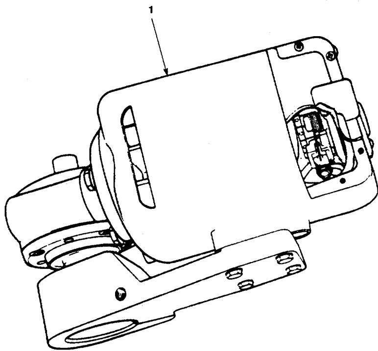
*Figure 4. Windshield Wiper Motor.*
