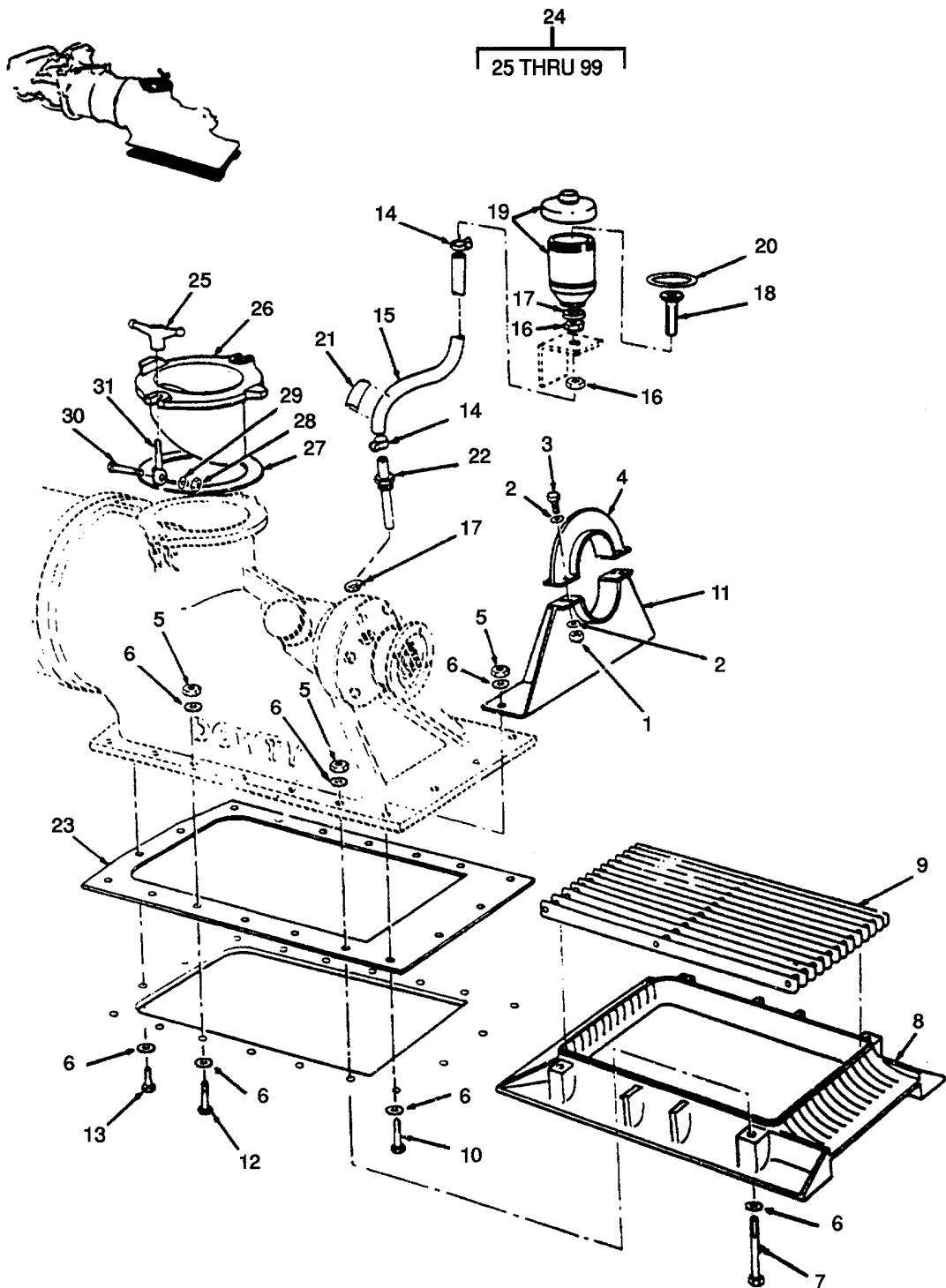
Figure 71. Hydro Jet Assembly (Sheet 1 of 5).
