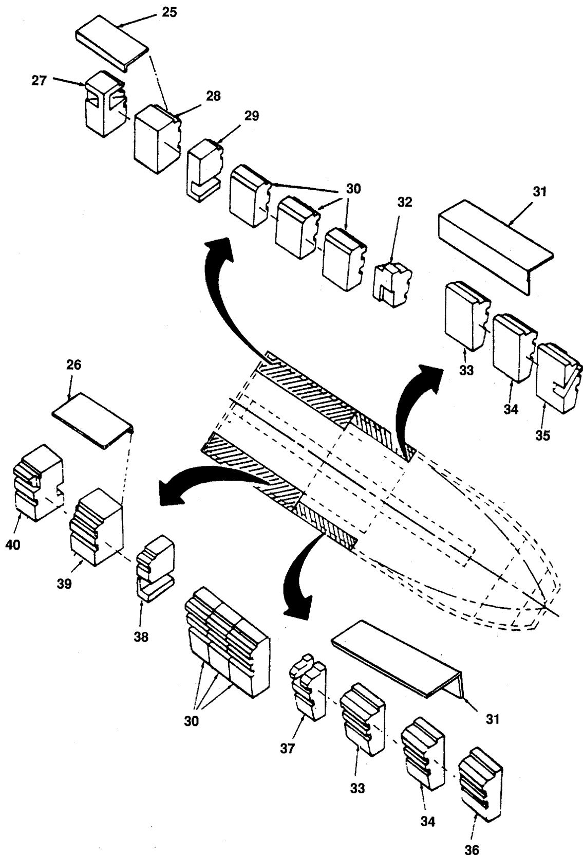
Figure 82. Buoyancy Blocks MK-2 (Sheet 3 of 7).
