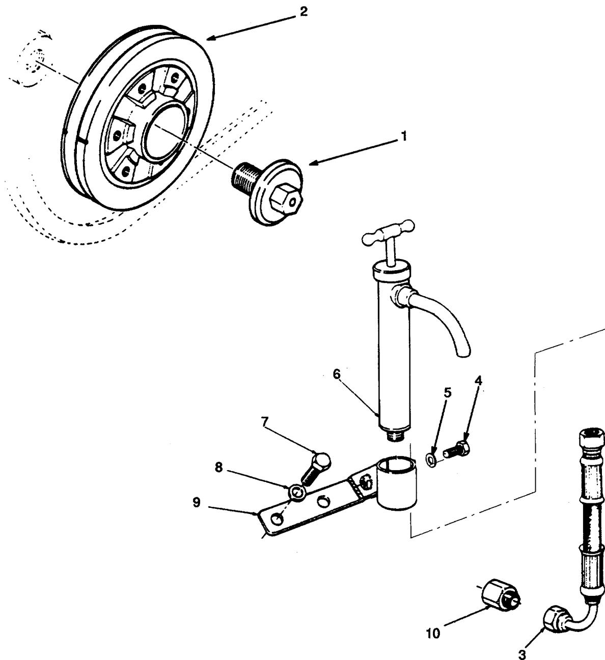
Figure 53. Crank Shaft Pulley and Sump Pump Assembly.
