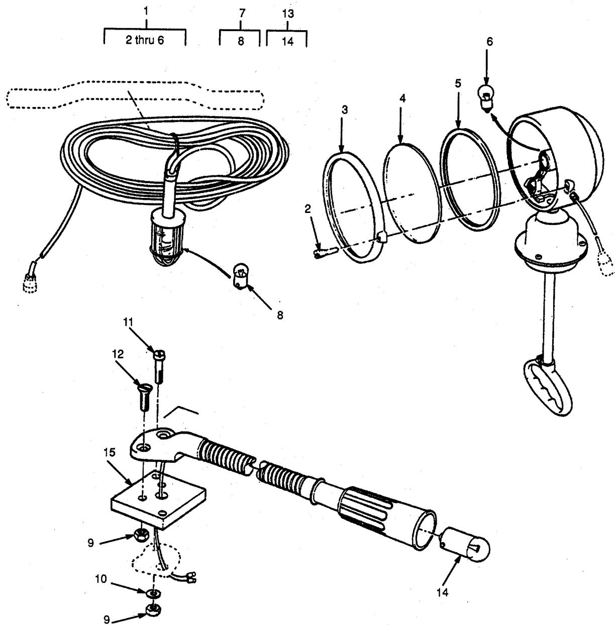
Figure 46. Searchlight, Inspection and Map Reading Lights.
