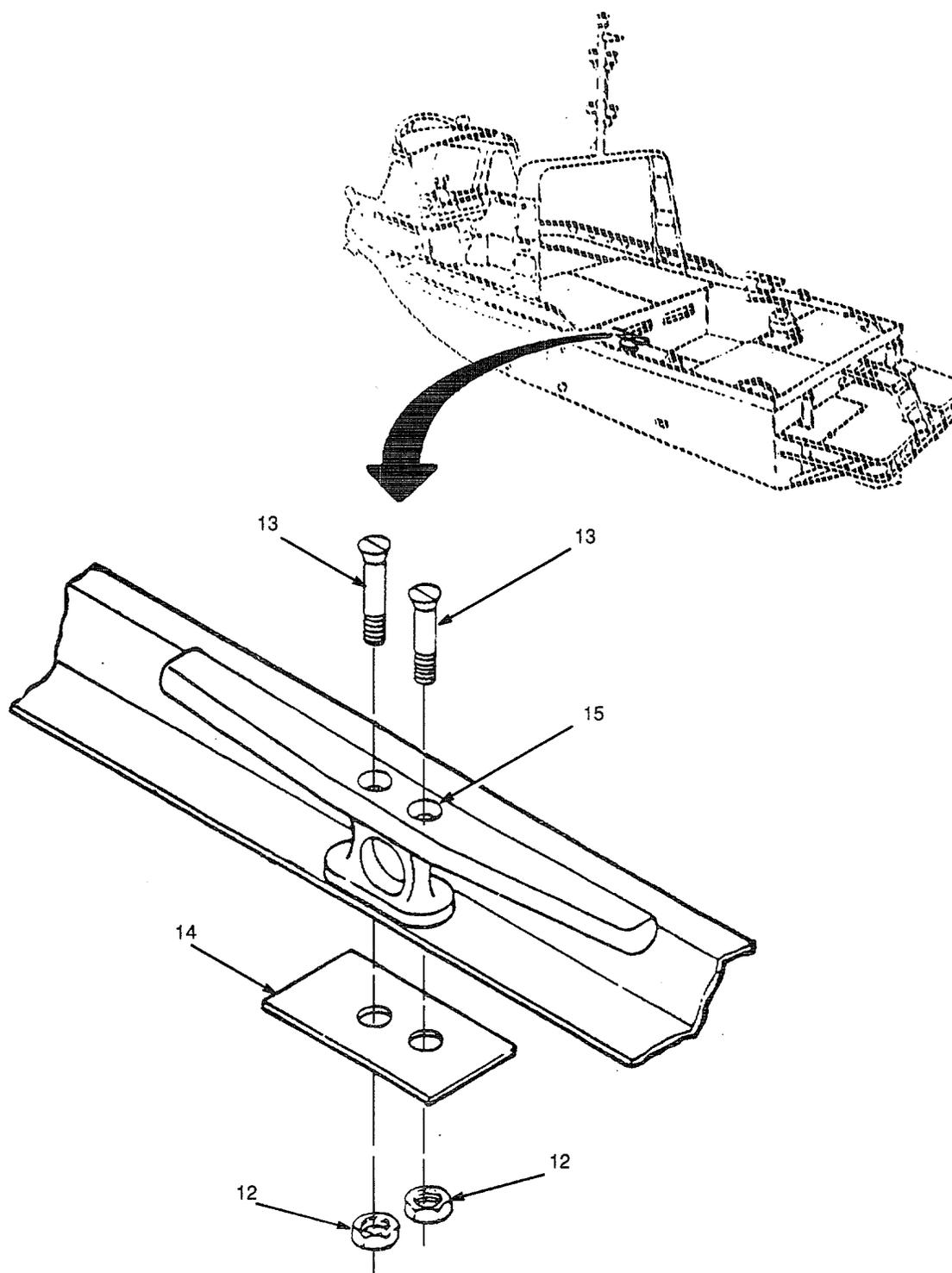
Figure 84. Diving Platform , Hinged Flap, (Sheet 2 of 2)
