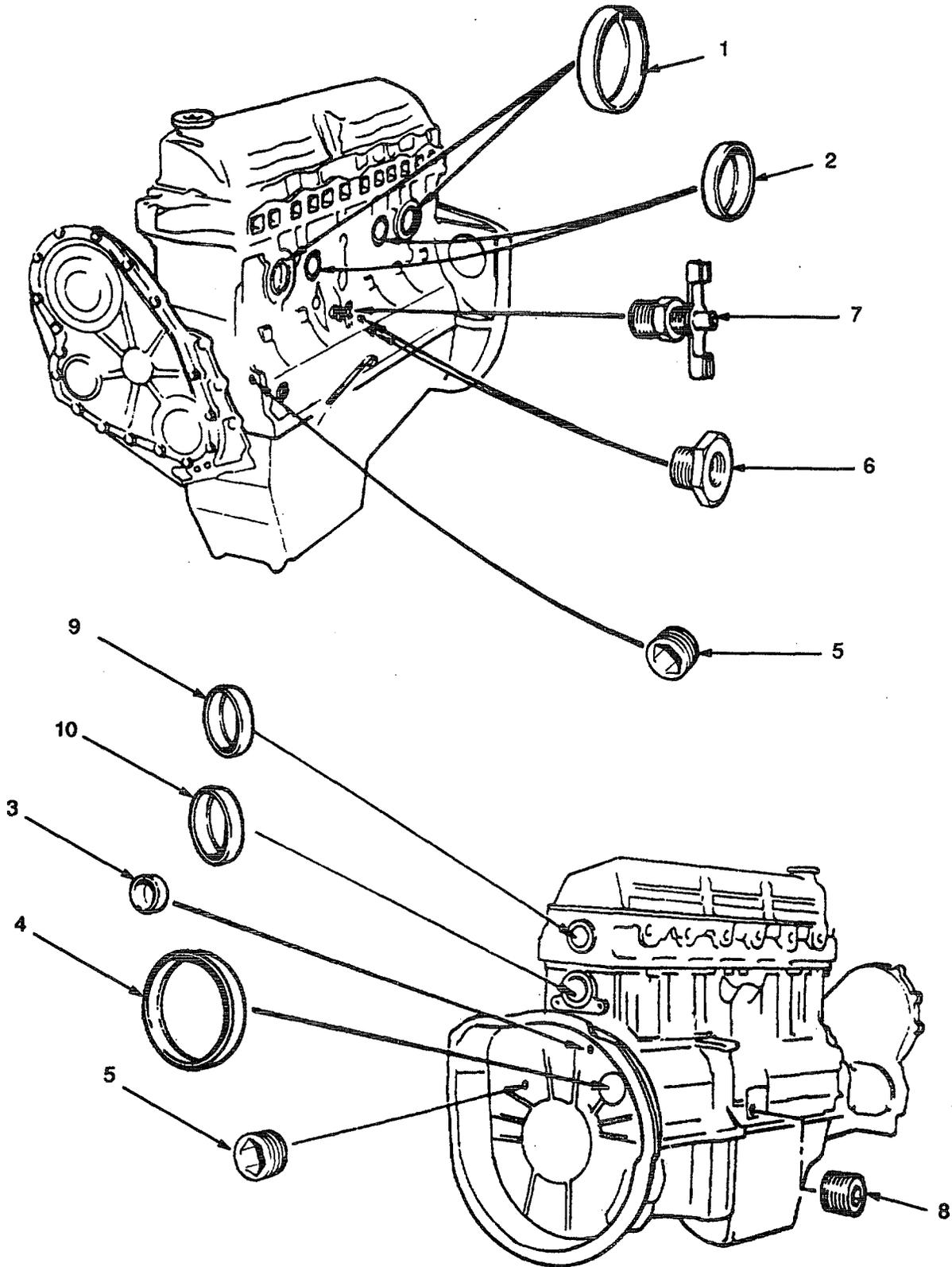
Figure 69. Core and Gallery Plugs, Block Drain Tap
