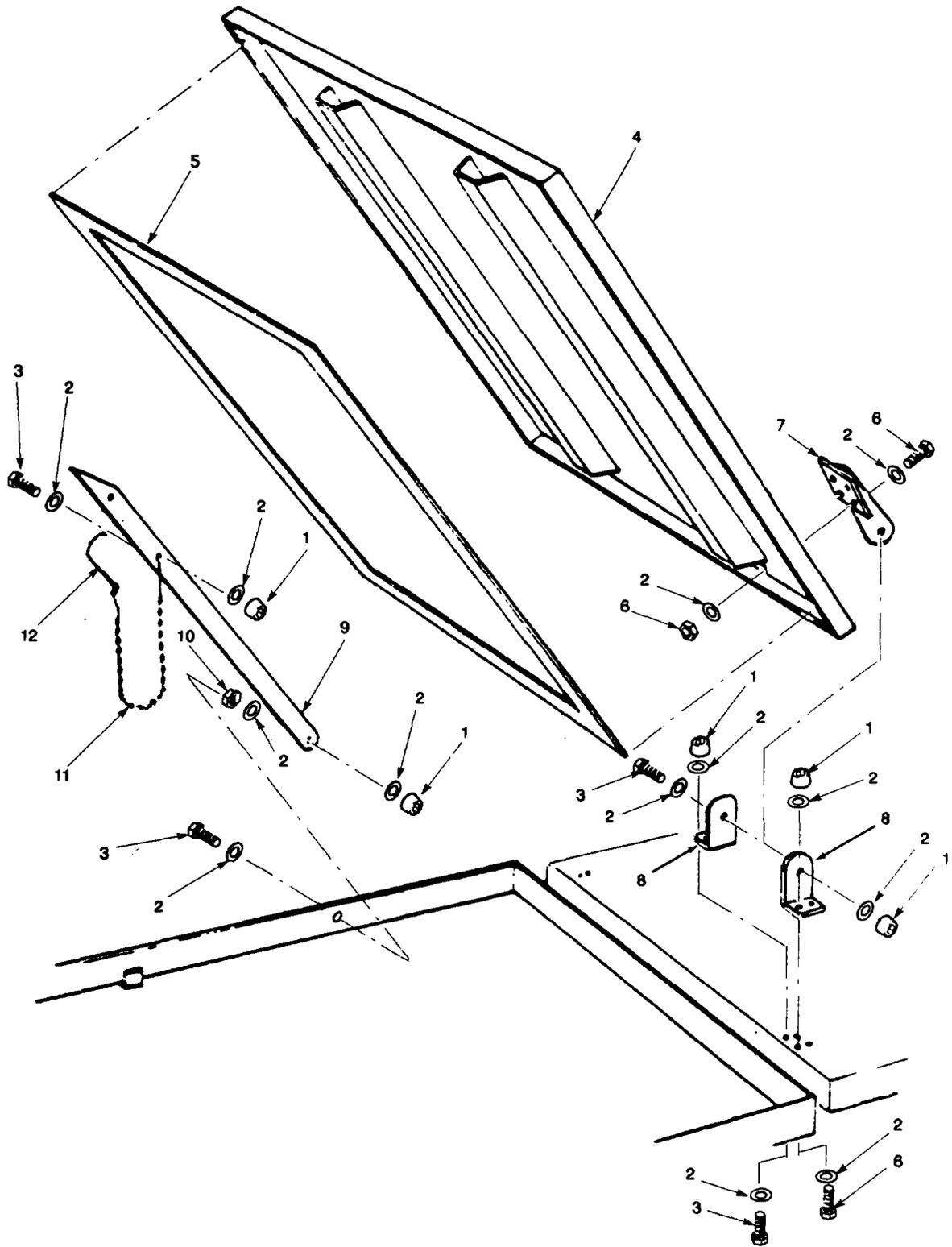
Figure 10. Jet Hatch Cover.
