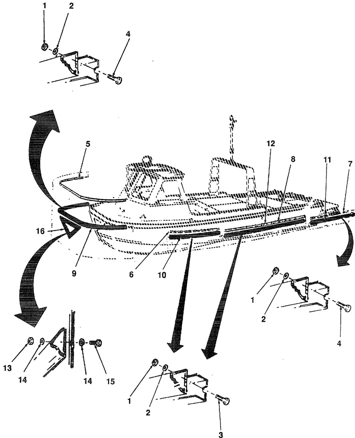
Figure 79. Fendering (Rubber Rubrail).
