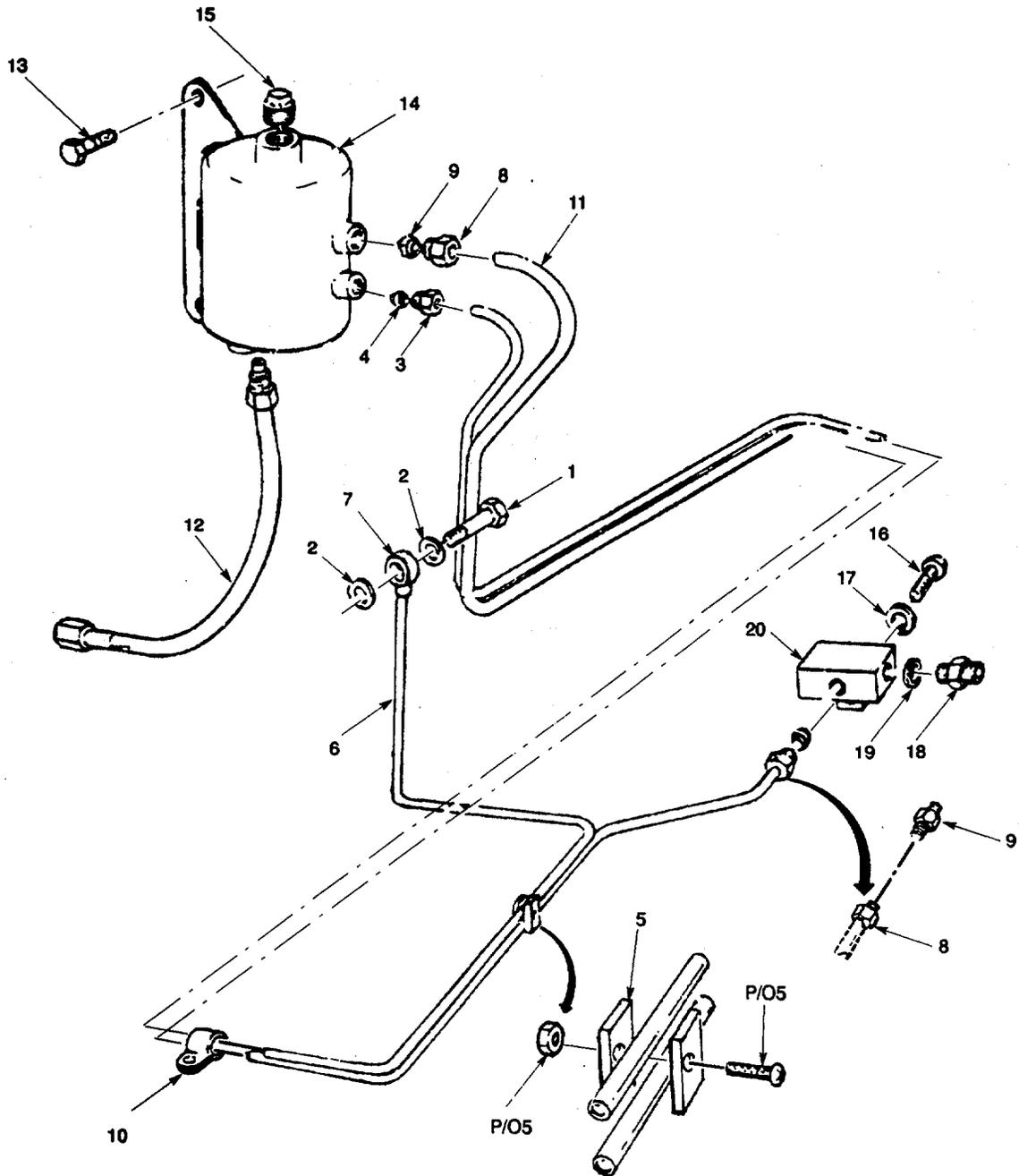
Figure 25. Thermostat Reservoir.
