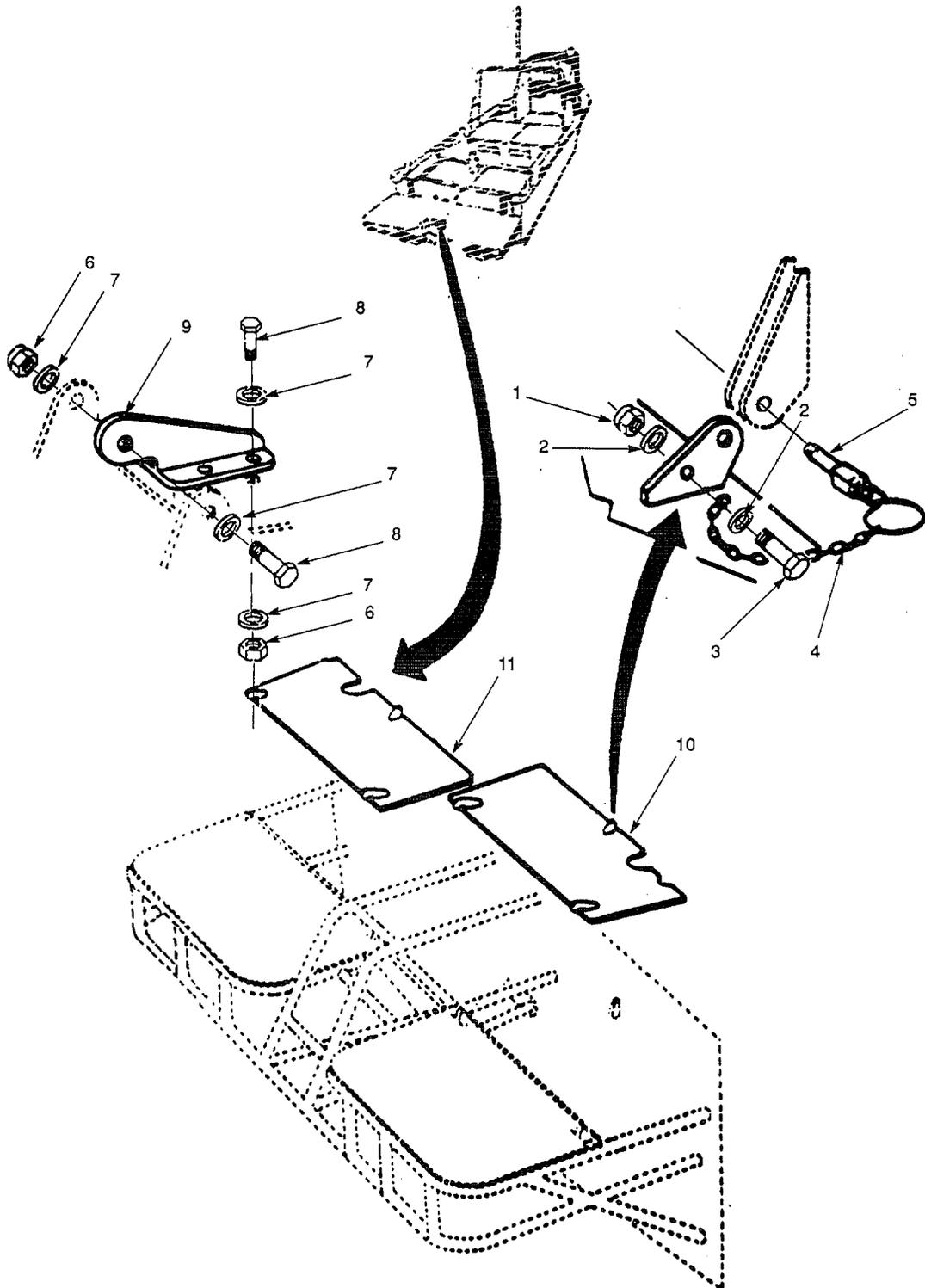
Figure 84. Diving Platform, Hinged Flap. (Sheet 1 of 2)
