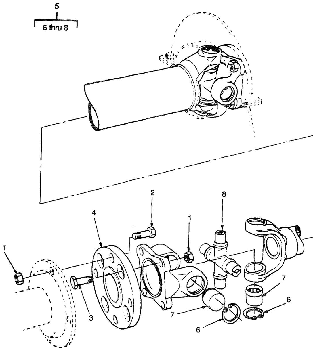
Figure 74. Drive Shaft Assembly.
