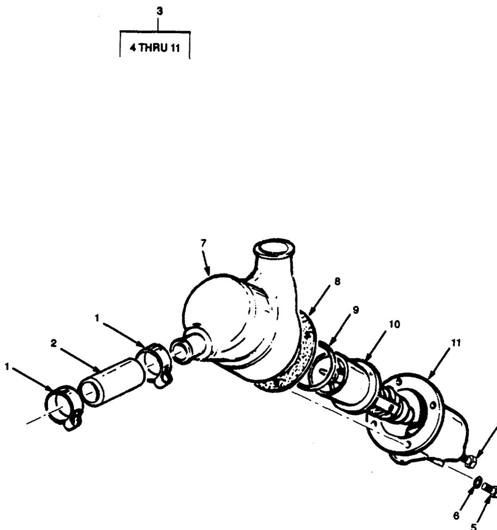
Figure 36. Thermostat Assembly.
