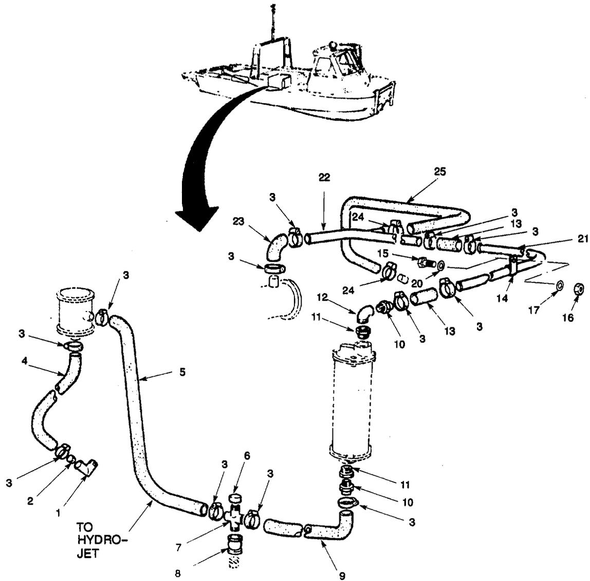
Figure 32. Raw Water (Sheet 1 of 3).
