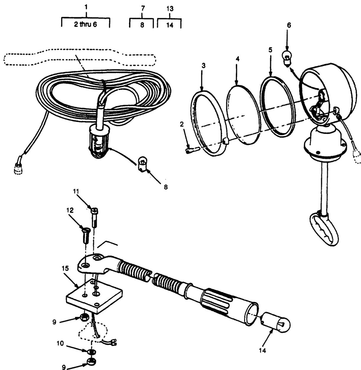
Figure 46. Searchlight, Inspection and Map Reading Lights.
