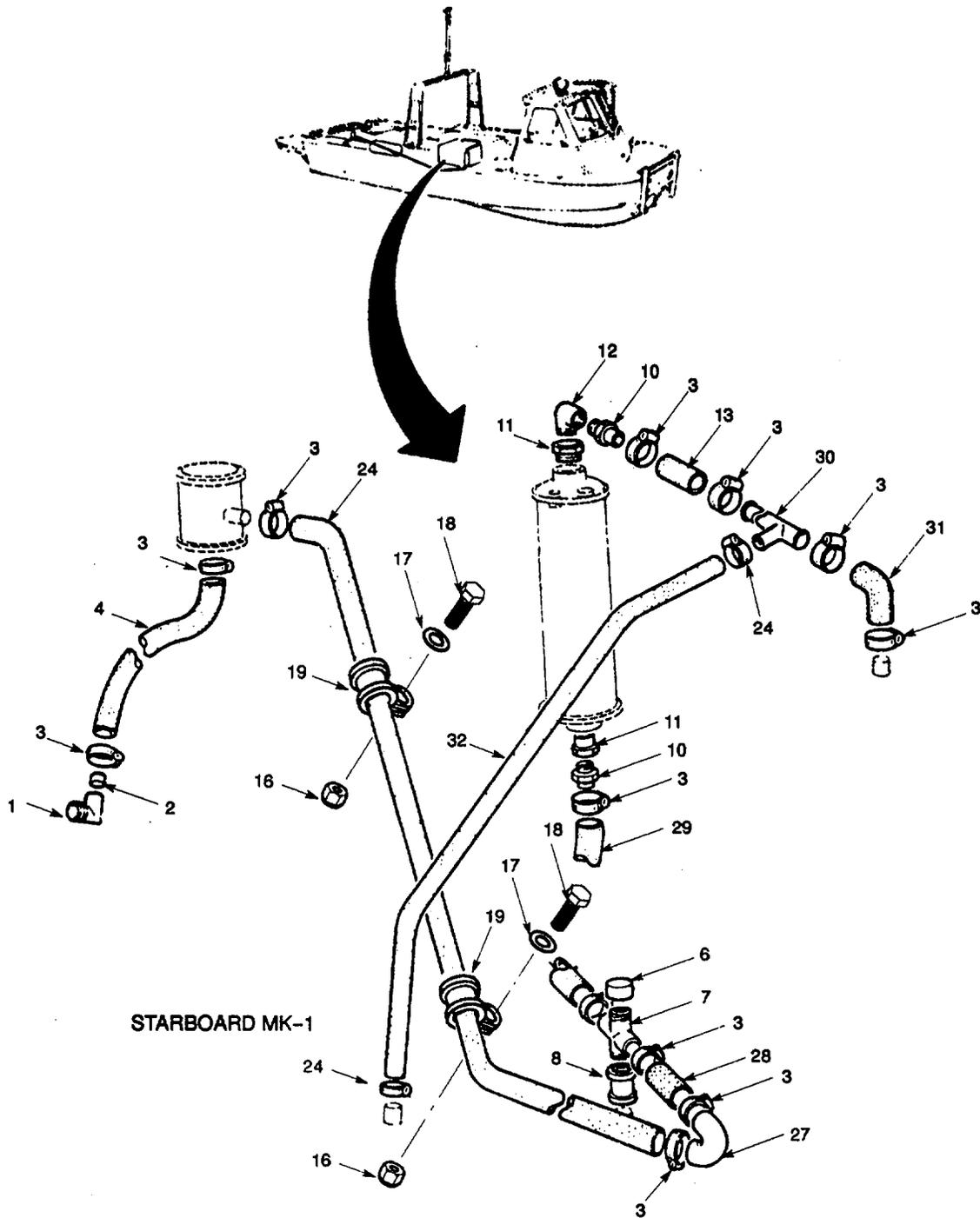
Figure 32. Raw Water (Sheet 2 of 3).
