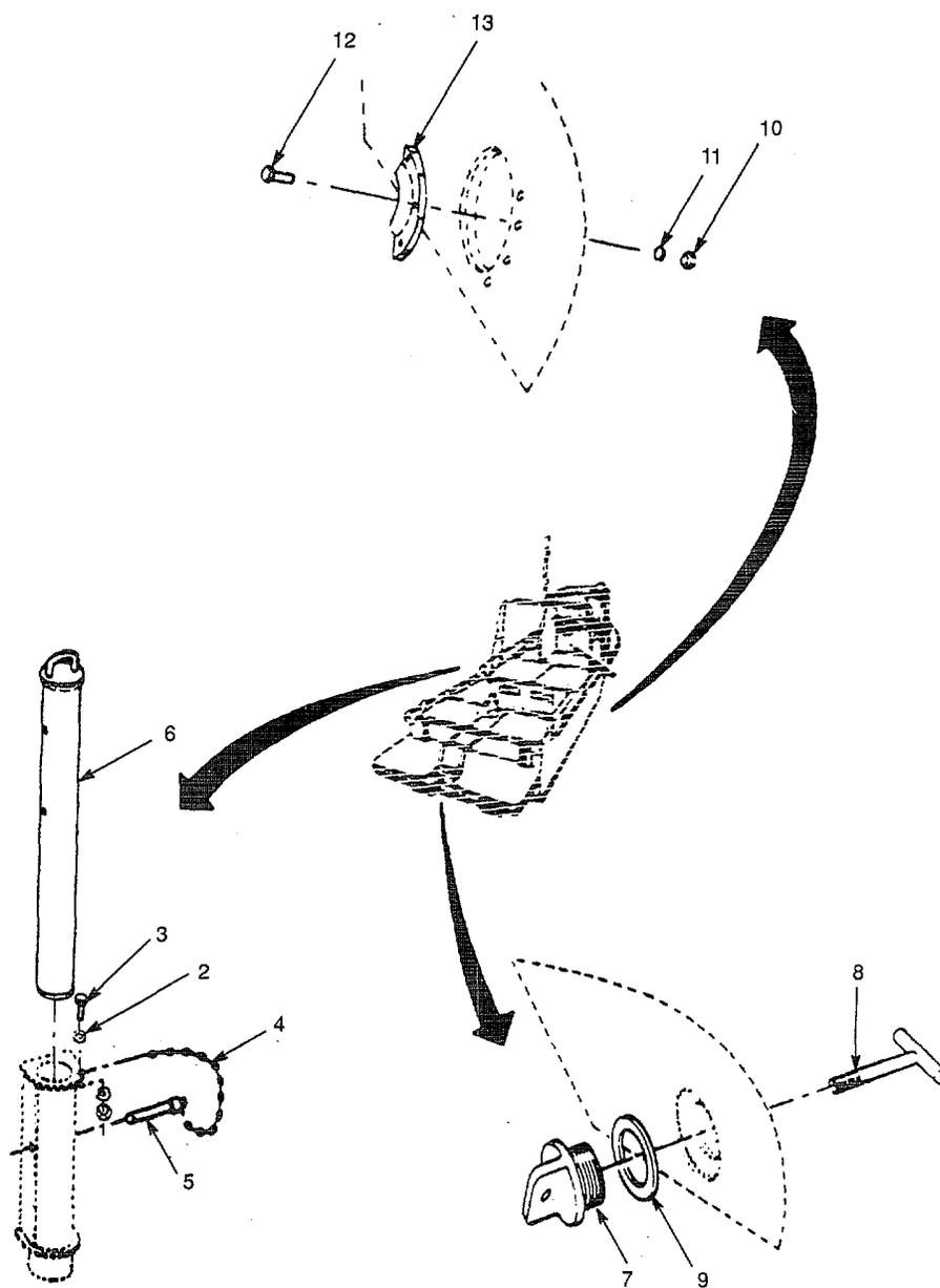
Figure 83. Beaching Legs and Bilge Drain Plug.
