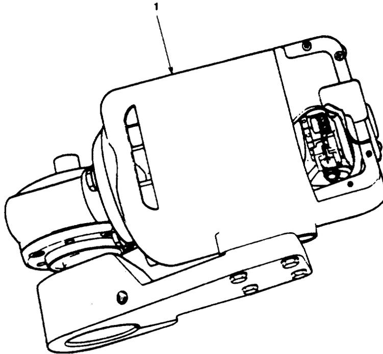
Figure 4. Windshield Wiper Motor.
