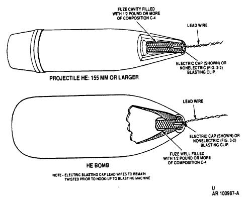
Figure 2-3. Priming large caliber conventional HE projectiles and large HE bombs
