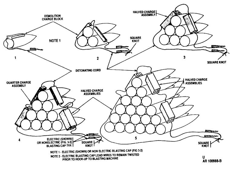
Figure 3-1. Placement of demolition charges on 1 to 21 rounds.
