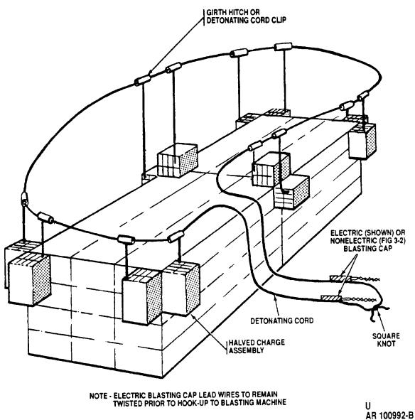
Figure 3-5. Typical placement of demolition charges on large quantities of boxed ammunition for 40mm and 105mm cartridges, hand grenades, and mines.
