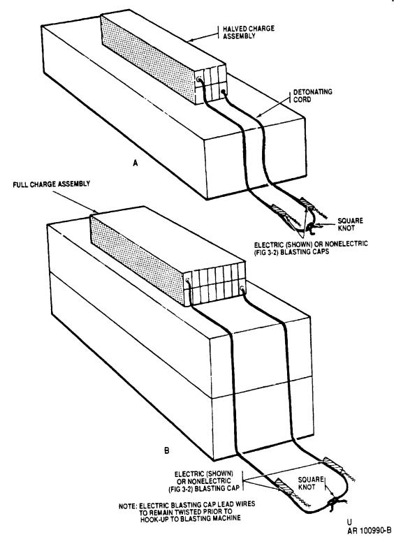
Figure 3-3. Typical placement of demolition charge assemblies on packed ammunition (A one box; B two, three or four boxes) for 40mm and 105mm cartridges, hand grenades, and mines.
