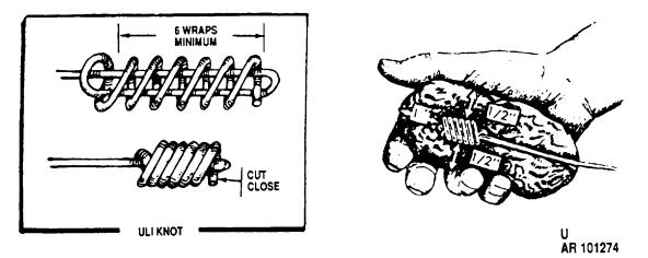
Figure 2-5. Detonating cord priming of plastic explosive.
