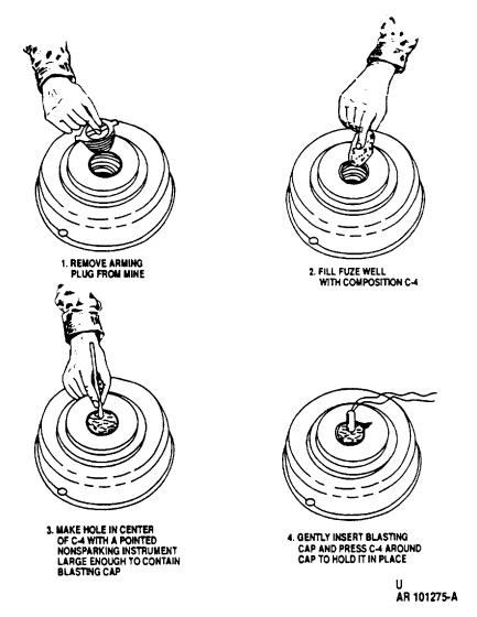
Figure 2-4. Fuzing mine M15 with blasting caps in primary fuzewell.
