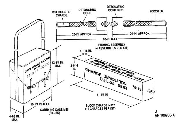
Figure 2-1. Demolition charge assembly M183.
