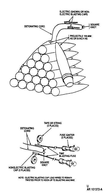
Figure 3-2. Placement of Large caliber conventional HE projectiles and large HE bombs on 1 to 21 rounds.
