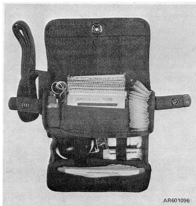
Figure 1. ABC-M18A2 chemical detector
