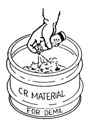
*b*. To prevent splashing, place towels or cloth in bottom of drum. Unlock actuator, invert the disperser, and discharge the remaining pressure into drum.
