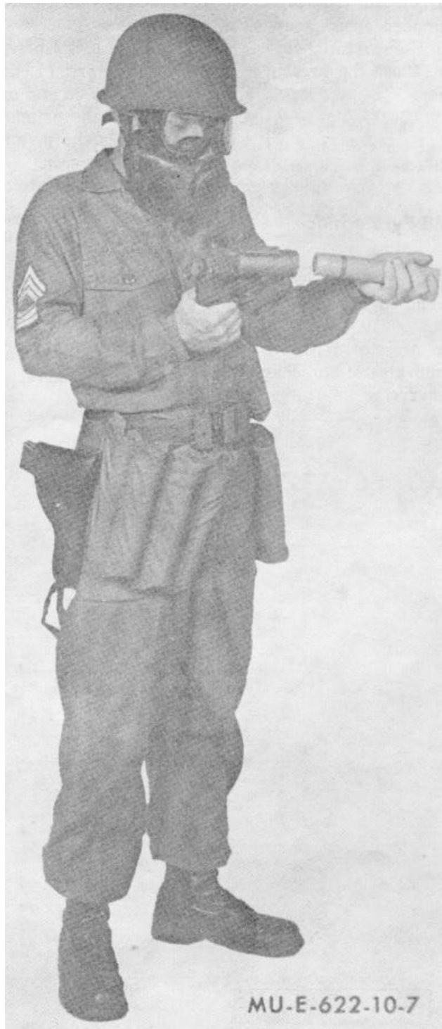
Figure 7. Loading cartridge into AN-M8 pyrotechnic pistol (typical).
