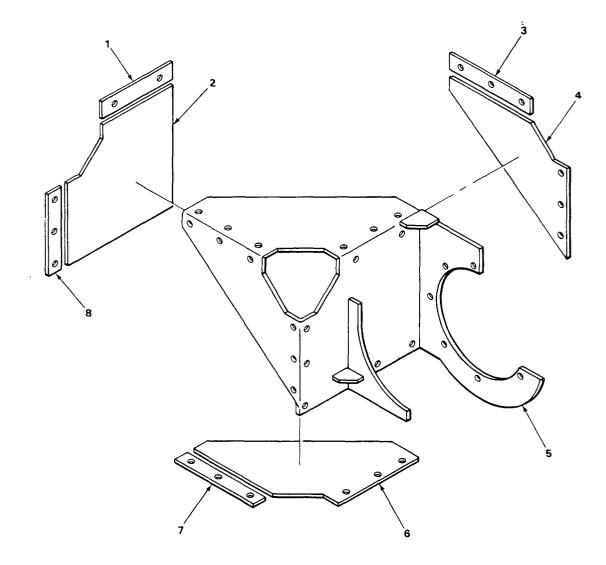
Figure 4. Bracket Assembly, Cradle.
