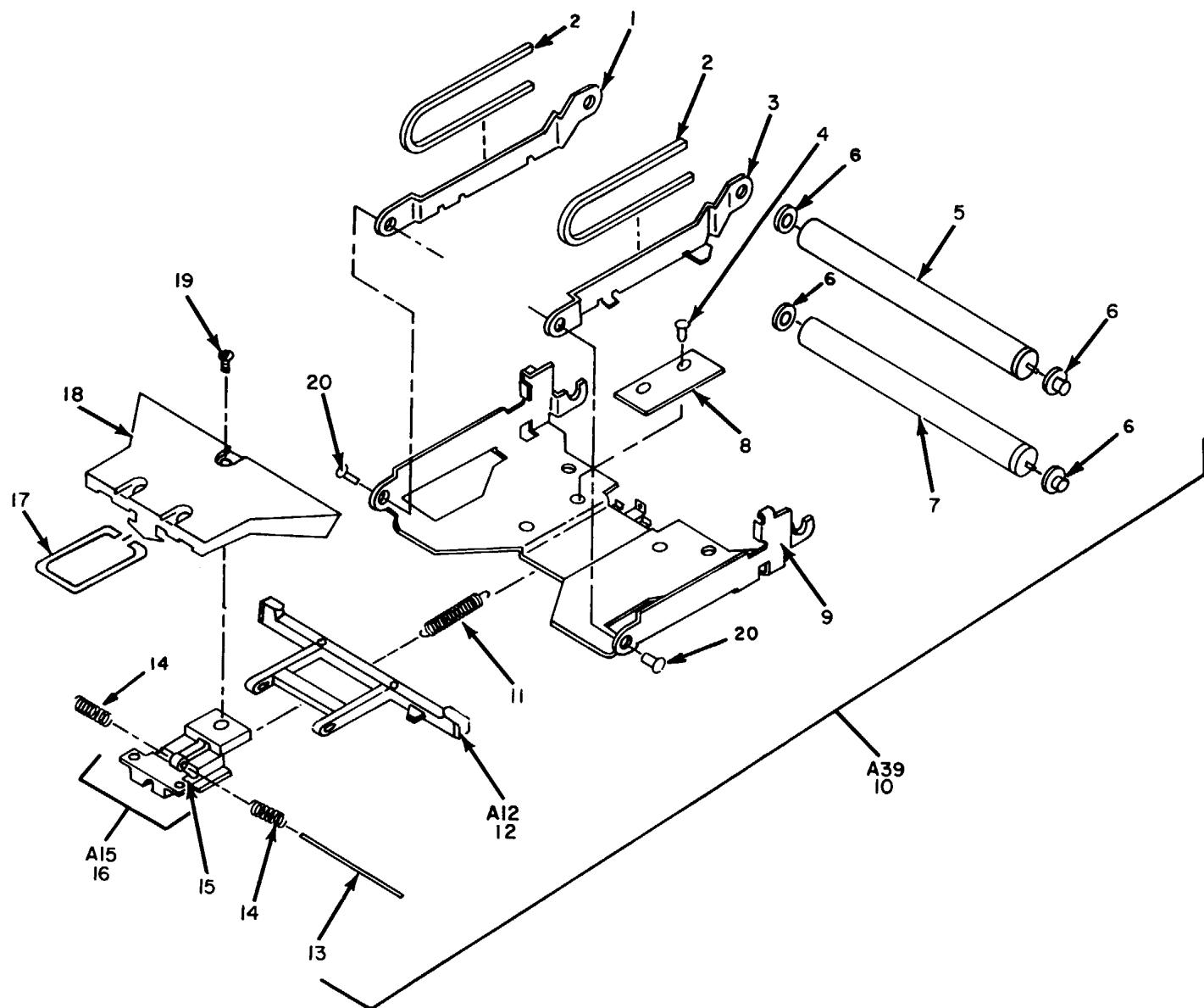
Figure 9. Door Assembly, Frame Roller Support Assembly.
