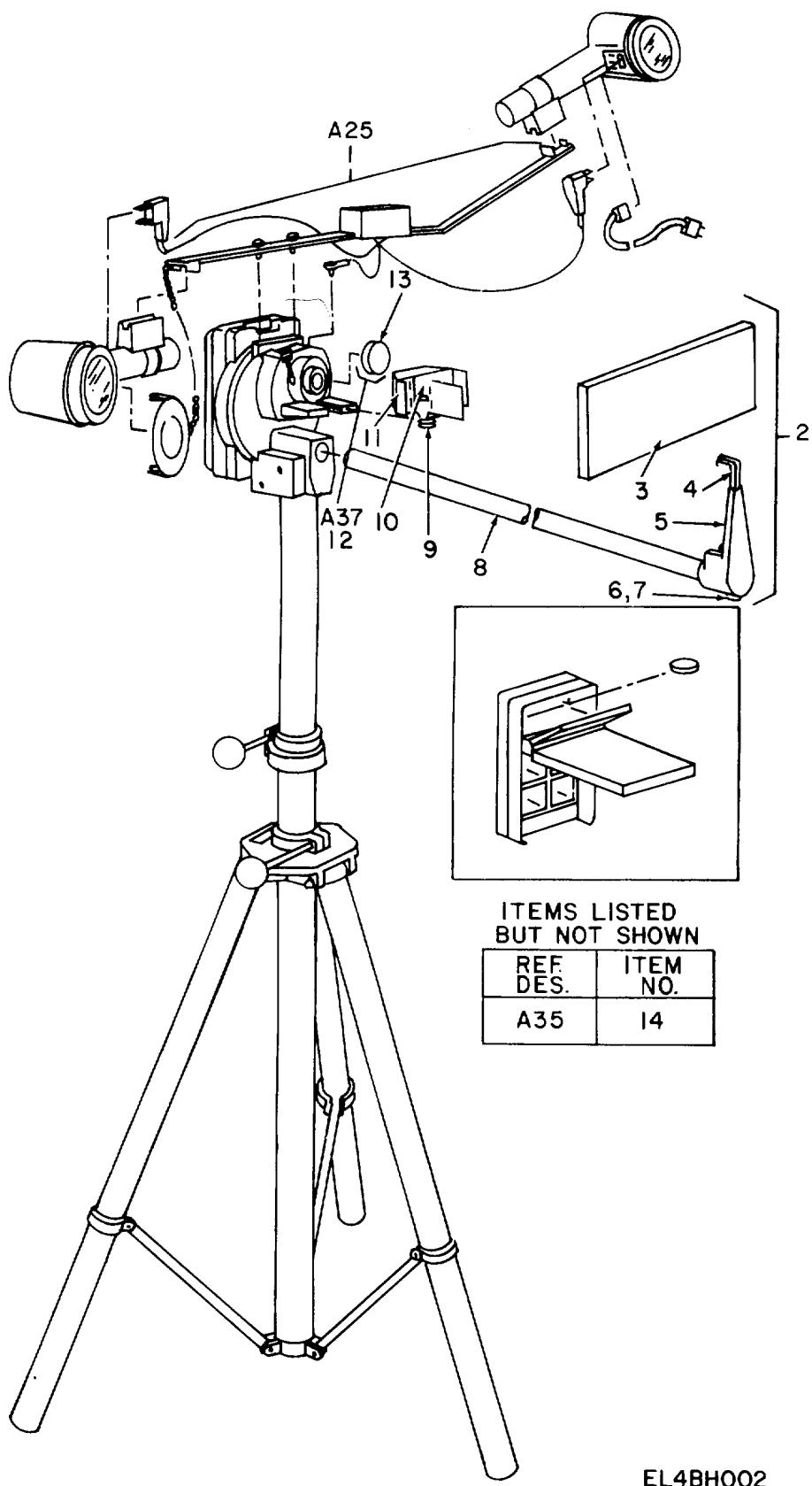
Figure 2. Camera Sets, Still Picture KS-19A4 and KS-19B, Assembled View.
