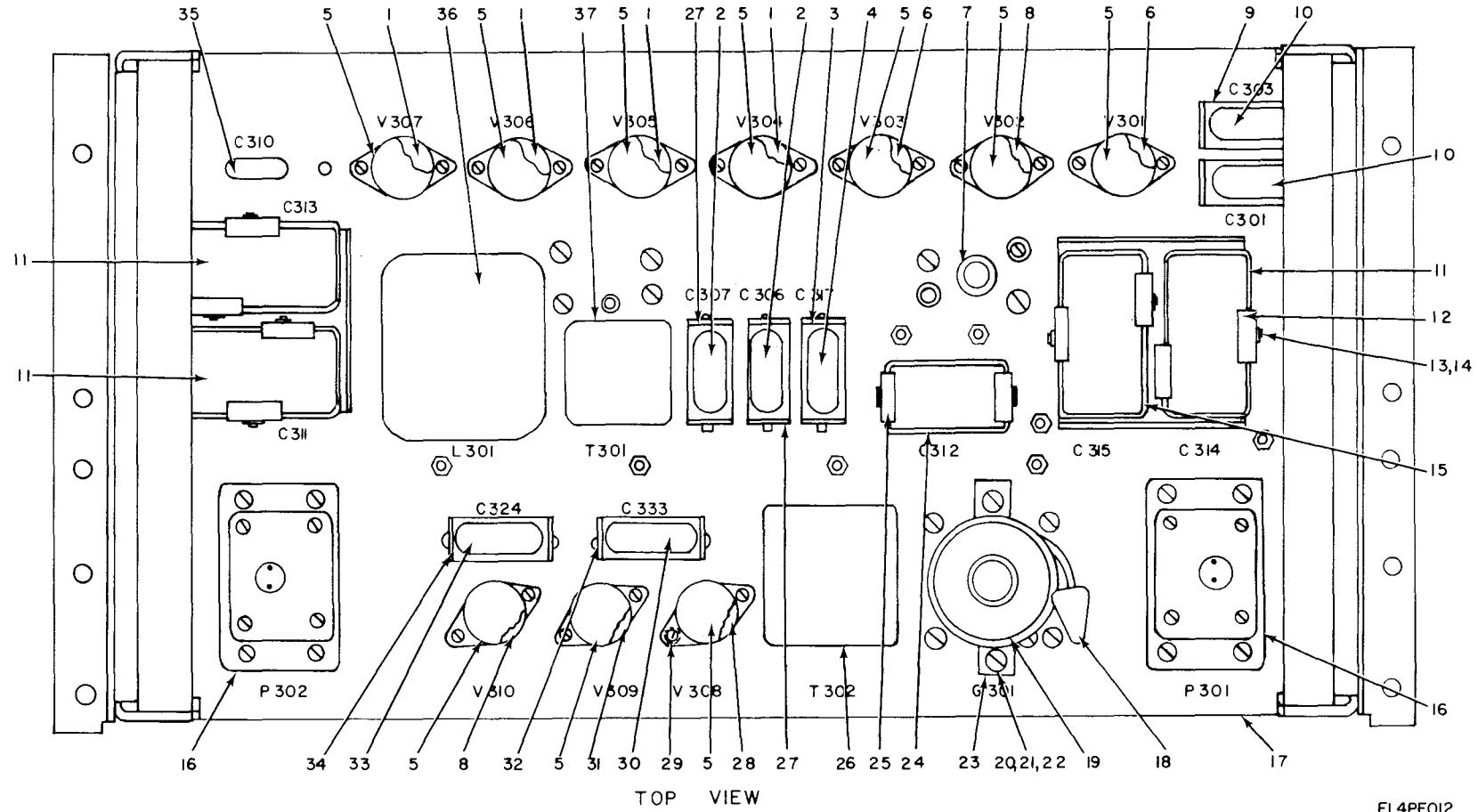
Figure 9. Converter, Signal Data CV-146A/TMQ-5 (Sheet 1 of 3).
