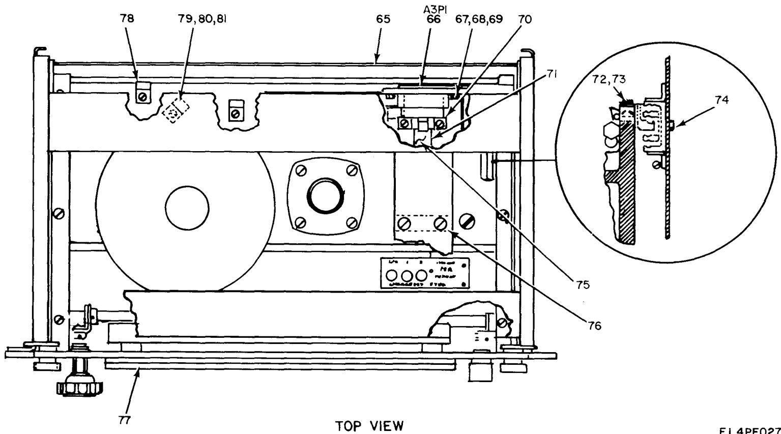
Figure 19. Recorder, Frequency Time RD-88C/TMQ-5 (Sheet 2 of 2).
