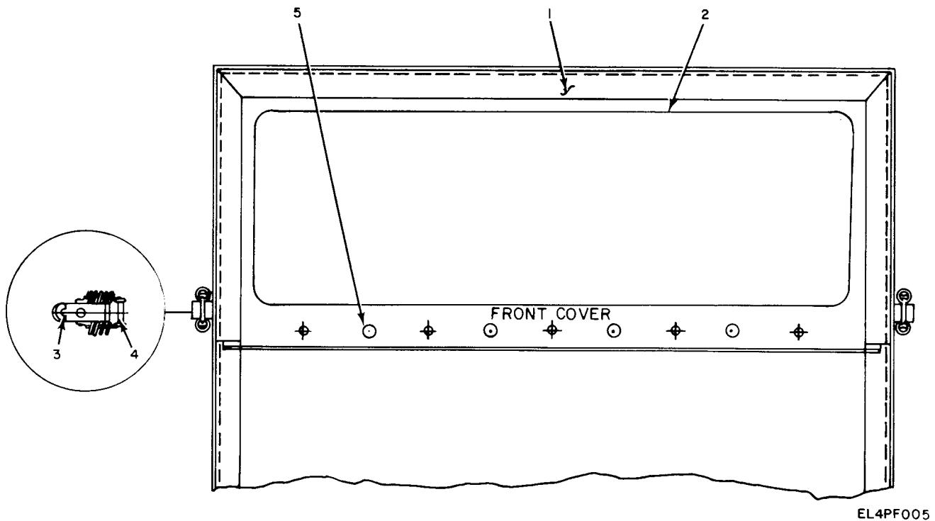
Figure 4. Cabinet, Electrical Equipment CY-1390A/TMQ-5, Front Cover Assembly.
