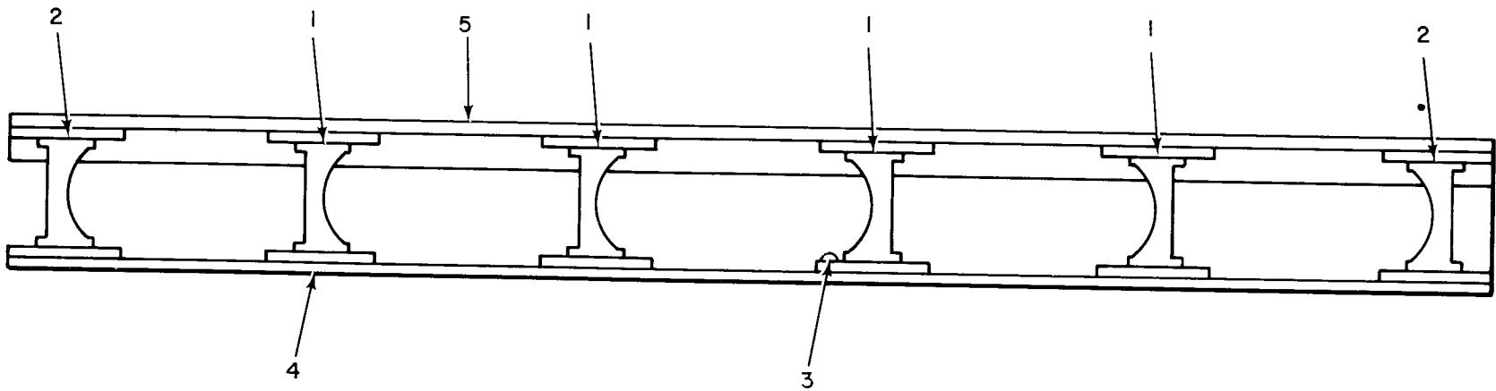
Figure 5. Cabinet, Electrical Equipment CY-1390A/TMQ-5, Vibration Mount Assemblies SCC125706GRPI
