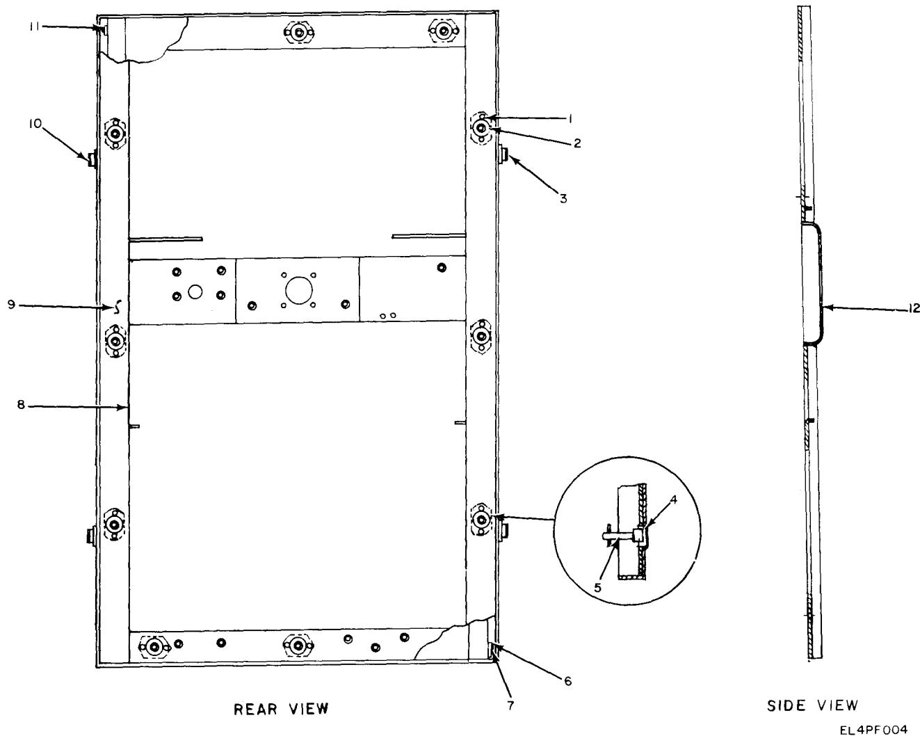
Figure 3. Cabinet, Electrical Equipment CY-1390A/TMQ-5, Rear Cover and Frame Assemblies.
