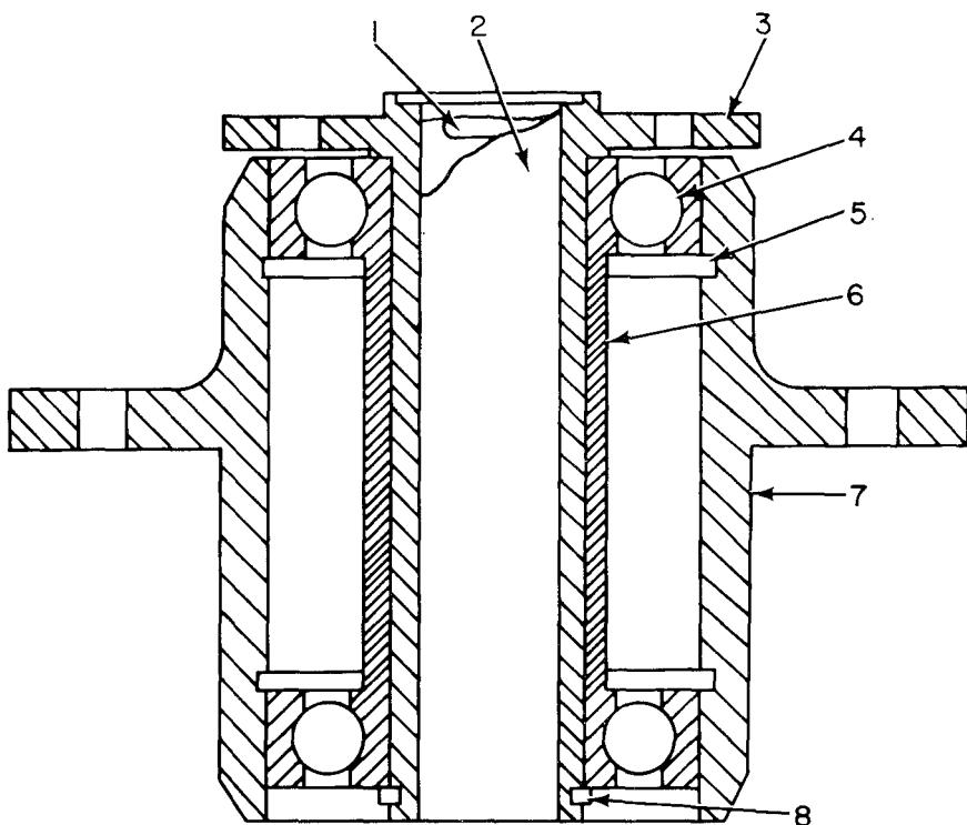
Figure 24. Recorder, Frequency Time RD-88C/TMQ-5, Hub Assembly.
