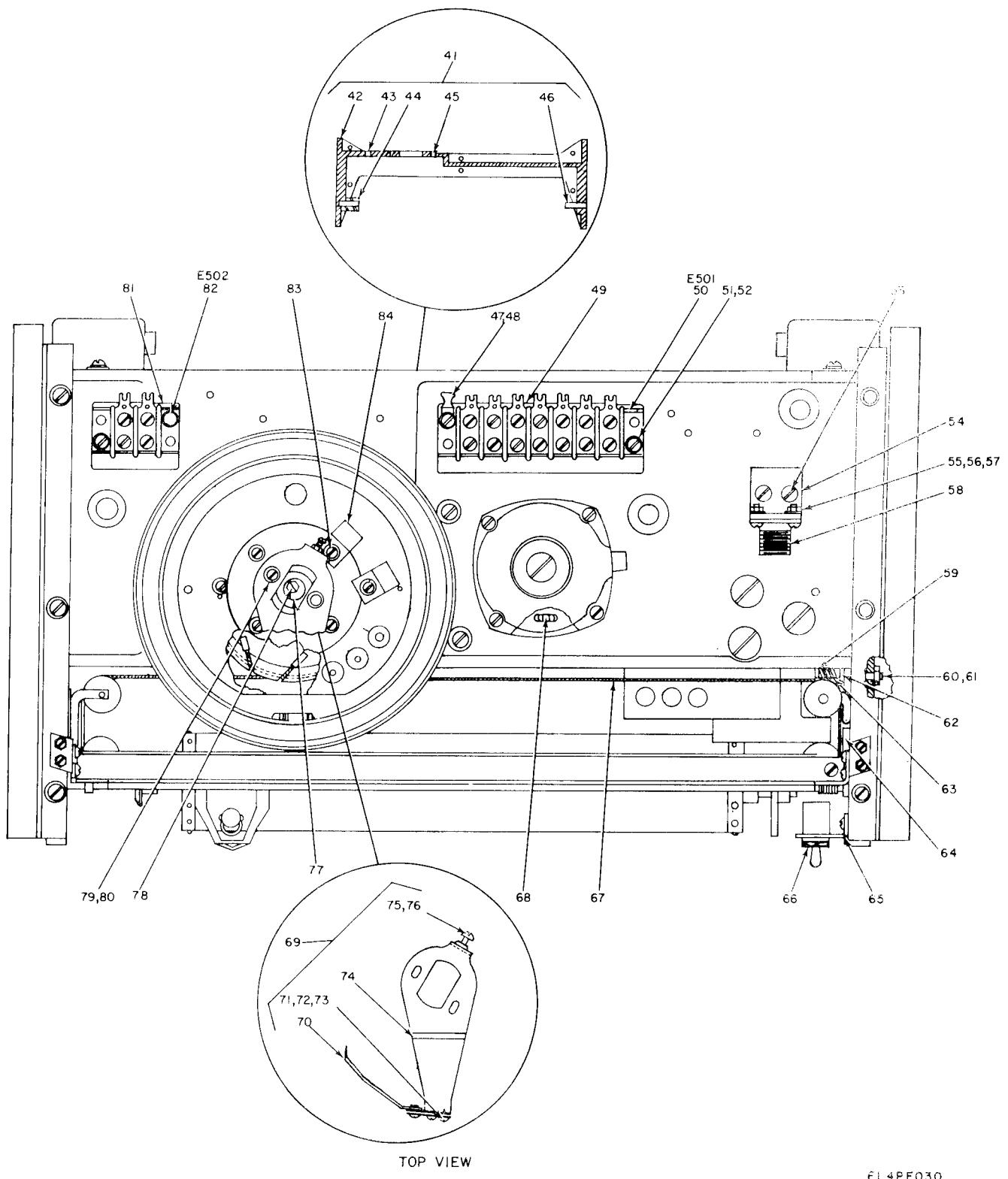
Figure 21. Recorder, Frequency Time RD-88C/TM0-5, Frame Assembly, Front and Top Views (Sheet 2 of 2).
