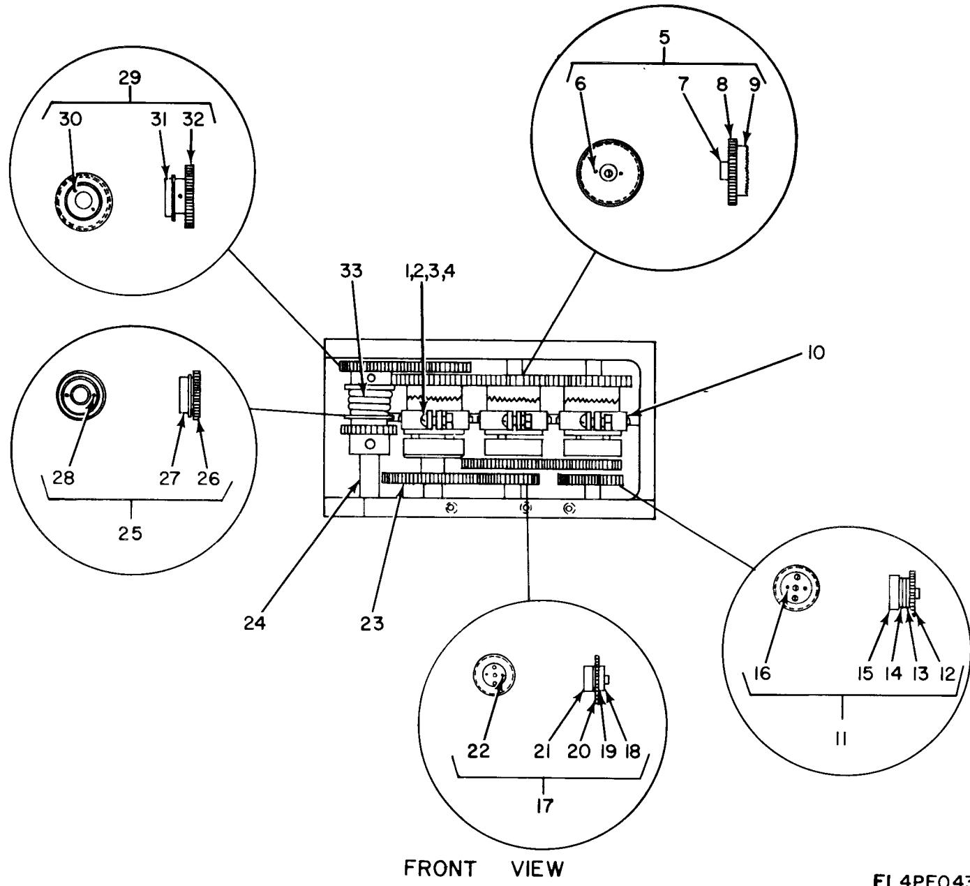
Figure 33. Recorder, Frequency Time RD-88C/TMQ-5, Housing Assembly (Sheet 1 of 2).
