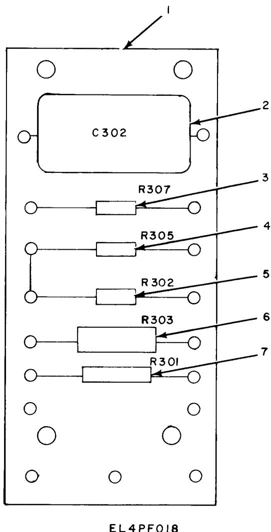
Figure 13. Converter, Signal Data CV-146A/TMQ-5, Terminal Board Assembly E318.
