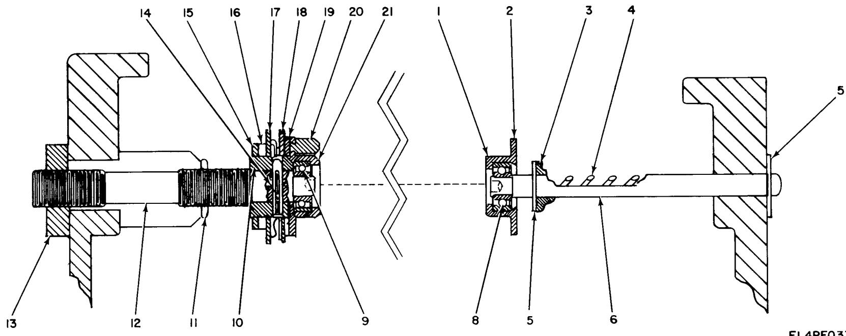
Figure 23. Recorder, Frequency Time RD-88C/TMQ-5, Shaft Assembly.
