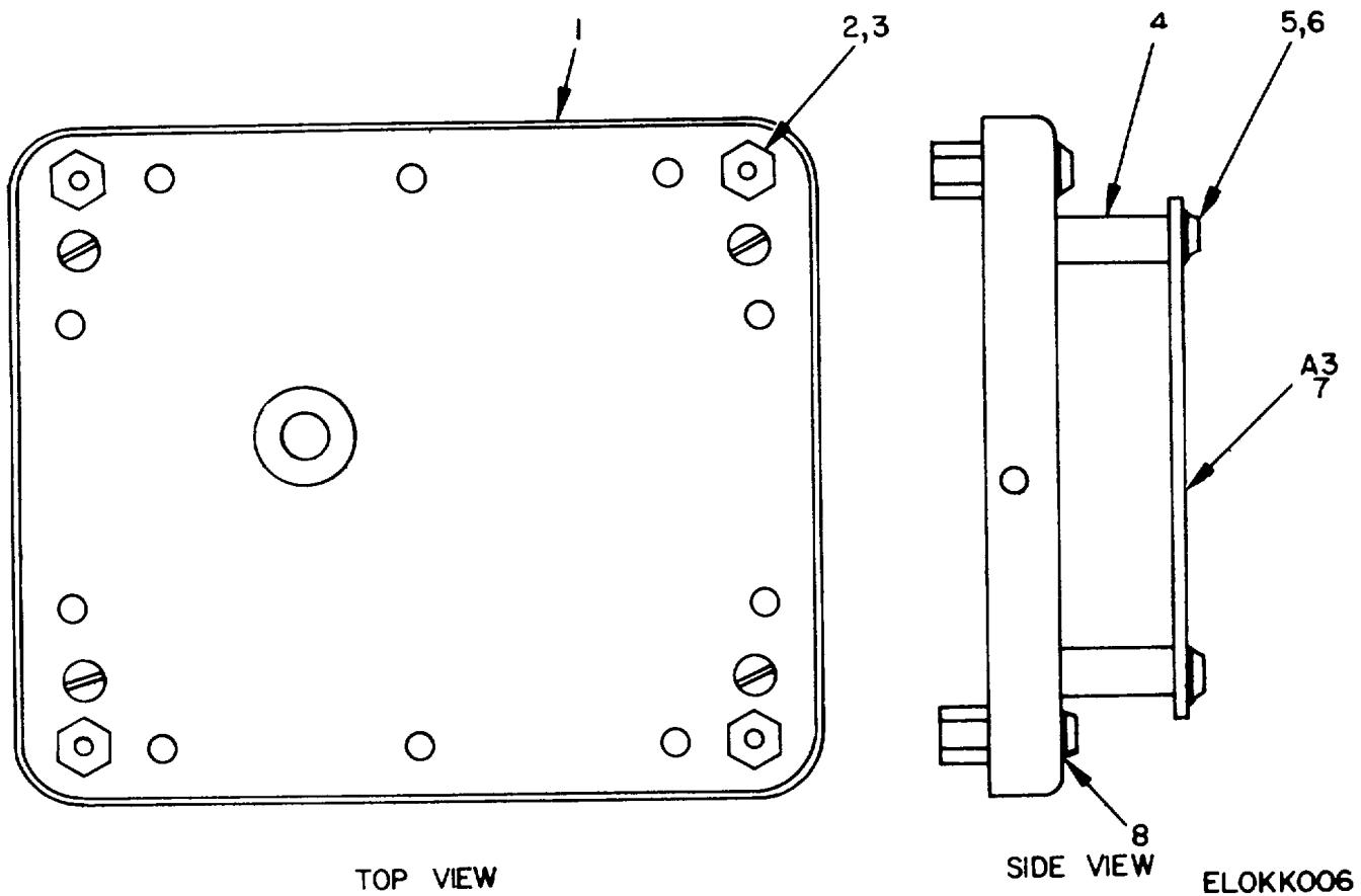
Figure 5. Shield Assembly: VFO.
