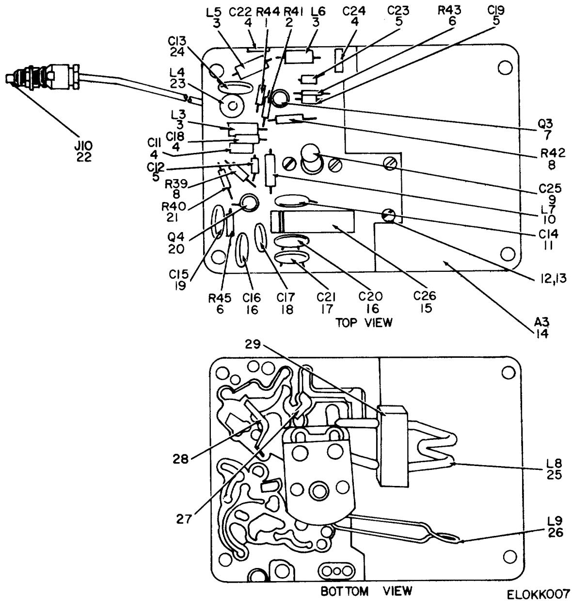
Figure 6. Board Assembly: VFO.
