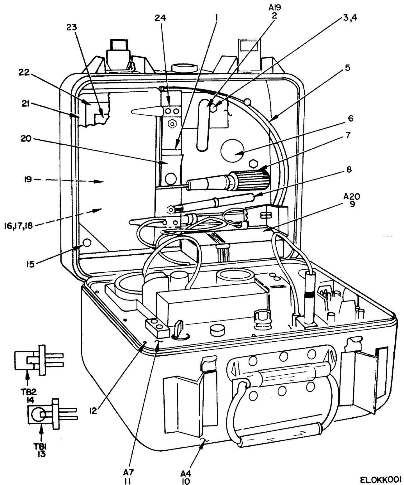
*Figure 1. Indicators, Channel Alignment ID-1189/PR and ID-1189(XE-2)/PR.*
