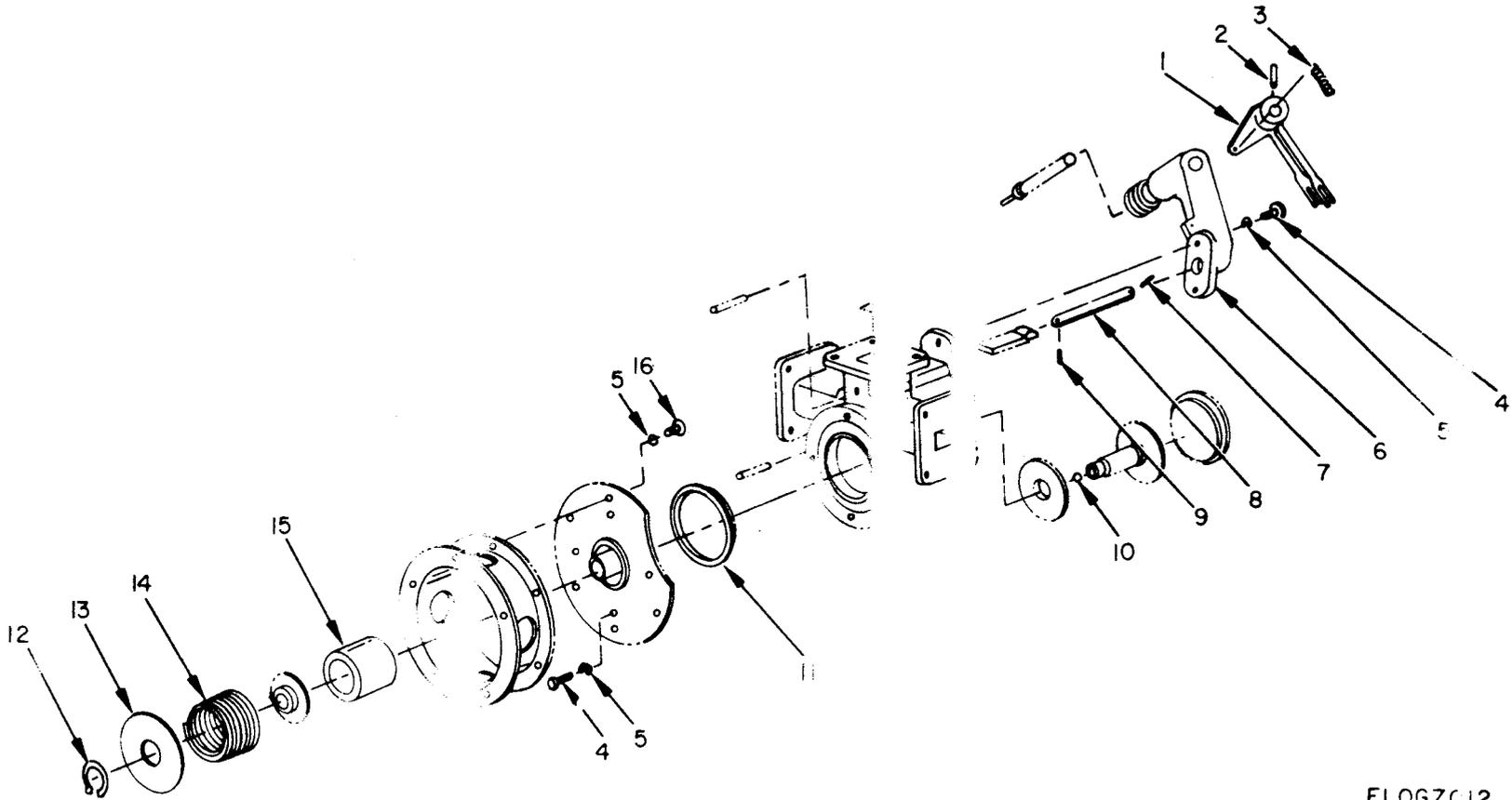
Figure 12. Tee Assembly, Frequency Meter, Exploded View.
