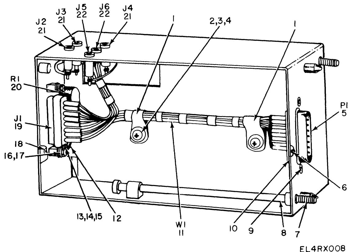
Figure 7. Extender Module MX-4894/URC (1A5).
