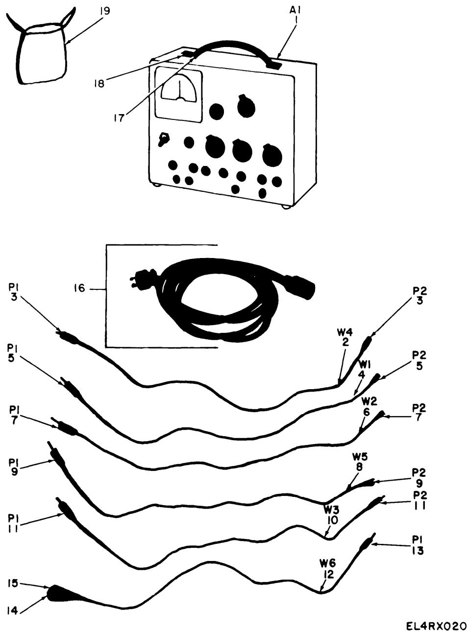
Figure 19. Test Set, Radio TS-1956/URC (1A32).
