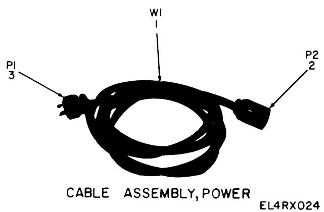
Figure 23. Cable Assembly, Power CX-9009/URC (1A32W7).
