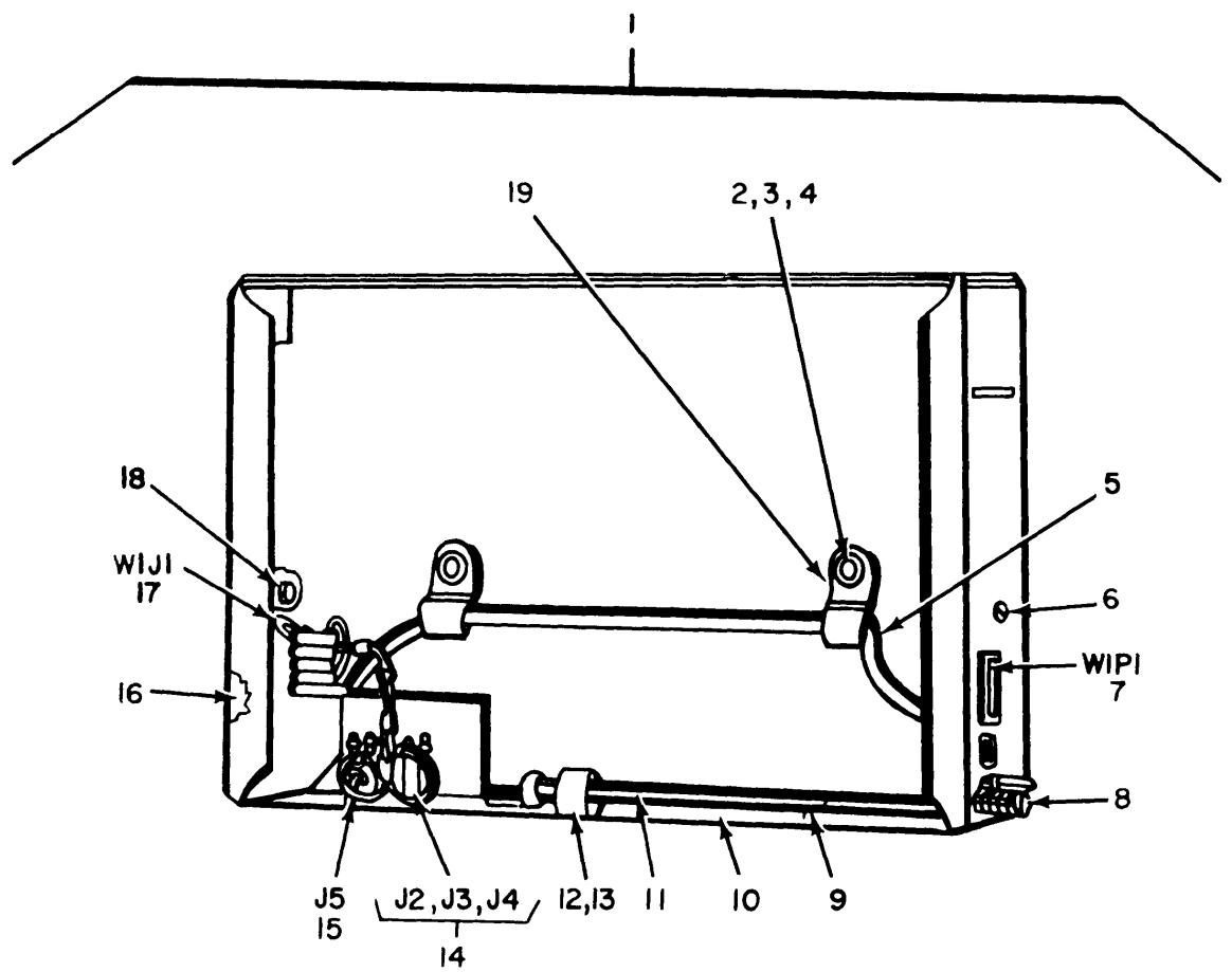
Figure 8. Extender Module MX-4893/URC (1A6) .
