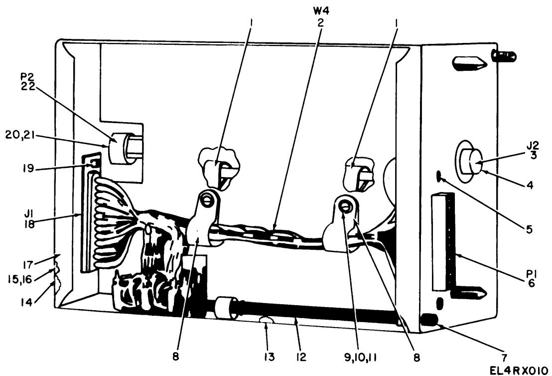
Figure 9. Extender Module MX-4891/URC (1A7).
