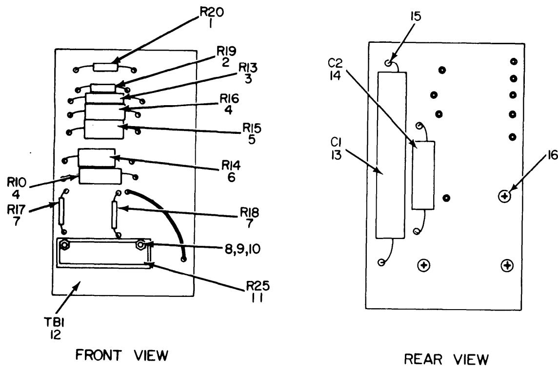
Figure 22. Test Set Subassembly (1A32A1A2).
