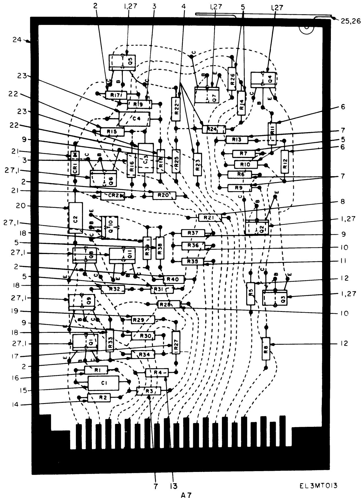
Figure 13. Test Set Subassembly A7.
