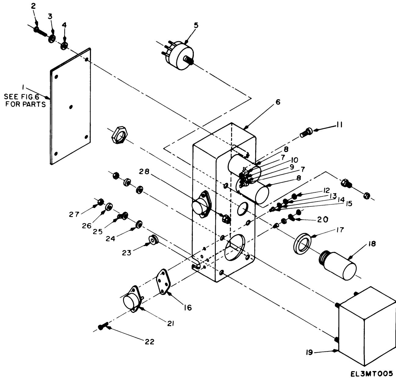
Figure 5. Power Supply Assembly.
