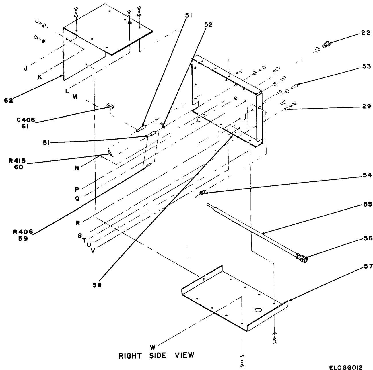
Figure 4. Generator, Signal TS-452E/U, Wavemeter (Sheet 3 of 3).
