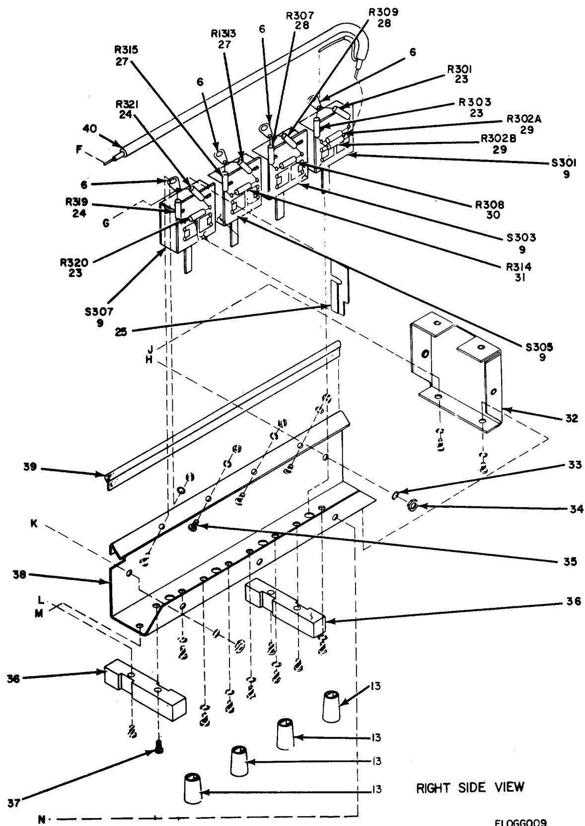
Figure 3. Generator, Signal TS-452E/U, Attenuator, Variable (Sheet 3 of 3).
