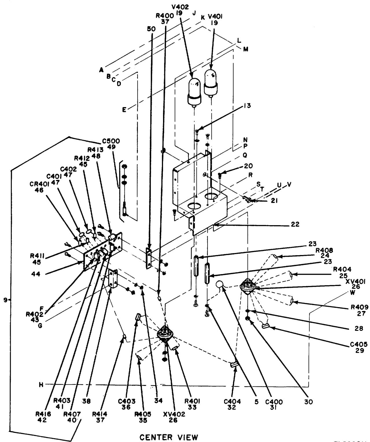
Figure 4. Generator, Signal TS-452E/U, Wavemeter (Sheet 2 of 3).
