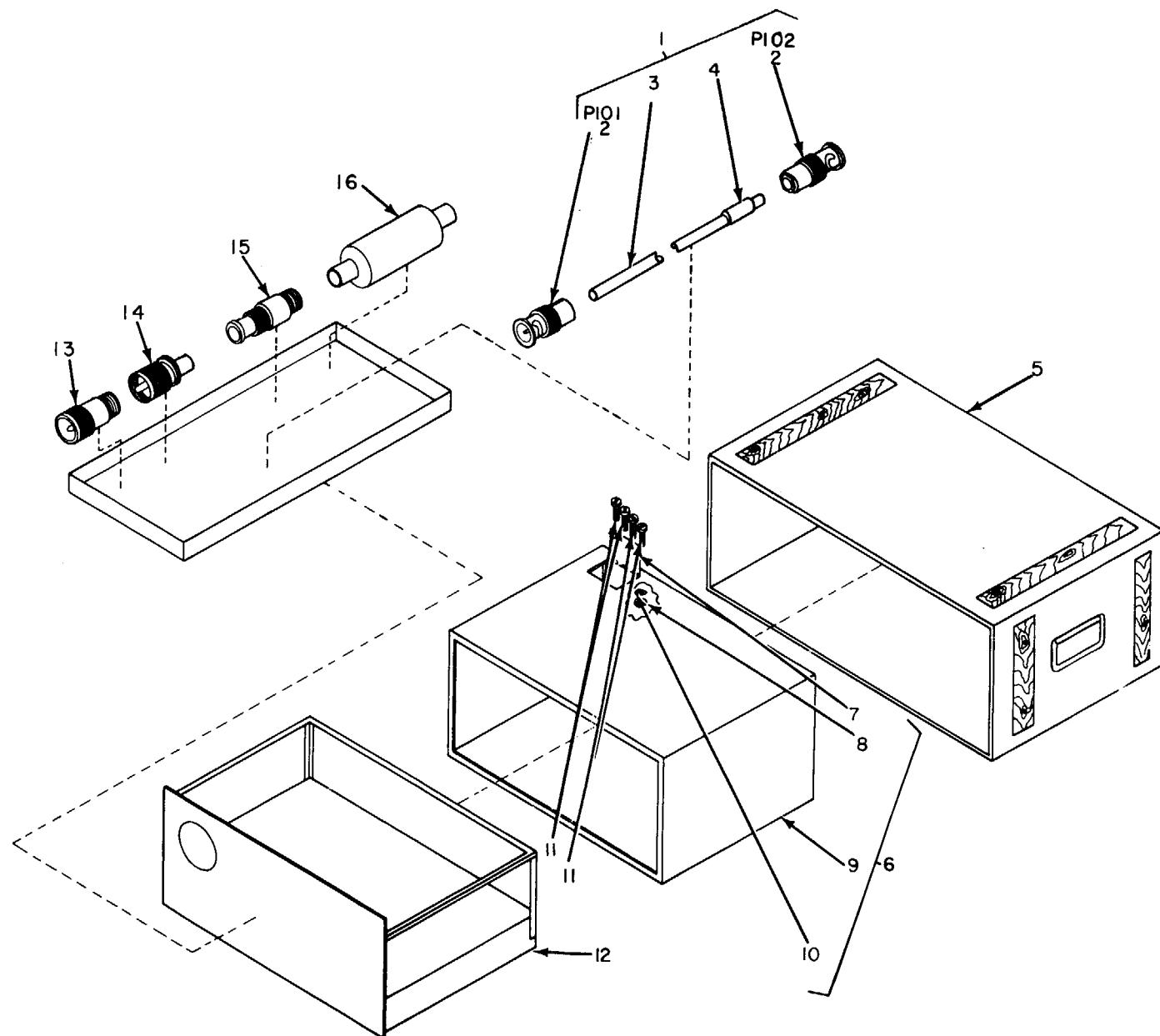
Figure 10. Generator, Signal TS-452E/U, Signal Generator Assembly.
