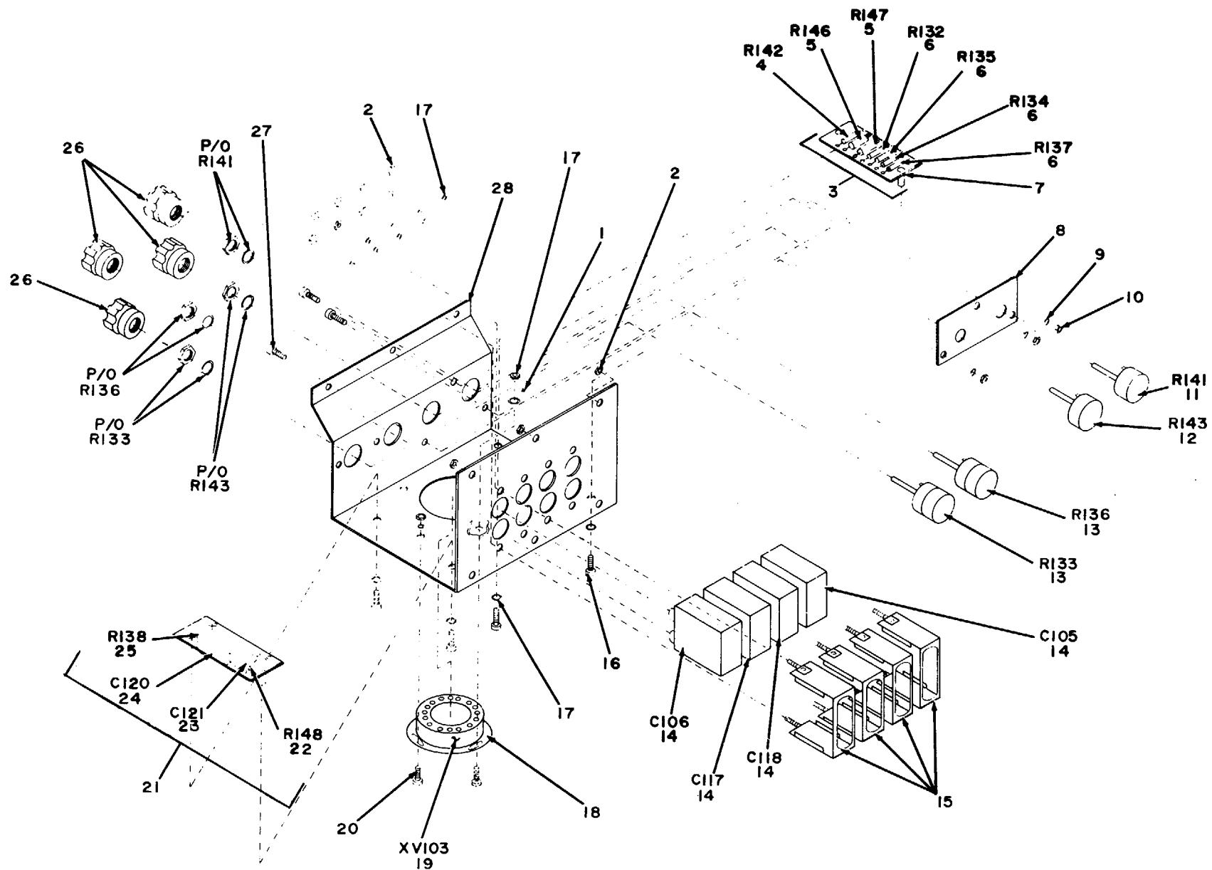
Figure 7. Generator, Signal TS-452E/U, Video Chassis Assembly.
