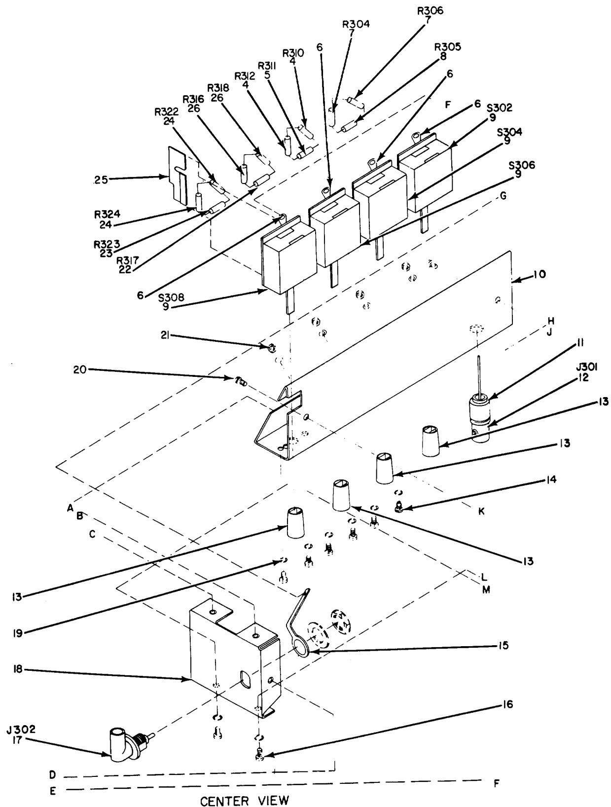
Figure 3. Generator, Signal TS-452E/U, Attenuator, Variable (Sheet 2 of 3).
