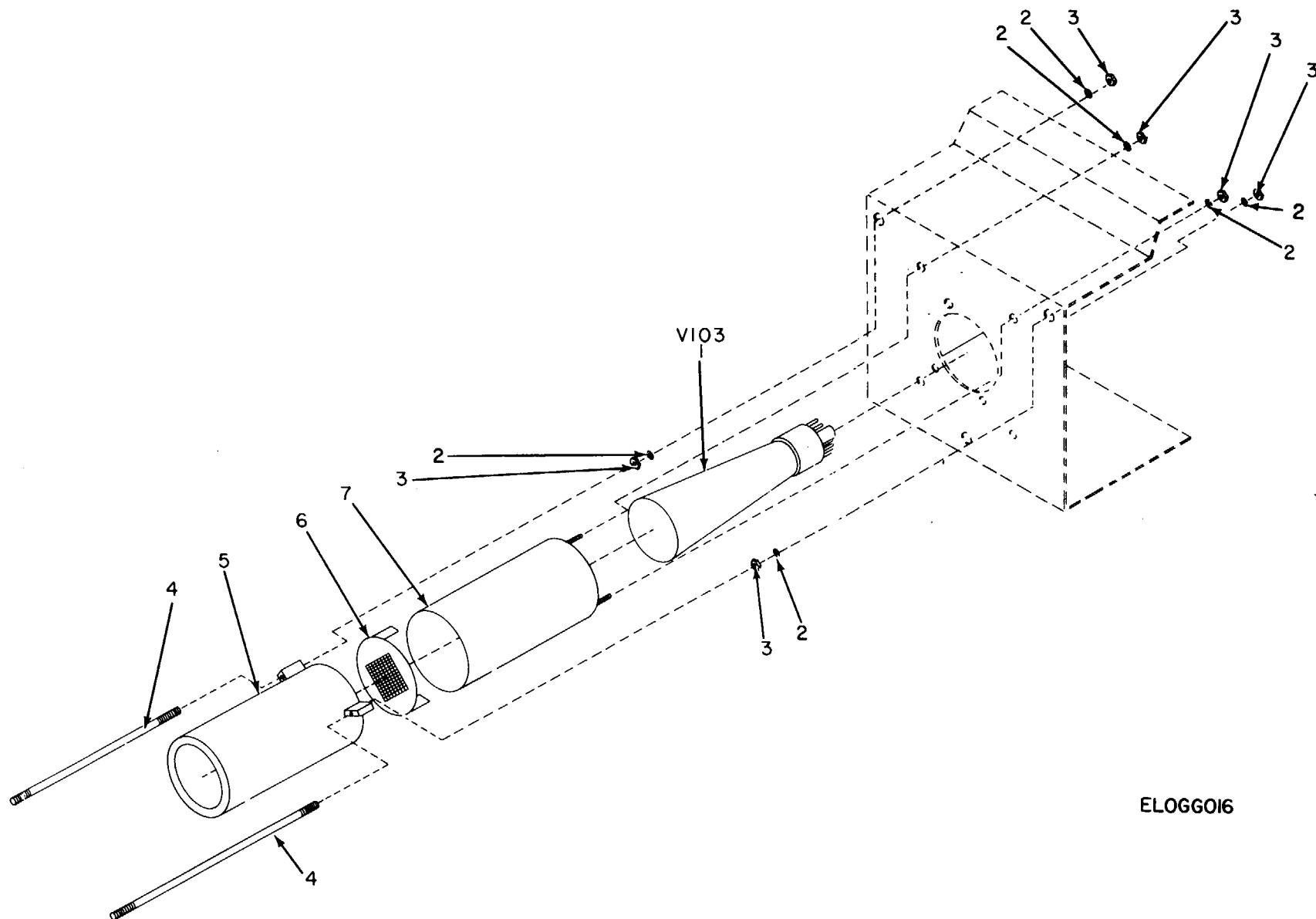
Figure 8. Generator, Signal TS-452E/U, CRT Light Shield Assembly.
