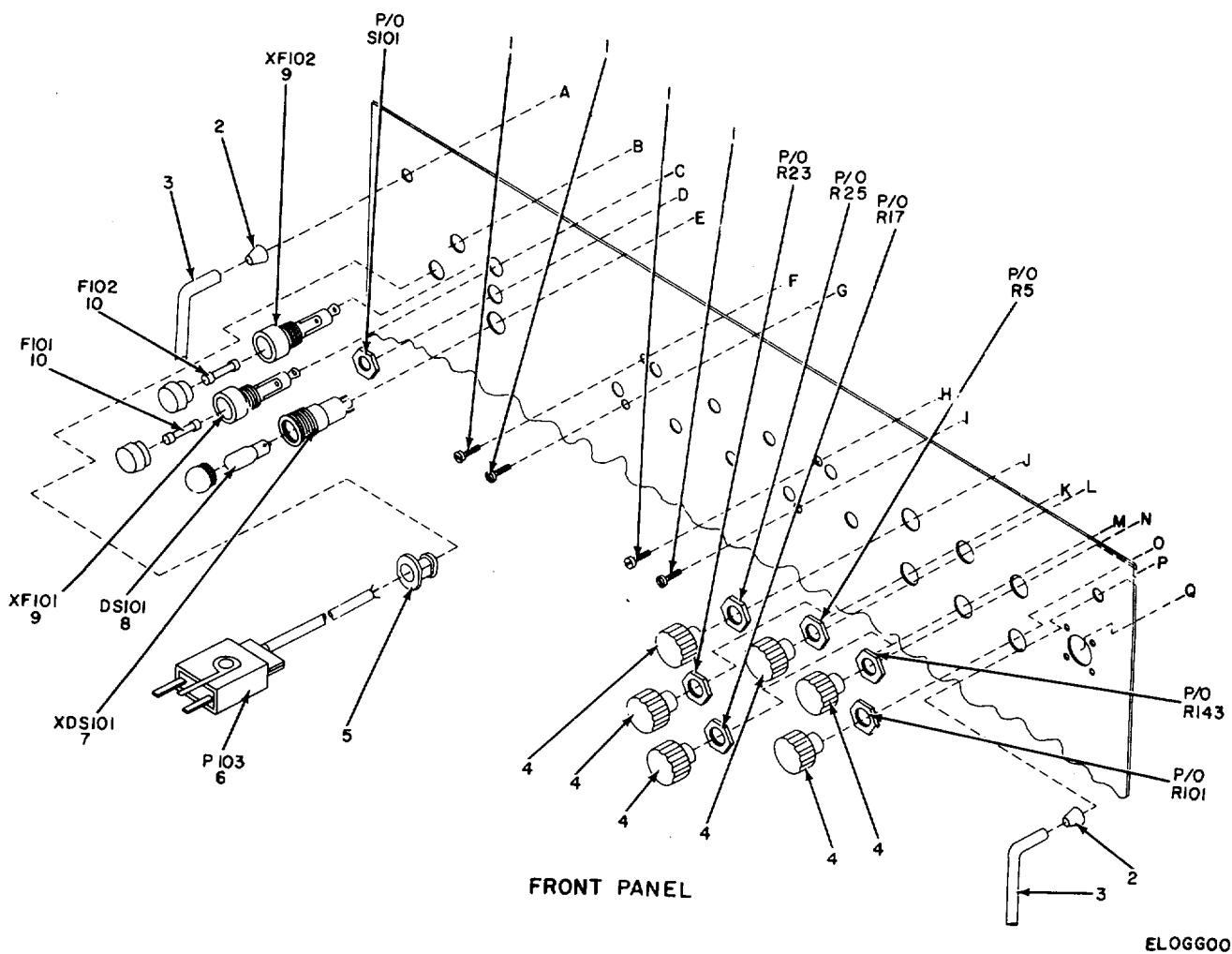
Figure 2. Generator, Signal TS-452E/U, Chassis (Sheet 1 of 3).
