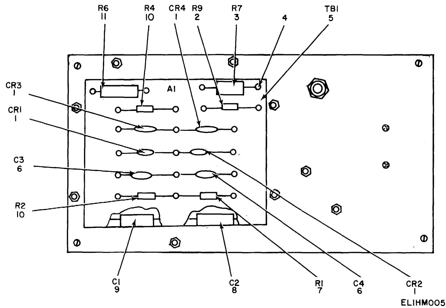
Figure 5. Circuit Card Assembly (A1A1A1).
