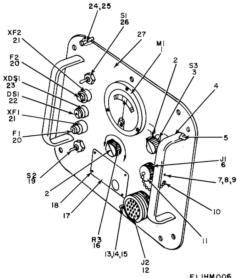
Figure 6. Panel Assembly (A1A2).
