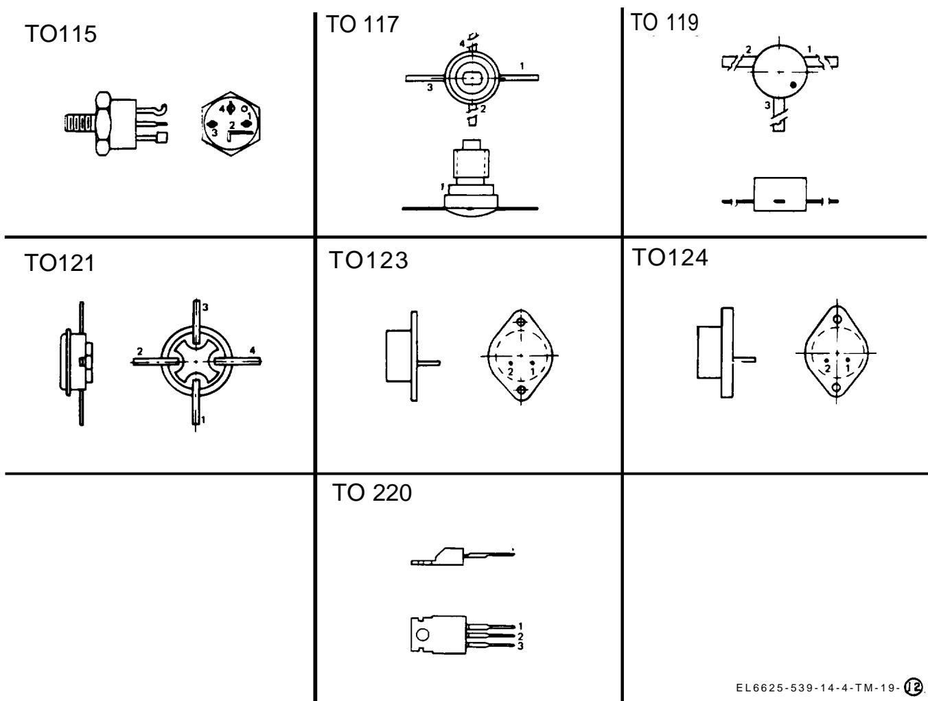
EL 6625-539-14-4-TM-19-**12**Figure D-1 **12**. Transistor outline drawings (sheet 12 of 12).
