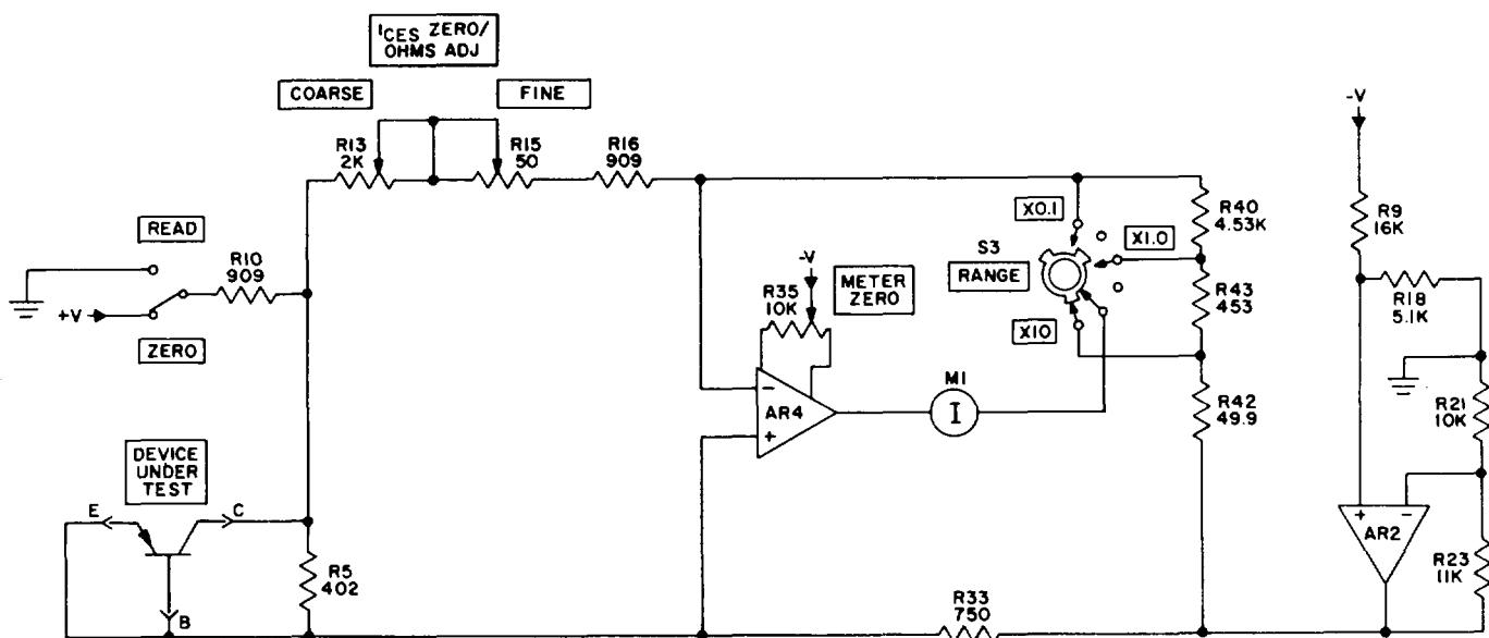
Figure 5-6.  $I_{CES}$  function test circuit, simplified schematic diagram.
