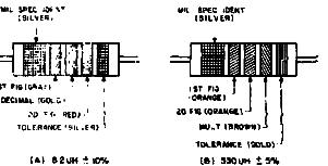
COLOR CODING FOR TUBULAR ENCAPSULATED RF CHOKES. AT A, AN EXAMPLE OF THE CODING FOR AN 82 MHZ CHOKE. AT B, THE COLOR BANDS FOR A 330 MHZ INDUCTOR ARE ILLUSTRATED.
