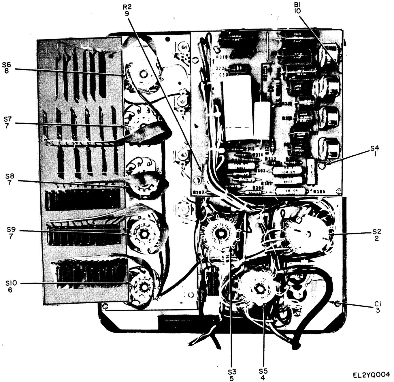
Figure 3. Voltmeter, Electronic ME-202B/U, Front Panel Rear View.
