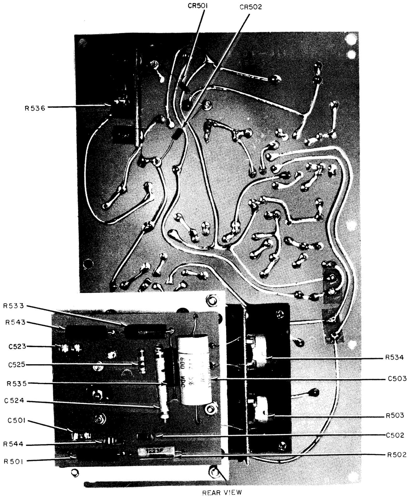
Figure 9. Voltmeter, Electronic ME-202B/U AC to DC Converter and Range Switch Assembly (Sheet 1 of 2).
