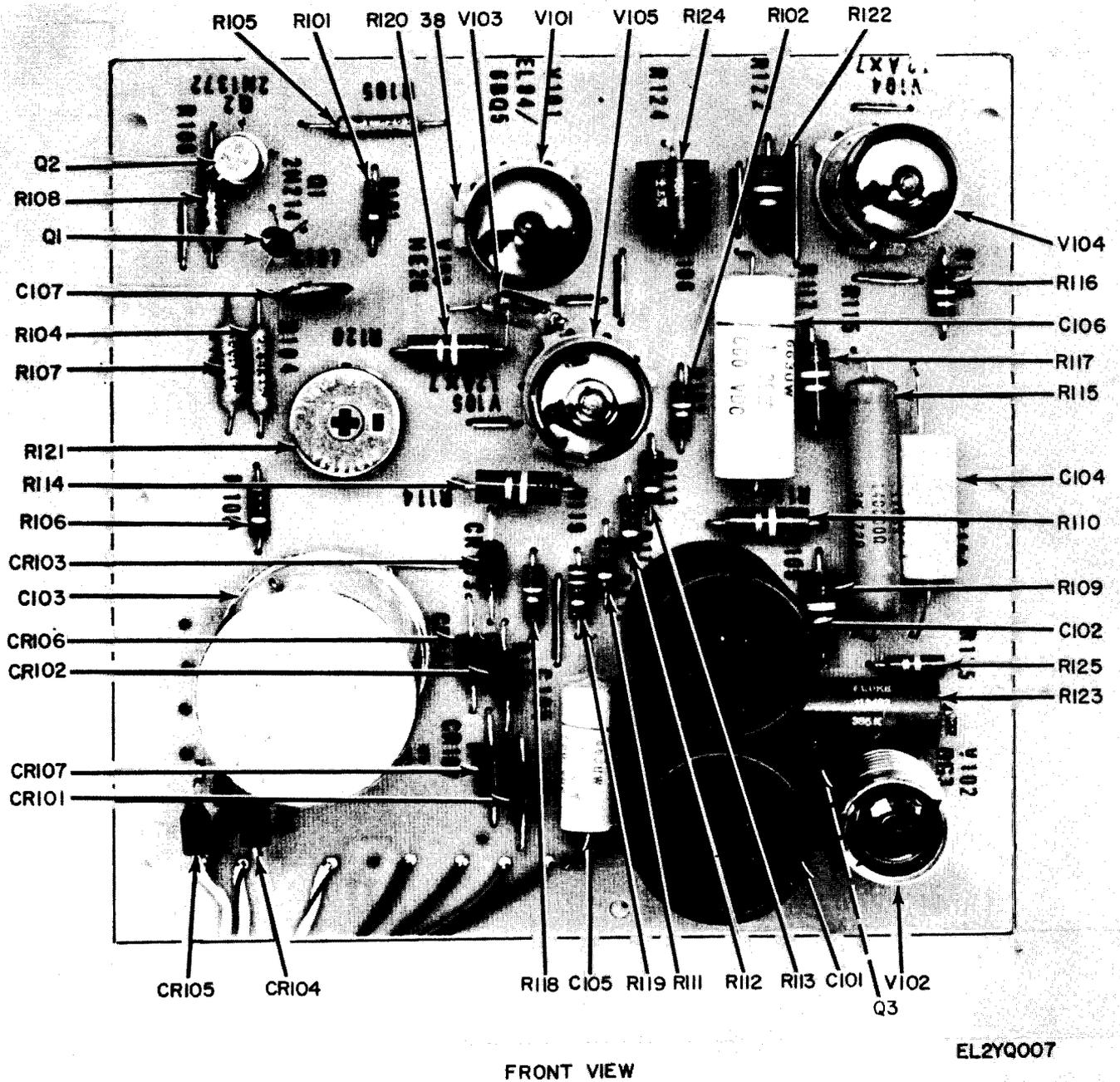
Figure 5. Voltmeter. Electronic ME.202B/U 500VDC Reference Supply Printed Circuit Board (Sheet 1 of 2).
