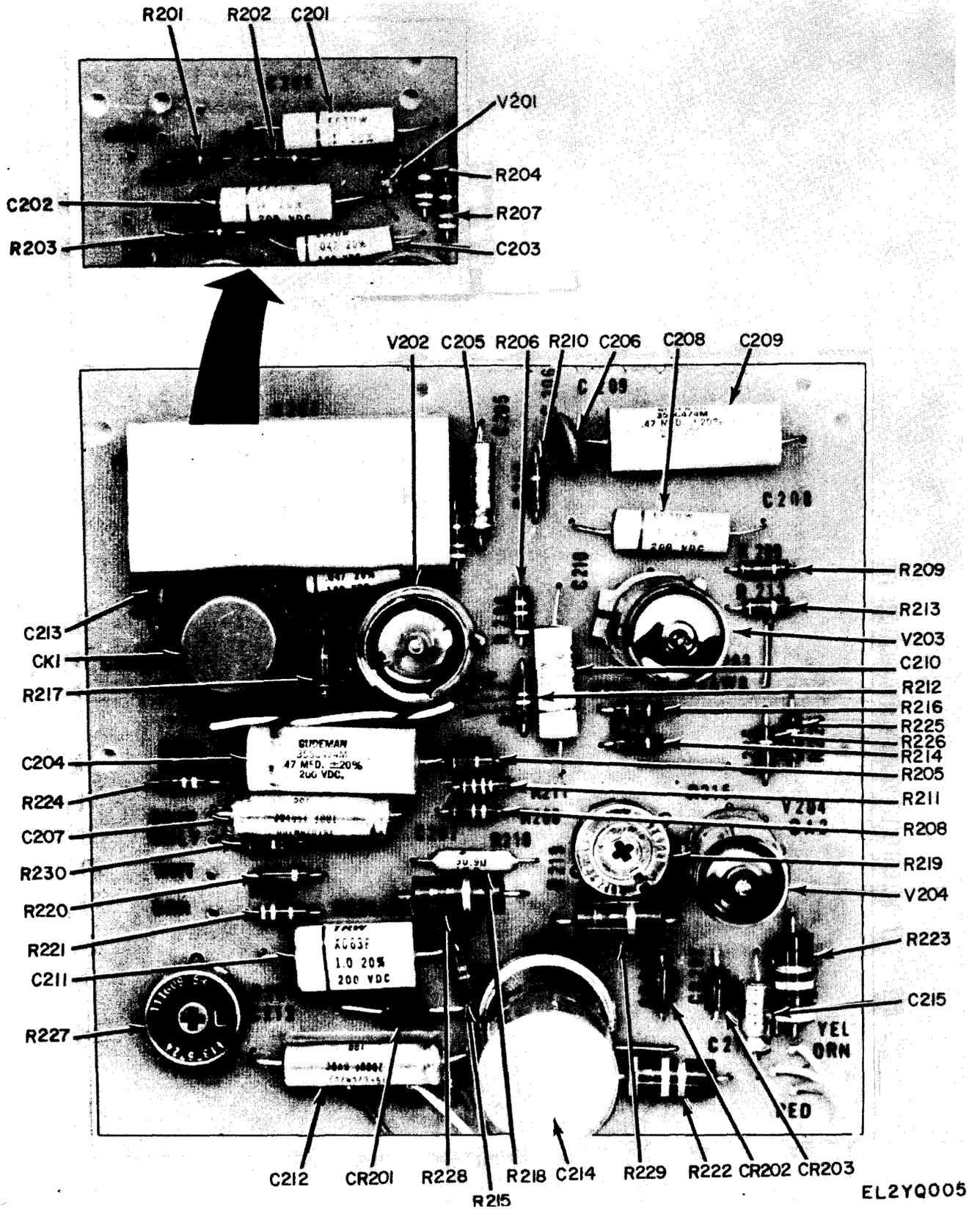
Figure 4. Voltmeter, Electronic ME-202B/U DCVTVM Printed Circuit Board (Sheet 1 of 2).
