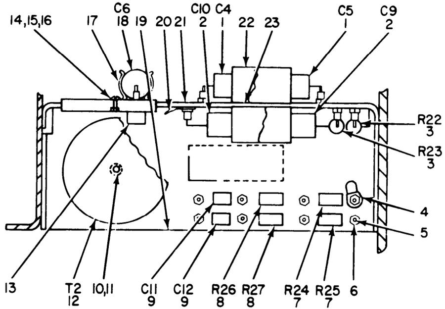
Figure 8. Test Set, Electronic Circuit Plug-In UniSAT AN/ARM-87, Transformer Bracket Assembly.
