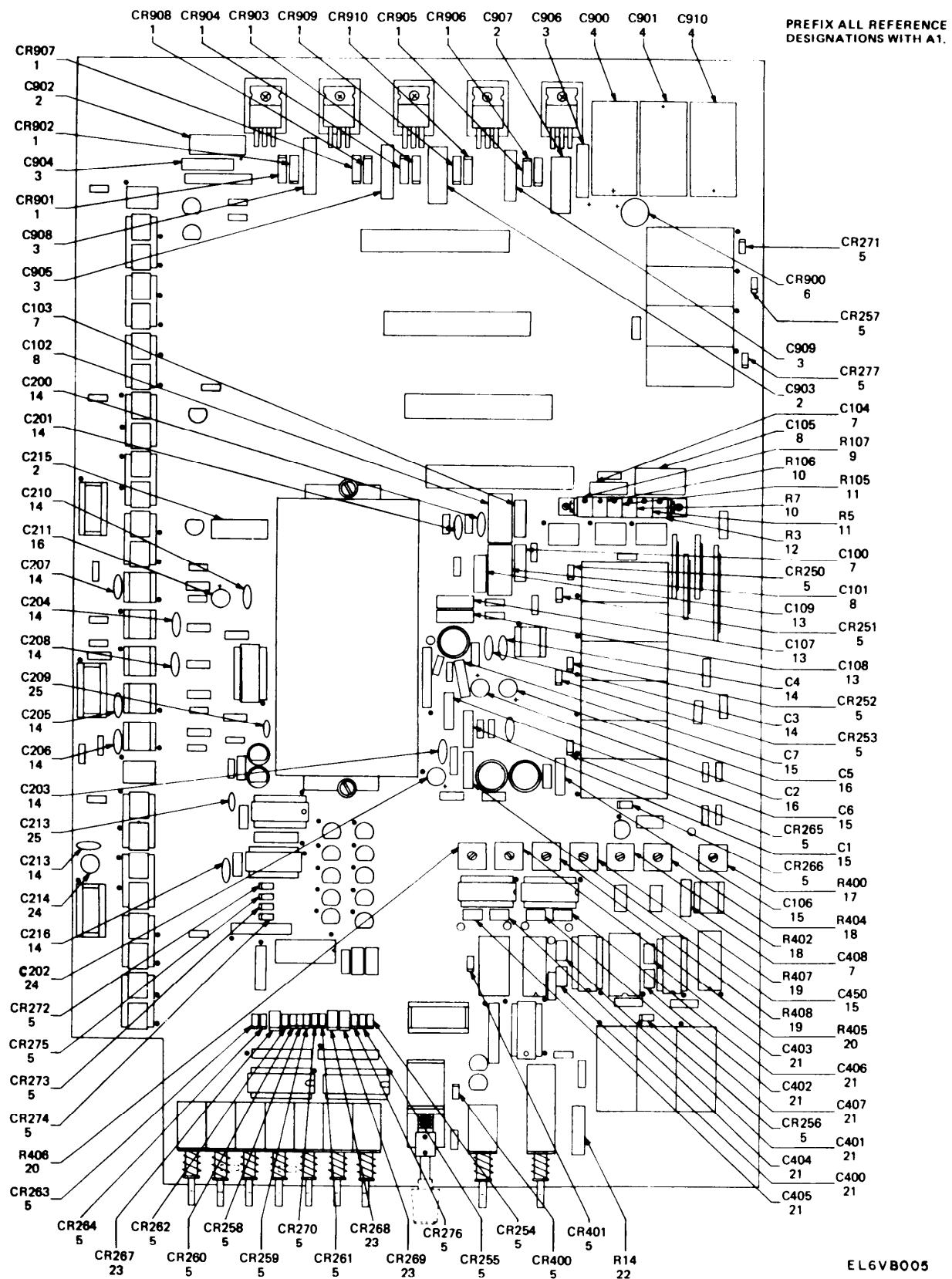
Figure 3. PCB, Analog Motherboard (Sheet 1 of 3).
