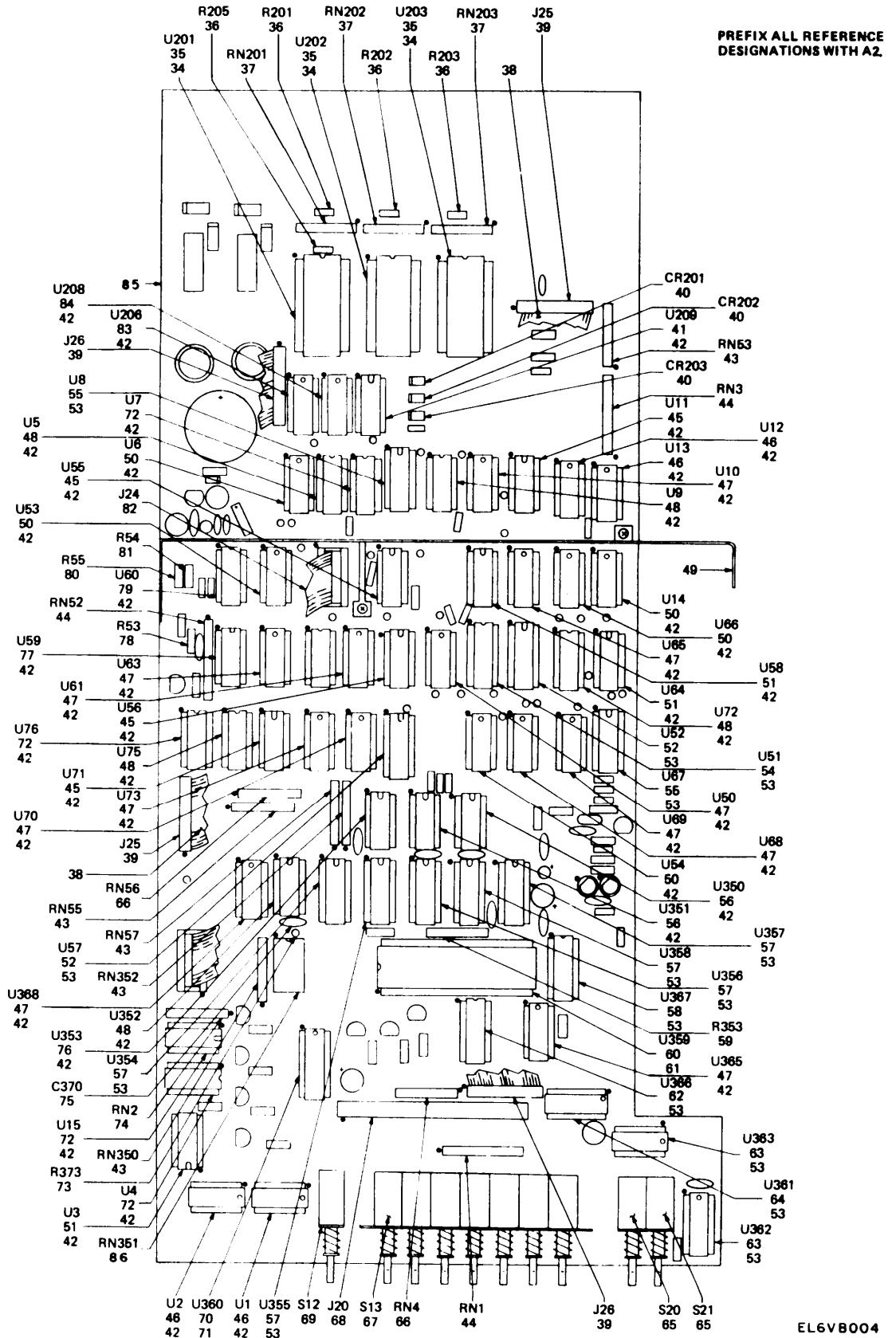
Figure 2. PCB, Digital Motherboard (Sheet 2 of 2).
