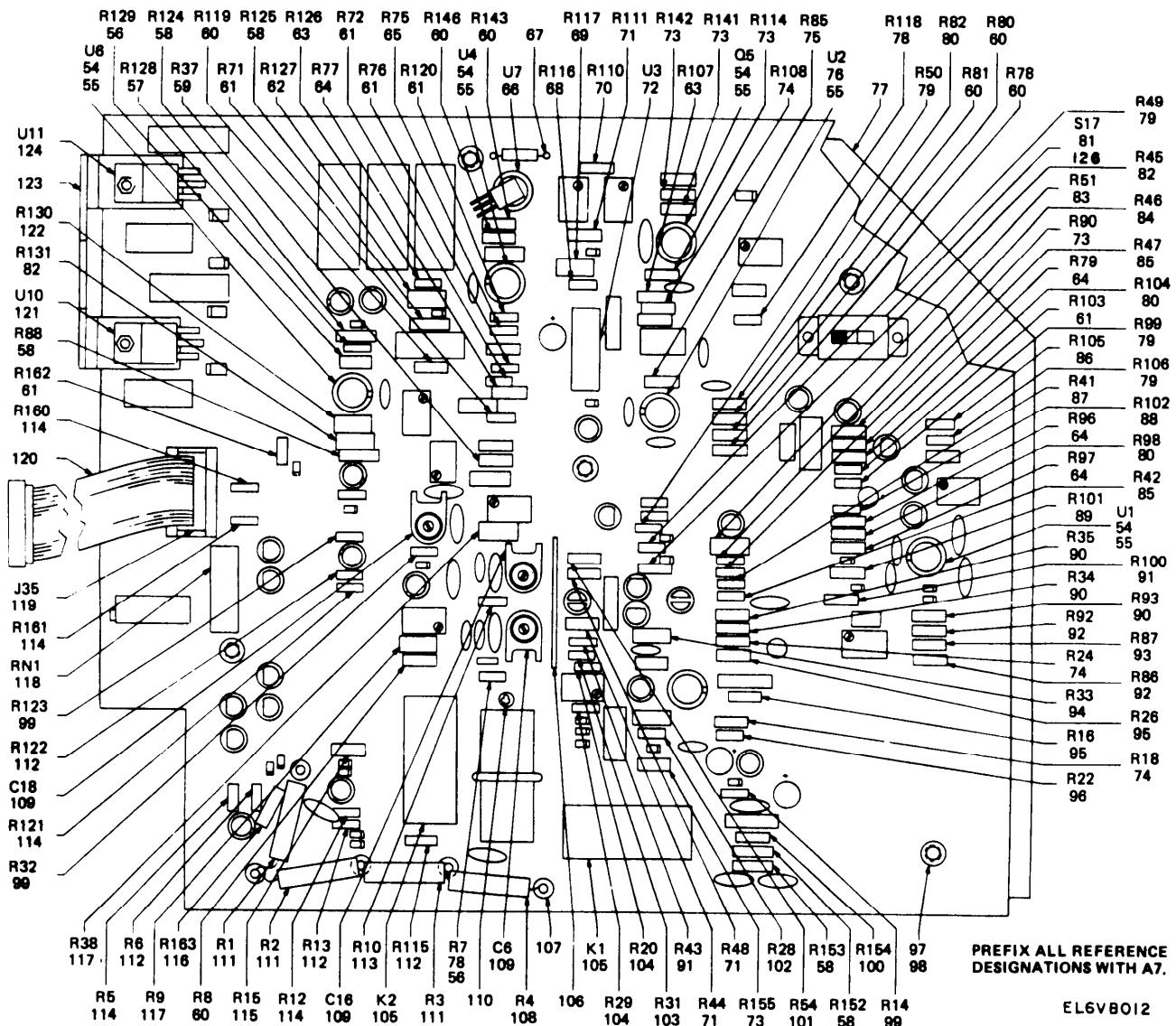
Figure 6. PCB, Ac to Dc Converter (Sheet 2 of 2).
