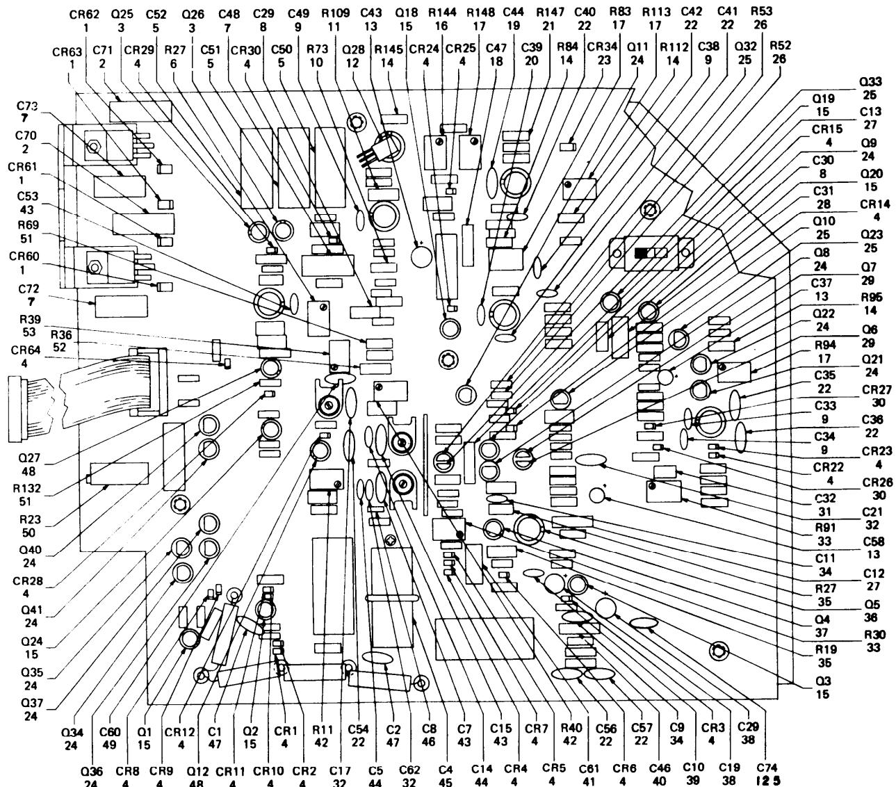
Figure 6. PCB, Ac to Dc Converter (Sheet 1 of 2).
