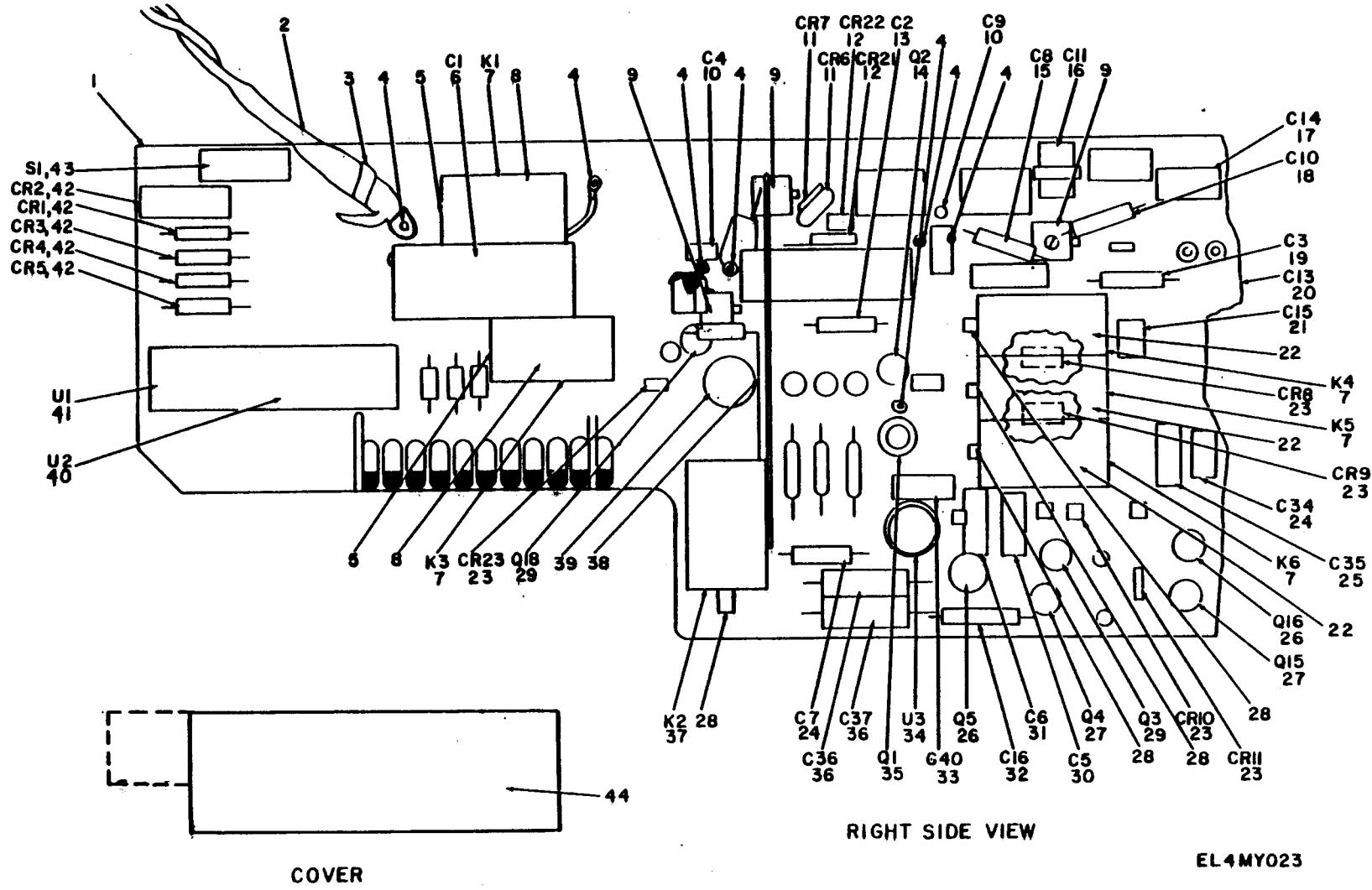
Figure 15. Plug-In, Electronic Test Equipment PL-1370/GSM-64B (Sheet 1 of 4).
