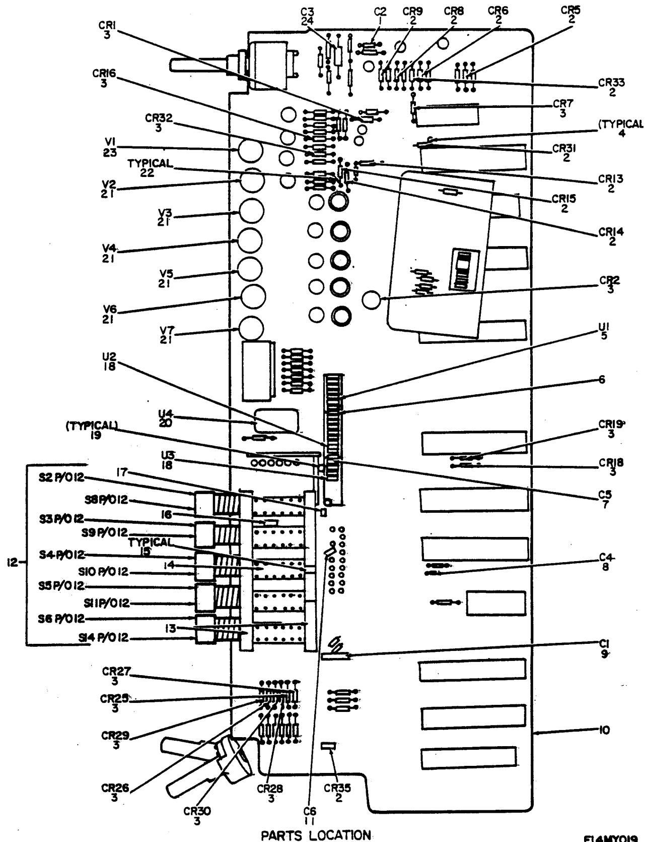
Figure 13. Display Assembly (Sheet 1 of 3).
