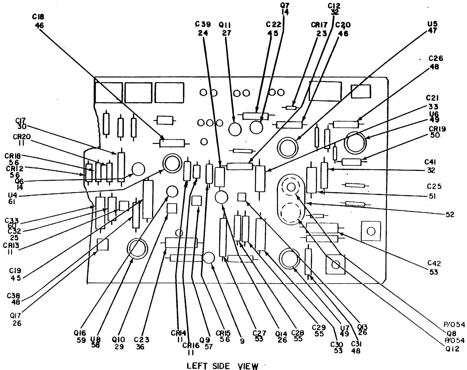
Figure 15. Plug-In, Electronic Test Equipment PL-1370/GSM-64B (Sheet 2 of 4).
