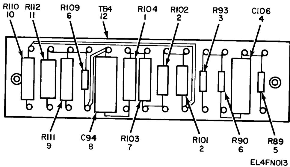
Figure 14. Meter, Modulation ME-57/U, Terminal Board Assembly (A6).
