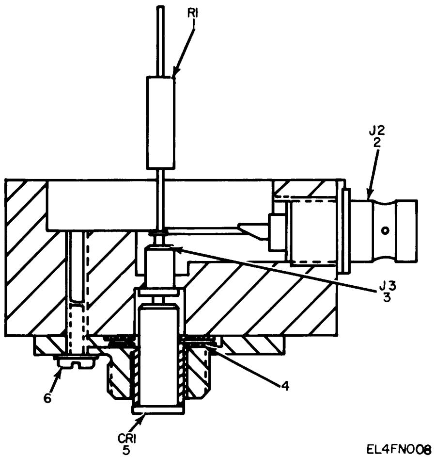
Figure 7. Meter, Modulation ME-57/U, Mixer Assembly.
