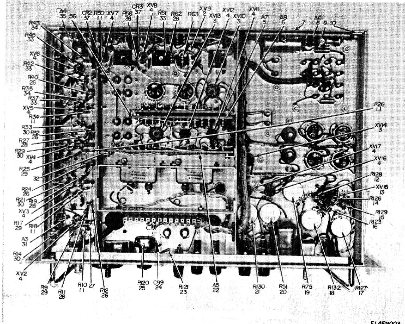
Figure 3. Meter, Modulation ME-57/U, Bottom Resistor Location.
