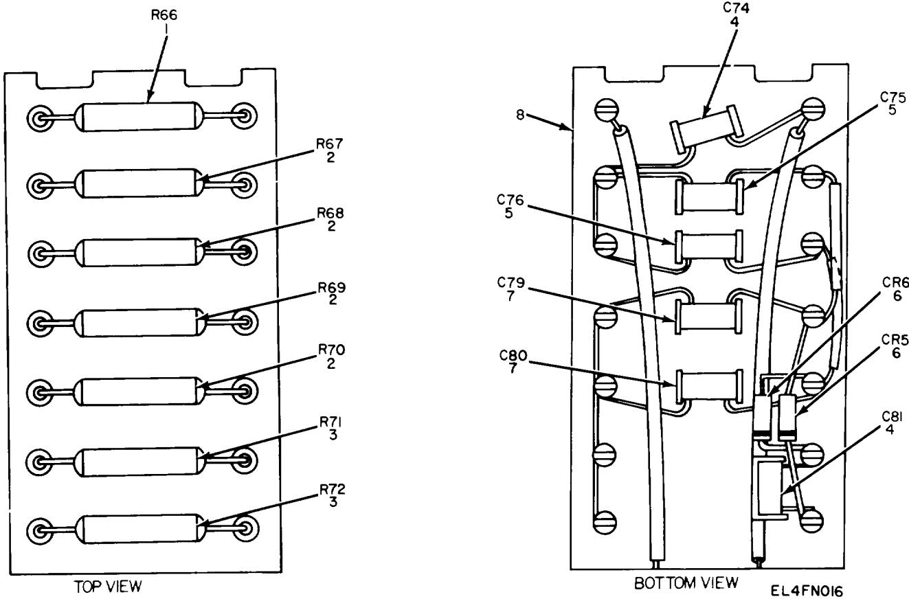
Figure 10. Meter, Modulation ME-57/U, Discriminator Terminal Board.
