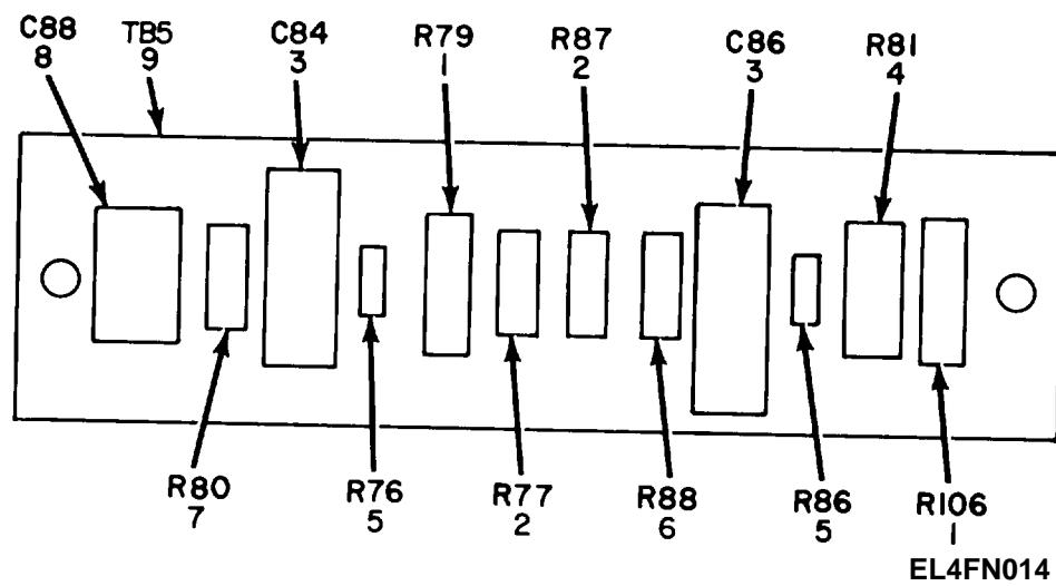
Figure 15. Meter, Modulation ME-57/U, Terminal Board Assembly (A7).
