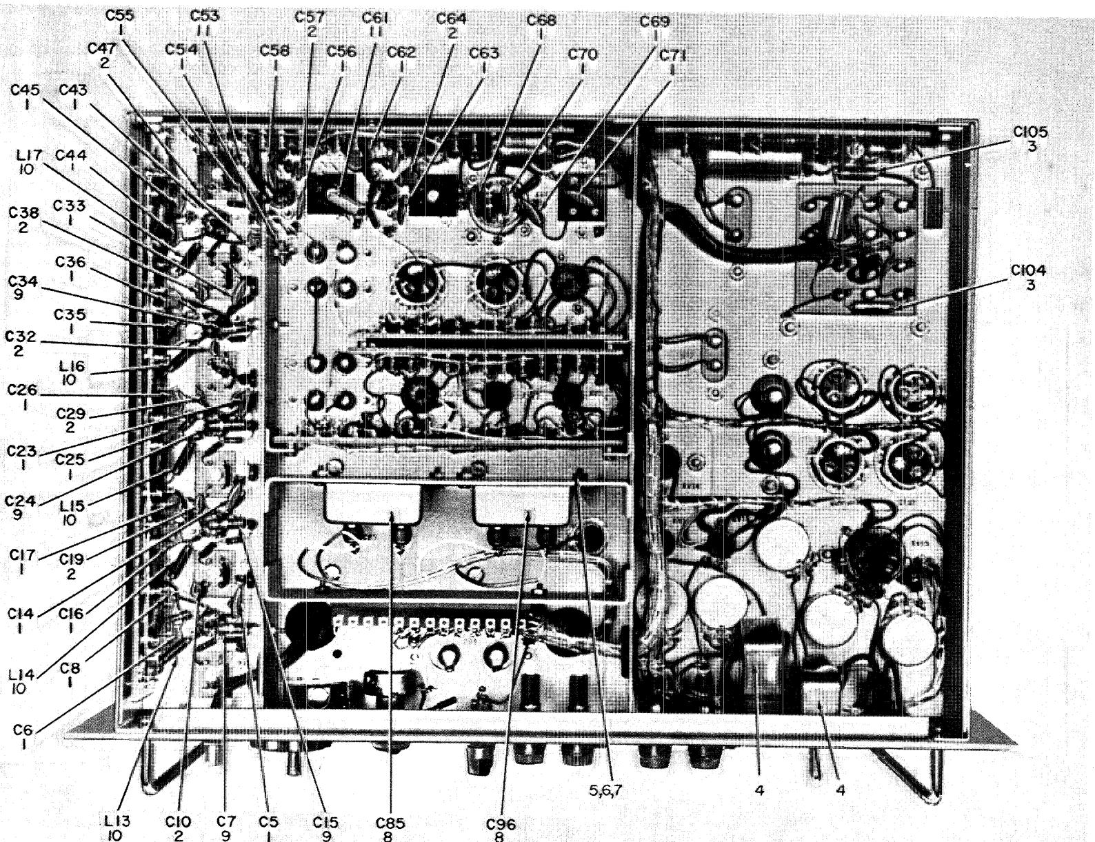
Figure 4. Meter, Modulation ME-57/U, Inductors and Capacitors Location.
