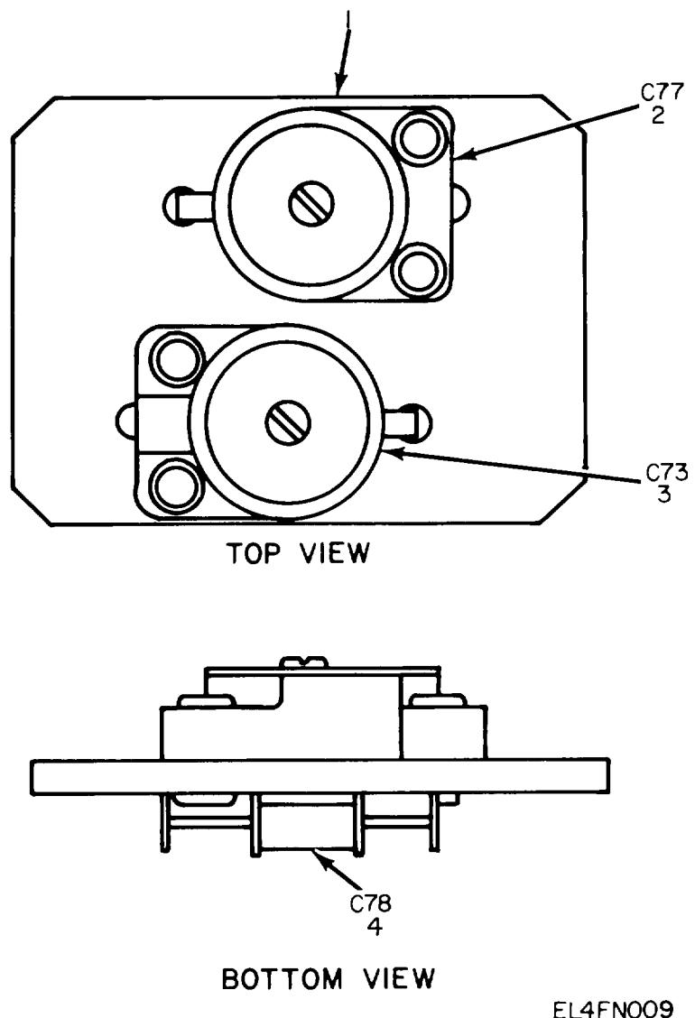
Figure 9. Meter, Modulation ME-57/U, Discriminator Board Cap Assembly.
