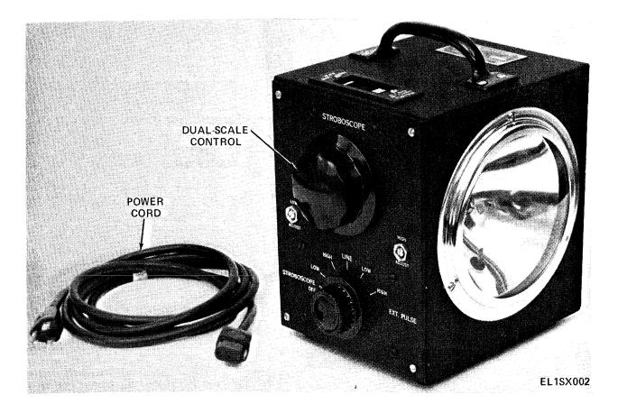
Figure 1-2, Stroboscope TS-805B/U, front view.
