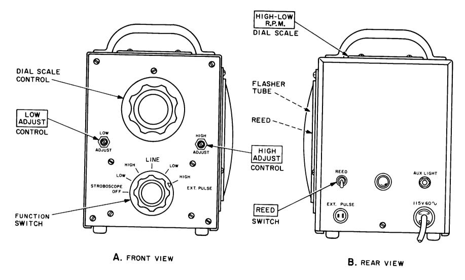
Figure 3-3. Stroboscope TS-805D/U operating controls, indicators, and connectors.
